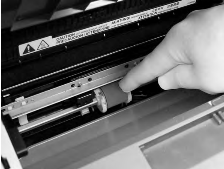
Figure 5-31 Remove the pickup roller (5 of 5)
