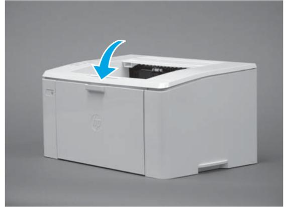
4. **M129/M134 only:** Lower the integrated scanner assembly (ISA) or the image scanner (IS).
