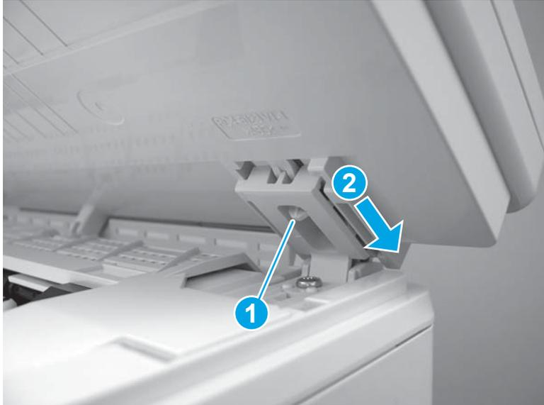
4. Rotate the ISA or IS towards the rear of the printer (callout 1), and then slide the ISA or IS toward the right side of the printer to release the left hinge (callout 2).
