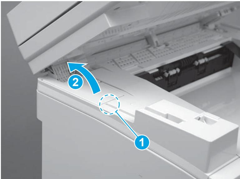
**Step 3: Remove the integrated scanner assembly (ISA) (MFP)**
