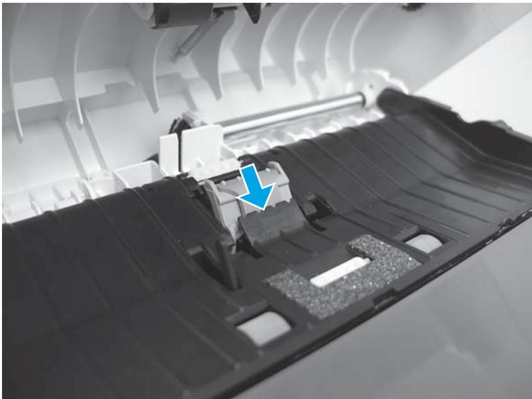
2. Push down on the separation pad to engage the pins on the assembly with the slots in the core assembly (callout 1), and then slide the separation pad toward the top cover (callout 2) to install it.
