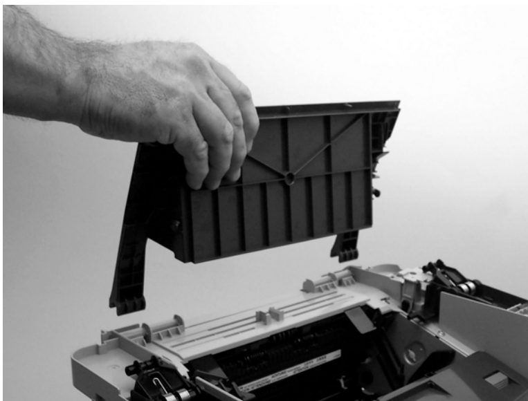
Figure 6-39 Remove the print-cartridge door (2 of 2)
