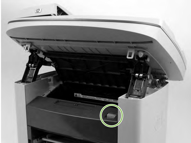
Figure 6-21 Remove the print cartridge (1 of 2)
