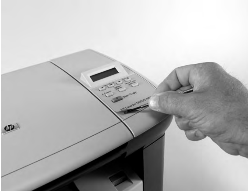
Figure 6-3 Remove the control-panel overlay
