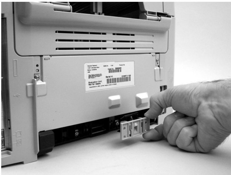
Figure 6-20 Remove the device separation pad (2 of 2)
