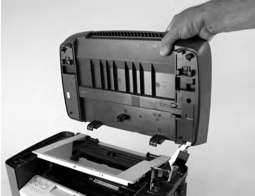
Figure 6-18 Remove the scanner assembly (11 of 11)
