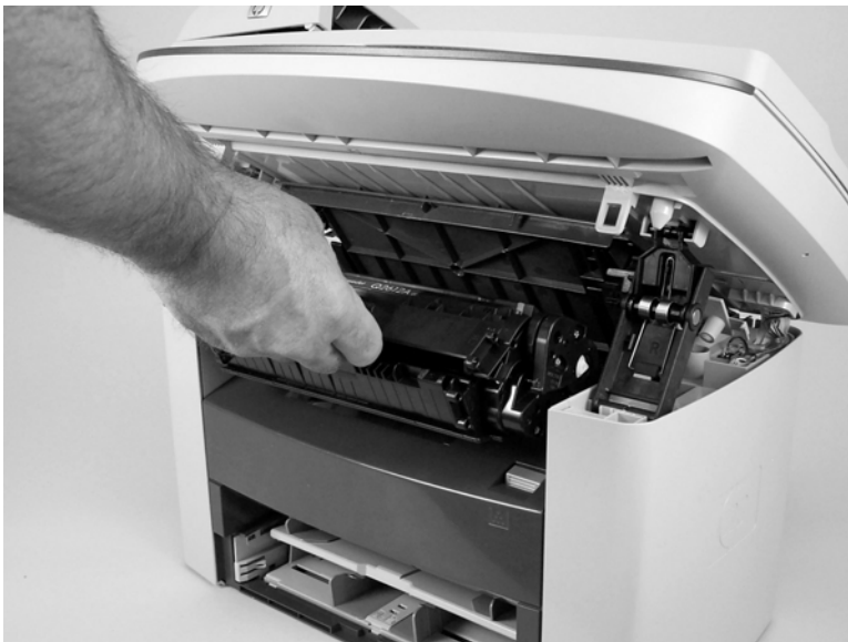
Figure 6-22 Remove the print cartridge (2 of 2)
