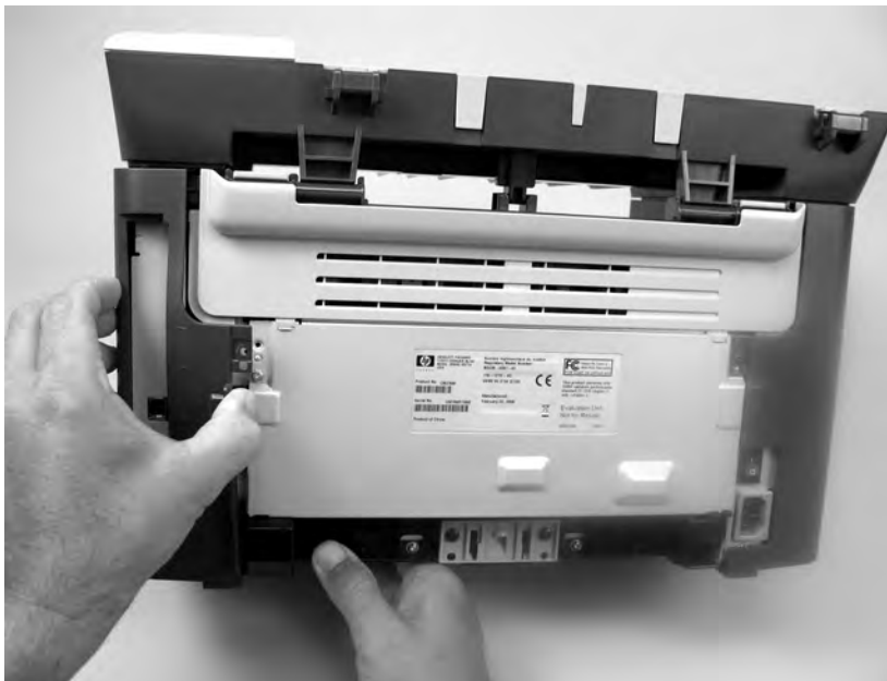
Figure 6-9 Remove the scanner assembly (2 of 11)
