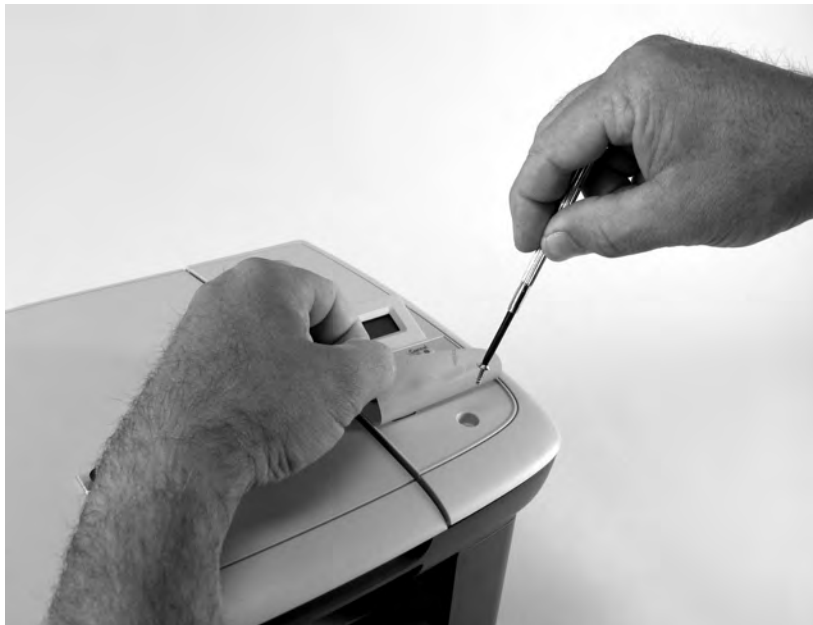
Figure 6-5 Remove the control panel (2 of 4)
