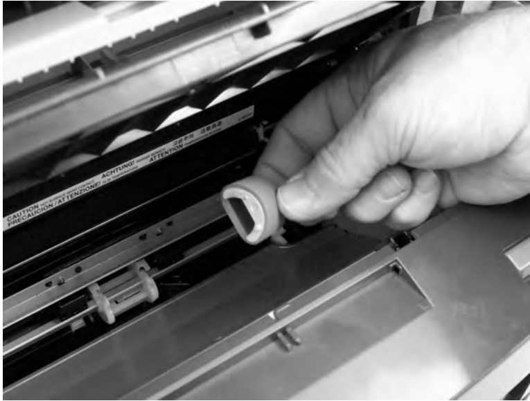
Figure 6-25 Remove the device pickup roller (3 of 5)
