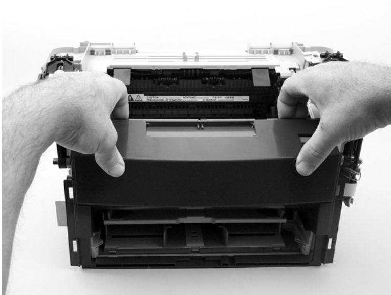
Figure 6-45 Remove the front cover (3 of 3)
