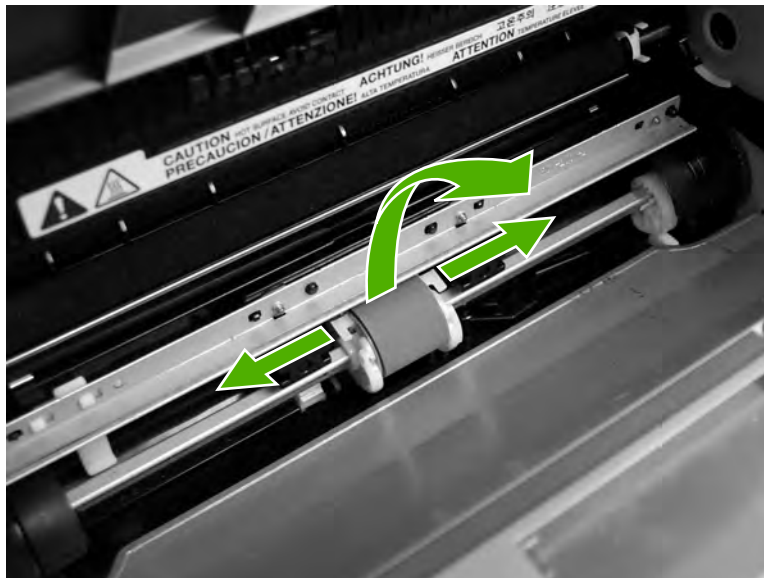
Figure 6-24 Remove the device pickup roller (2 of 5)
