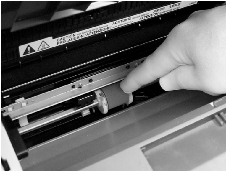
Figure 6-27 Remove the device pickup roller (5 of 5)
