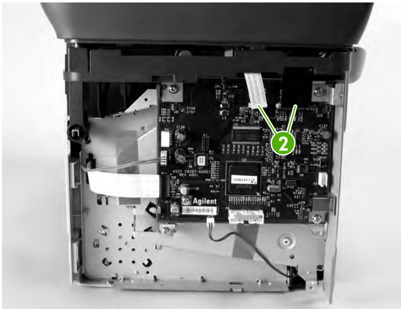
Figure 6-11 Remove the scanner assembly (4 of 11)
