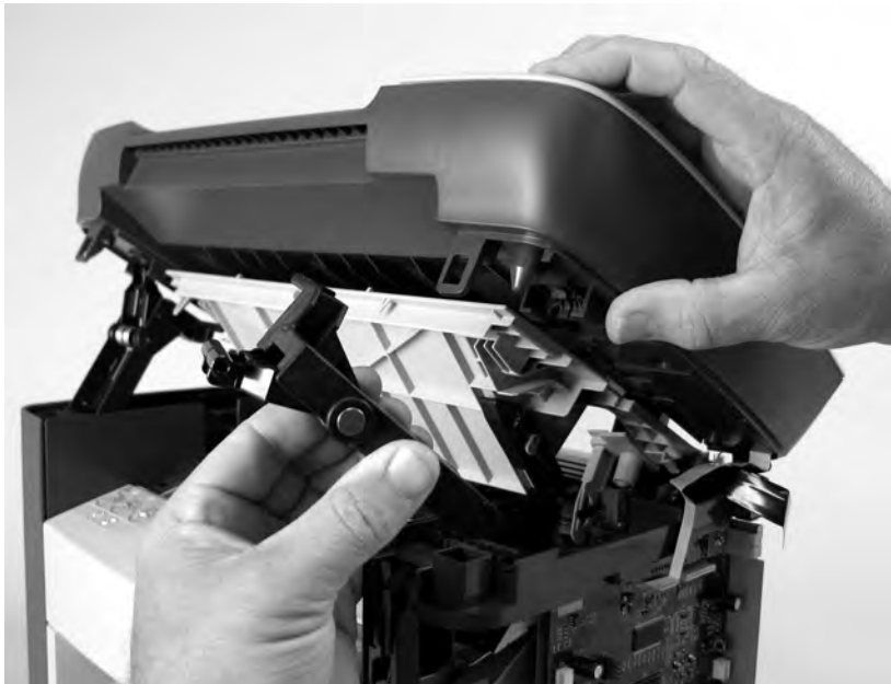
Figure 6-17 Remove the scanner assembly (10 of 11)
