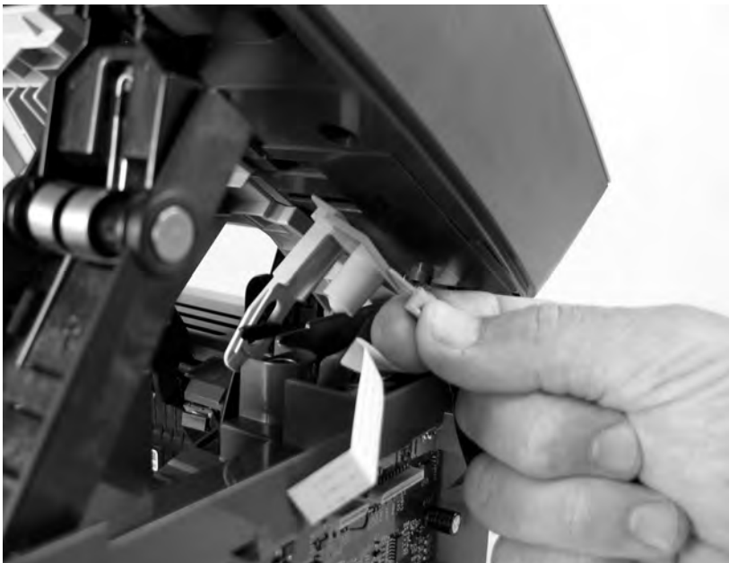
Figure 6-15 Remove the scanner assembly (8 of 11)
