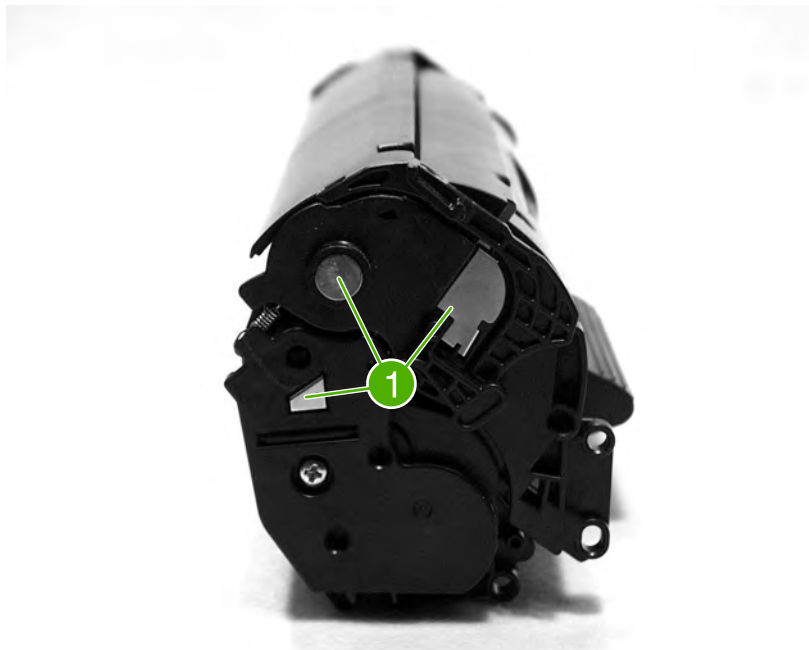
Figure 7-7 Print-cartridge high-voltage contacts
