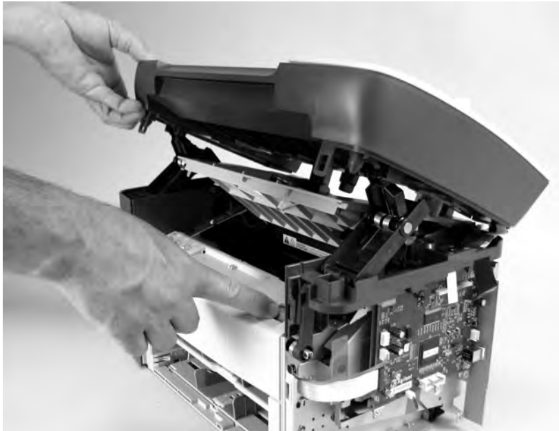
Figure 6-12 Remove the scanner assembly (5 of 11)
