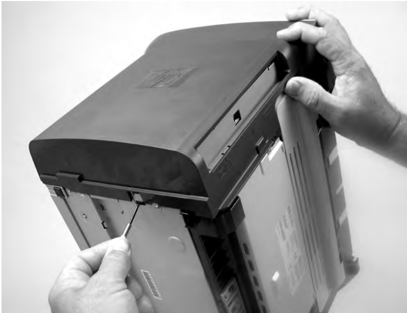
Figure 6-10 Remove the scanner assembly (3 of 11)
