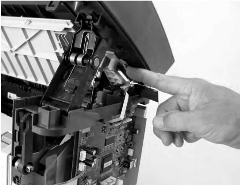
Figure 6-14 Remove the scanner assembly (7 of 11)
