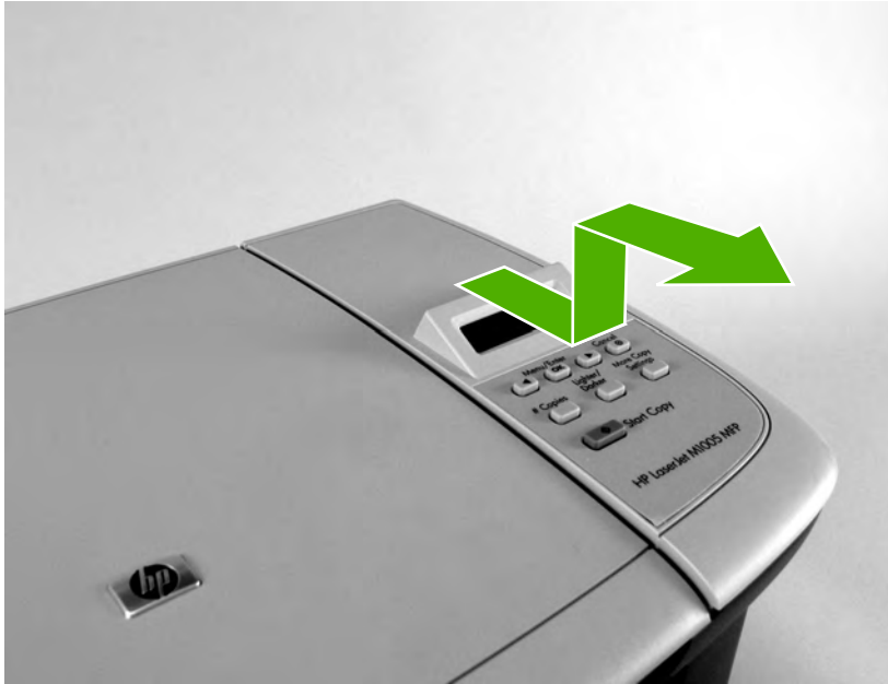
Figure 6-6 Remove the control panel (3 of 4)
