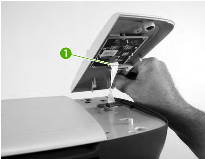
Figure 6-7 Remove the control panel (4 of 4)
