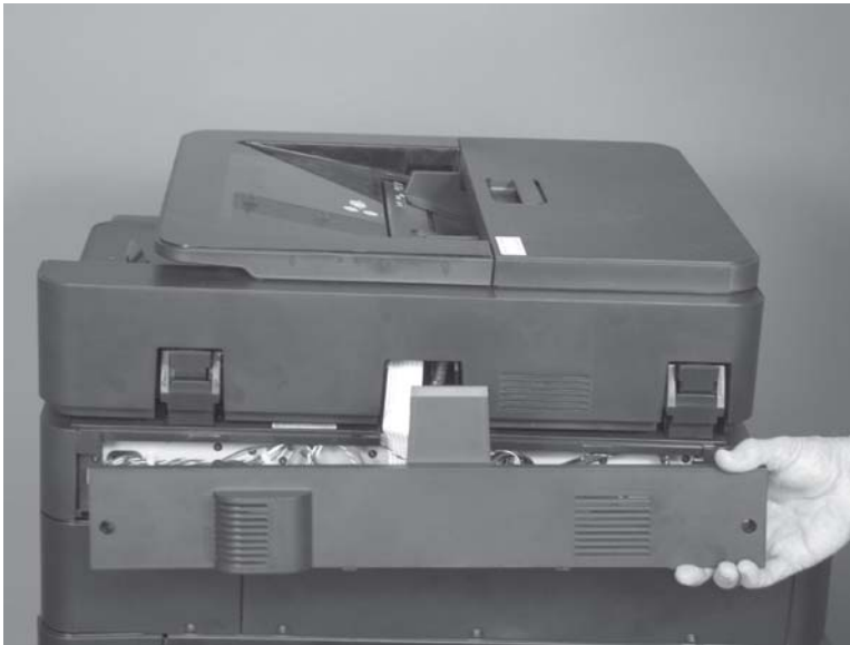
Figure 1-115 Remove the scanner back cover (M880; 2 of 2)
