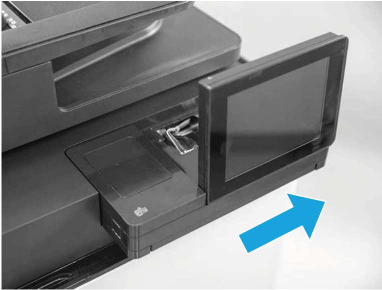
Figure 1-66 Remove the control panel assembly (M880; 7 of 8)
