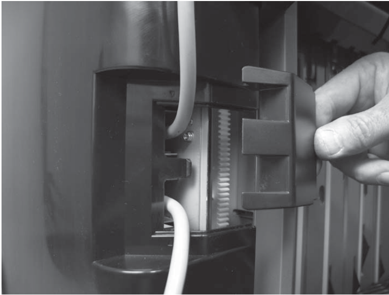
Figure 1-732 Remove the bin cable guide cover (5 of 6)
