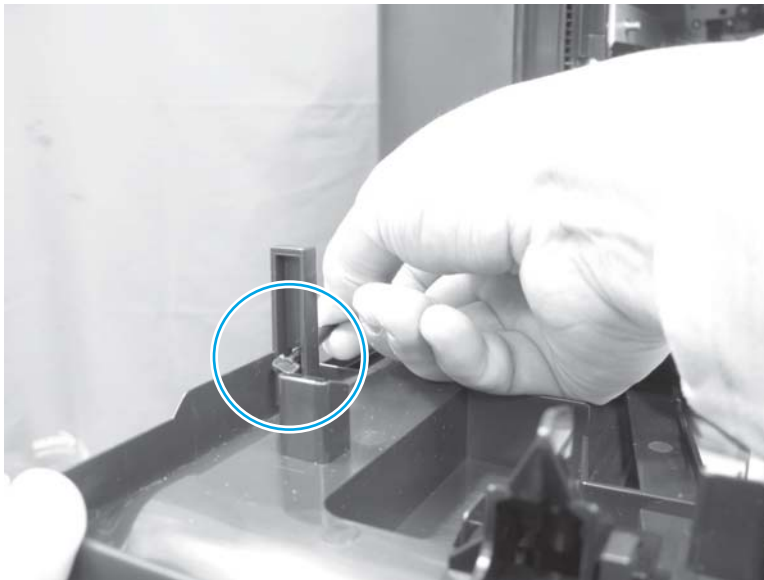
Figure 1-187 Remove the left front cover (1 of 5)
