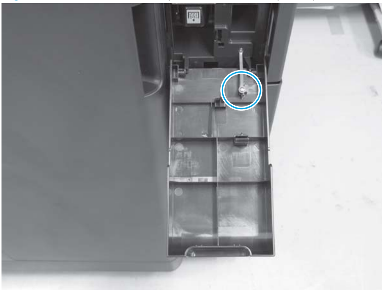
Figure 1-1025 Remove the punch front cover (1 of 2)
