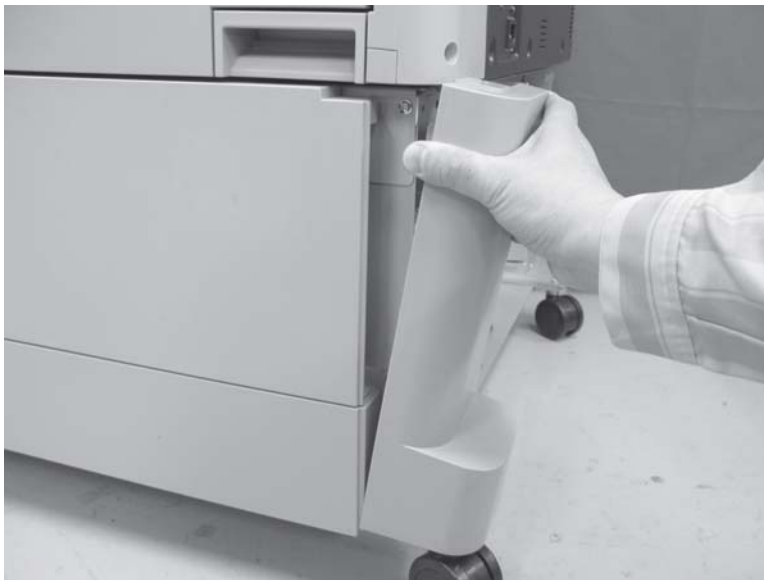
Figure 1-631 Remove the HCI, 1x500, and 3x500 right rear cover (4 of 4)
