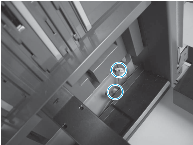
Figure 1-990 Remove the saddle assembly (1 of 13)
