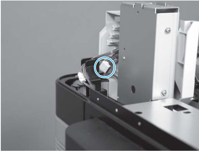
Figure 1-506 Remove the face-down delivery assembly (M880; 18 of 19)
