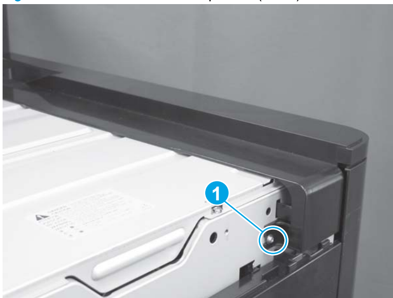
Figure 1-159 Remove the front top cover (1 of 2)
