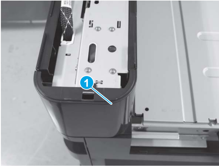
Figure 1-155 Remove the left upper rear cover and rear upper B cover (M880; 2 of 3)
