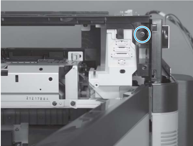
Figure 1-475 Remove the VOC fan (M880; 1 of 6)
