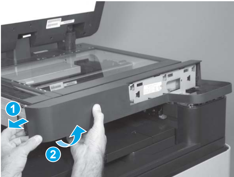
Figure 1-126 Remove the scanner front cover (M880; 7 of 8)
