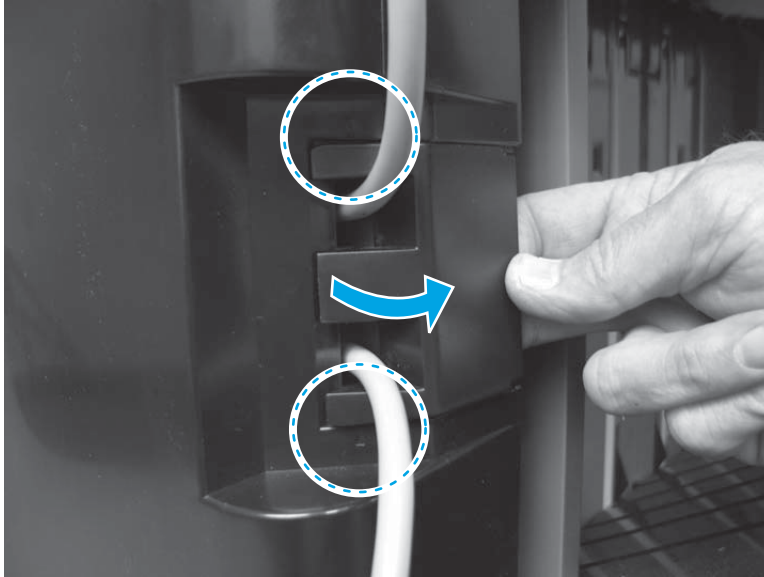
Figure 1-730 Remove the bin cable guide cover (3 of 6)
