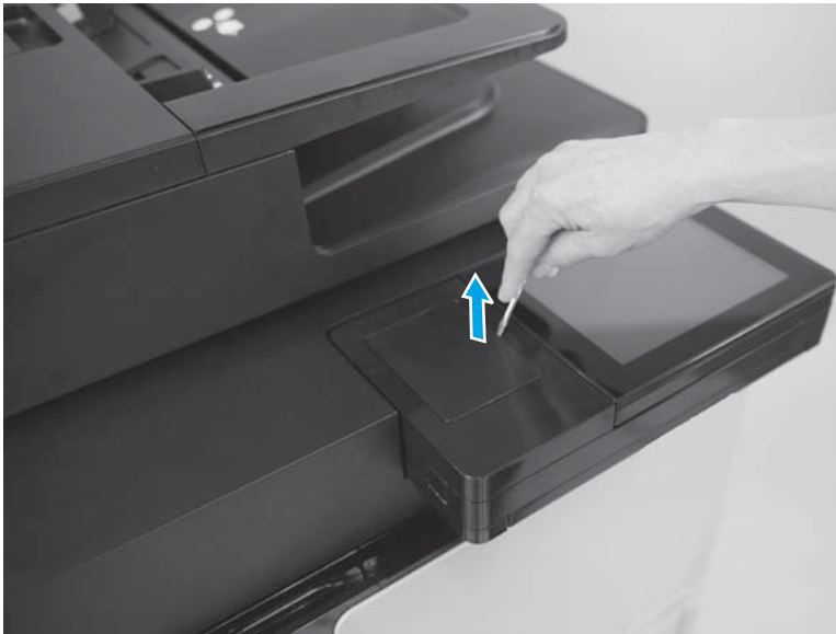
Figure 1-131 Remove the HIP cover (M880; 2 of 3)
