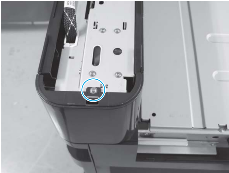
Figure 1-154 Remove the left upper rear cover and rear upper B cover (M880; 1 of 3)
