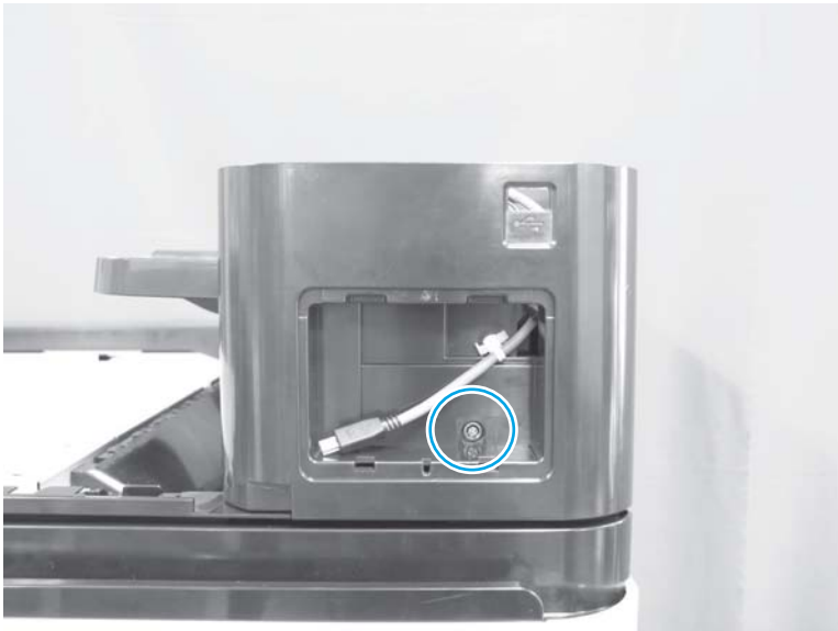
Figure 1-166 Remove the right upper front cover (M855; 1 of 2)
