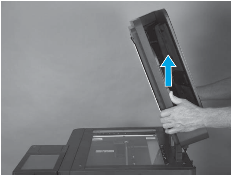
Figure 1-222 Remove the document feeder assembly (M880; 7 of 9)
