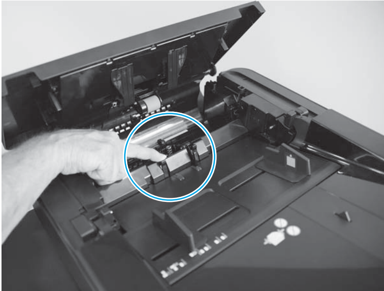
Figure 1-93 Reinstall the document-feeder separation pad (M880; 1 of 5)
