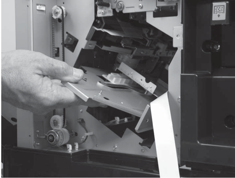
Figure 1-835 Remove the staple assembly (6 of 7)
