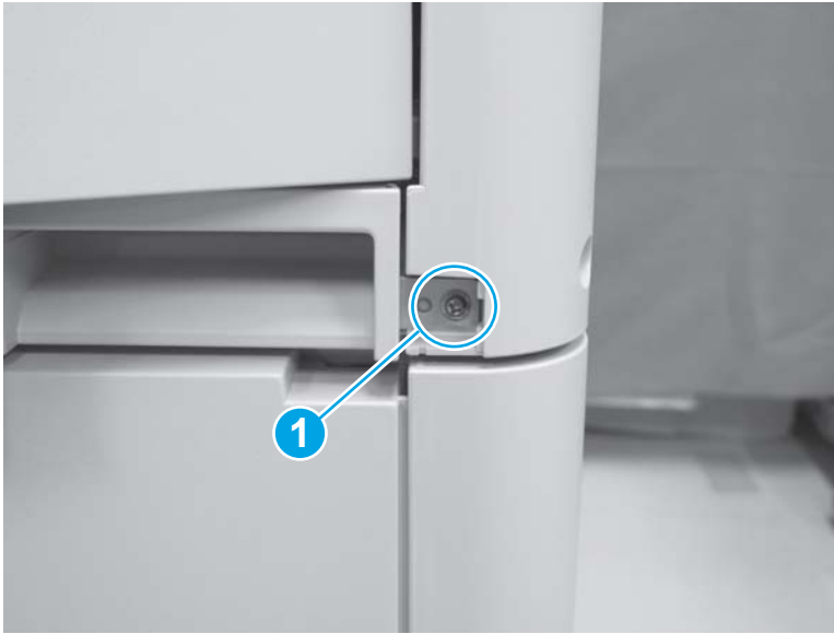
Figure 1-262 Remove the multipurpose tray (Tray 1) drive assembly (2 of 13)
