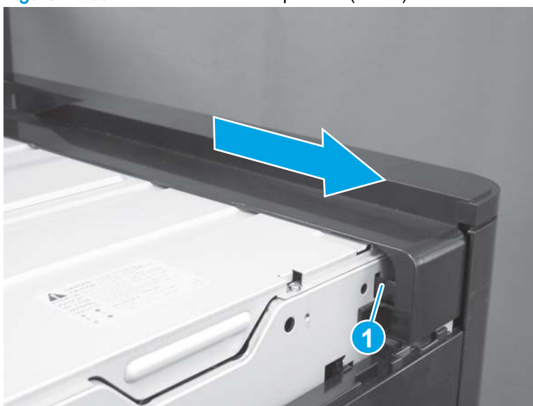
Figure 1-160 Remove the front top cover (2 of 2)
