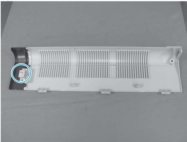
Figure 1-210 Remove the right rear cover (2 of 2)
