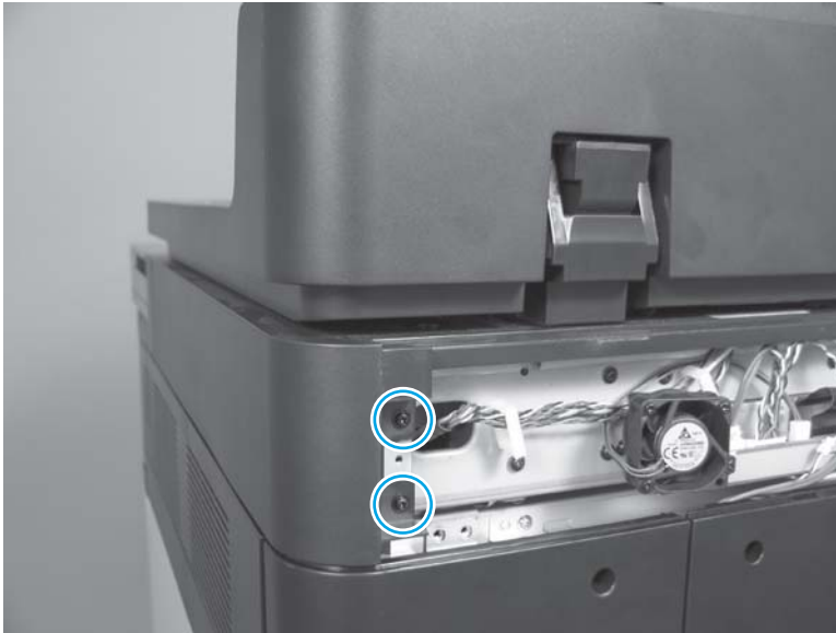
Figure 1-118 Remove the scanner right cover (M880; 1 of 2)
