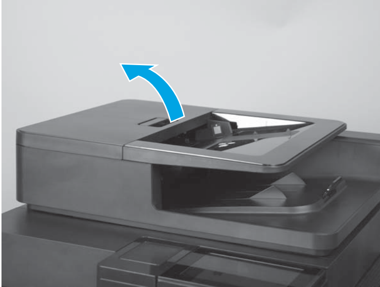
Figure 1-89 Remove the document-feeder separation pad (M880; 1 of 4)
