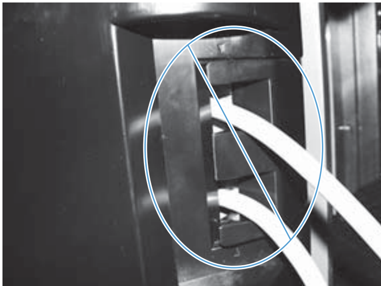
Figure 1-735 Bin cable guide cover incorrectly installed
