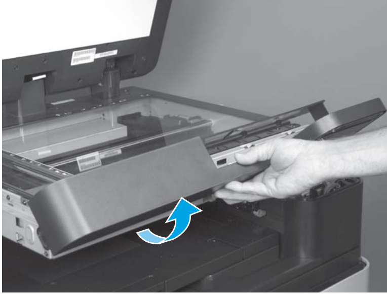
Figure 1-127 Remove the scanner front cover (M880; 8 of 8)
