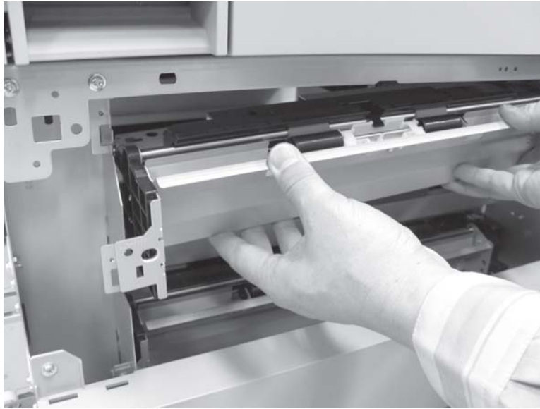
Figure 1-598 Remove the 3x500 Tray 3 pickup assembly (4 of 4)
