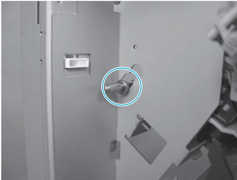
Figure 1-843 Remove the operation tray assembly (4 of 11)
