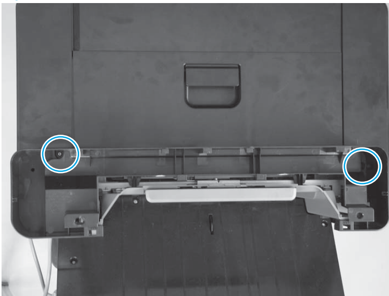
Figure 1-697 Remove the lower stepped cover assembly (1 of 5)
