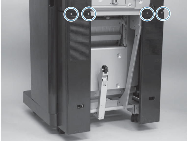
Figure 1-686 Remove the latch lower covers (front and rear; 1 of 3)
