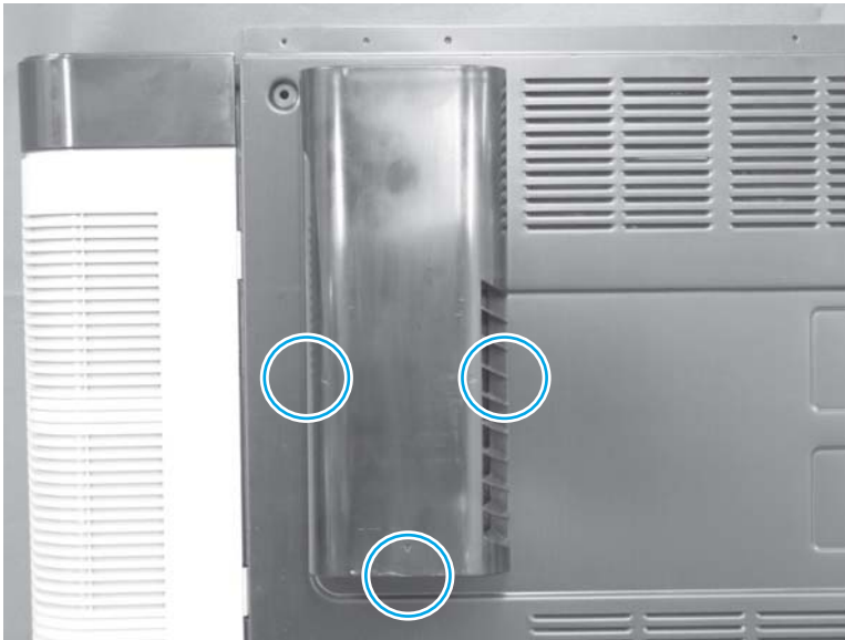
Figure 1-207 Install a replacement rear cover (1 of 2)
