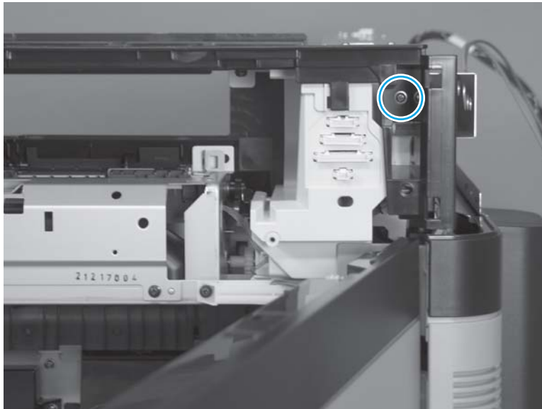
Figure 1-489 Remove the face-down delivery assembly (M880; 1 of 19)
