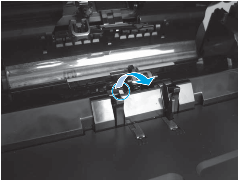
Figure 1-90 Remove the document-feeder separation pad (M880; 2 of 4)
