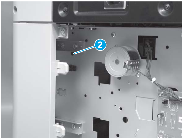
Figure 1-592 Reinstall the 1x500 Tray 3 pickup assembly (2 of 4)
