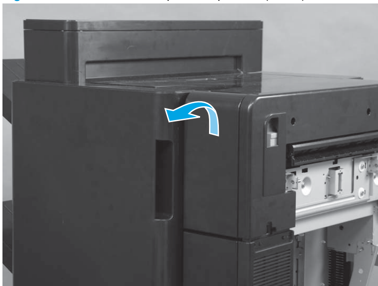
Figure 1-1039 Remove the punch top cover (2 of 6)
