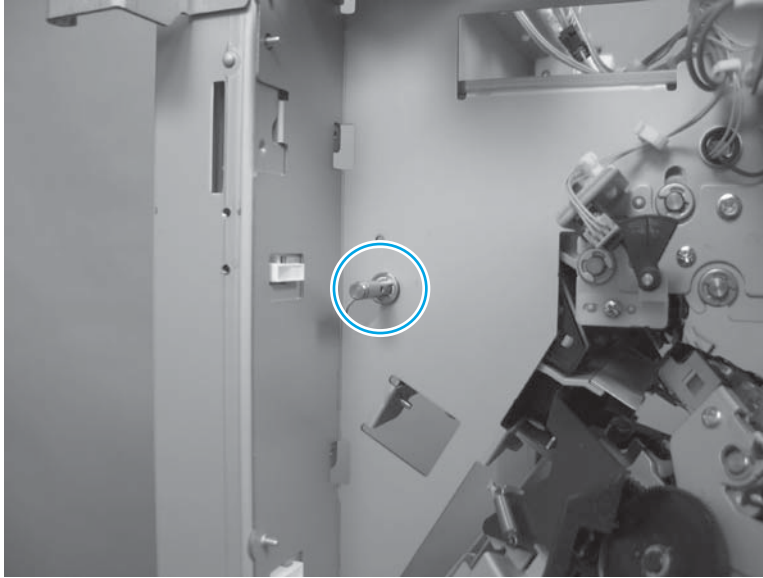
Figure 1-842 Remove the operation tray assembly (3 of 11)
