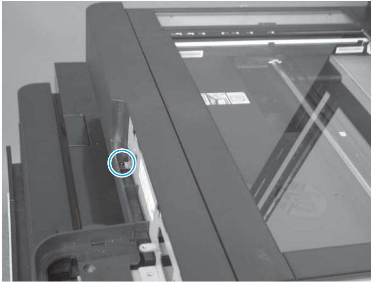
Figure 1-123 Remove the scanner front cover (M880; 4 of 8)
