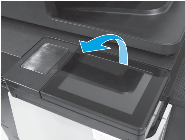
Figure 1-60 Remove the control panel assembly (M880; 1 of 8)
