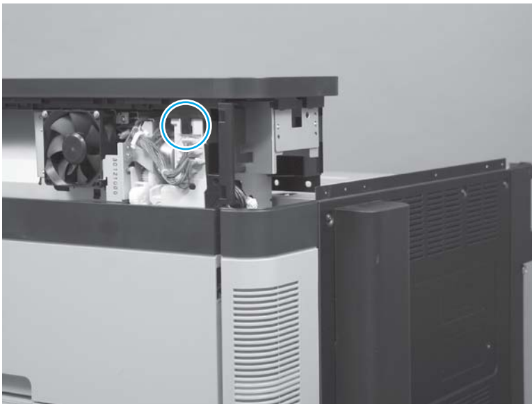
Figure 1-174 Remove the right upper cover (M855; 5 of 9)
