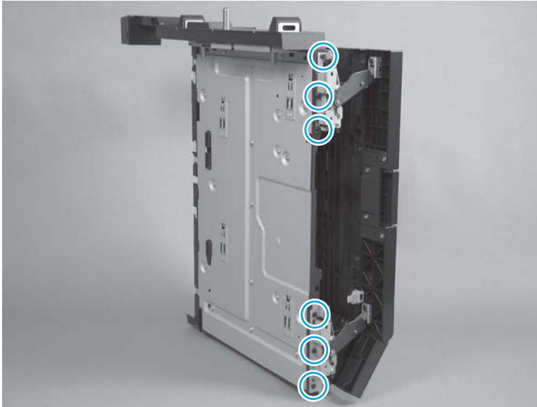
Figure 1-666 Remove the IPTU upper and lower guide assemblies (3 of 9)
