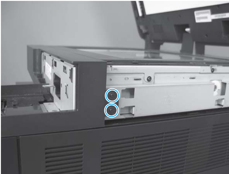
Figure 1-122 Remove the scanner front cover (M880; 3 of 8)
