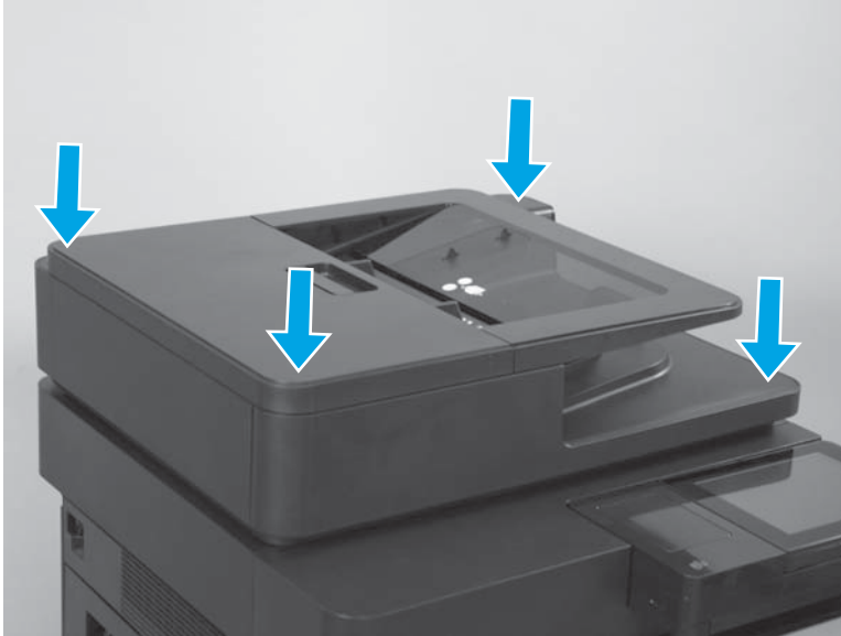
Figure 1-41 Install a replacement document feeder white backing (M880; 4 of 6)
