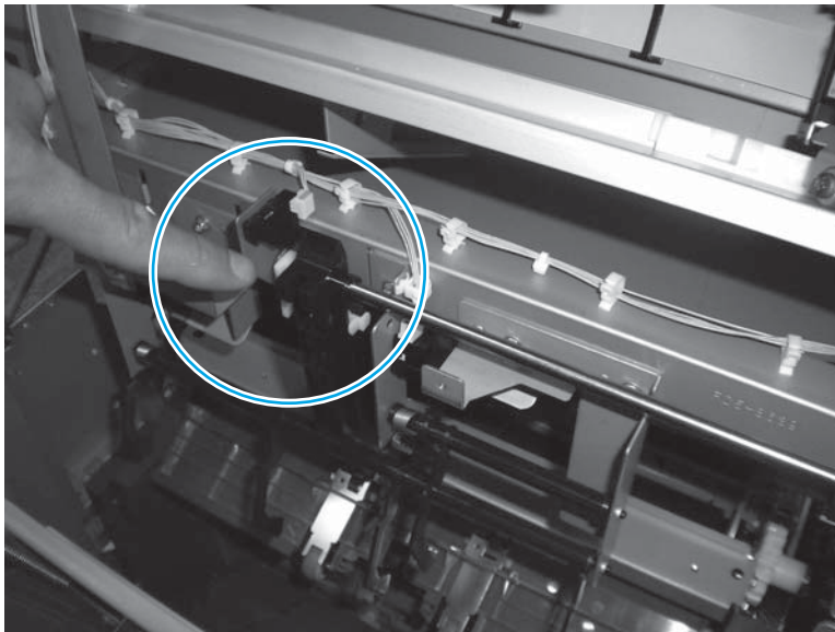
Figure 1-812 Reinstall the height wall assembly
