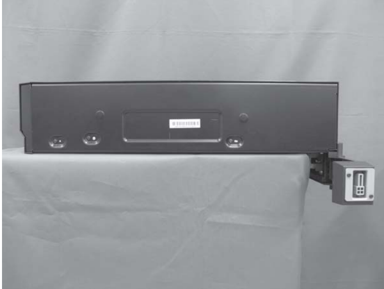
Figure 1-634 Incorrect placement of the IPTU for servicing
