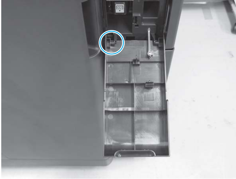
Figure 1-1026 Remove the punch front cover (2 of 2)
