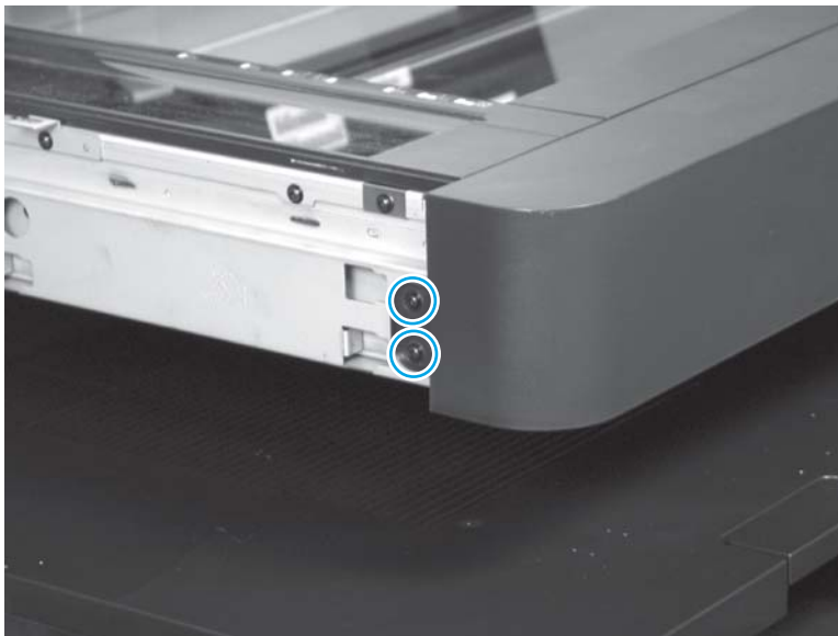
Figure 1-124 Remove the scanner front cover (M880; 5 of 8)
