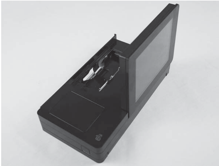
Figure 1-71 Remove the keyboard assembly (M880; 1 of 7)
