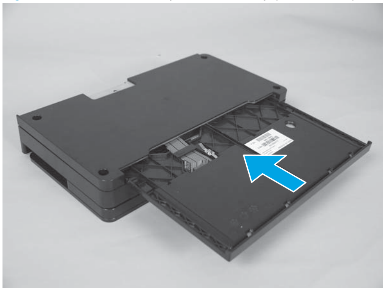
Figure 1-79 Reinstall the keyboard assembly (M880; 2 of 7)
