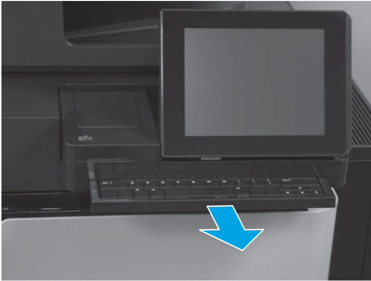
Figure 1-62 Remove the control panel assembly (M880; 3 of 8)
