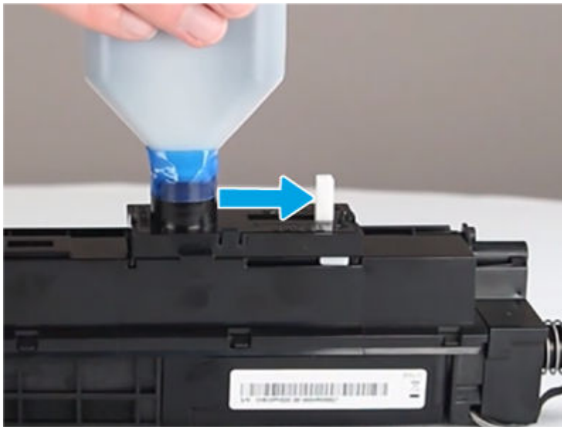
Figure 6-955 Open the shutter
