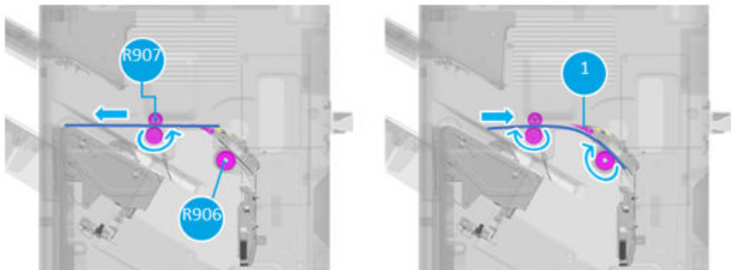
Figure 3-318 Buffer unit operation, view 5
