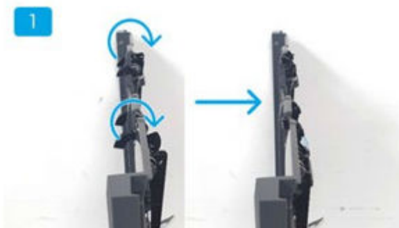
Figure 3-306 Paper holding unit operation, view 1
