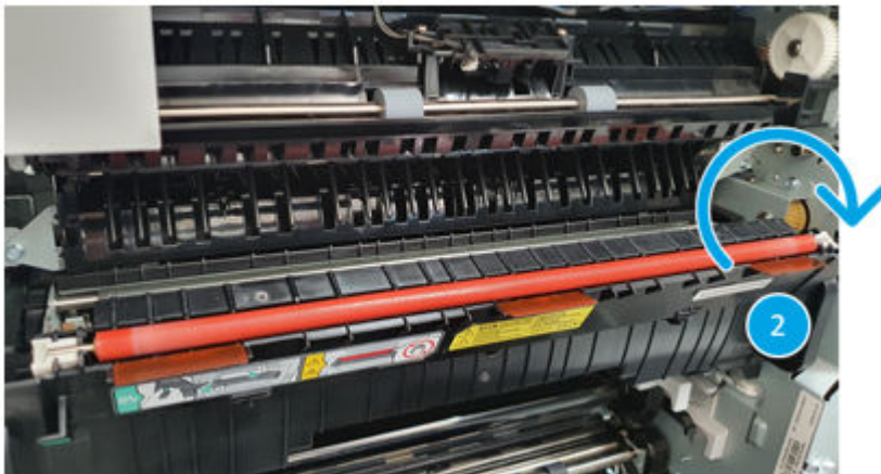
Figure 3-82 Fuser gap sensor operation, view 2
