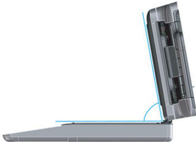
Figure 3-142 Document feeder open (maximum 65°)
