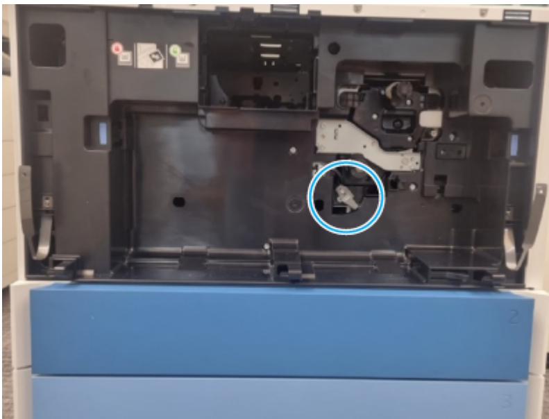
Figure 6-913 Avoid damaging the drum engage lever
