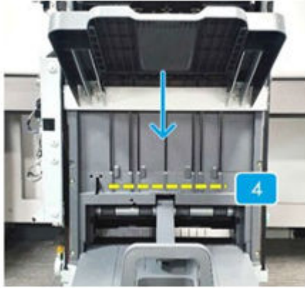
Figure 3-309 Paper holding unit operation, view 4
