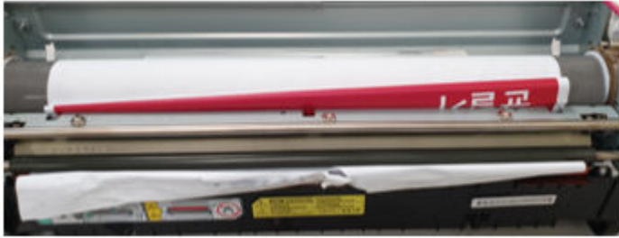
Figure 3-83 Wrap jam in the fuser unit
