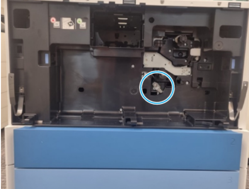
Figure 6-1038 Avoid damaging the drum engage lever
