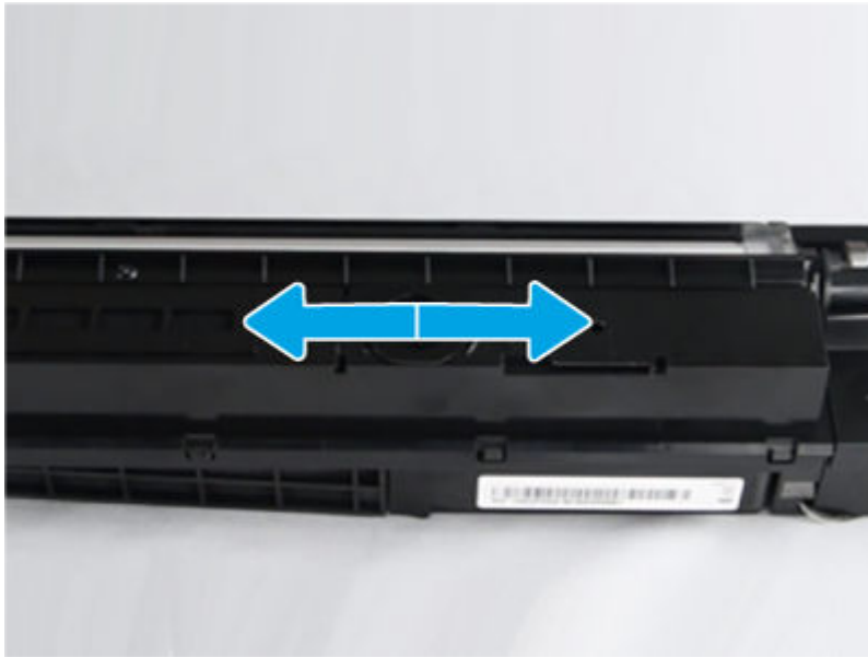
Figure 6-959 Distribute the toner powder
