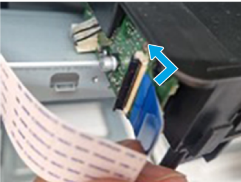
Figure 6-868 Locking clip open
