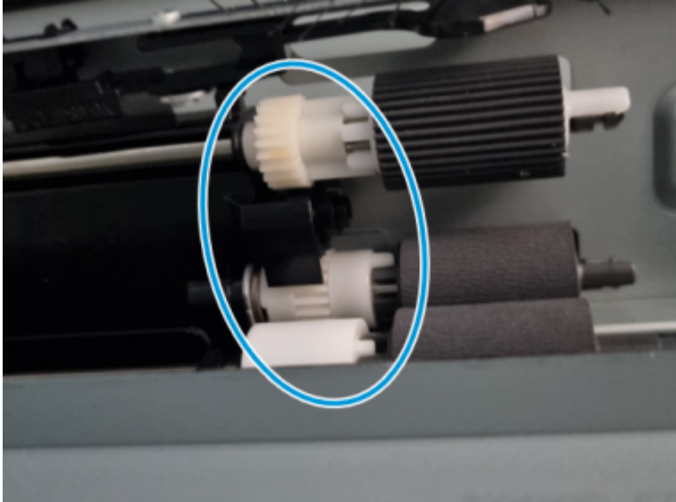
Figure 6-327 Rollers and couplers installed
