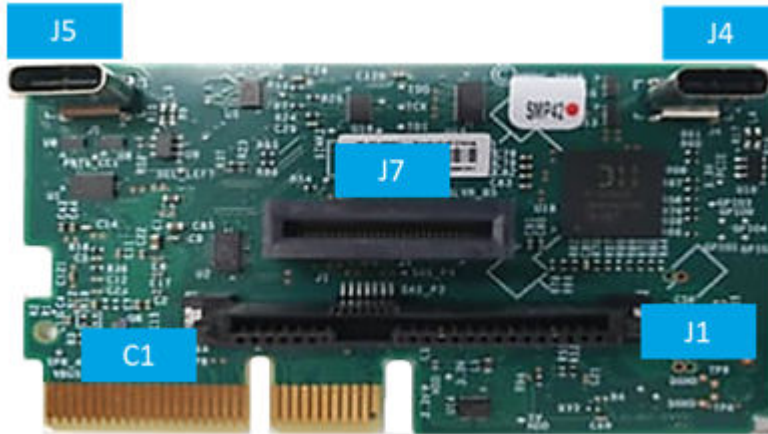
Figure 3-95 Riser card for HDD, two USB Type C ports, and accelerator board
