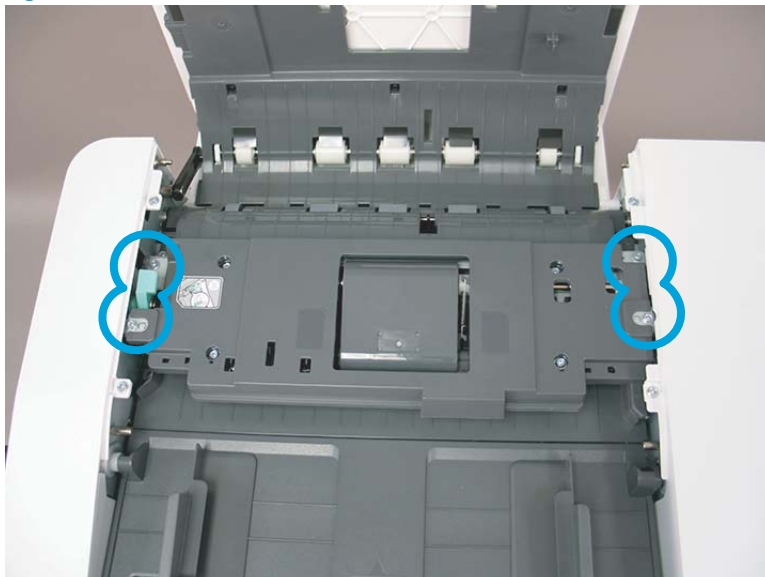
Figure 2-800 Remove four screws.
