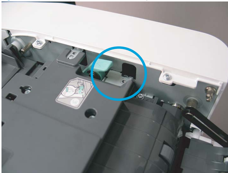
Figure 2-804 Rotate pick/feed roller assembly to release sheet metal tab from ADF frame.
