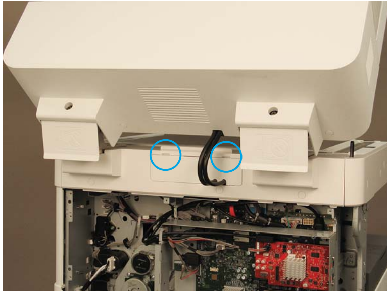
Figure 2-902 Remove document feeder connector cover
