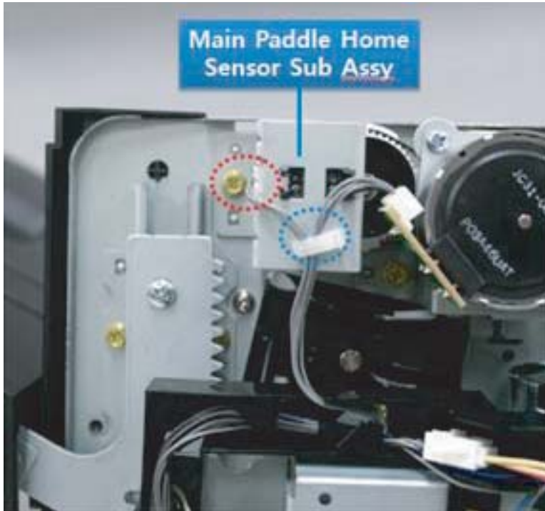
Figure 6-203 Remove the main paddle home sensor sub assembly
