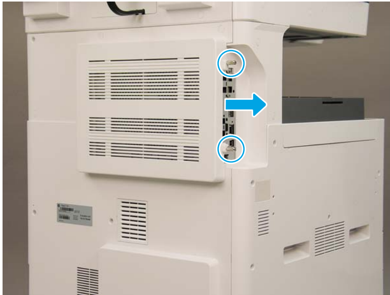
Figure 2-150 Remove the formatter cover
