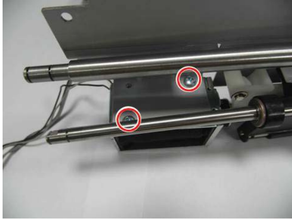
Figure 2-657 Remove two screws
