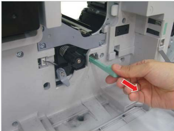
Figure 2-455 Remove the paper dust brush
