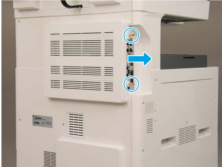
Figure 2-384 Remove the formatter cover
