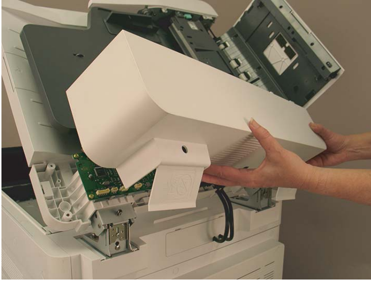
Figure 2-843 Remove back cover.
