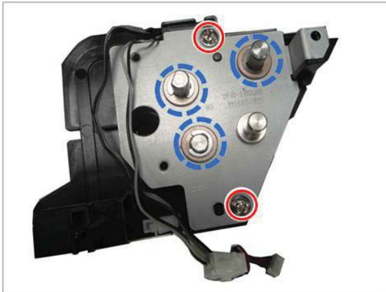
Figure 2-655 Remove the bracket-rear
