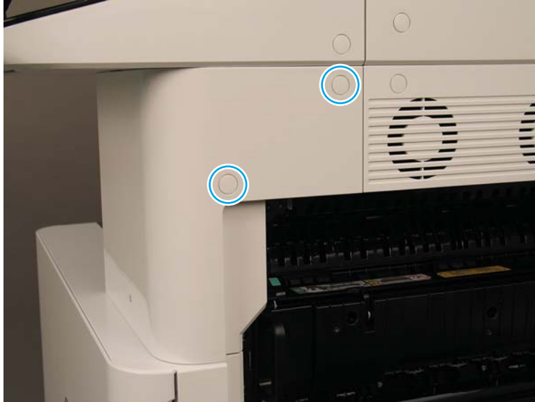
Figure 2-216 Remove two screws and rotate the cover
