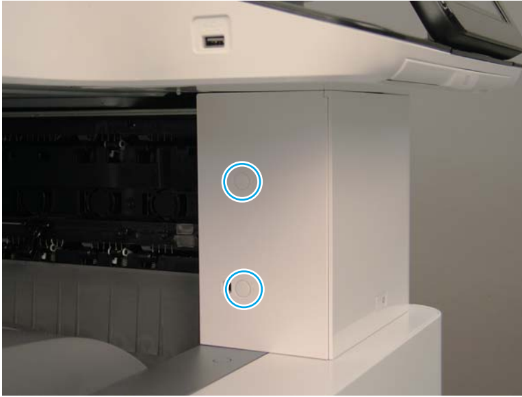
Figure 2-18 Remove the front top inner cover
