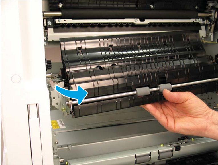
Figure 2-113 Rotate pickup unit 1
