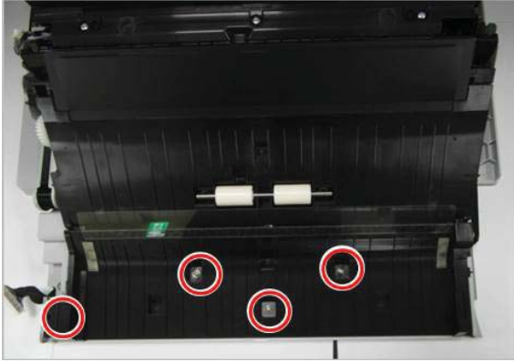
Figure 2-587 Remove four screws
