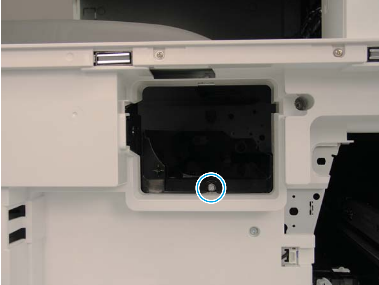
Figure 2-226 Remove one screw
