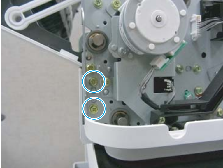
Figure 2-864 Remove two screws
