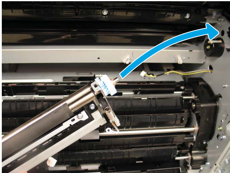
Figure 2-445 Install the gear side of the shaft
