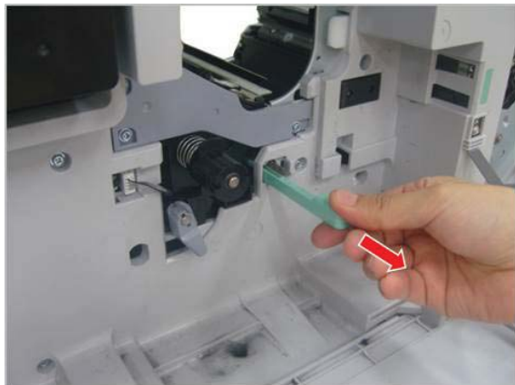
Figure 2-57 Remove the paper dust brush
