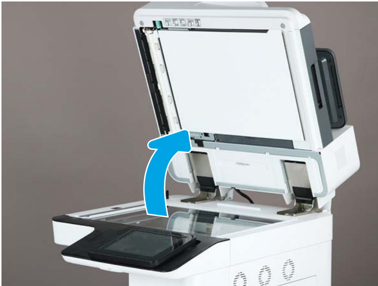
Figure 2-8 Open document feeder unit
