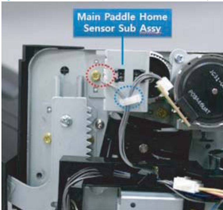
Figure 6-241 Remove the main paddle home sensor sub assembly
