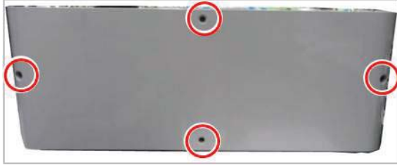
Figure 2-958 Remove the rear cover
