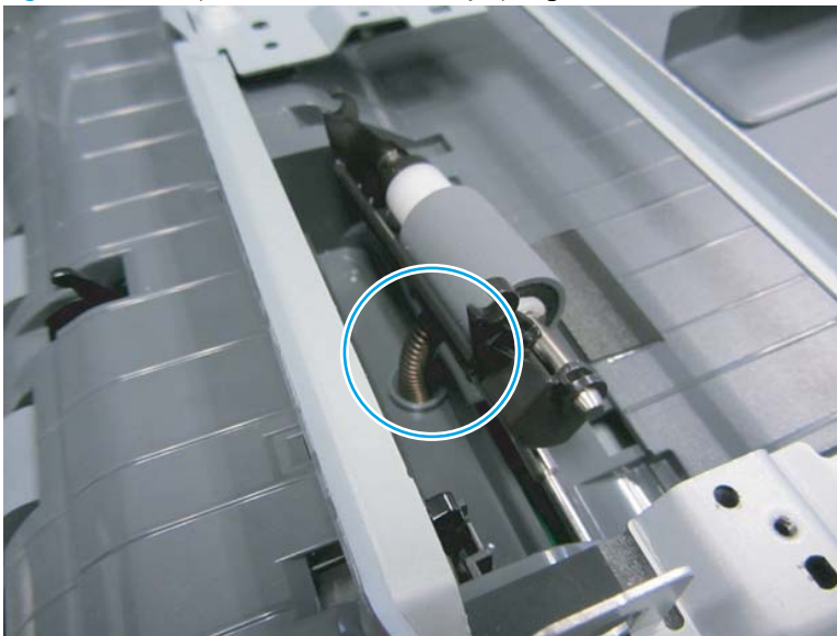
Figure 2-735 Separation roller assembly spring
