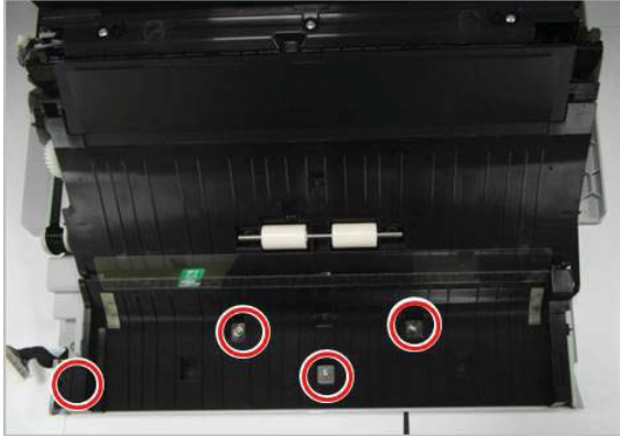
Figure 2-637 Remove four screws
