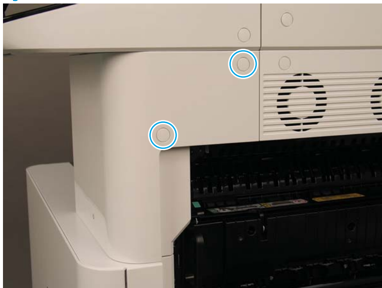
Figure 2-358 Remove two screws and rotate the cover
