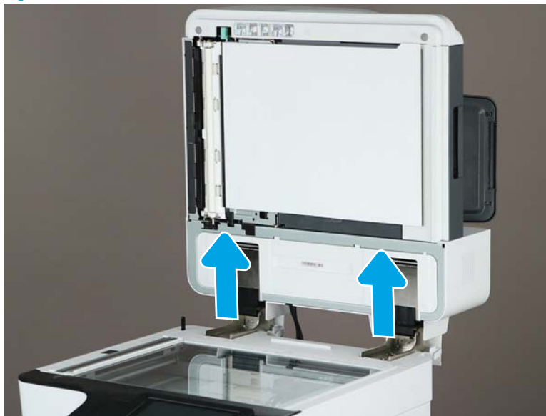
Figure 2-761 Release the document feeder
