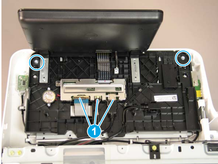
Figure 2-72 Remove the control panel screws and disconnect connectors
