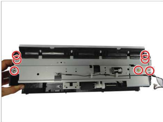
Figure 2-656 Remove seven screws
