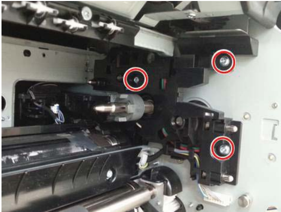
Figure 2-414 Remove three screws and the high voltage terminal
