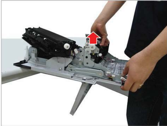
Figure 2-553 Release the Tray 1 door
