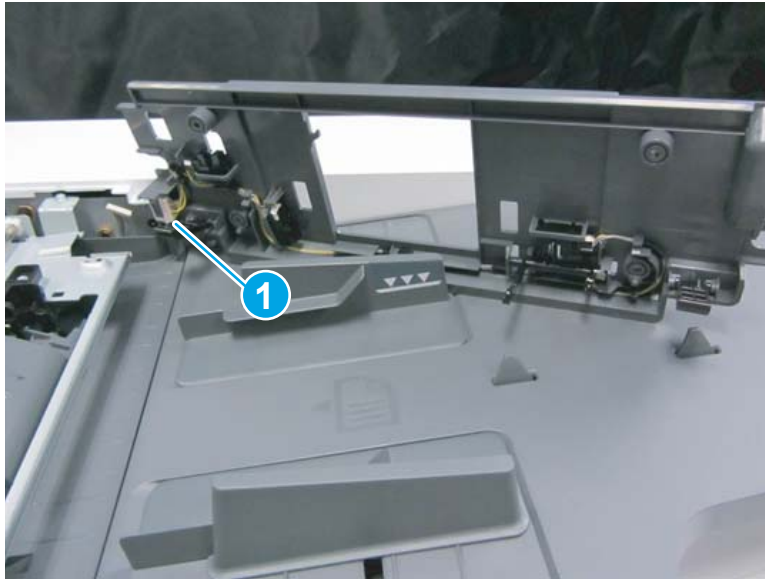
Figure 2-728 Turn the cover over and disconnect connector
