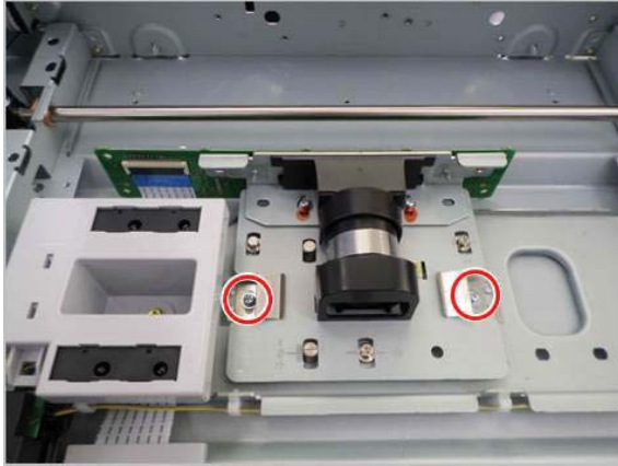
Figure 2-901 Remove screws and release scanner imaging unit
