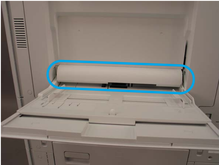
Figure 2-329 Remove the cover
