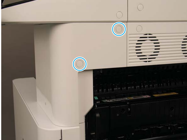
Figure 2-19 Remove two screws and rotate the cover
