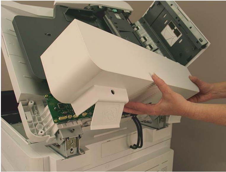
Figure 2-855 Remove back cover.
