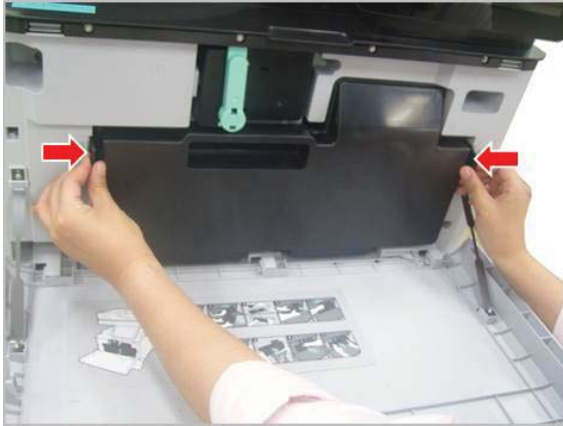
Figure 2-21 Remove the TCU
