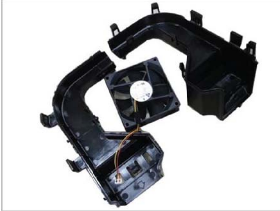
Figure 2-187 Remove the fuser fan
