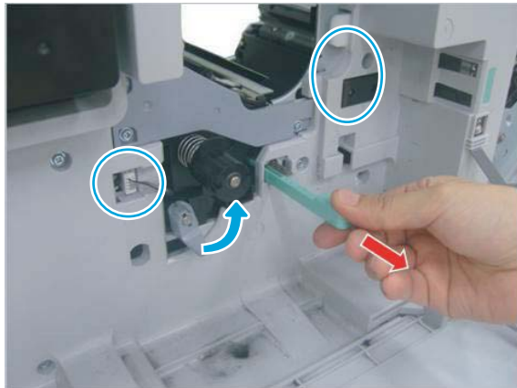
Figure 2-369 Remove the paper dust brush
