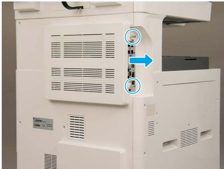
Figure 2-36 Remove the formatter cover
