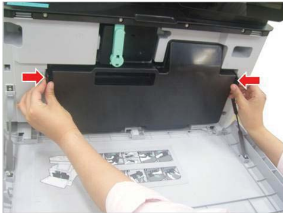
Figure 2-464 Remove the TCU
