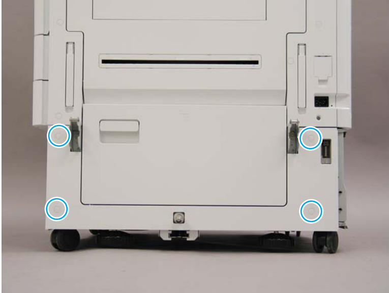
Figure 2-921 Remove the lower right cover
