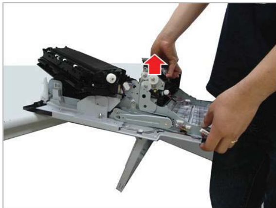
Figure 2-653 Release the Tray 1 door
