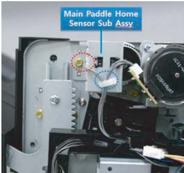
Figure 6-177 Remove the main paddle home sensor sub assembly
