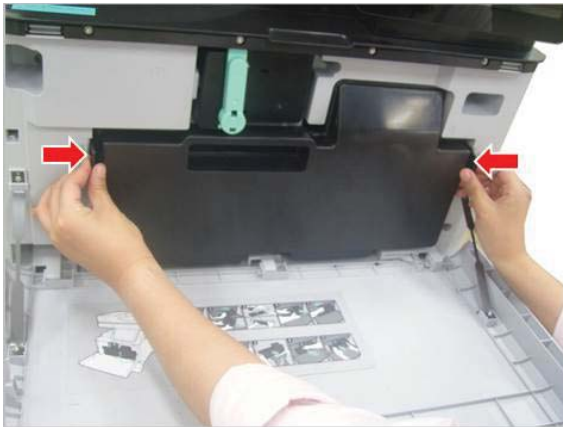
Figure 2-367 Remove the TCU
