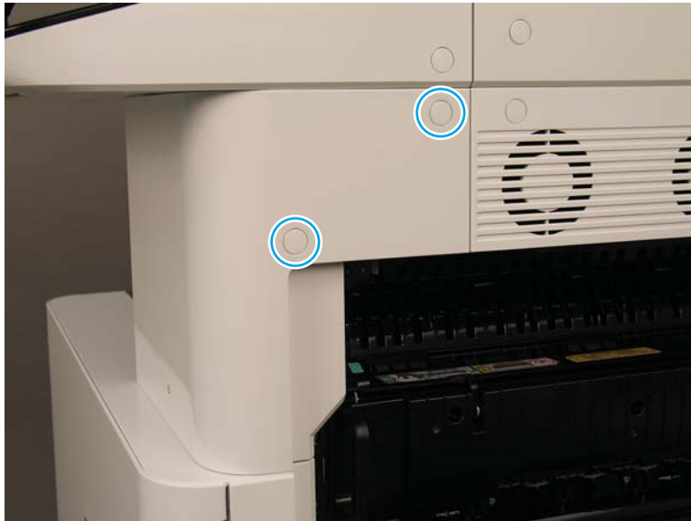
Figure 2-365 Remove two screws and rotate the cover
