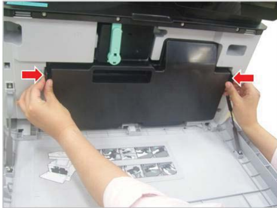
Figure 2-56 Remove the TCU
