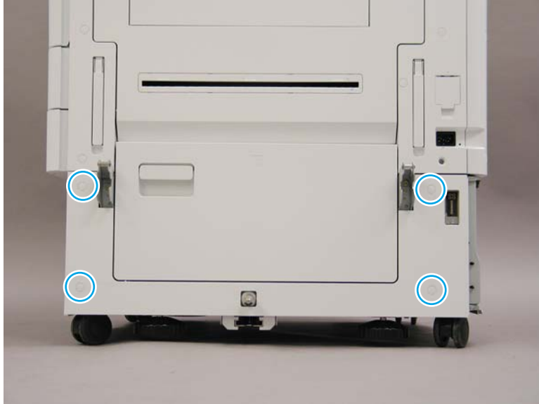
Figure 2-936 Remove the lower right cover
