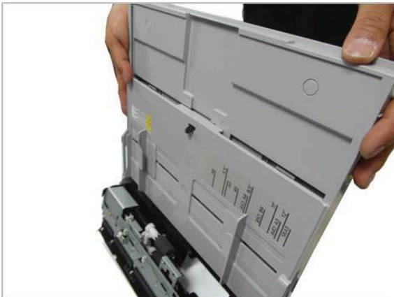
Figure 2-628 Remove the Tray 1 tray upper
