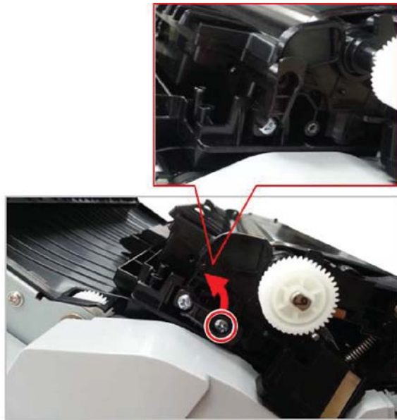
Figure 2-663 Remove one screw and position the lever
