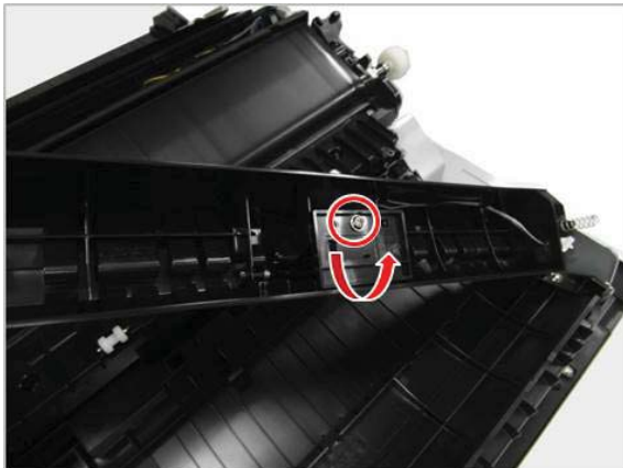
Figure 2-566 Remove one screw
