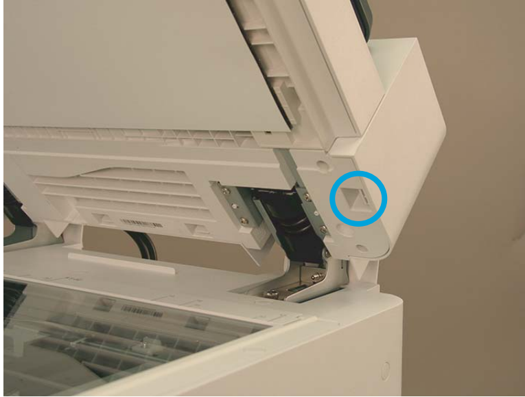
Figure 2-675 Release one tab on the right side of back cover.
