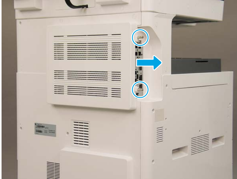
Figure 2-347 Remove the formatter cover
