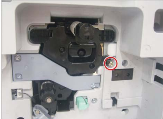
Figure 2-322 Loosen one screw
