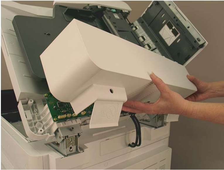
Figure 2-686 Remove back cover.
