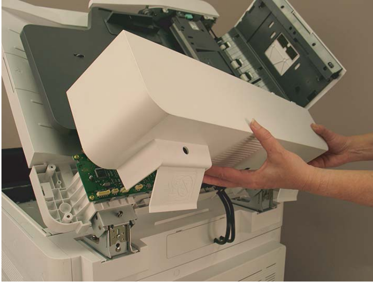
Figure 2-849 Remove back cover.
