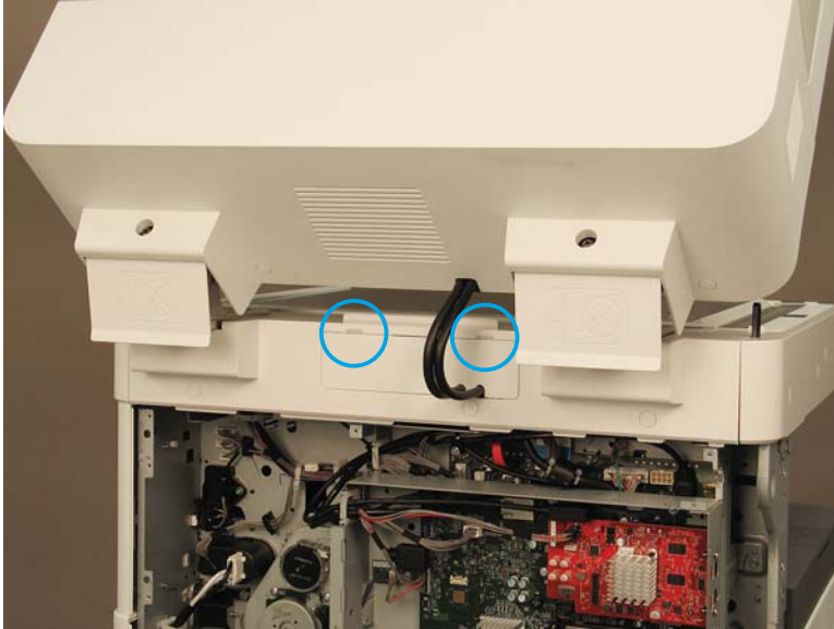
Figure 2-870 Remove document feeder connector cover
