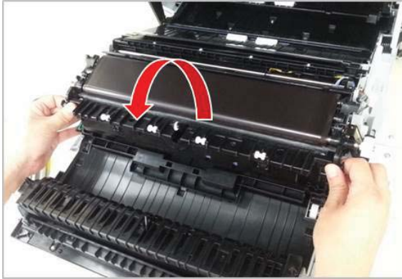
Figure 2-665 Remove the PTB assembly
