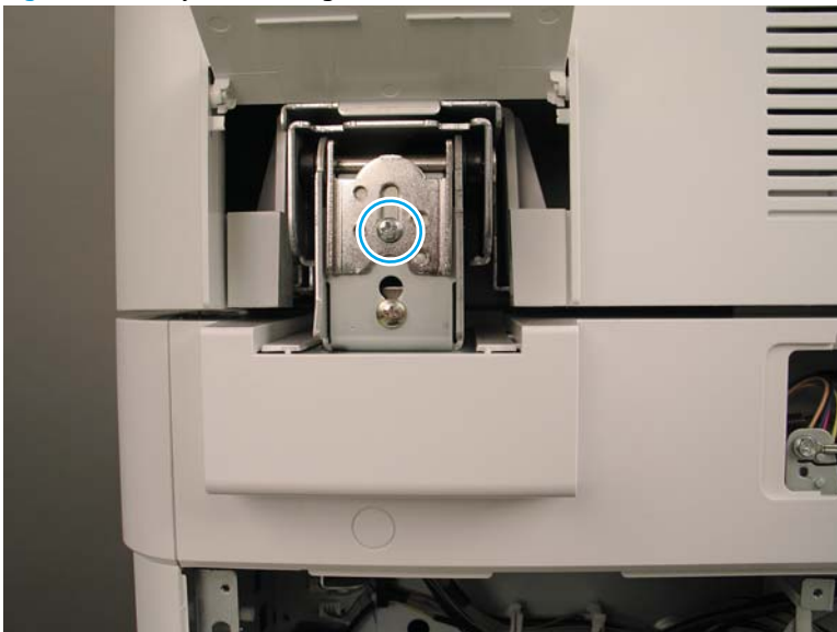
Figure 3-50 Adjust ADF hinge
