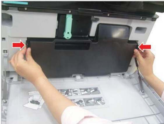
Figure 2-218 Remove the TCU
