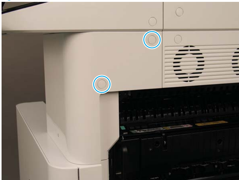
Figure 2-15 Remove two screws and rotate the cover
