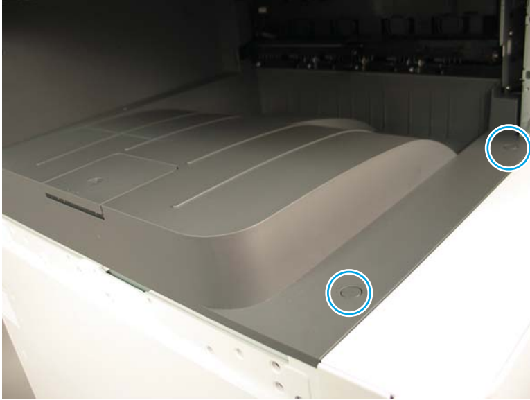
Figure 2-465 Remove the exit cover
