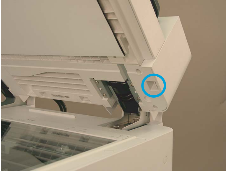
Figure 2-738 Release one tab on the right side of back cover.
