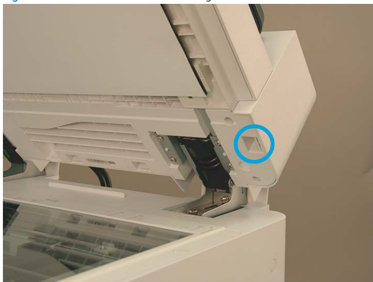
Figure 2-721 Release one tab on the right side of back cover.
