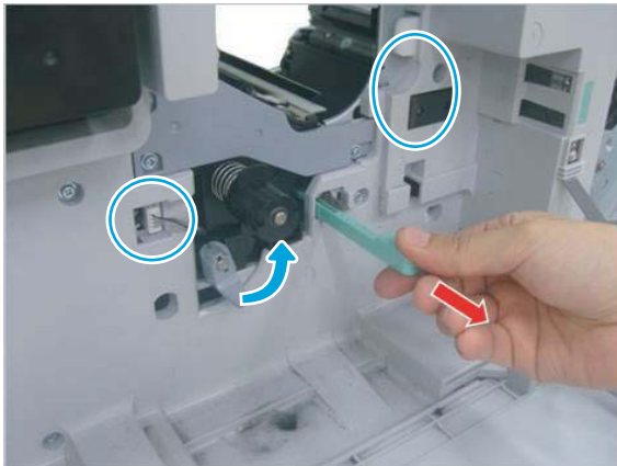
Figure 2-466 Remove the paper dust brush
