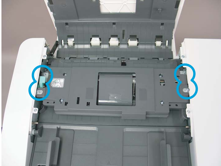
Figure 2-695 Remove four screws.
