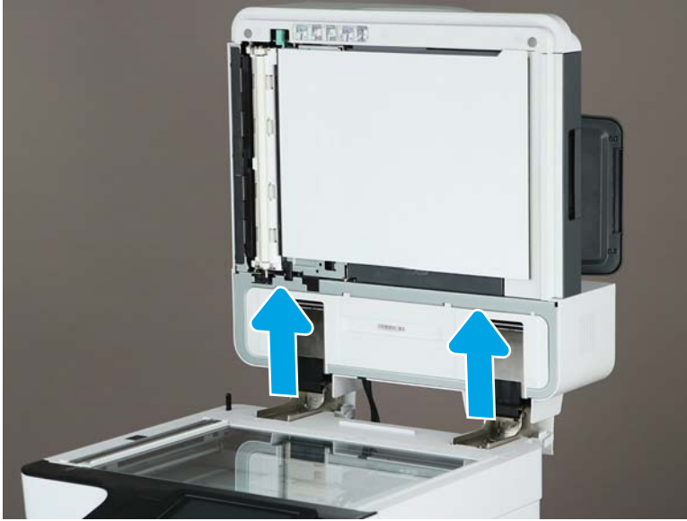
Figure 2-908 Remove two screws and lift up to remove ADF
