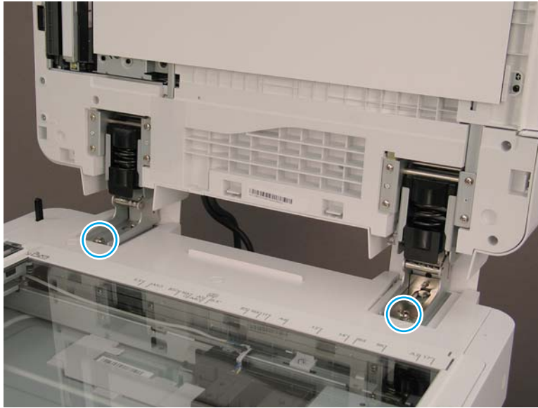
Figure 2-64 Lift and remove the document feeder
