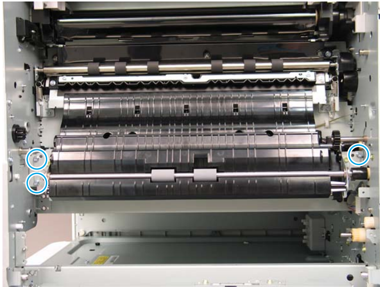
Figure 2-112 Remove three screws
