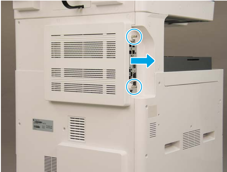
Figure 2-375 Remove the formatter cover
