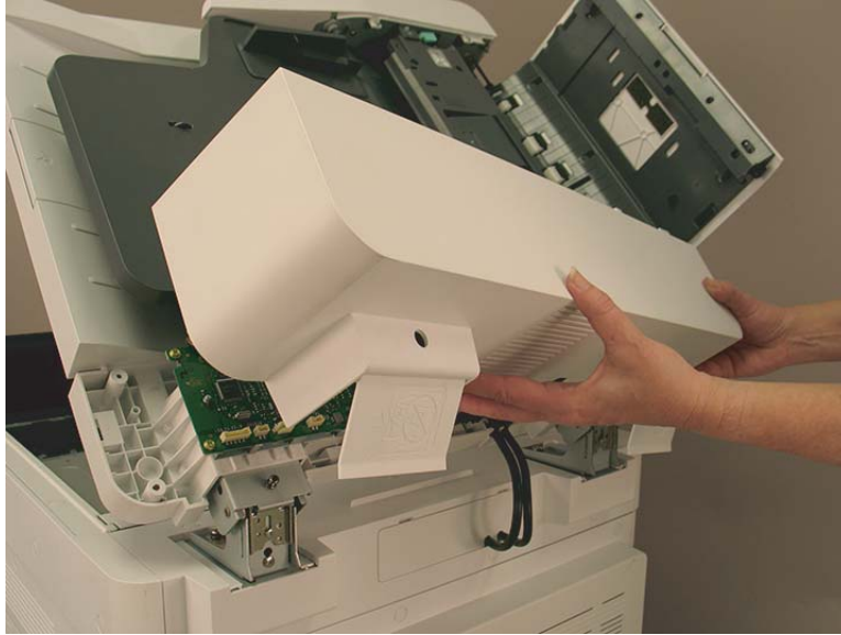
Figure 2-781 Remove back cover.
