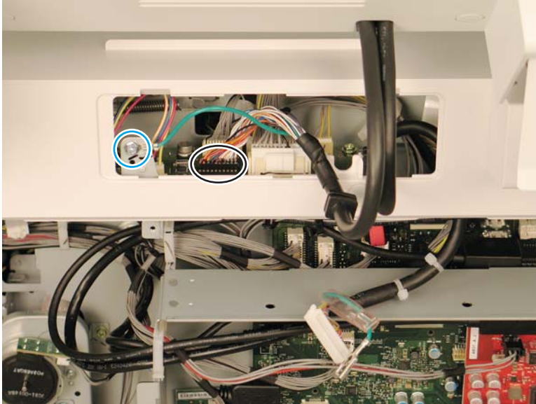
Figure 2-904 Disconnect document feeder harness
