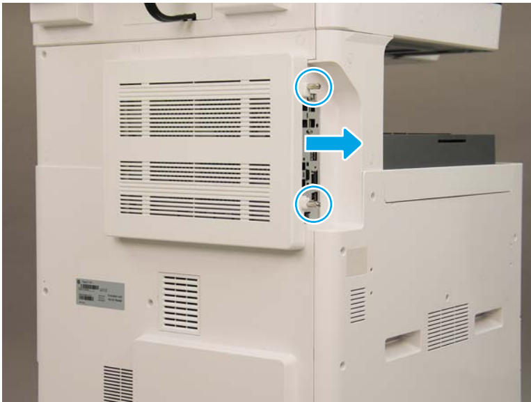
Figure 2-42 Remove the formatter cover
