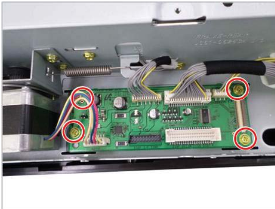
Figure 2-754 Remove screws and release scanner PCA
