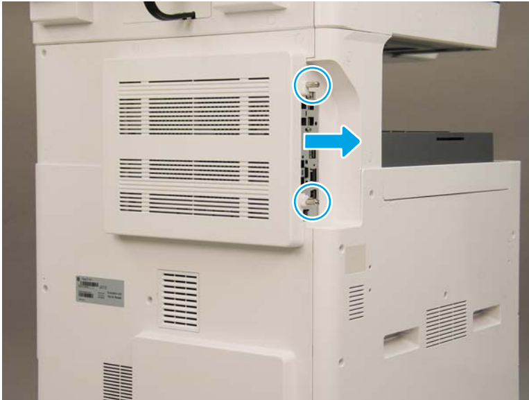
Figure 2-668 Remove the formatter cover and the upper rear cover
