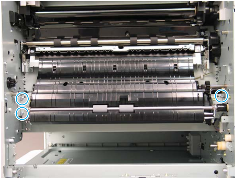
Figure 2-508 Remove three screws
