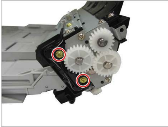
Figure 2-654 Remove two screws and three gears
