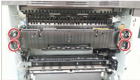
Figure 2-267 Fuser unit screw locations
