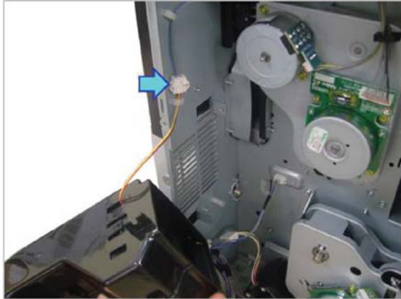
Figure 2-185 Disconnect one connector
