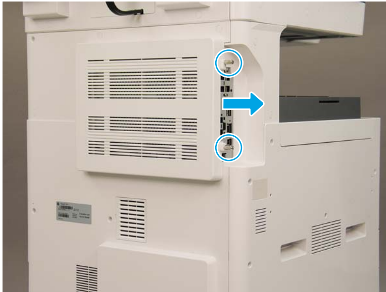
Figure 2-471 Remove the formatter cover
