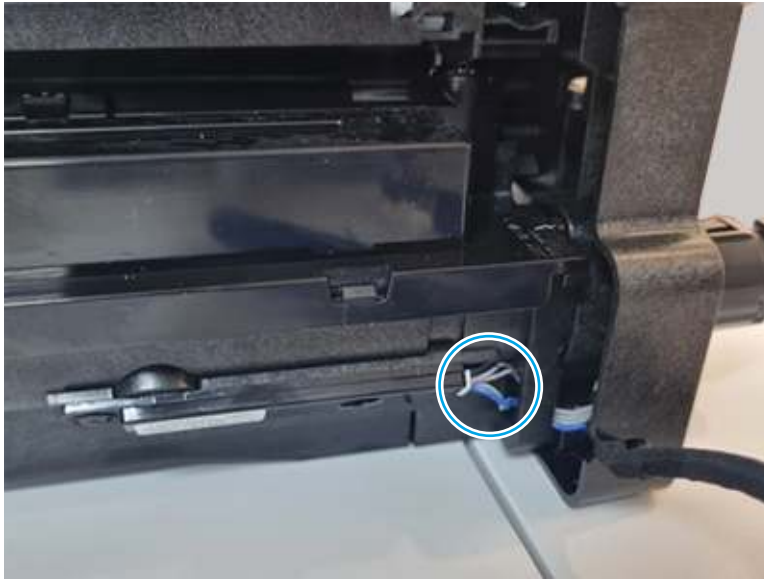
Figure 6-455 Disconnect one connector
