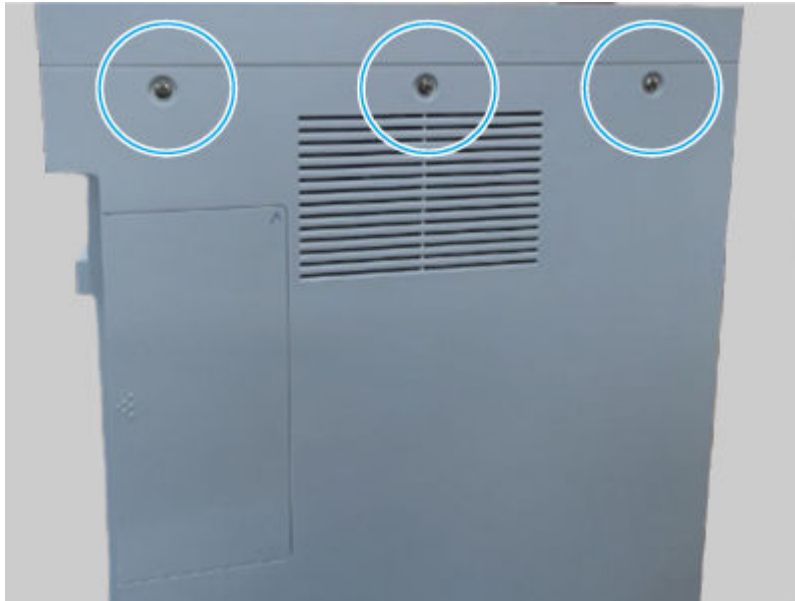
Figure 6-2109 Remove three screws
