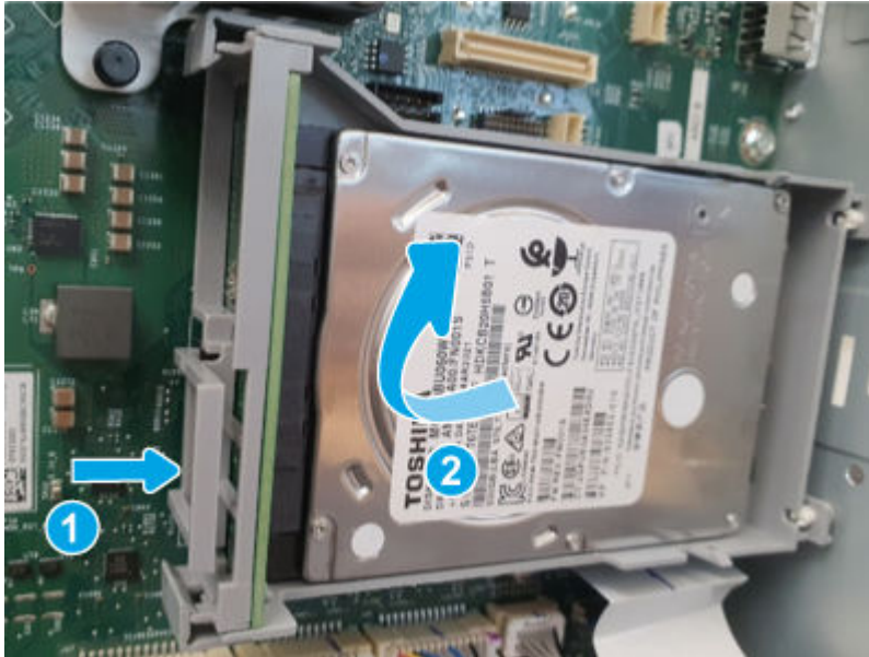
Figure 6-836 Remove the HDD
