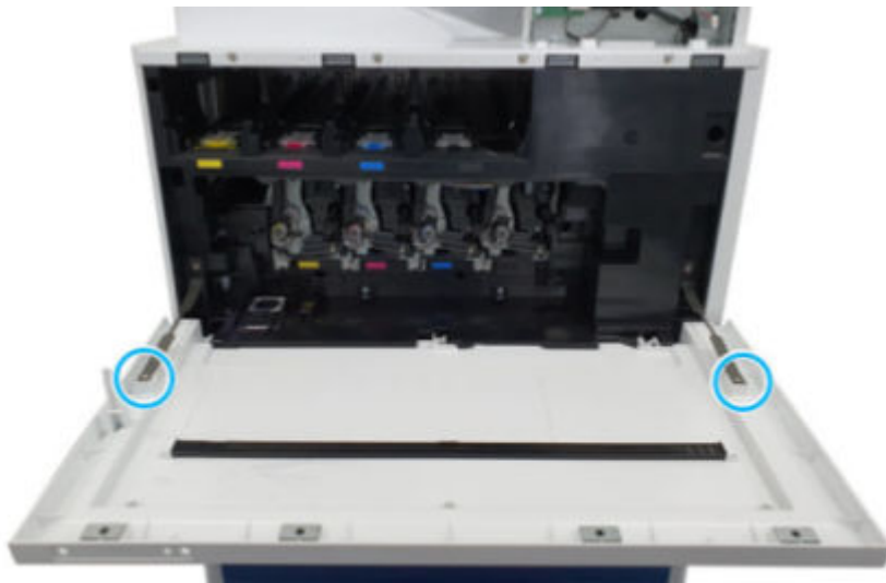
Figure 6-654 Remove two screws
