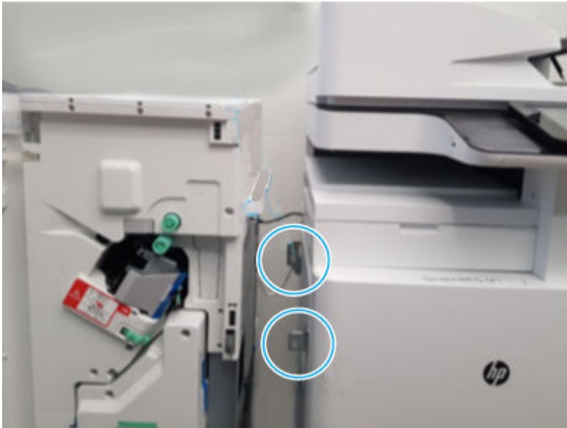
Figure 6-1405 Disconnect two connectors
