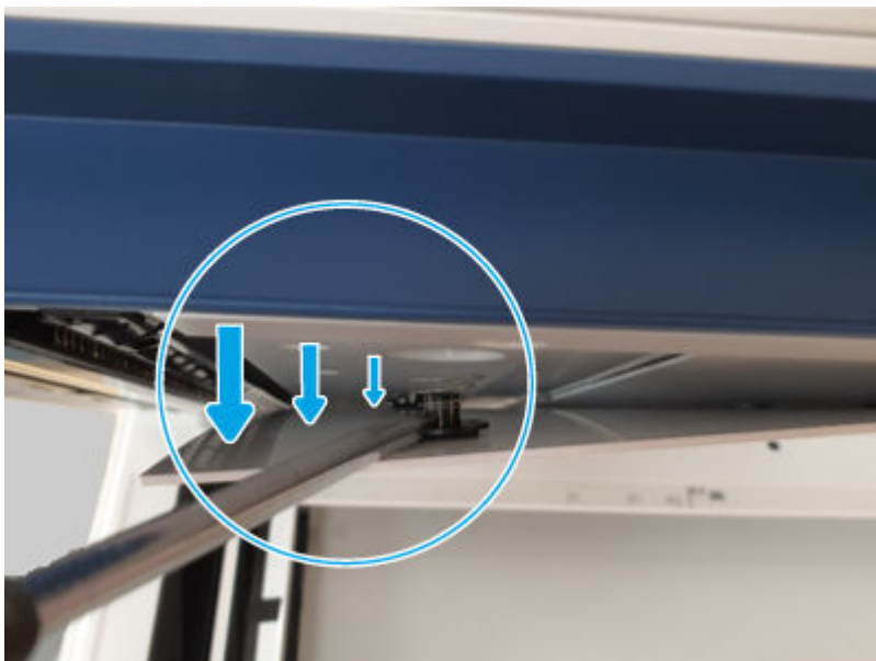
Figure 6-944 Remove the white backing
