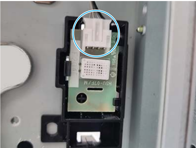
Figure 6-769 Disconnect one connector
