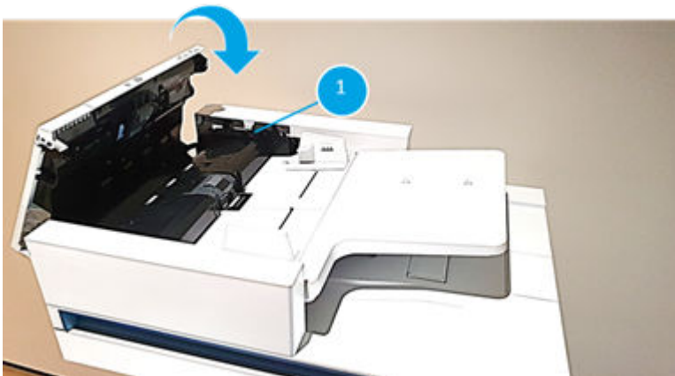
Figure 3-142 Document feeder simplex operation, view 1
