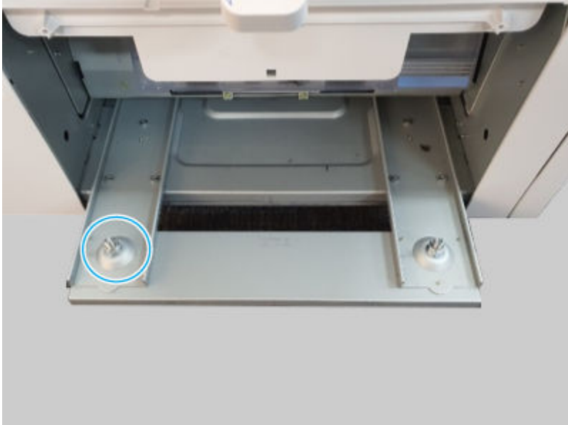
Figure 6-2098 Remove the nut
