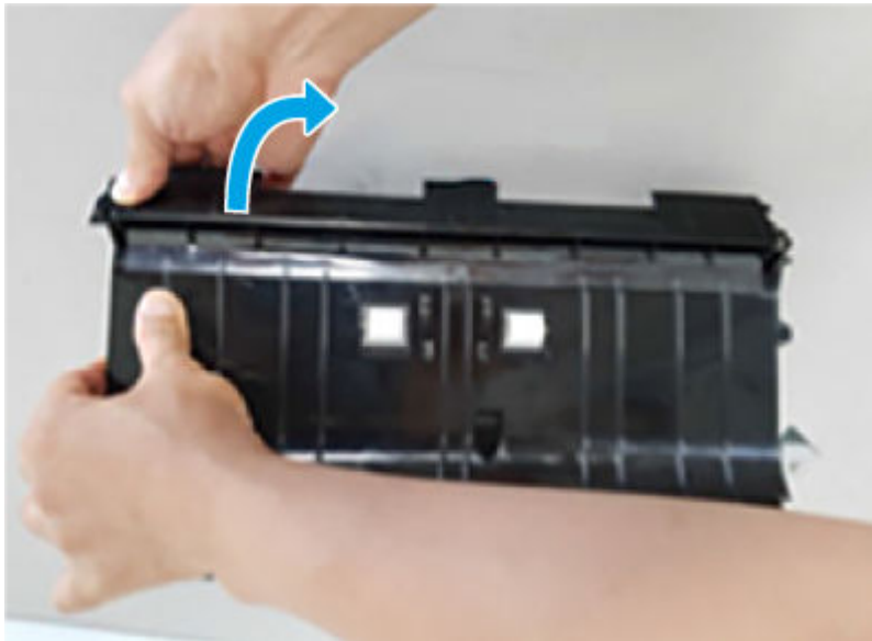
Figure 6-1467 Remove the diverter
