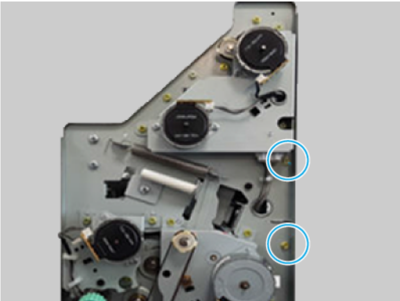
Figure 6-2391 Remove two screws
