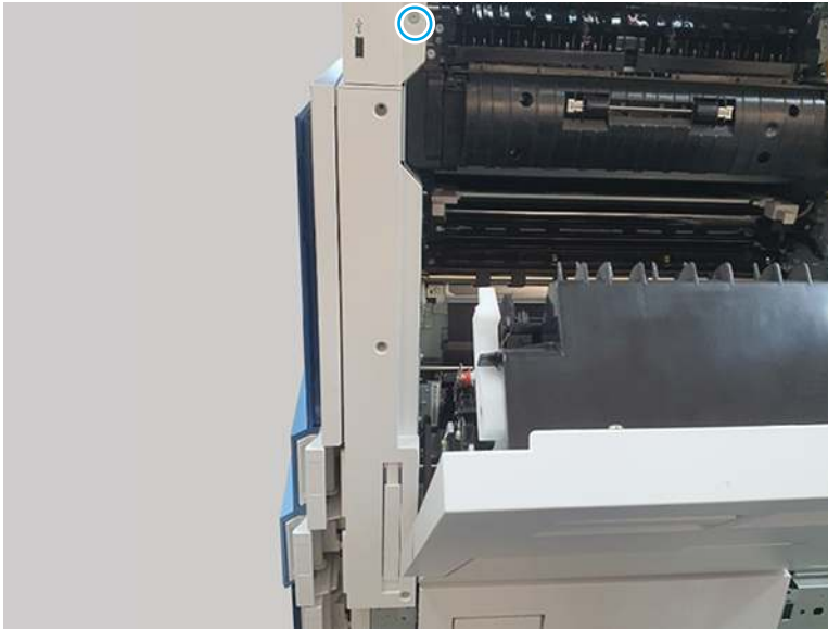
Figure 6-37 Open the right door and remove screw
