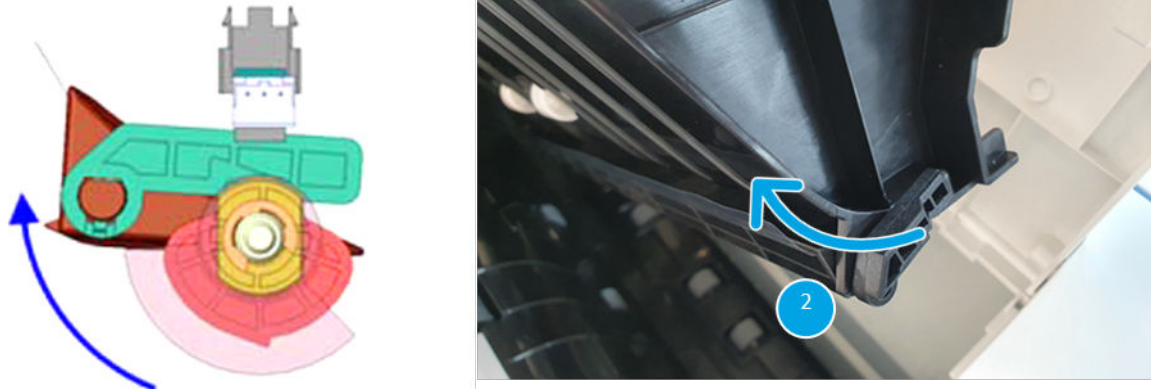
Figure 3-243 Tray diverter unit operation, view 2
