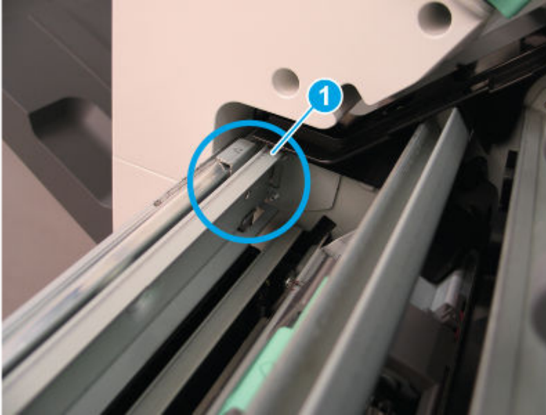
Figure 6-2552 Check rail alignment (2 of 2)
