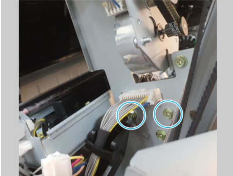
Figure 6-1885 Remove two screws
