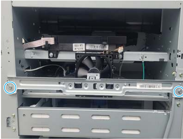
Figure 6-676 Remove two screws
