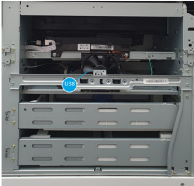
Figure 3-97 Detail view of the temperature and humidity measurement sensor, view 3
