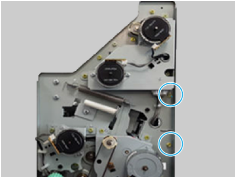
Figure 6-2494 Remove two screws
