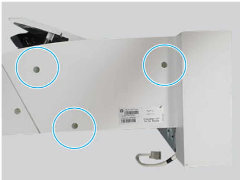
Figure 6-3188 Remove three screws
