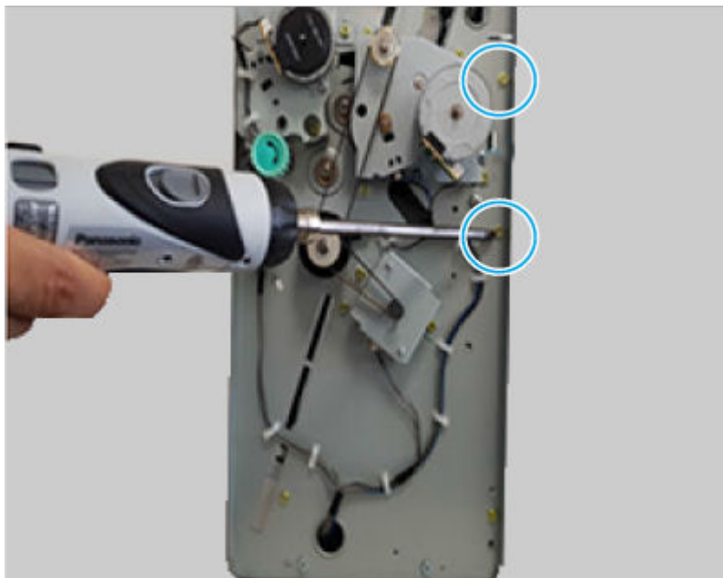
Figure 6-2327 Remove two screws
