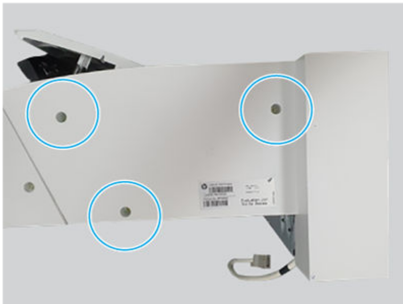
Figure 6-2786 Remove three screws
