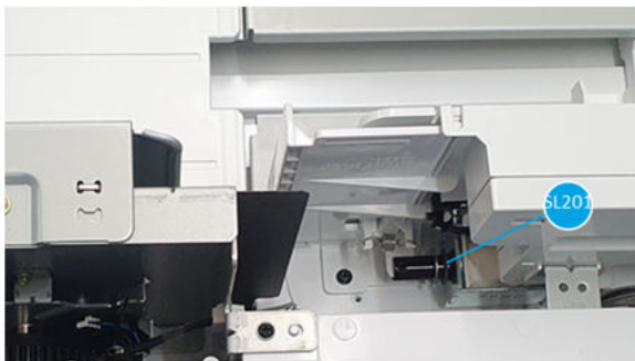
Figure 3-205 Detailed view of HCI motor (3 of 3)
