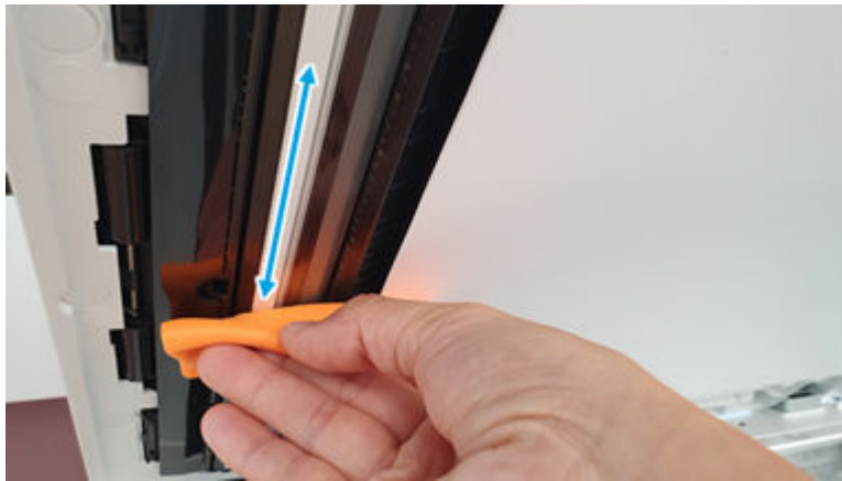
Figure 3-165 ADF image scanner cleaning
