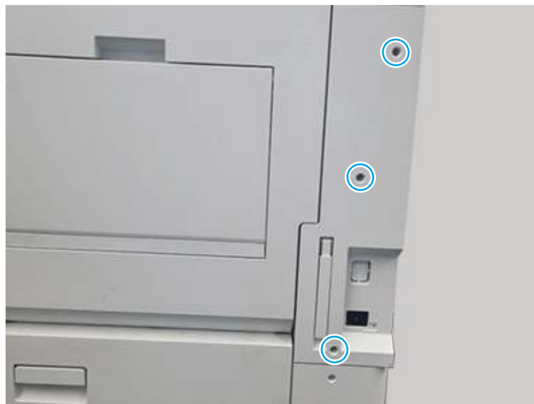
Figure 6-763 Remove three screws
