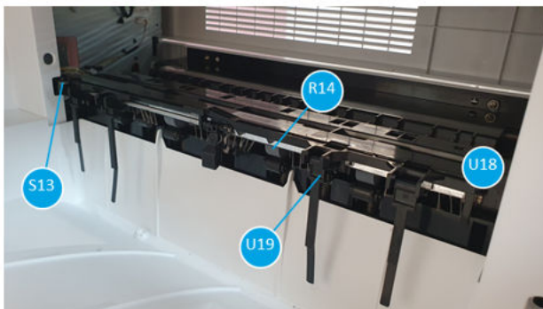
Figure 3-39 Detail view of exit unit (1 of 2)
