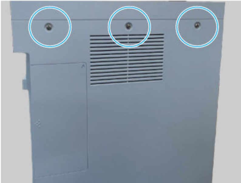
Figure 6-1594 Remove three screws
