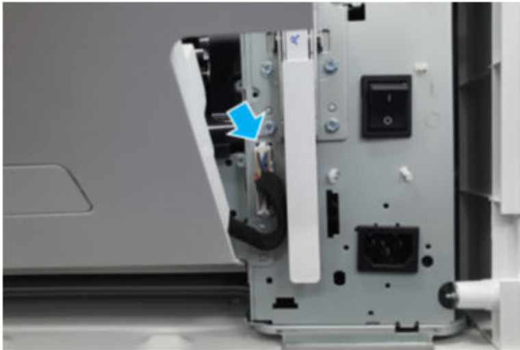
Figure 6-225 Disconnect one connector
