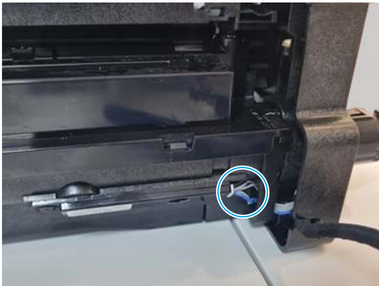
Figure 6-685 Disconnect one connector
