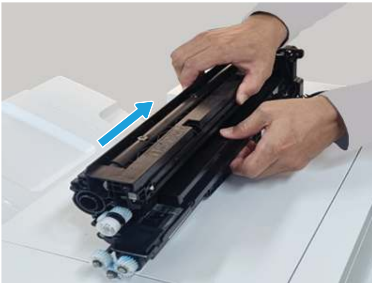
Figure 6-716 Remove the drum unit
