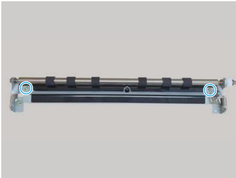
Figure 6-339 Remove two screws
