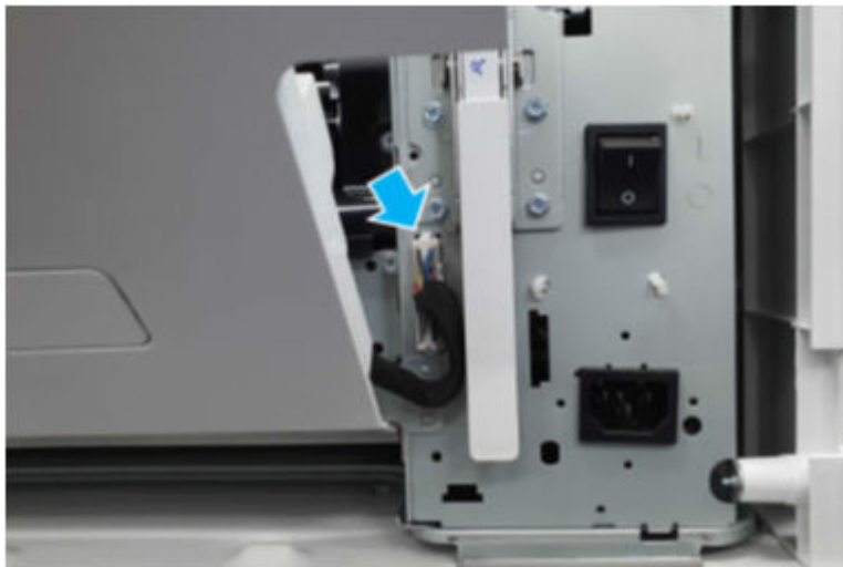
Figure 6-330 Disconnect one connector
