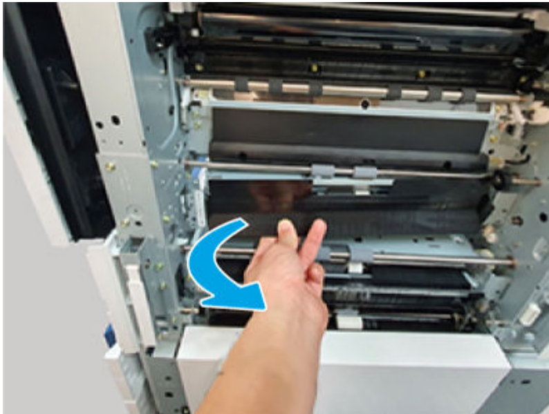
Figure 6-191 Rotate the assembly away from the printer
