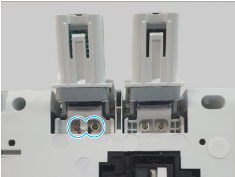
Figure 6-1007 Remove two screws
