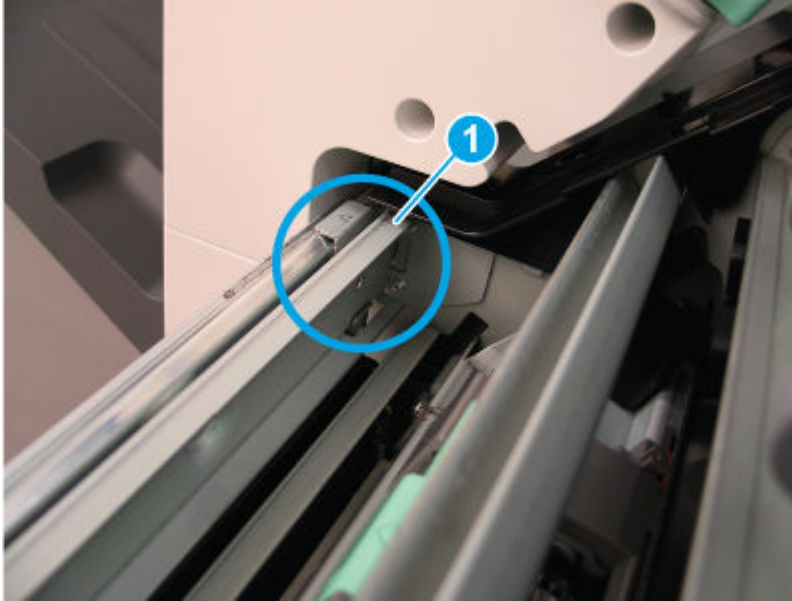
Figure 6-2202 Check rail alignment (2 of 2)
