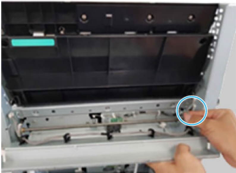
Figure 6-2395 Disconnect one connector
