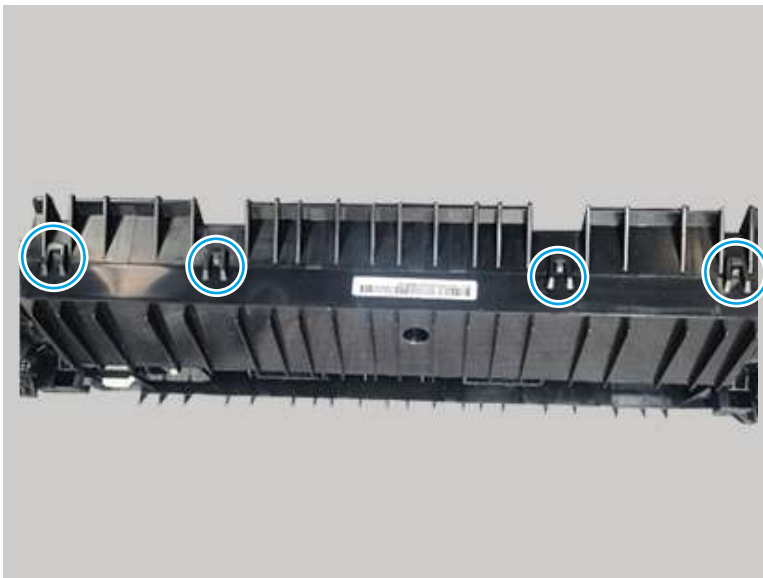
Figure 6-430 Release four hooks
