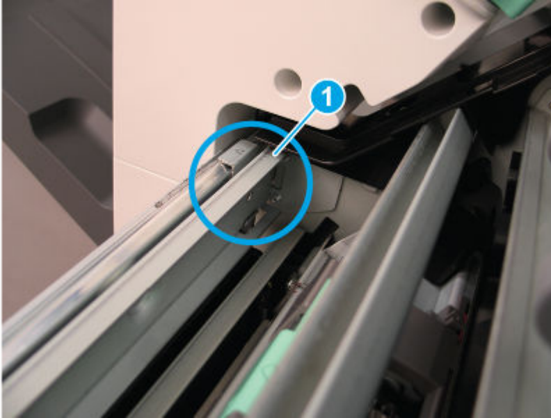
Figure 6-2138 Check rail alignment (2 of 2)
