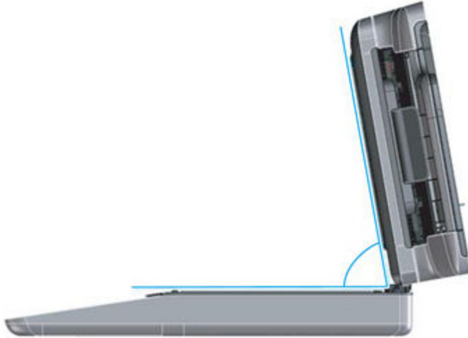
Figure 3-164 Document feeder open (maximum 65°)
