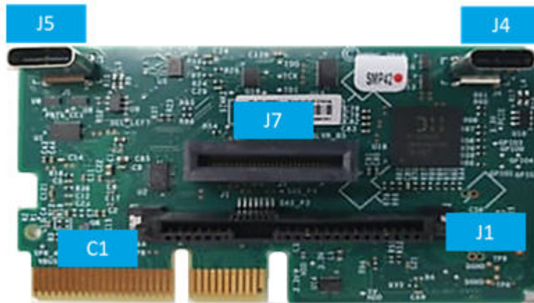
Figure 3-106 Riser card for HDD, two USB Type C ports, and accelerator board
