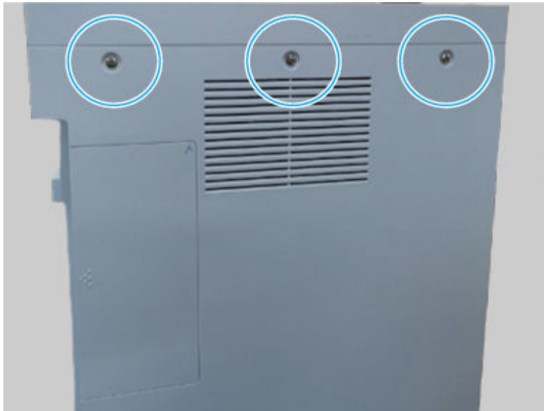
Figure 6-1366 Remove three screws
