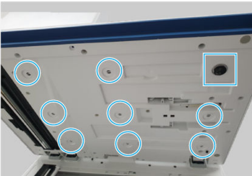
Figure 6-948 Install the remaining suspension clips
