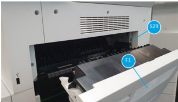
Figure 3-98 Detail view of the temperature and humidity measurement sensor, view 4
