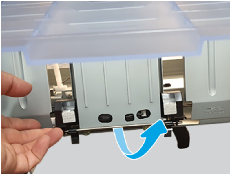
Figure 6-2254 Lift the fence
