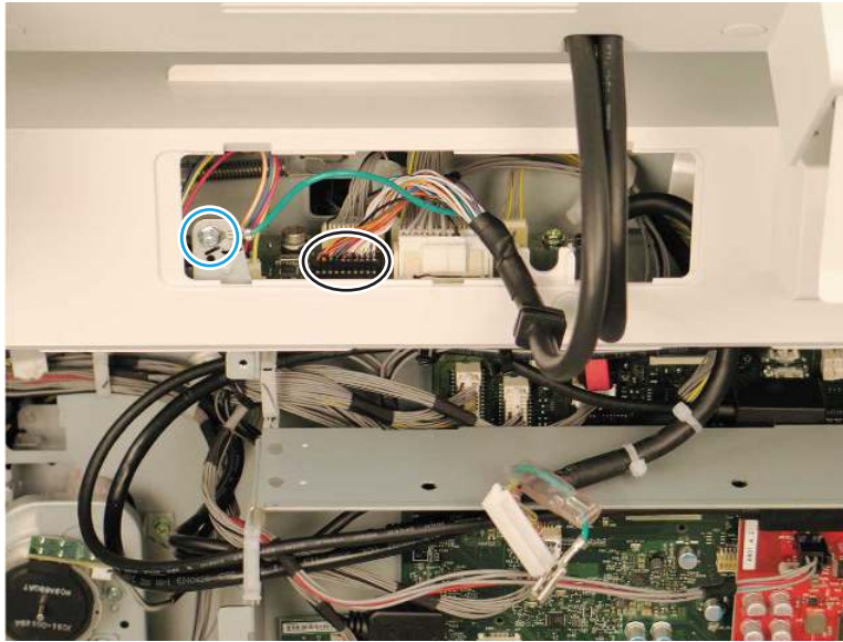
Figure 2-27 Disconnect document feeder harness
