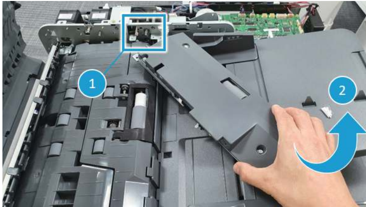
Figure 2-378 Remove the pickup roller assembly
