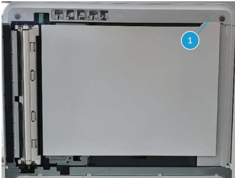
Figure 2-285 Open the document feeder
