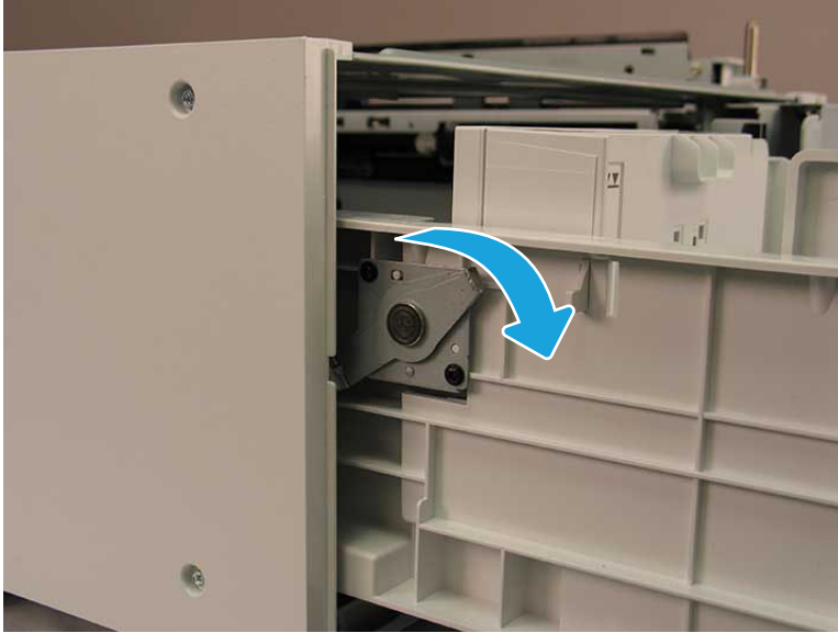
Figure 2-558 Release the tray left side hook lever
