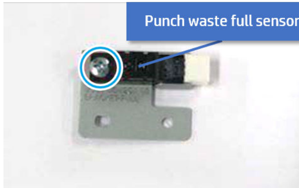
Figure 7-788 Remove the punch waste full sensor
