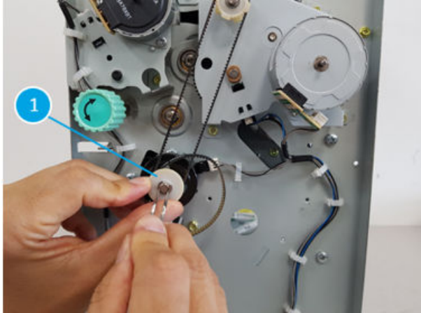
Figure 5-1486 Remove white washer
