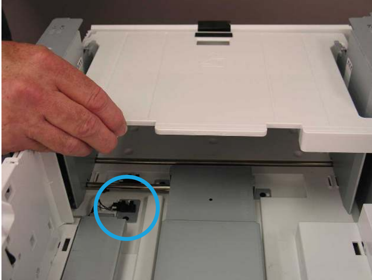
Figure 2-571 Remove the HCI photo interrupter and sensor bracket
