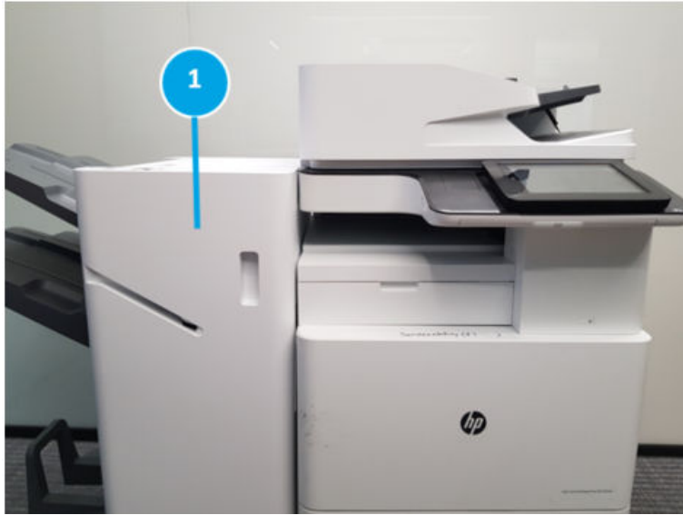
Figure 5-148 Open the front door
