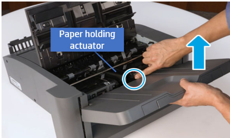
Figure 7-724 Remove the output tray.
