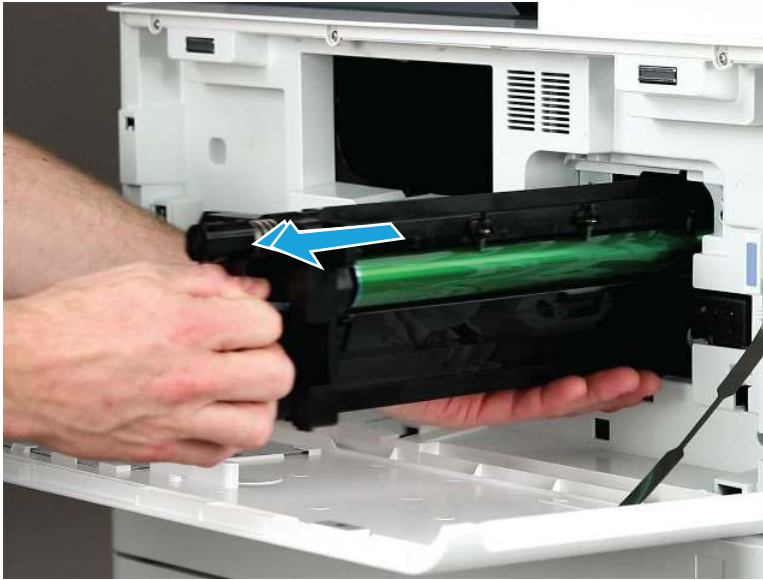
Figure 2-124 Remove drum unit
