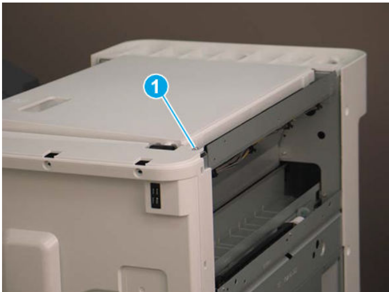
Figure 5-950 Remove one screw
