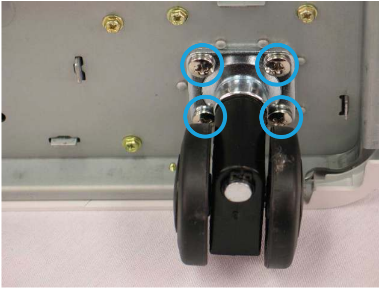
Figure 2-517 Remove the HCI caster wheel
