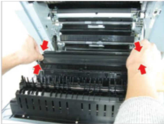
Figure 2-225 Remove transfer roller
