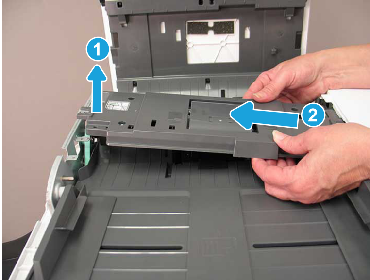
Figure 2-302 Release the pick/feed roller assembly
