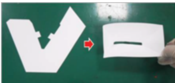
Figure 2-117 Fold protective sheet
