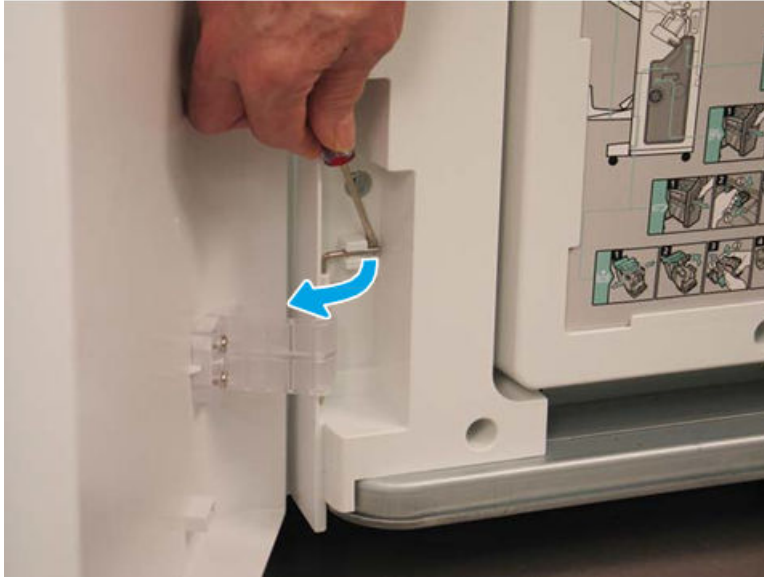
Figure 5-340 Release the lower hinge pin
