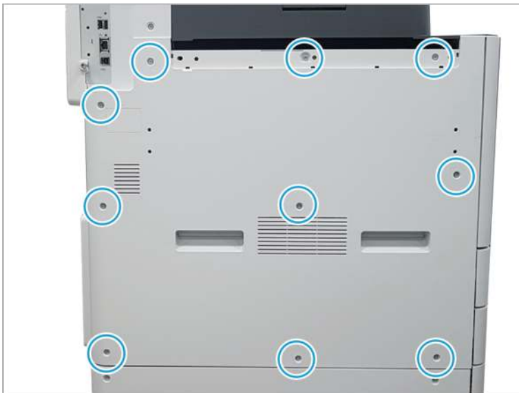
Figure 2-97 Remove the left cover
