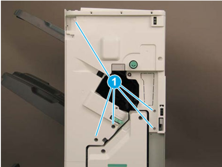
Figure 5-482 Remove the front cover
