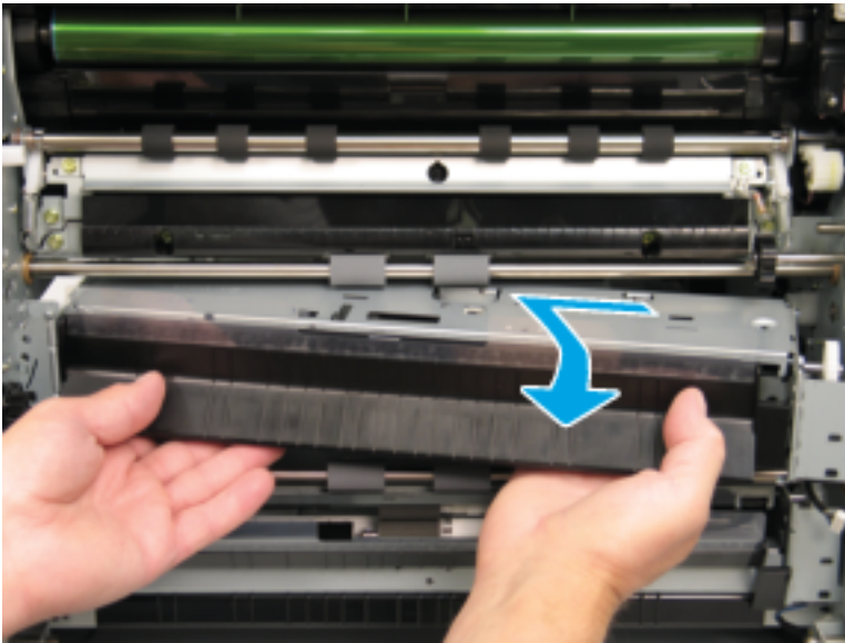
Figure 2-203 Remove the pickup assembly
