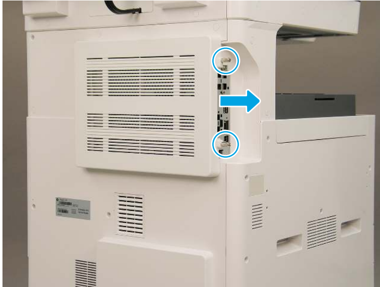
Figure 2-23 Remove the formatter cover
