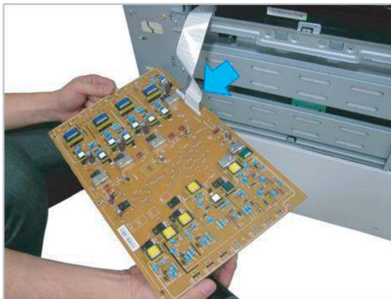
Figure 2-99 Remove the HVPS board
