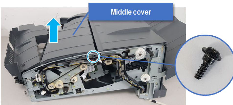
Figure 7-64 Remove the middle cover
