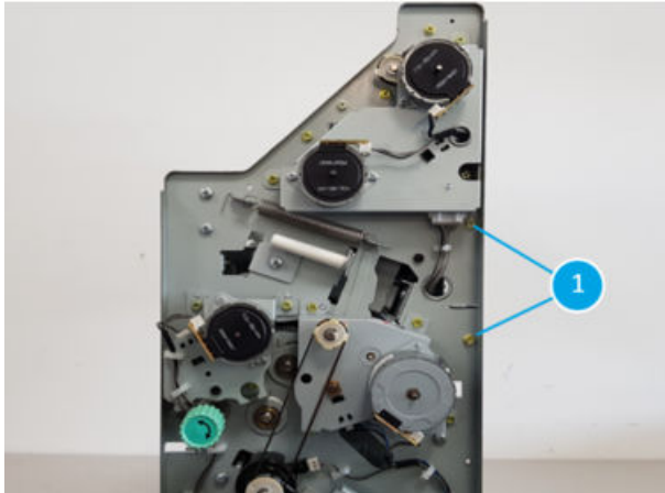
Figure 5-1578 Remove two screws at the front of the booklet maker
