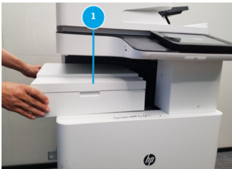
Figure 5-125 Pull out the bridge unit
