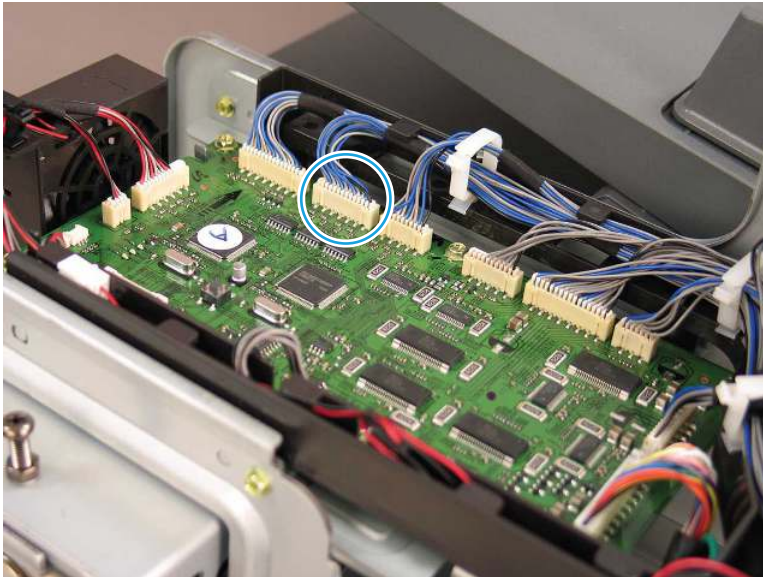
Figure 2-367 Disconnect one connector
