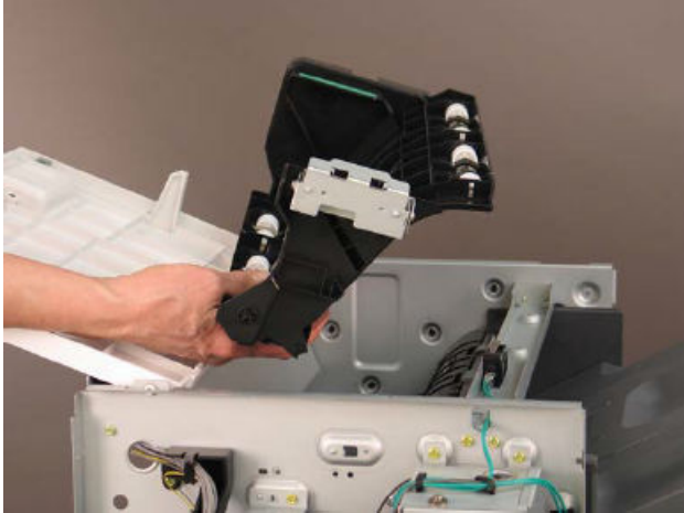
Figure 5-328 Remove the top jam access cover
