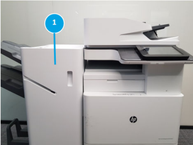
Figure 5-122 Open the front door
