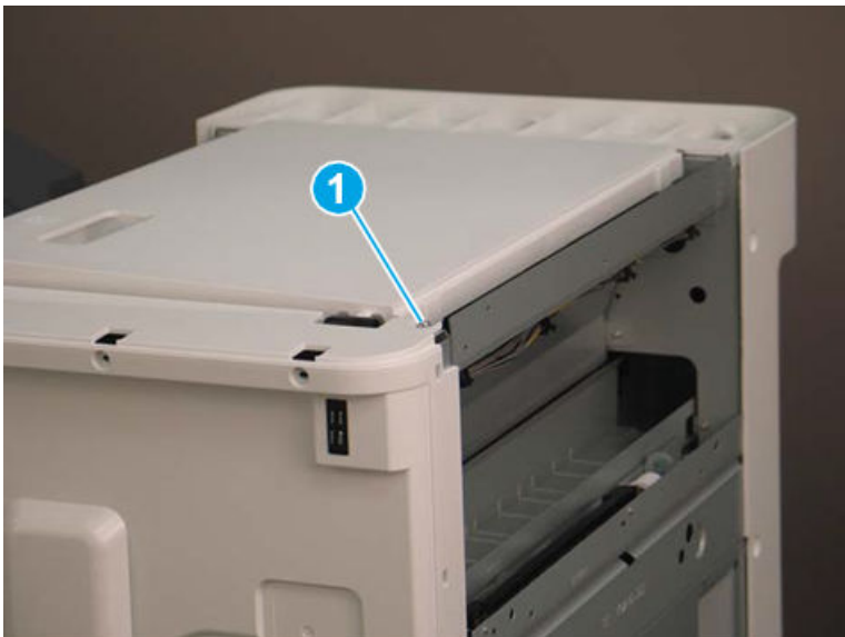
Figure 5-993 Remove one screw
