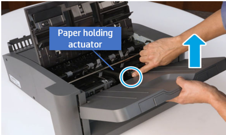
Figure 7-170 Remove the output tray.
