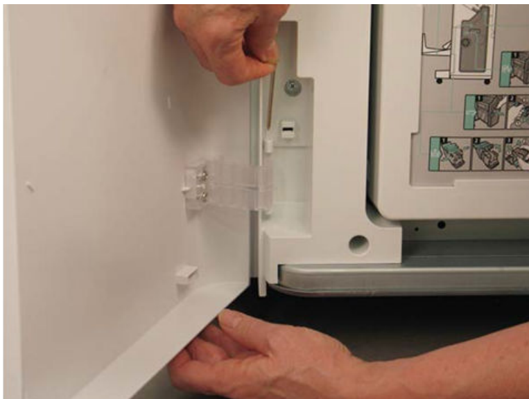
Figure 5-478 Remove the lower hinge pin
