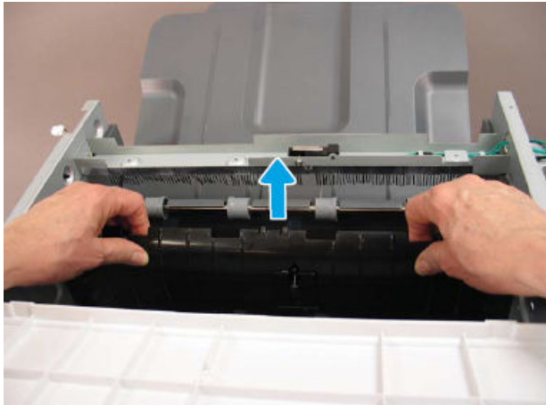
Figure 5-354 Remove the top lower feed assembly
