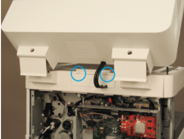
Figure 2-39 Remove document feeder connector cover
