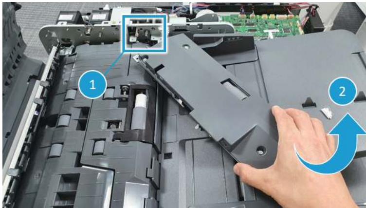
Figure 2-357 Remove the pickup roller assembly
