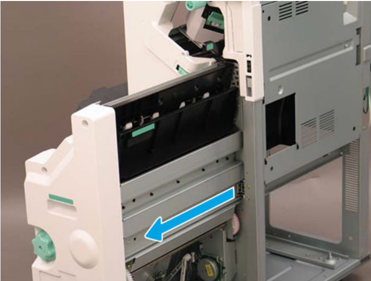
Figure 5-1538 Extend the right rail
