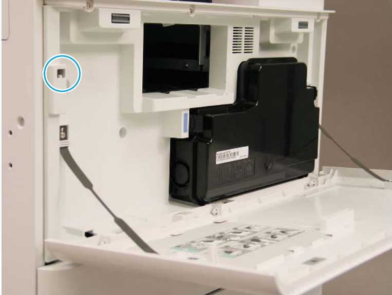
Figure 3-12 Defeat the toner cartridge door interlock
