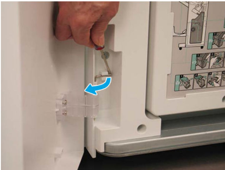
Figure 5-989 Release the lower hinge pin
