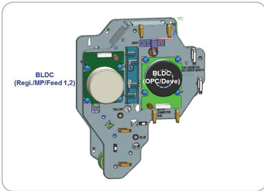
Figure 1-27 Main drive unit (rear view)
