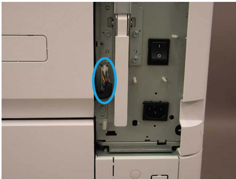
Figure 2-101 Disconnect right door connector
