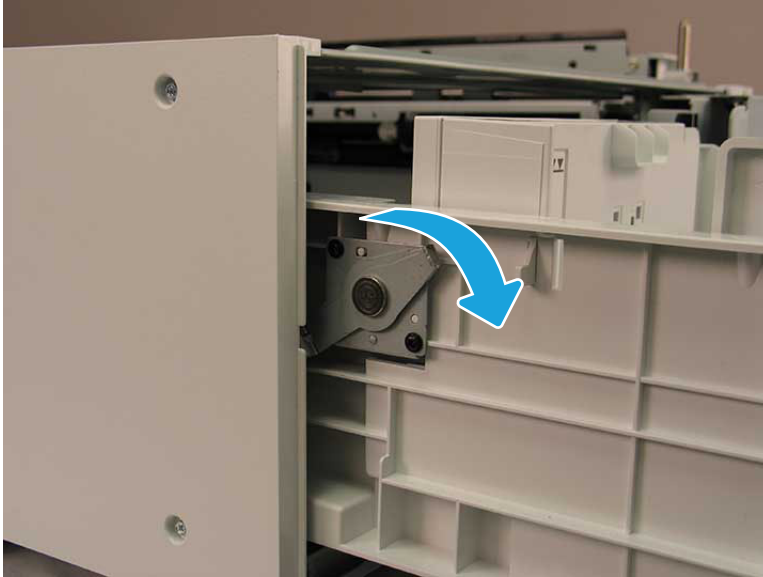
Figure 2-521 Release the tray left side hook lever
