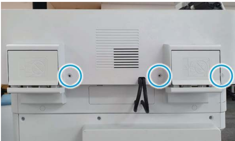
Figure 2-288 Remove 3 caps and 3 screws.
