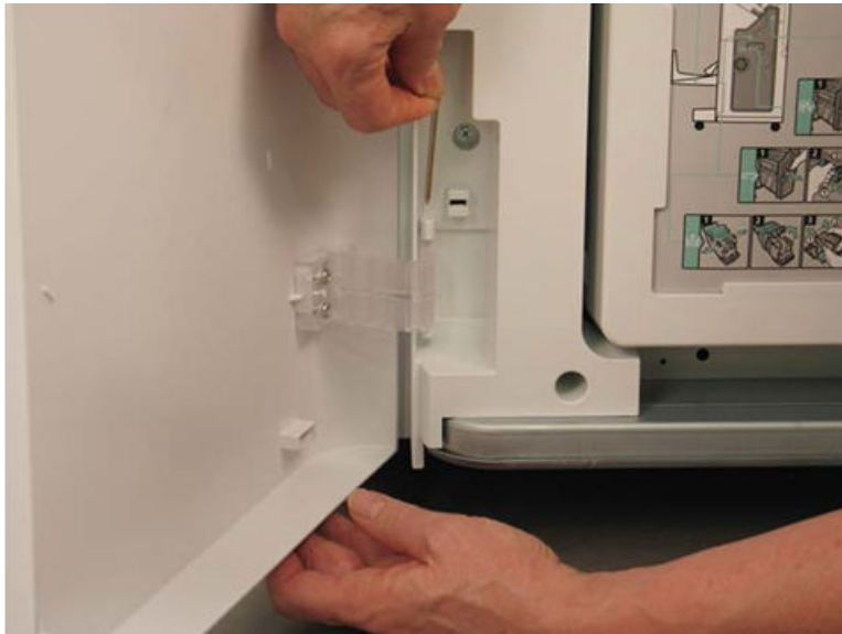
Figure 5-1389 Remove the lower hinge pin
