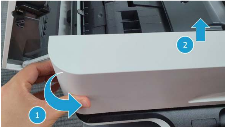
Figure 2-344 Remove the document feeder front cover
