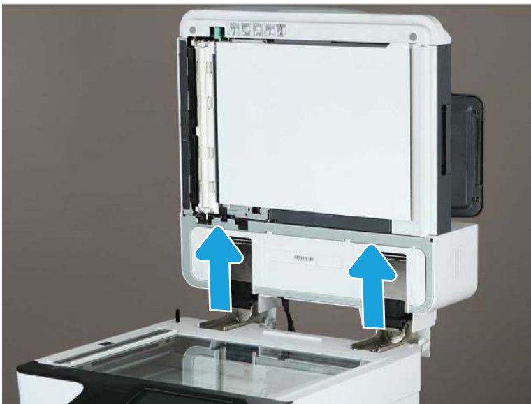
Figure 2-38 Release the document feeder
