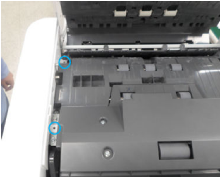
Figure 2-291 Remove the document feeder front cover top screws
