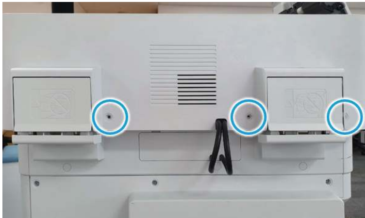
Figure 2-295 Remove 3 caps and 3 screws.
