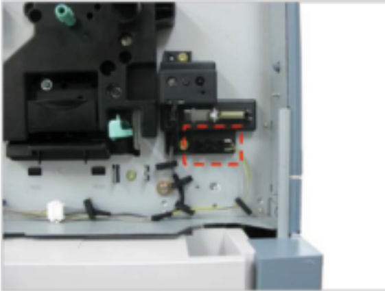
Figure 2-210 Disconnect connector and remove sensor
