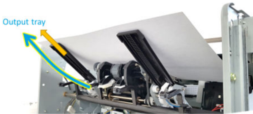
Figure 7-25 Inner finisher system - paper support unit operation
