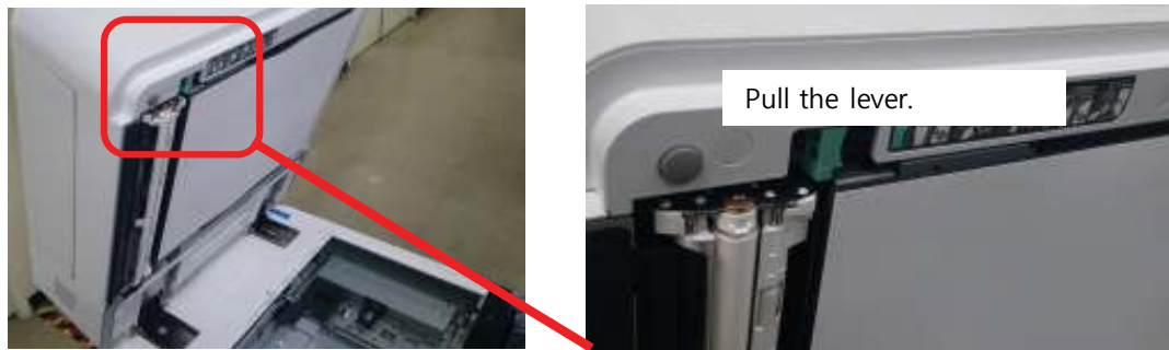
Figure 1-63 Flow document feeder dual sensor cleaning method (1 of 2)
