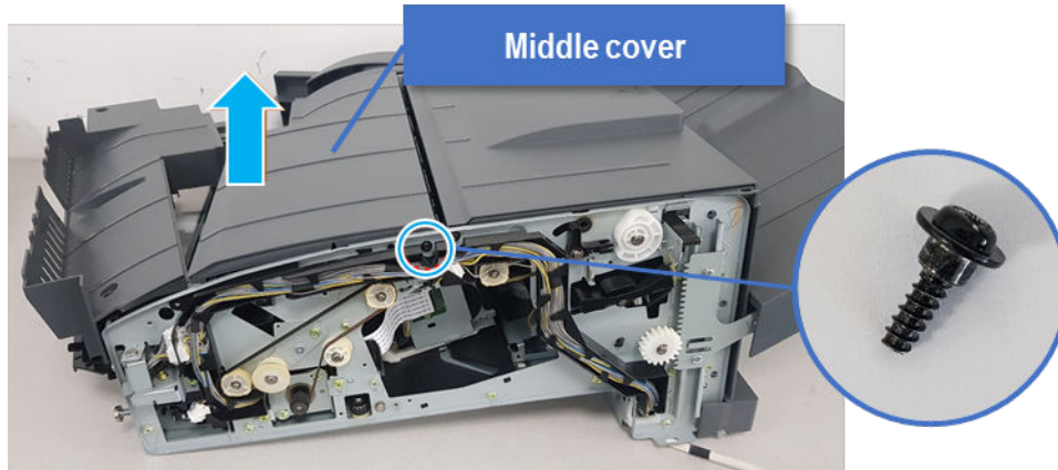
Figure 7-778 Remove the middle cover
