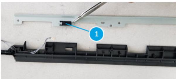
Figure 5-1906 Remove the booklet exit sensor
