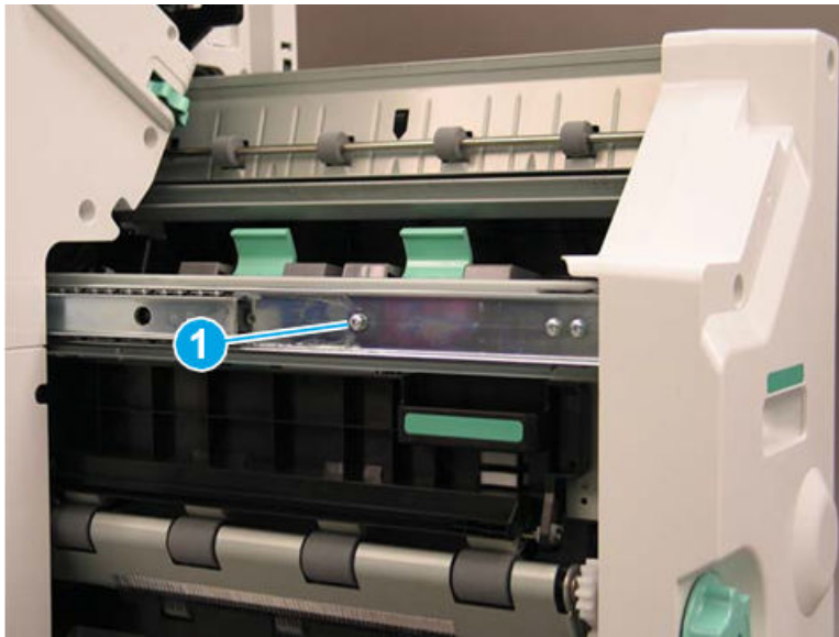
Figure 5-1533 Remove one screw
