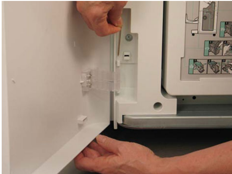
Figure 5-319 Remove the lower hinge pin
