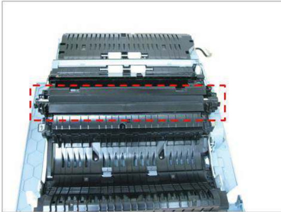
Figure 2-275 Remove transfer roller assembly
