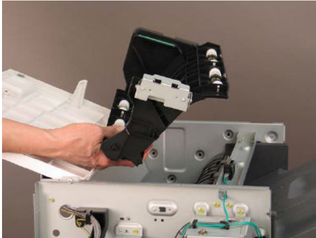
Figure 5-394 Remove the top jam access cover
