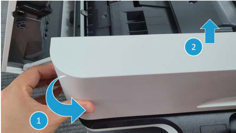
Figure 2-411 Remove the document feeder front cover
