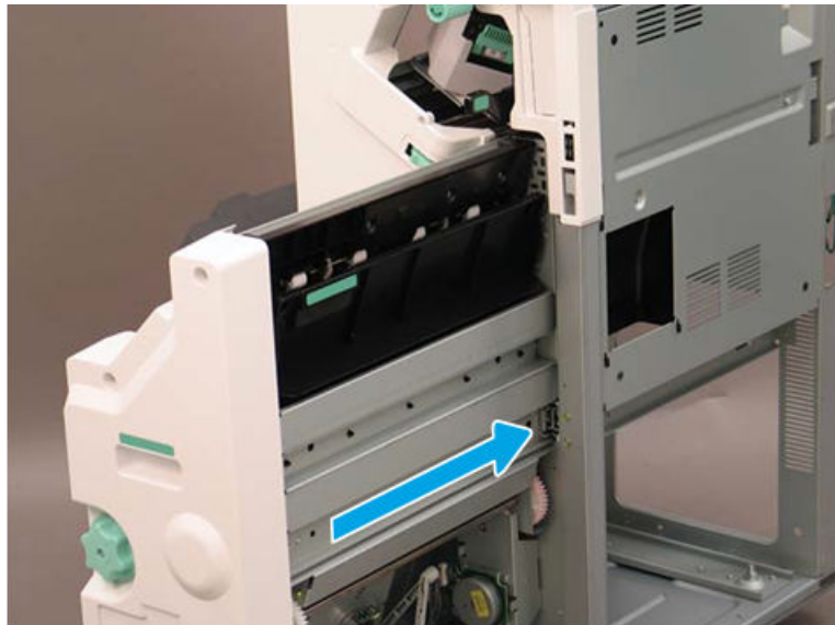
Figure 5-1532 Slide the right rail
