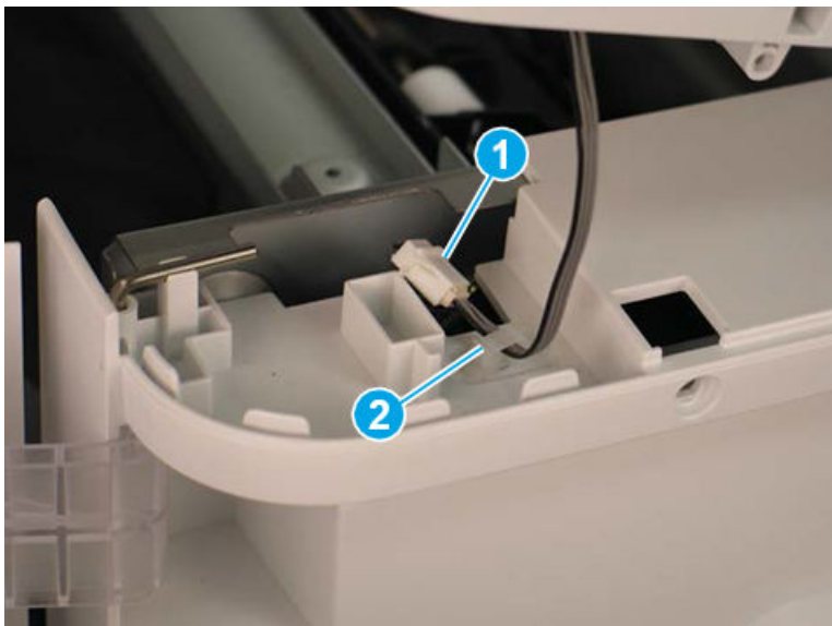
Figure 5-178 Disconnect one connector and release retainer
