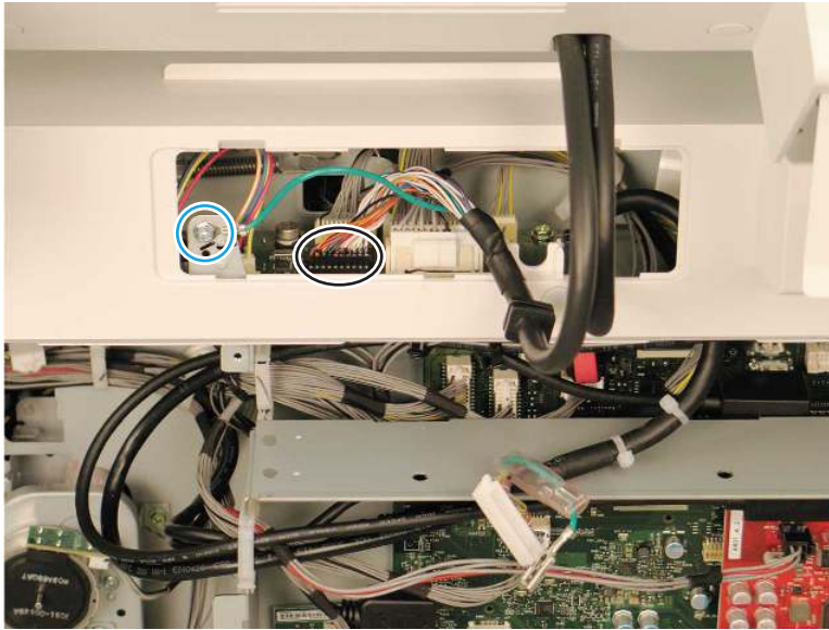
Figure 2-35 Disconnect document feeder harness
