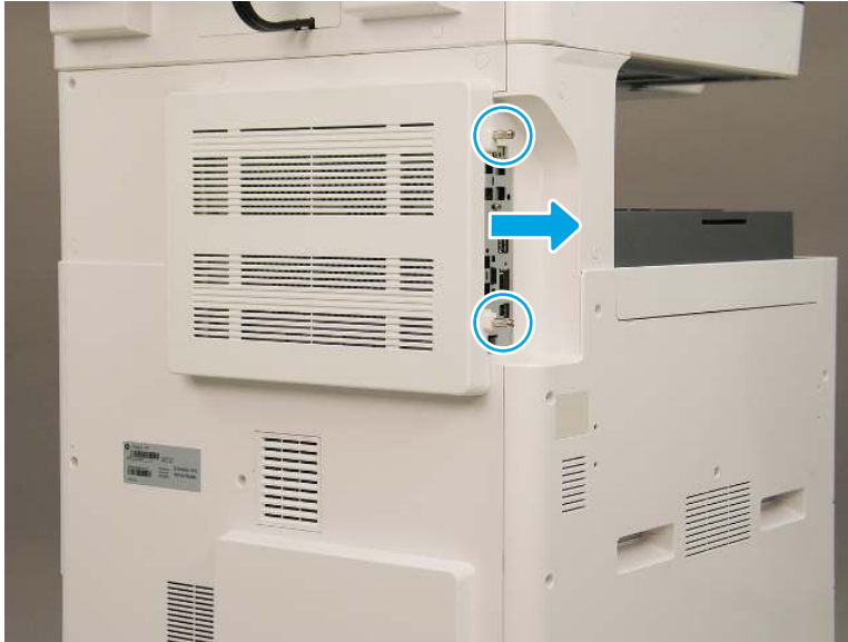
Figure 2-17 Remove the formatter cover
