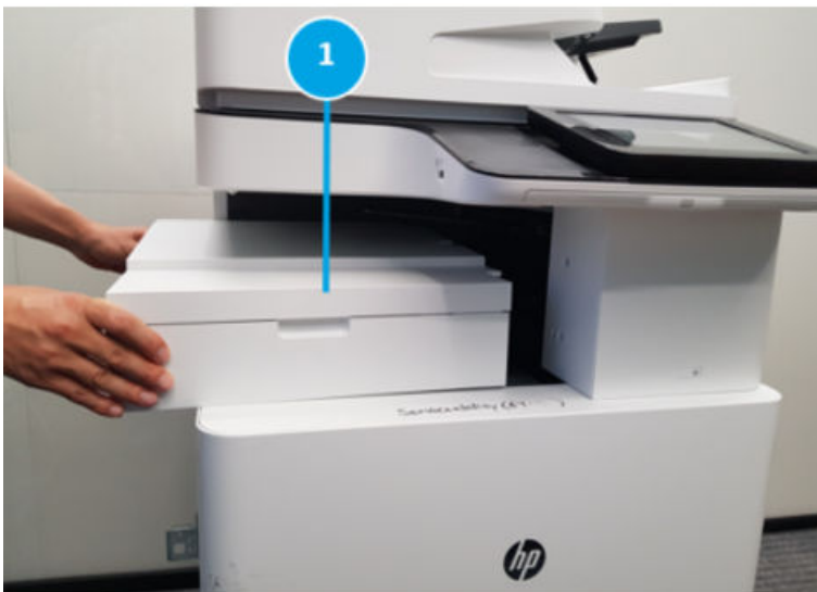
Figure 5-151 Pull out the bridge unit
