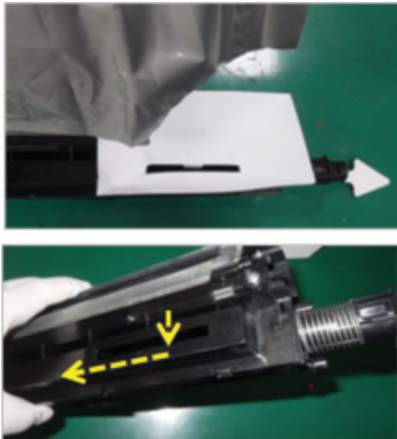
Figure 2-119 Fill developer unit with developer powder
