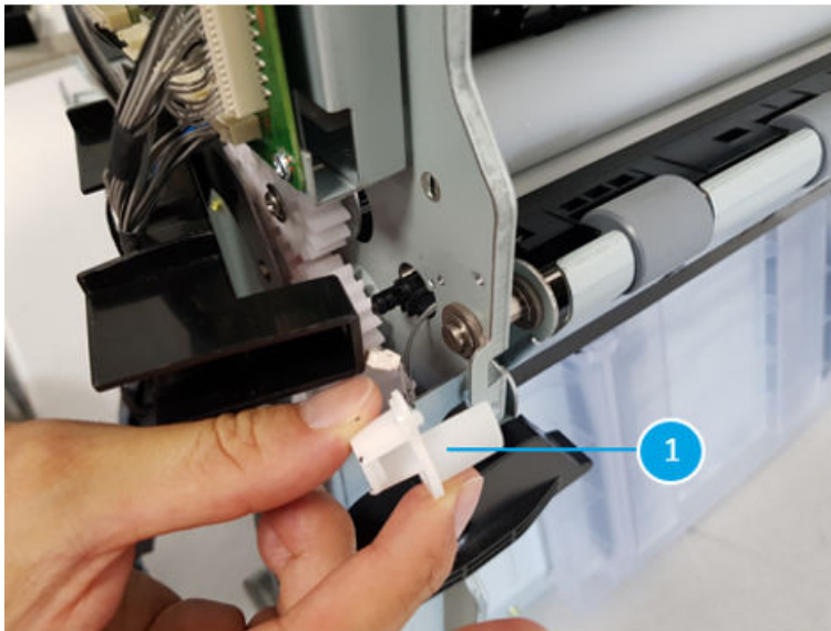
Figure 5-1864 Remove the white bush
