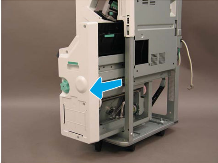
Figure 5-1528 Slide the booklet maker away from the finisher
