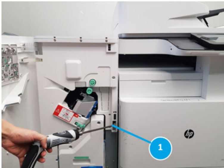
Figure 5-149 Pull the locker out
