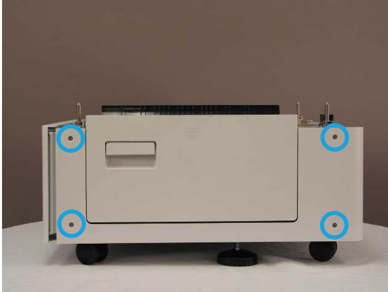
Figure 2-504 Remove four screws
