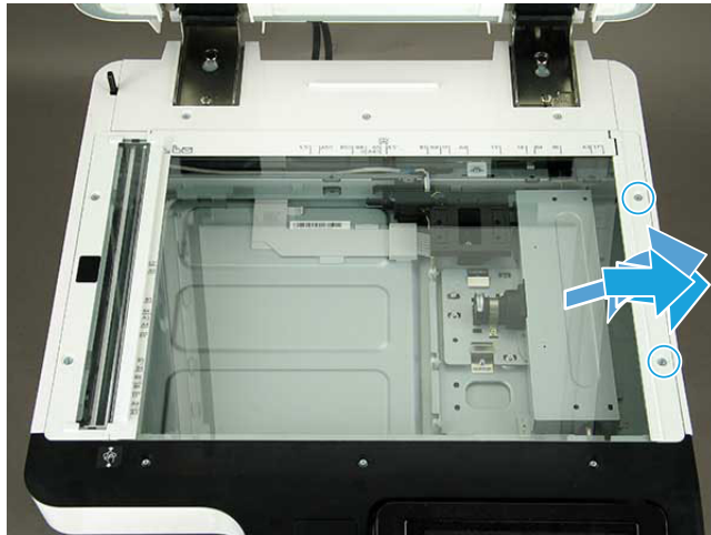
Figure 2-435 Remove scanner glass
