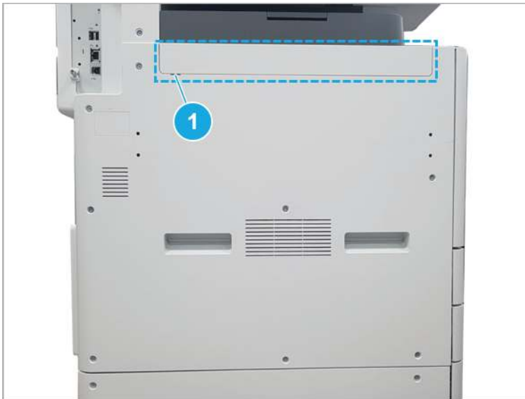
Figure 2-96 Remove the left trim cover
