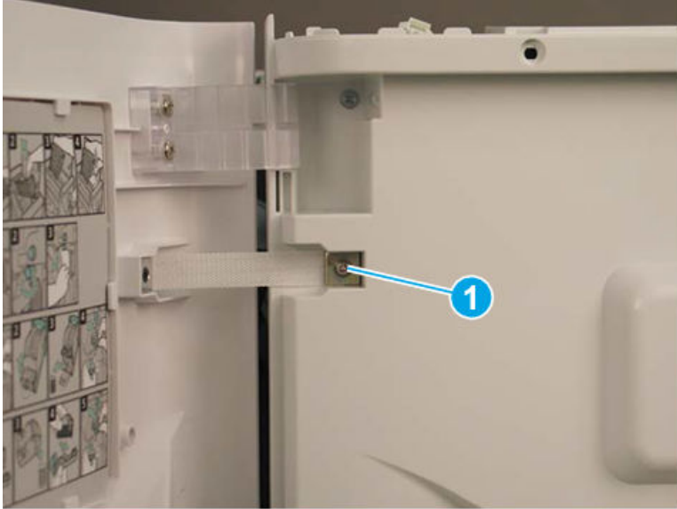
Figure 5-342 Remove the front door
