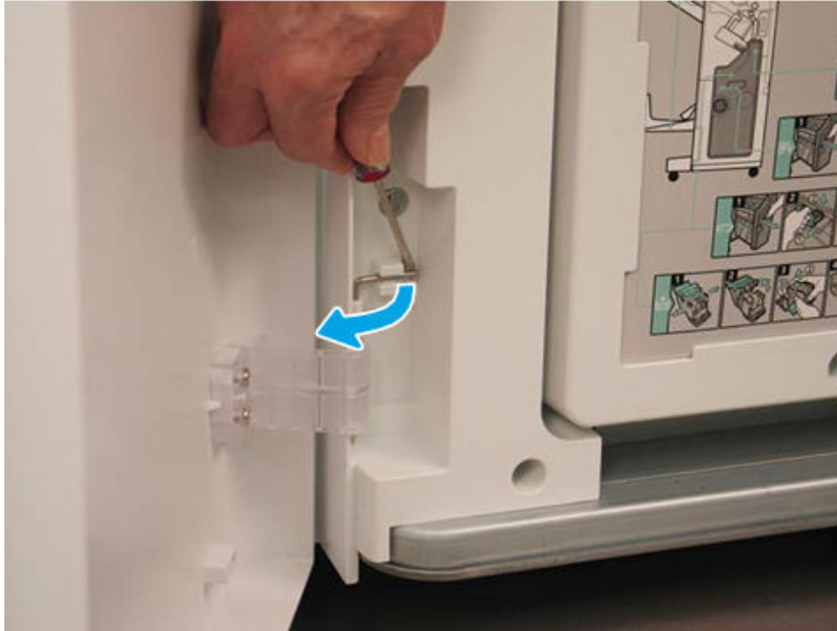
Figure 5-318 Release the lower hinge pin
