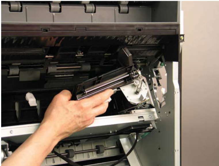
Figure 5-664 Remove the front tamper
