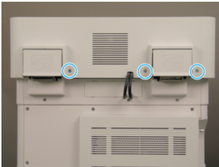
Figure 2-404 Remove the document feeder back cover bottom screws
