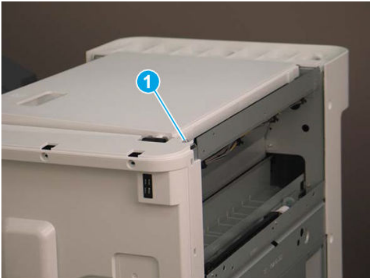
Figure 5-236 Remove one screw
