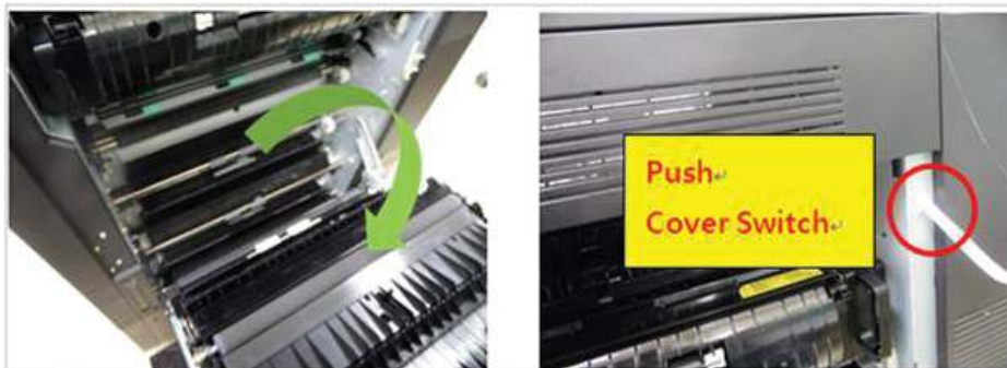
Figure 3-72 Open right door and push cover switch
