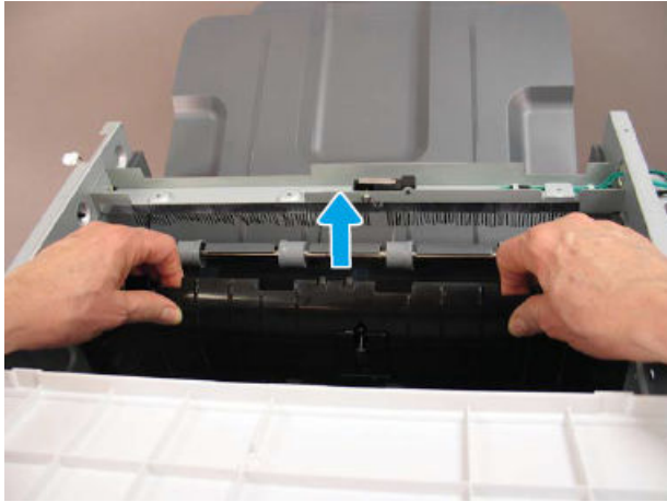
Figure 5-398 Remove the top lower feed assembly
