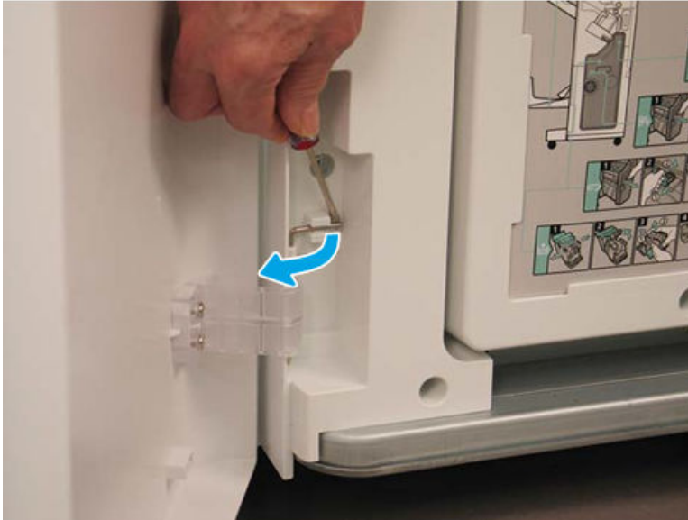
Figure 5-1388 Release the lower hinge pin
