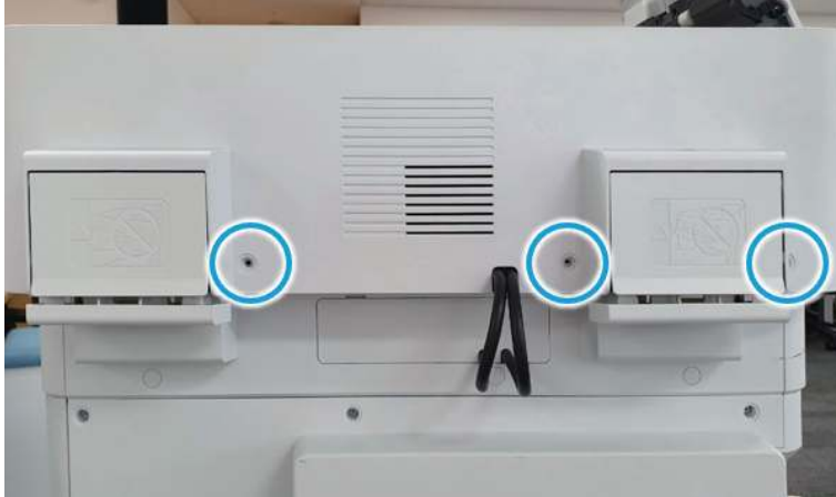
Figure 2-316 Remove 3 caps and 3 screws.
