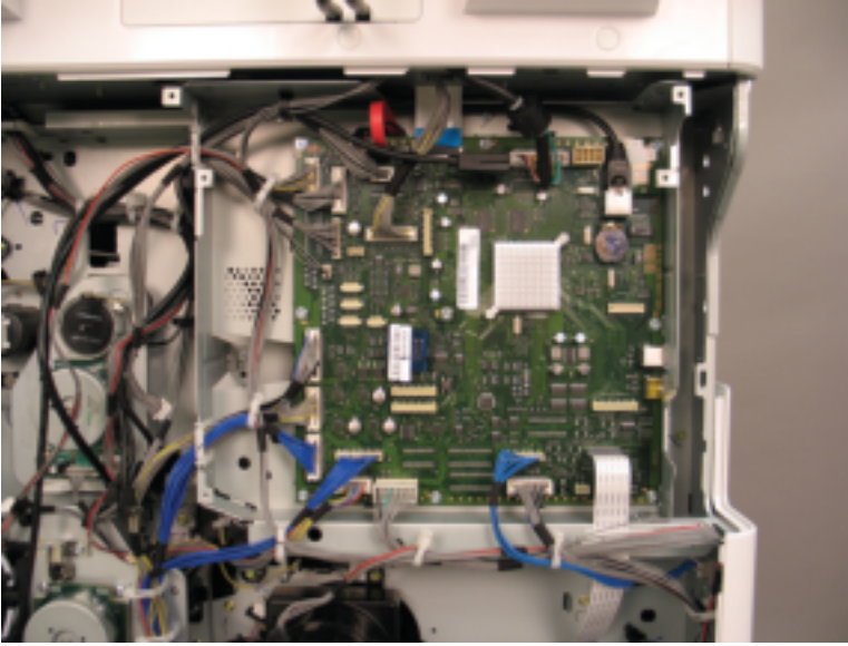
Figure 2-219 Remove the main board connectors and screws
