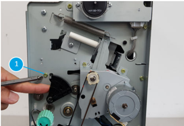
Figure 5-1684 Remove one screw at the front of the booklet maker
