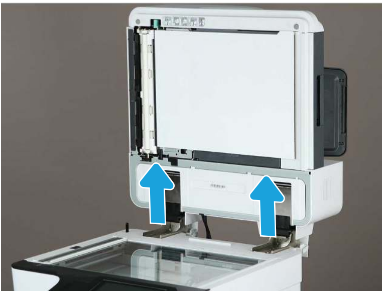
Figure 2-30 Release the document feeder
