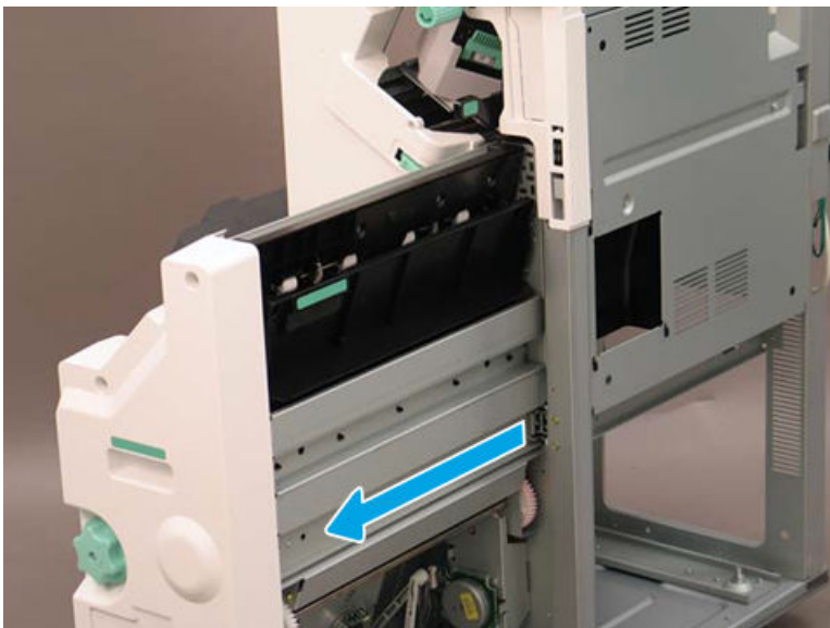
Figure 5-1462 Extend the right rail
