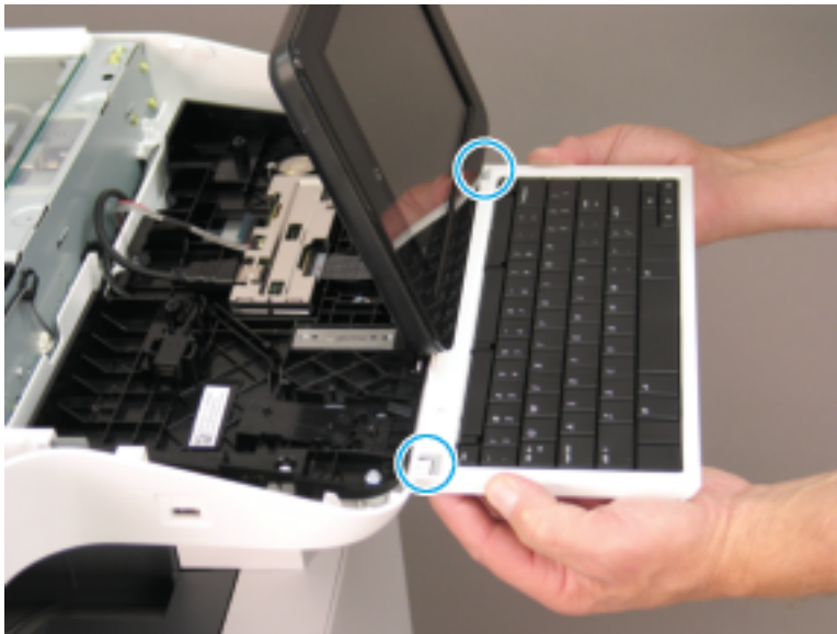
Figure 2-48 Remove the keyboard
