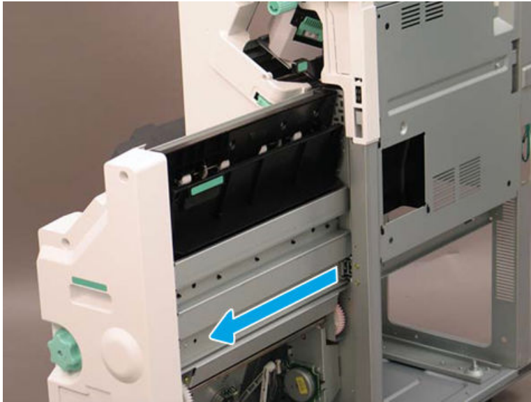
Figure 5-1820 Extend the right rail
