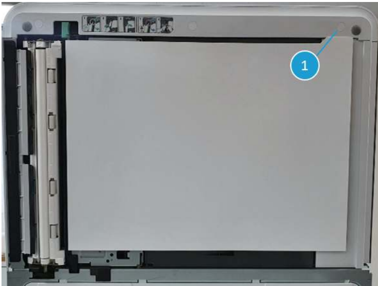
Figure 2-343 Open the document feeder
