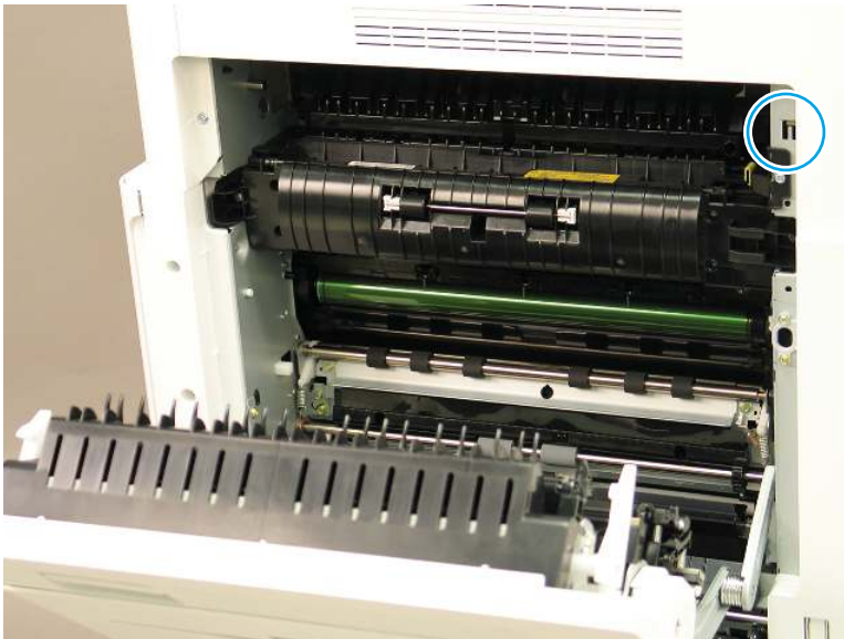
Figure 3-13 Defeat the front door interlock
