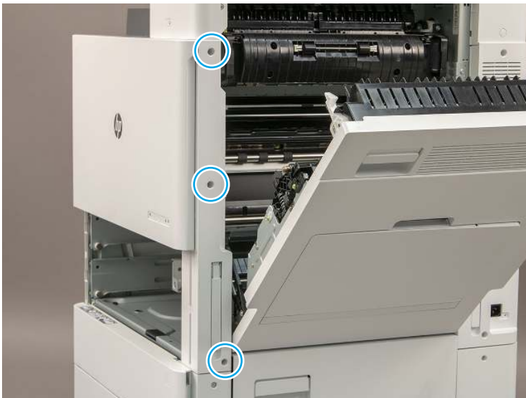
Figure 2-232 Remove the right front cover
