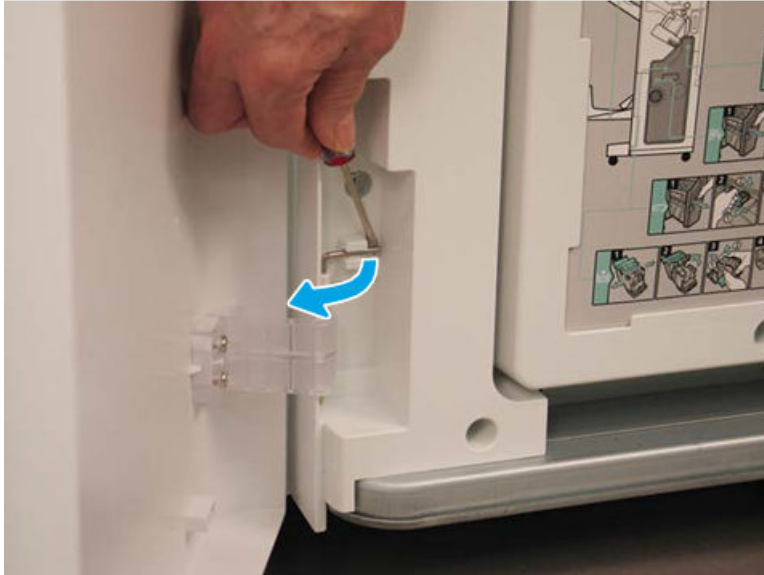
Figure 5-424 Release the lower hinge pin
