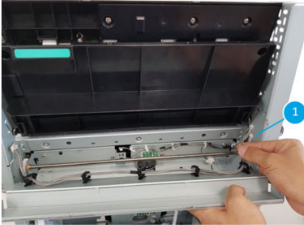
Figure 5-1761 Disconnect one connector
