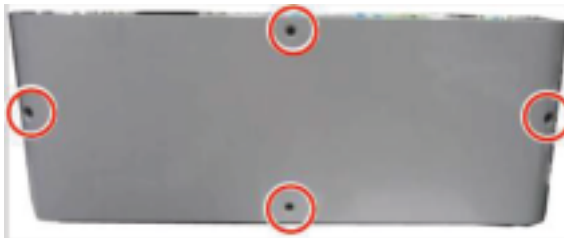
Figure 2-460 Remove the DCF rear cover
