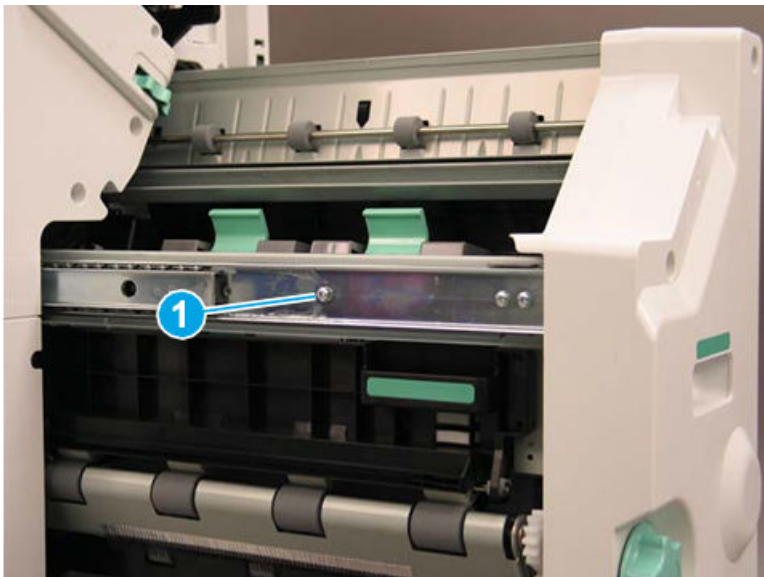
Figure 5-1927 Remove one screw
