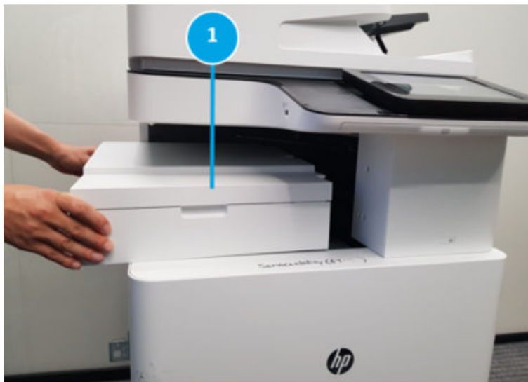
Figure 5-135 Pull out the bridge unit
