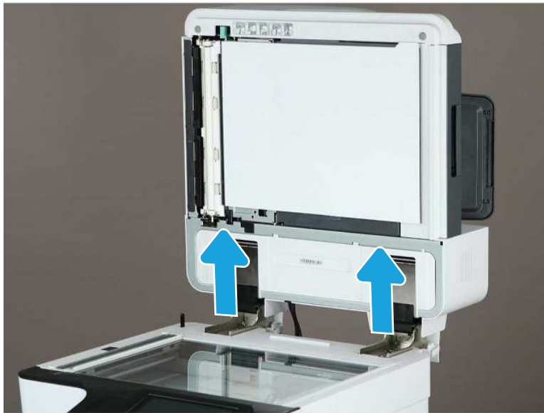
Figure 2-44 Release the document feeder
