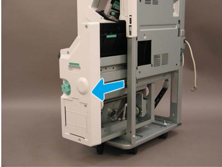
Figure 5-1922 Slide the booklet maker away from the finisher
