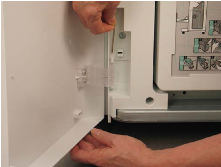
Figure 5-947 Remove the lower hinge pin
