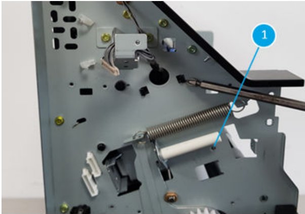
Figure 5-1695 Remove one screw
