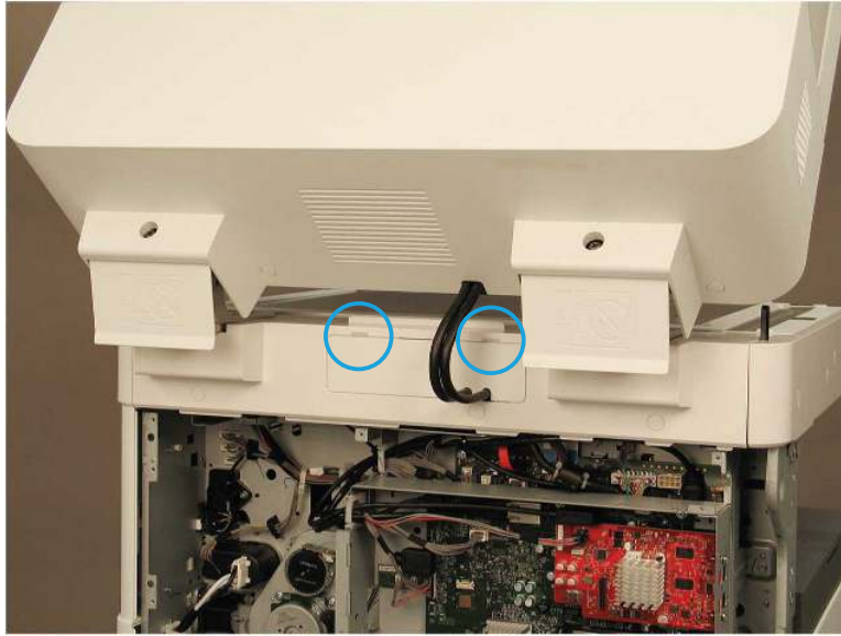
Figure 2-33 Remove document feeder connector cover
