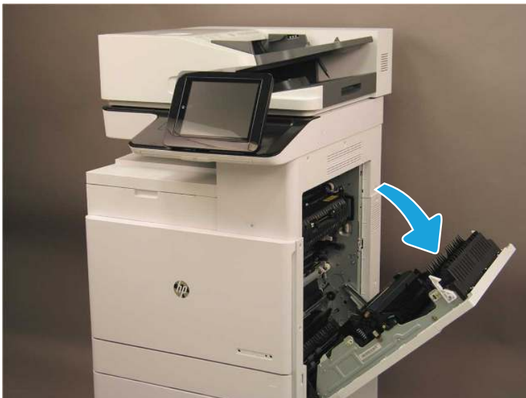
Figure 2-11 Open the right door
