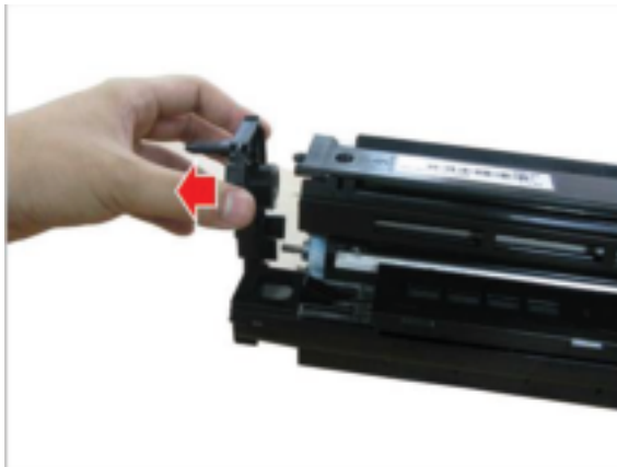
Figure 2-127 Remove rear cover
