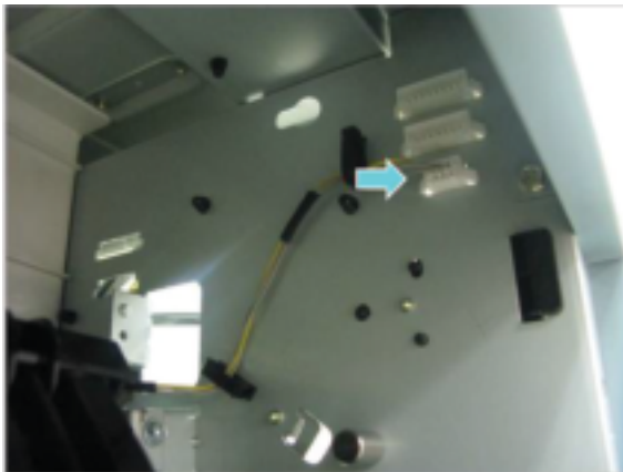
Figure 2-70 Disconnect exit unit connector and cable restraints
