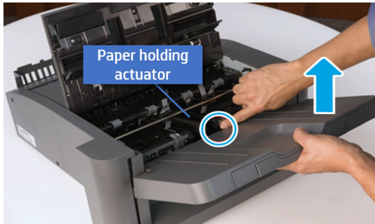
Figure 7-576 Remove the output tray.
