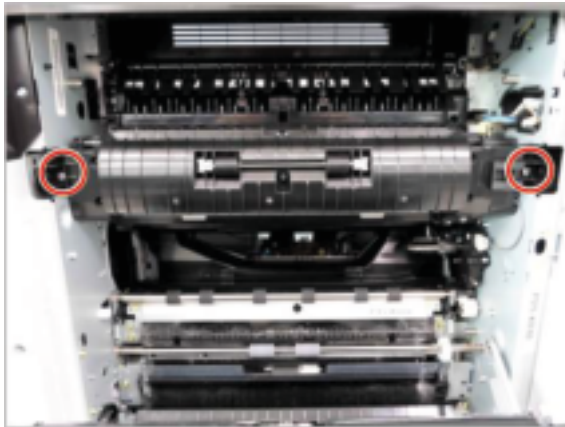
Figure 2-107 Remove two fuser unit screws
