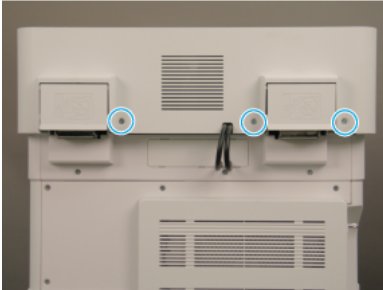
Figure 2-413 Remove the document feeder back cover bottom screws
