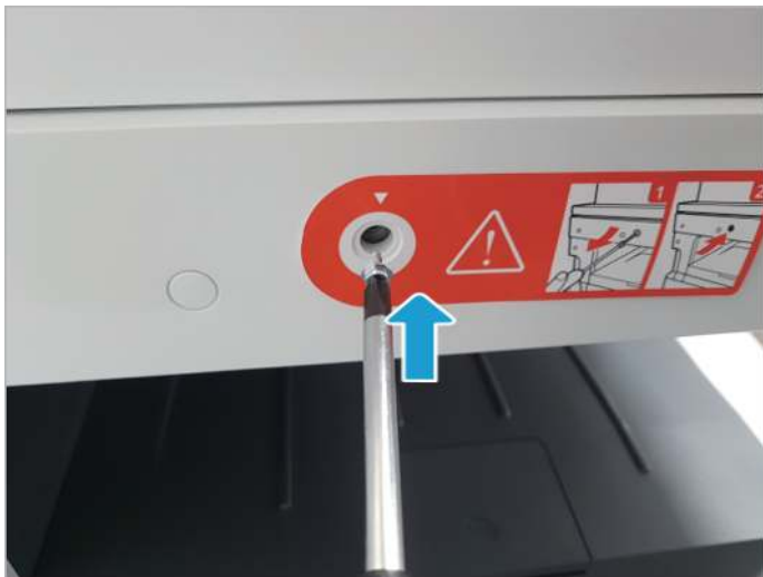
Figure 1-45 Tighten scan locking screw
