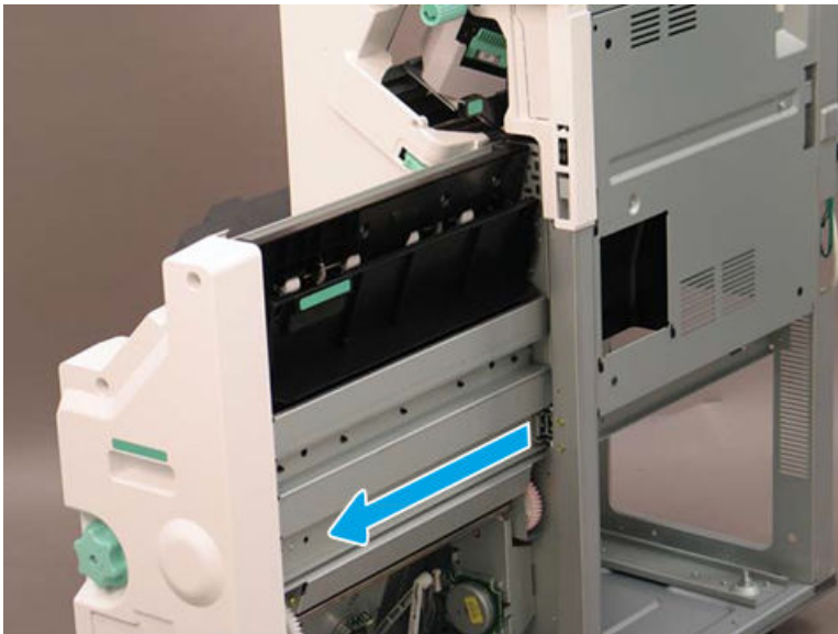
Figure 5-1889 Extend the right rail
