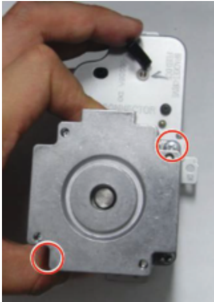
Figure 2-463 Remove the feed motor
