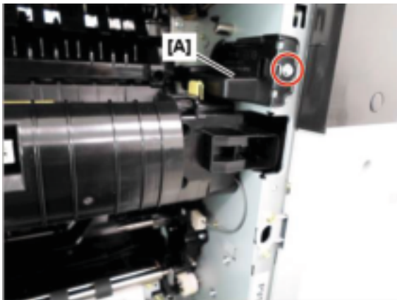
Figure 2-105 Remove one screw
