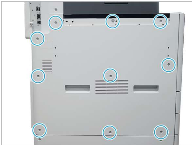
Figure 2-93 Remove the left cover
