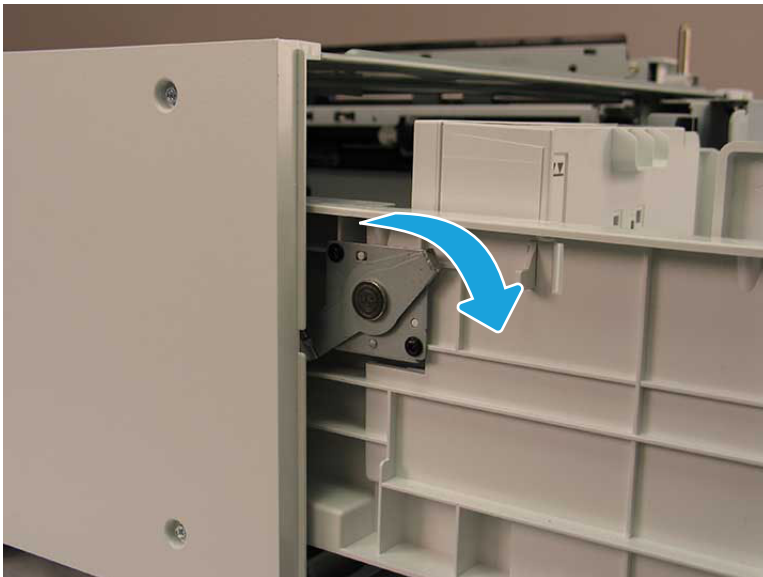
Figure 2-568 Release the tray left side hook lever
