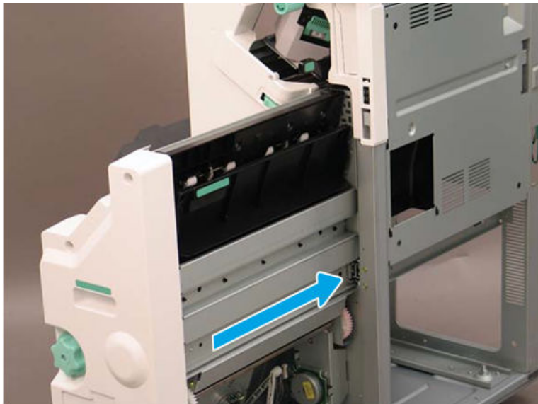
Figure 5-1565 Slide the right rail
