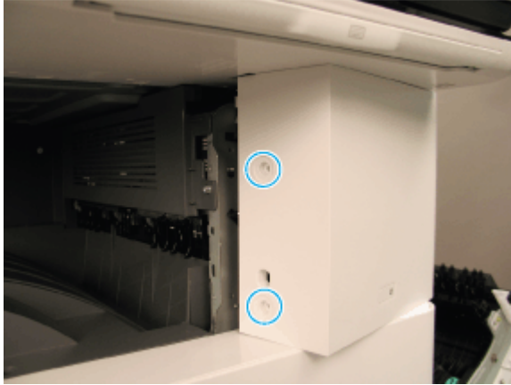
Figure 2-144 Remove the power-switch cover
