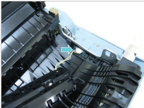
Figure 2-157 Remove right-door exit
