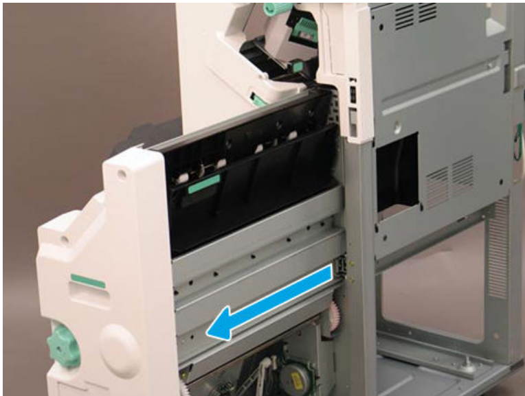
Figure 5-1680 Extend the right rail
