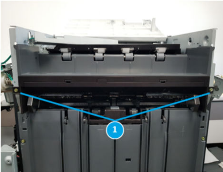
Figure 5-439 Remove two screws
