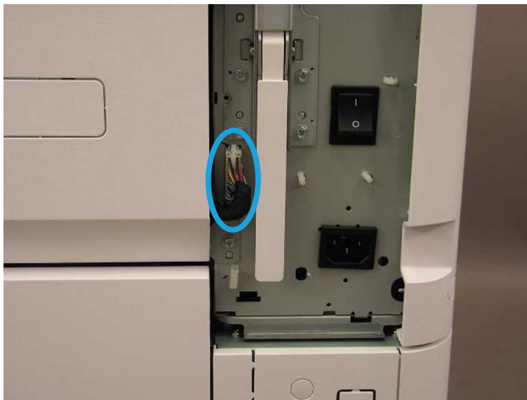
Figure 2-199 Disconnect right door connector
