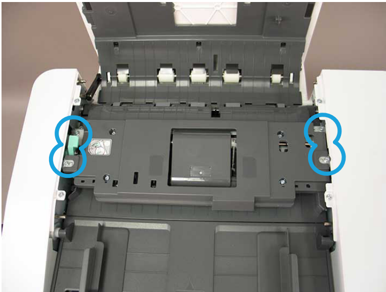
Figure 2-297 Remove four screws
