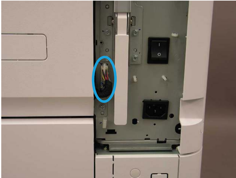
Figure 2-245 Disconnect right door connector
