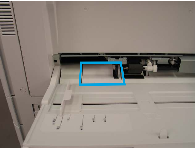
Figure 2-263 Remove MP-cover base
