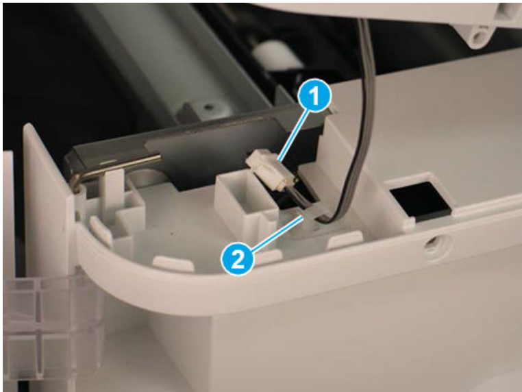
Figure 5-1362 Disconnect one connector and release retainer
