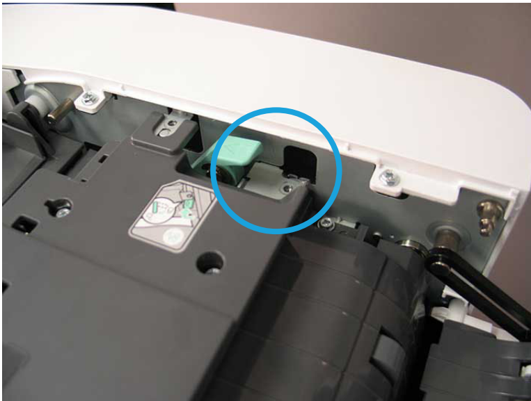
Figure 2-301 Release the sheet metal tab from ADF frame
