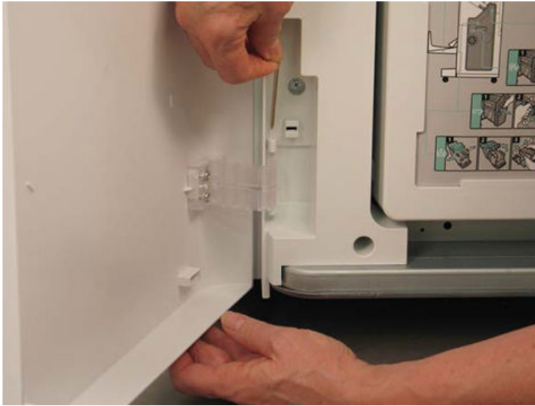
Figure 5-926 Remove the lower hinge pin
