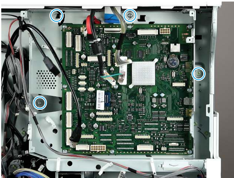
Figure 2-222 Remove the main board cage screws
