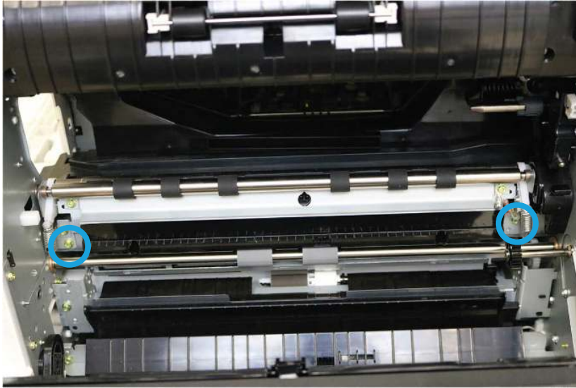
Figure 2-193 Remove screws and guide feed roller
