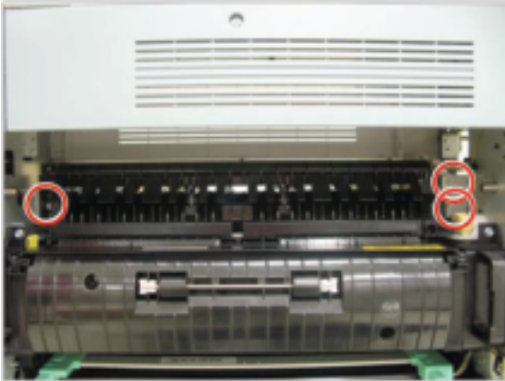
Figure 2-71 Remove screws and exit unit
