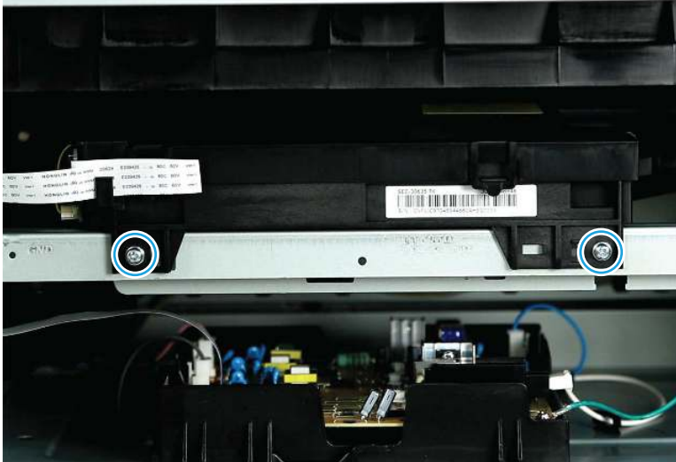
Figure 2-94 Remove the laser scanner assembly
