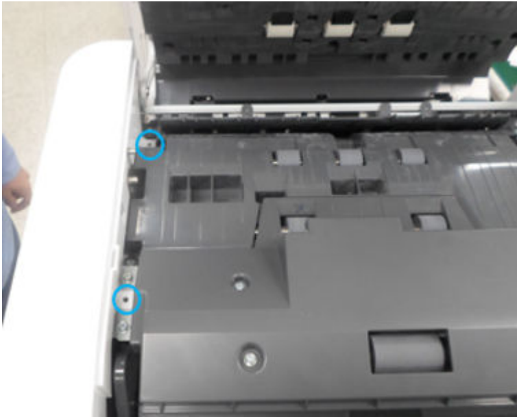
Figure 2-351 Remove the document feeder front cover top screws
