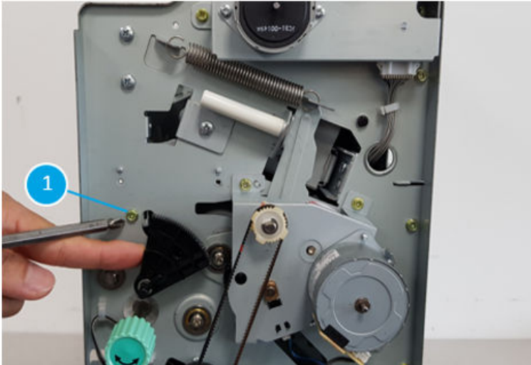
Figure 5-1857 Remove one screw at the front of the booklet maker
