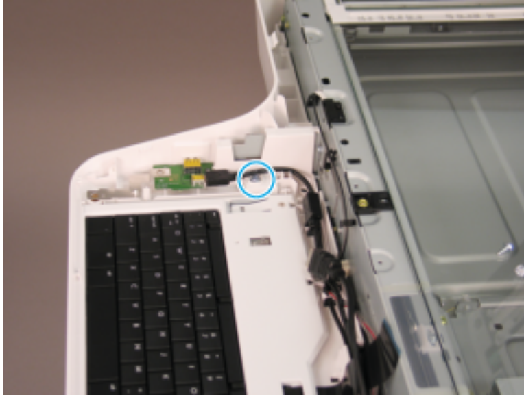
Figure 2-47 Remove USB interconnect cable
