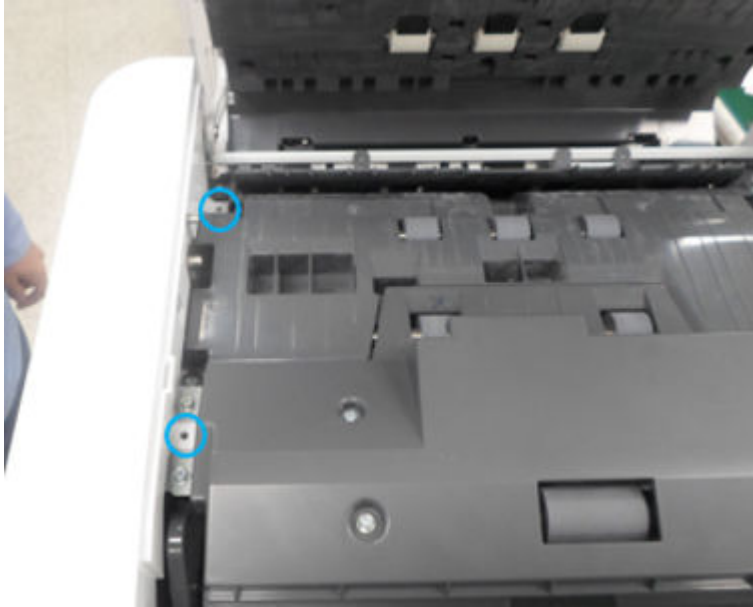
Figure 2-409 Remove the document feeder front cover top screws
