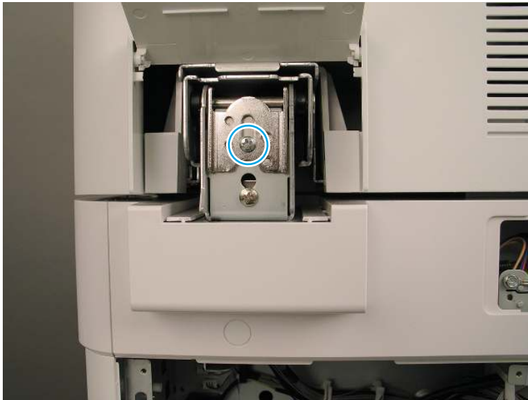
Figure 3-79 Adjust ADF hinge
