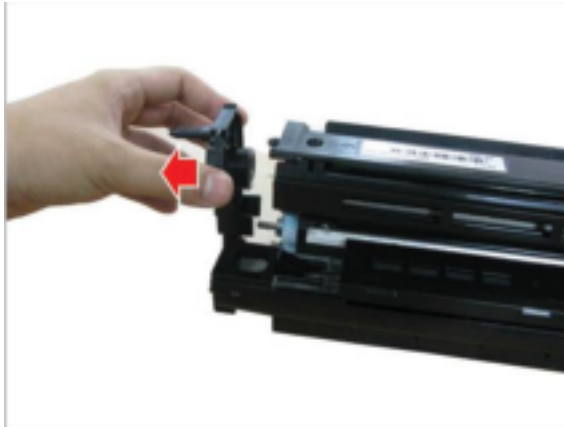
Figure 2-113 Remove rear cover
