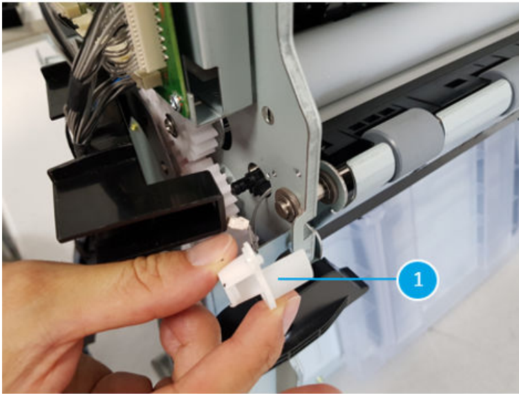
Figure 5-1900 Remove the white bush
