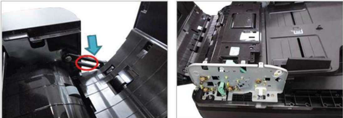
Figure 3-66 Remove linker and front cover
