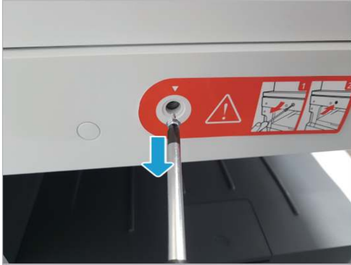
Figure 1-44 Remove scan locking screw
