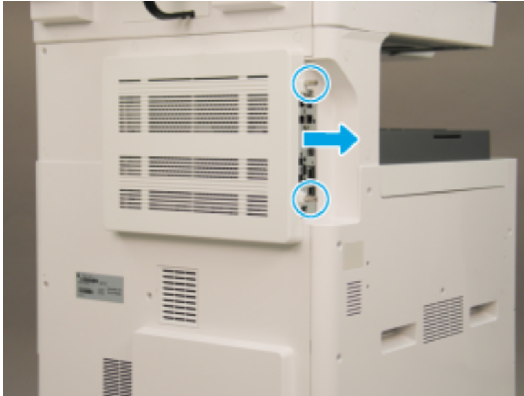
Figure 2-132 Remove the formatter cover
