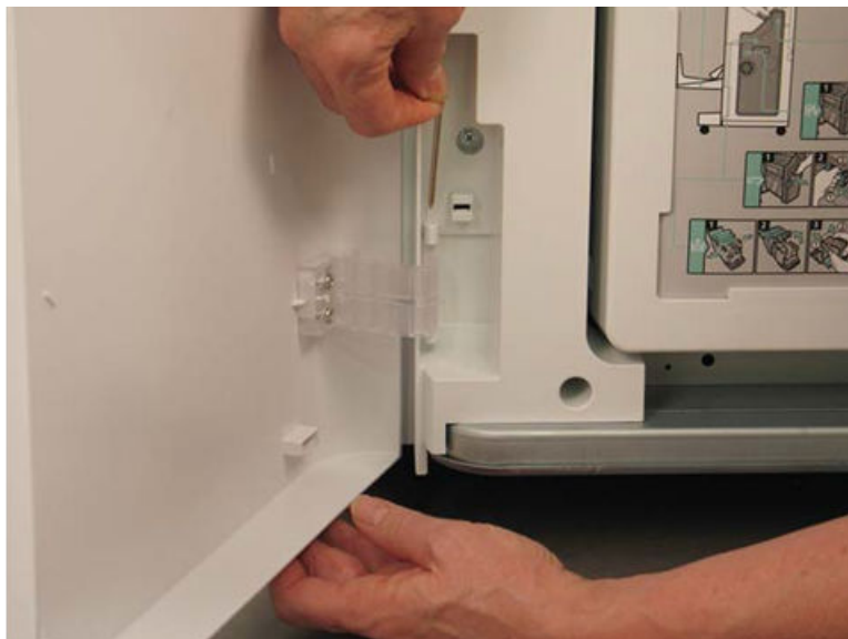
Figure 5-1366 Remove the lower hinge pin
