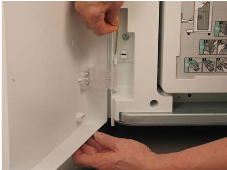
Figure 5-523 Remove the lower hinge pin
