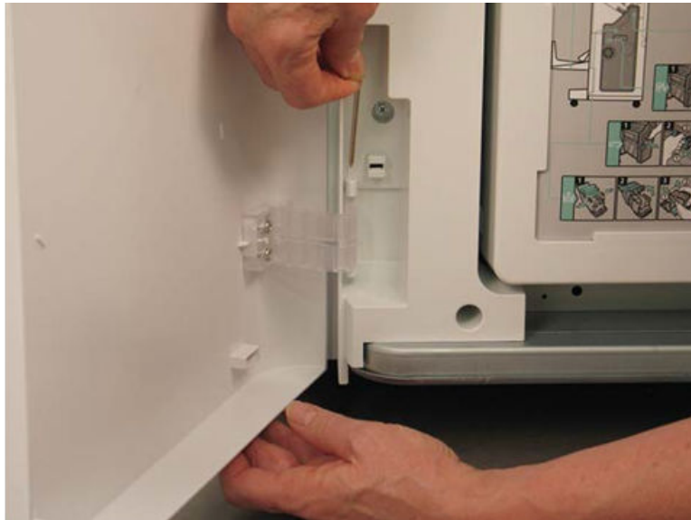
Figure 5-341 Remove the lower hinge pin
