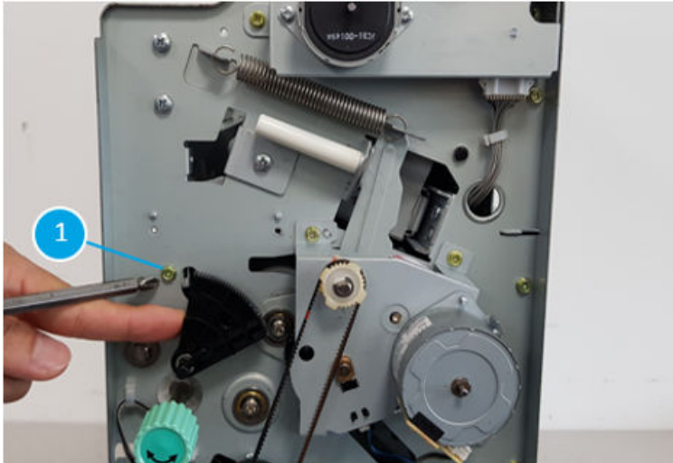
Figure 5-1824 Remove one screw at the front of the booklet maker
