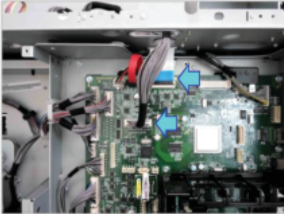
Figure 2-53 Disconnect scan cables
