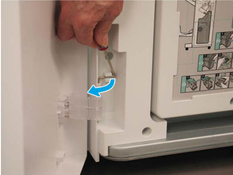
Figure 5-849 Release the lower hinge pin
