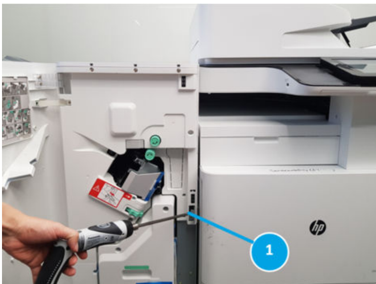
Figure 5-142 Pull the locker out
