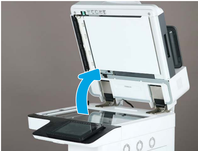
Figure 2-6 Open document feeder unit
