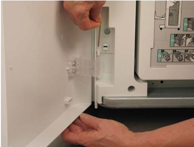
Figure 5-1127 Remove the lower hinge pin
