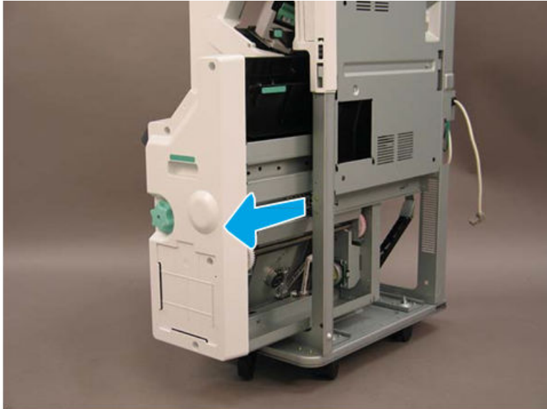
Figure 5-1879 Slide the booklet maker away from the finisher
