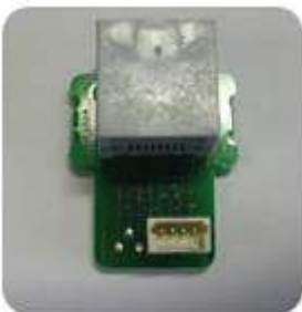
Figure 1-80 Toner CRUM joint PCA
