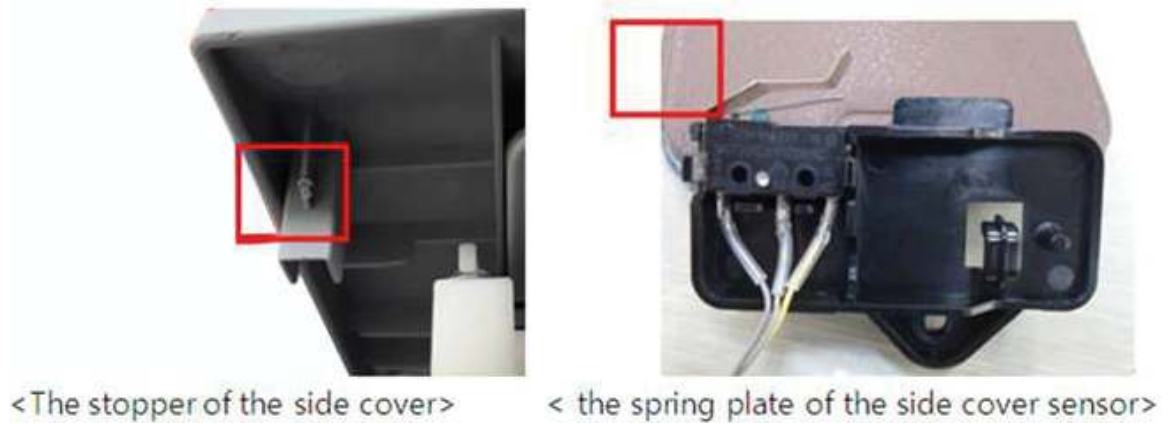
Figure 3-74 Right door sensor spring plate is damaged
