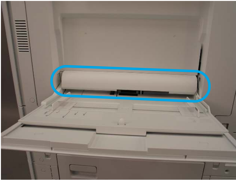
Figure 2-270 Remove the cover
