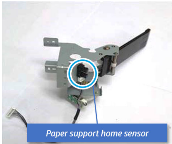
Figure 7-236 Remove the paper support home sensor
