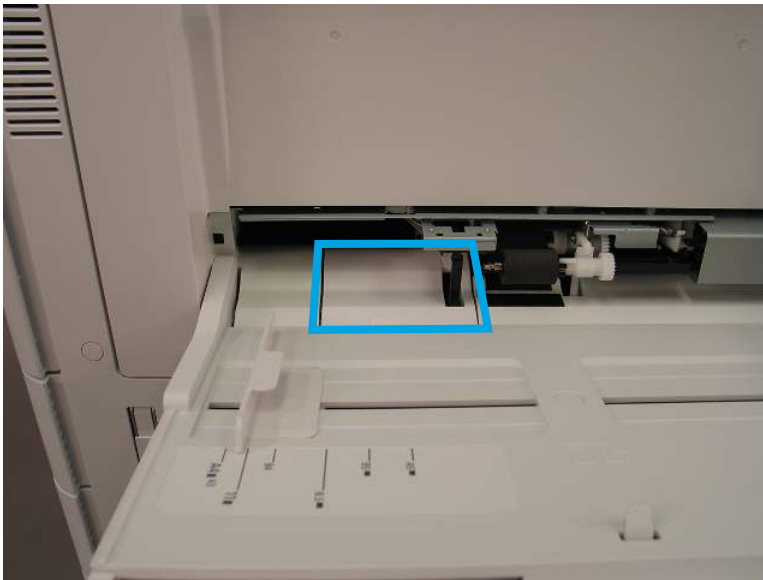
Figure 2-271 Remove the cover
