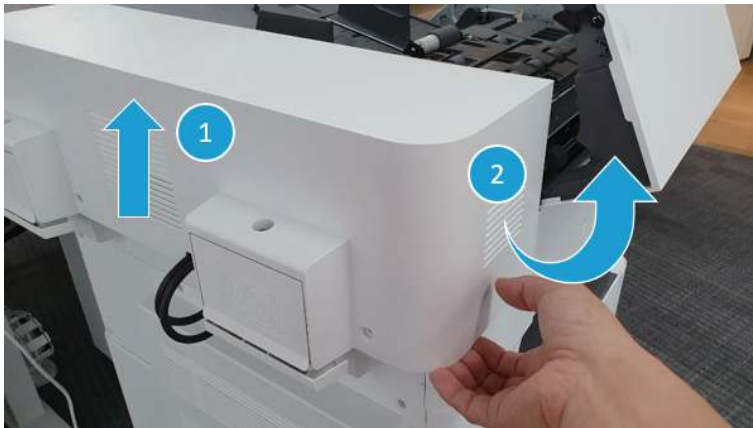
Figure 2-317 Release the top back cover.
