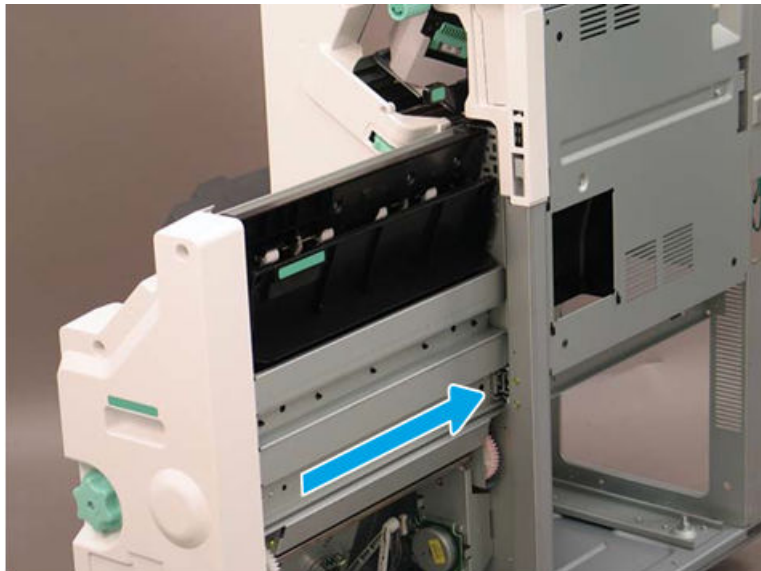
Figure 5-1456 Slide the right rail
