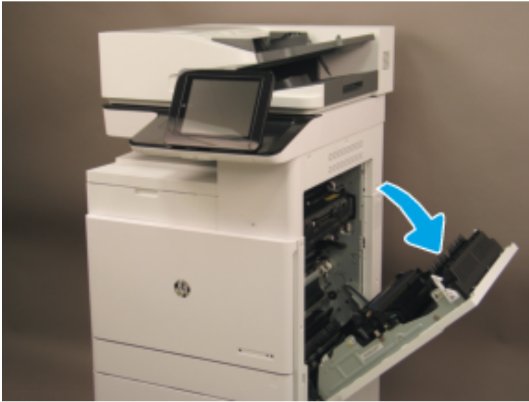
Figure 2-226 Open right door
