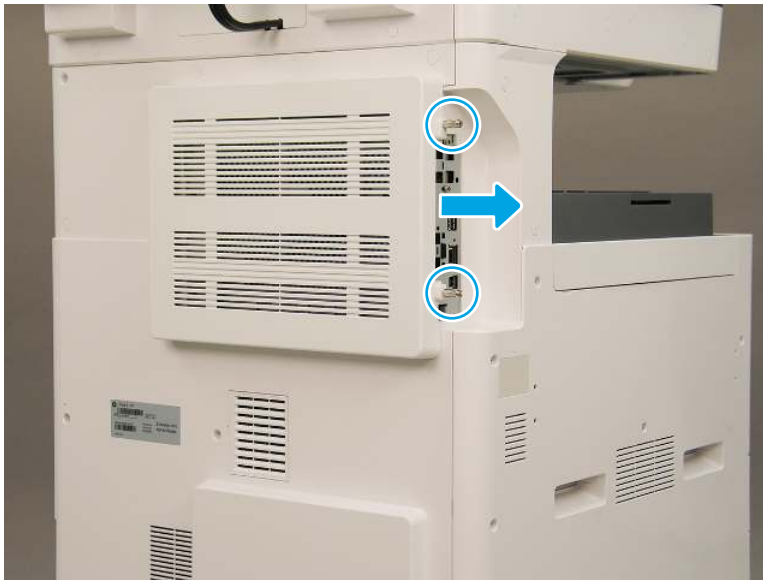
Figure 2-129 Remove the formatter cover
