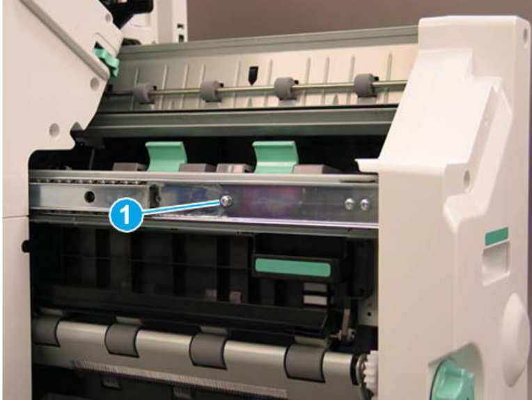
Figure 5-1566 Remove one screw
