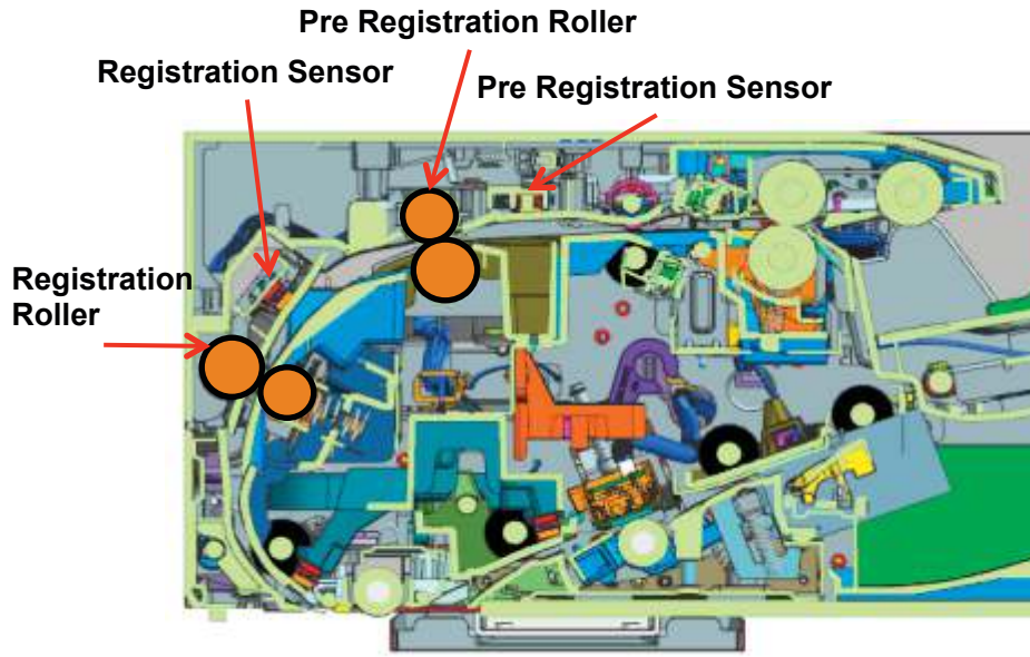
Figure 1-59 Flow document feeder registration
