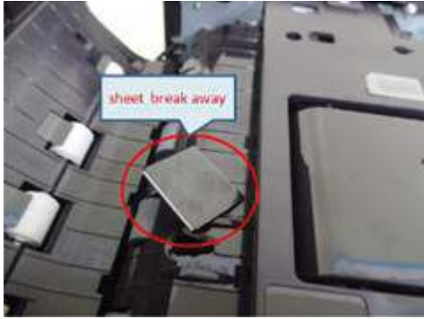
Figure 3-64 Check Sponge-Damper Separation position
