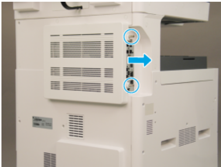
Figure 2-72 Remove the formatter cover
