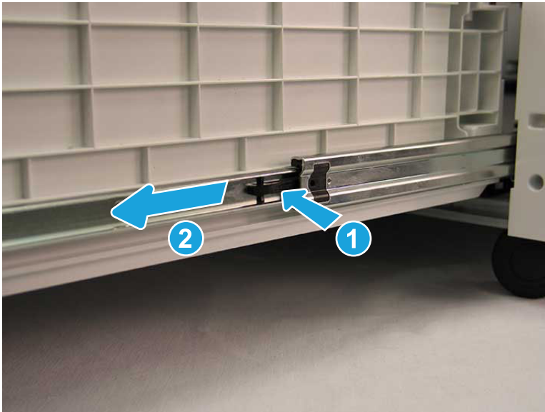
Figure 2-559 Release the tray right-side slide lock
