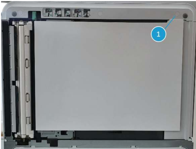
Figure 2-410 Open the document feeder
