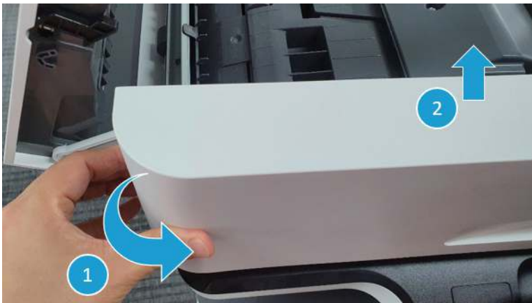
Figure 2-293 Remove the document feeder front cover
