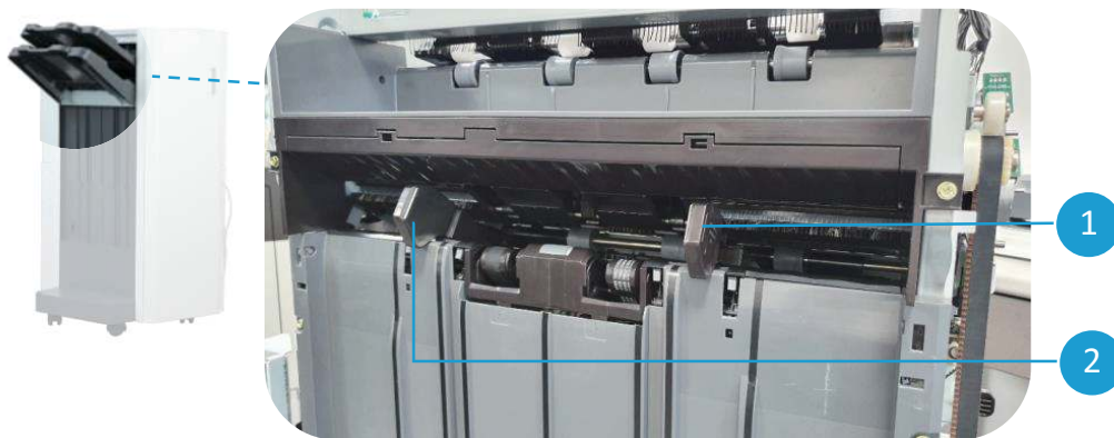
Figure 5-43 Tamper unit detail view - left-right
