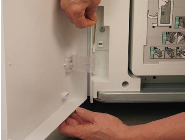
Figure 5-167 Remove the lower hinge pin
