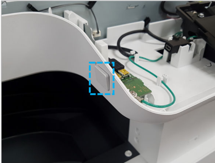
Figure 2-187 Remove the USB cover cap
