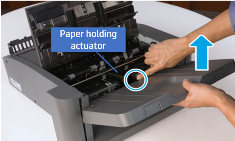
Figure 5-576 Remove the output tray.
