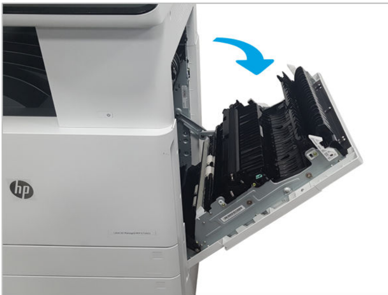
Figure 2-46 Open the right door
