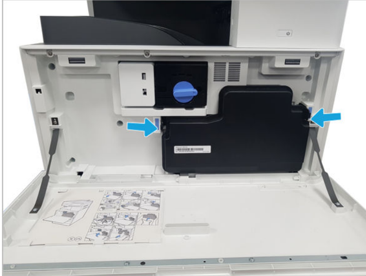
Figure 2-45 Remove the TCU
