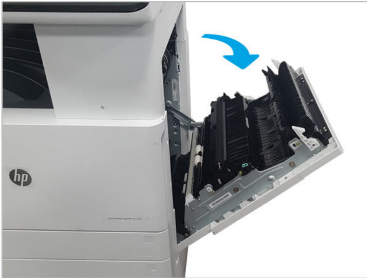
Figure 2-109 Open the right door
