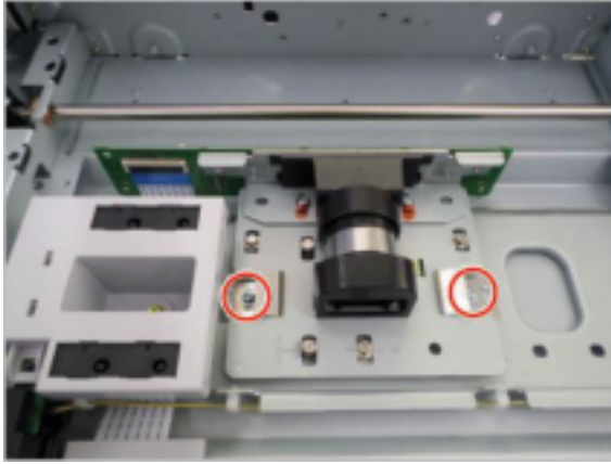
Figure 2-294 Remove screws and release scanner imaging unit
