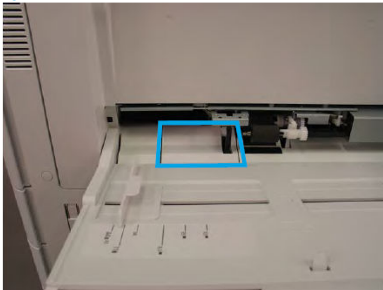
Figure 2-207 Remove the MP sensor cover
