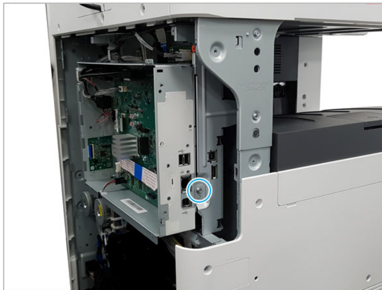
Figure 2-96 Remove the formatter cage side screw
