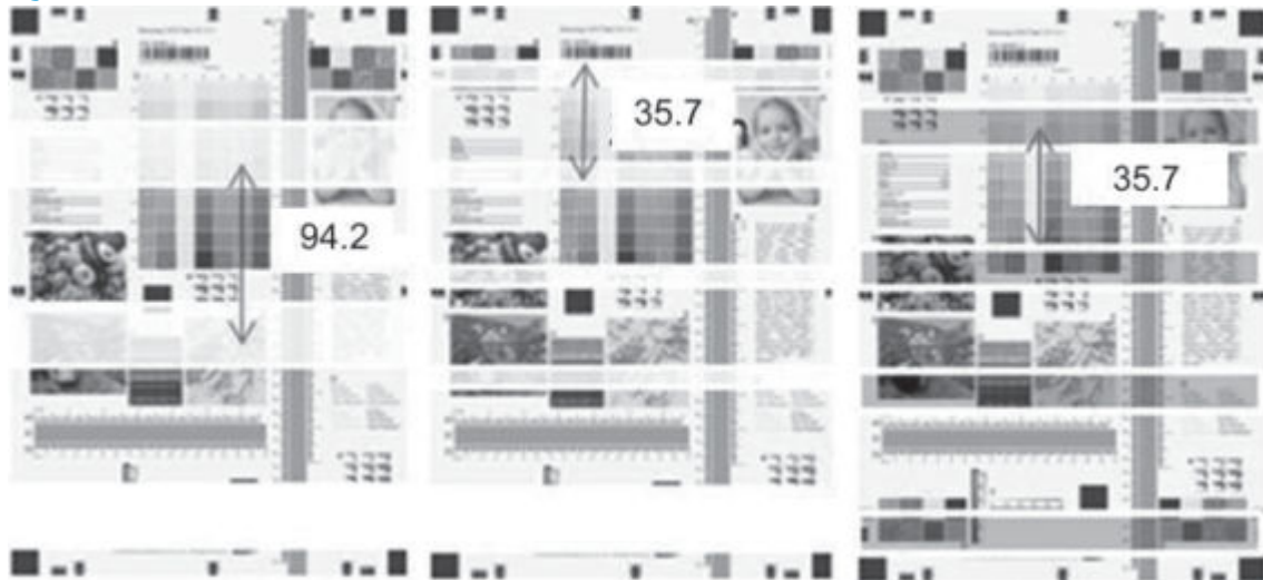
Figure 3-54 Periodic light or dark lines and dots (cross-feed direction)
