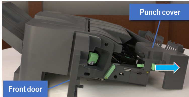
Figure 5-469 Open the front door and punch cover.
