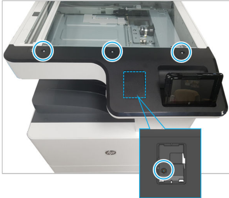
Figure 2-255 Remove the ADF bezel
