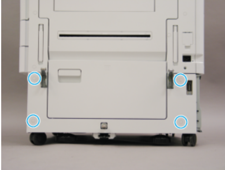
Figure 2-337 Remove the lower right cover
