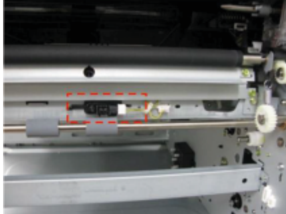
Figure 2-154 Remove feed sensor
