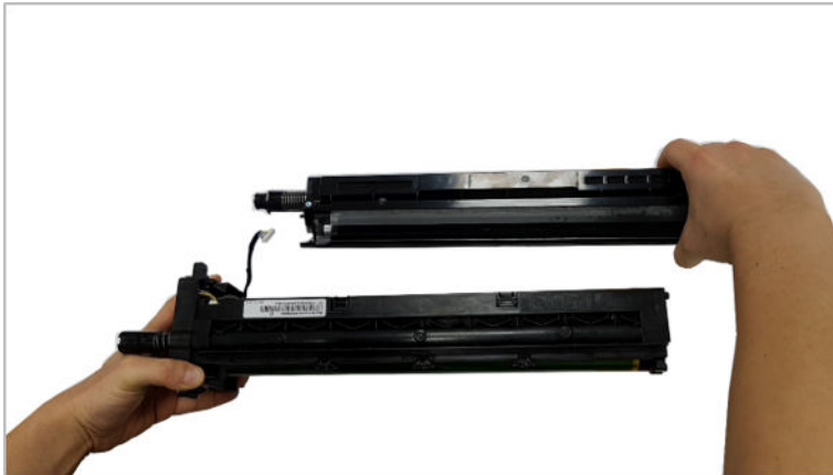
Figure 2-52 Separate developer and drum units
