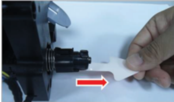
Figure 2-59 Remove arrow label
