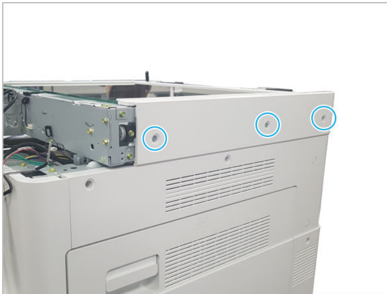
Figure 2-283 Release the right scanner cover
