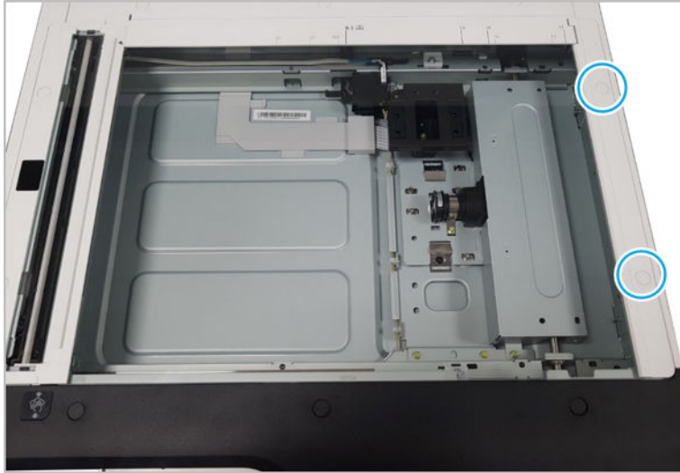
Figure 2-295 Remove screws and scanner glass right cover
