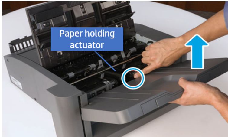
Figure 5-742 Remove the output tray.
