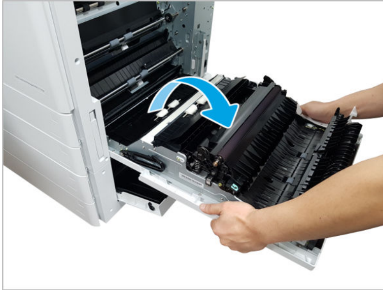
Figure 2-236 Remove right door
