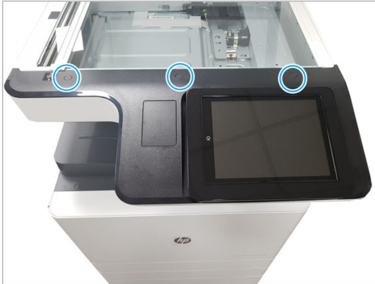
Figure 2-277 Remove the ADF bezel
