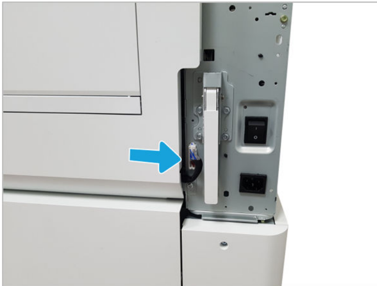
Figure 2-200 Disconnect right door connector
