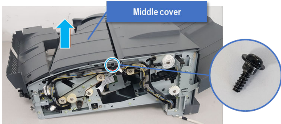
Figure 5-615 Remove the middle cover
