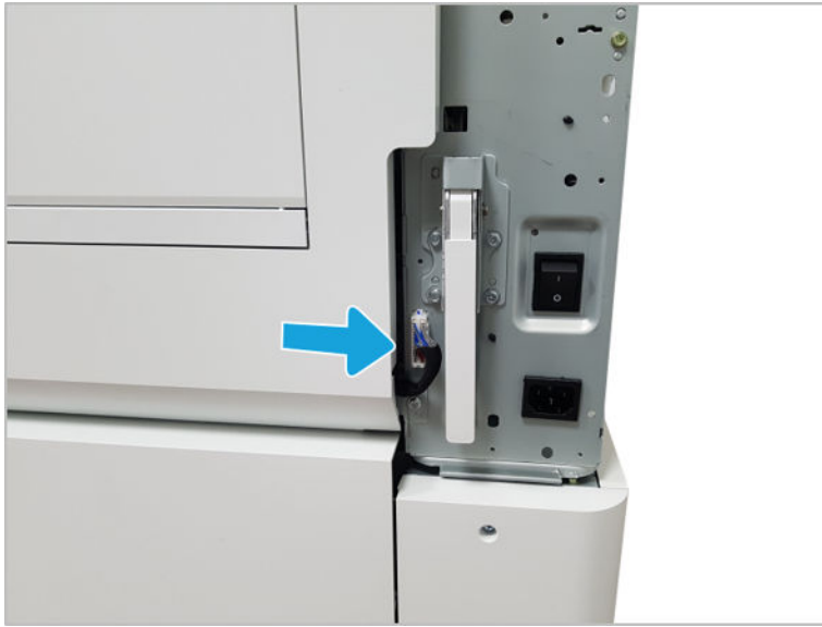
Figure 2-210 Disconnect right door connector
