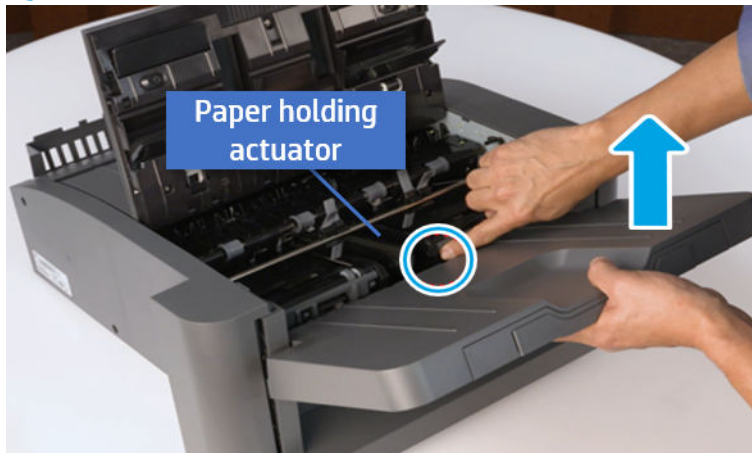
Figure 5-507 Remove the output tray.
