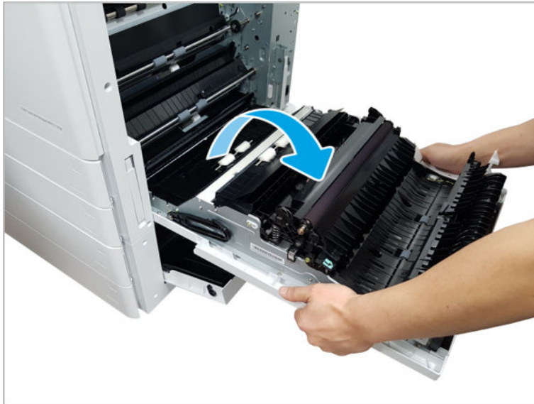
Figure 2-130 Remove right door
