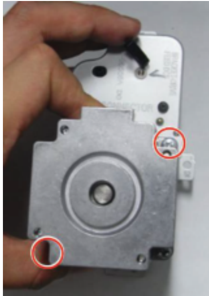
Figure 2-345 Remove the feed motor
