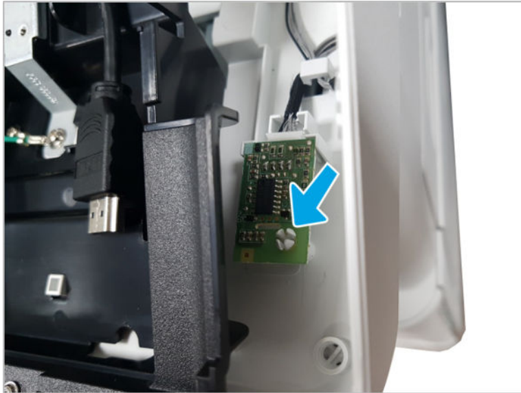
Figure 2-189 Release the latch
