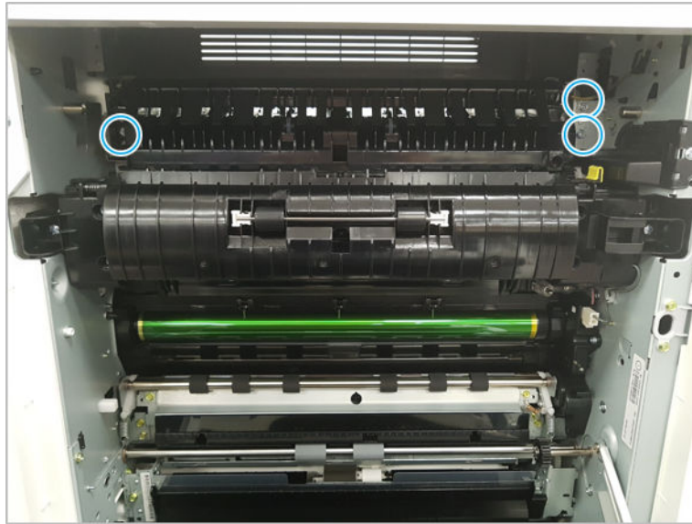
Figure 2-15 Remove screws and exit unit
