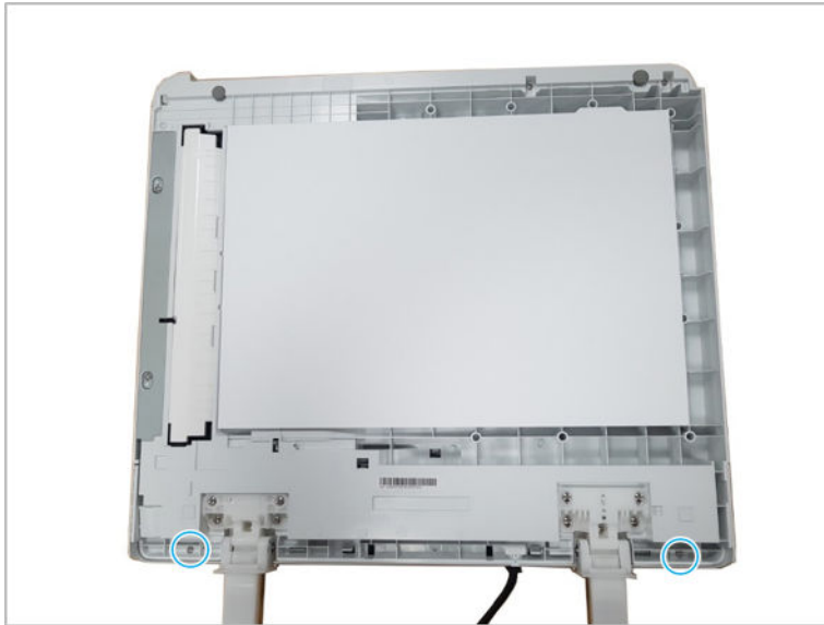
Figure 2-316 Remove two screws and release the hooks
