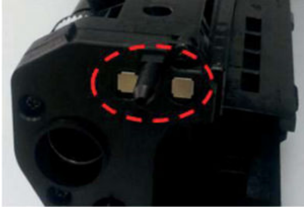
Figure 3-53 Clean contaminated CR terminal
