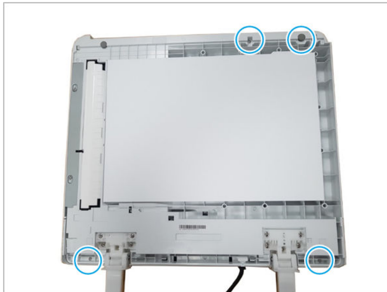
Figure 2-320 Remove four screws and release the hooks
