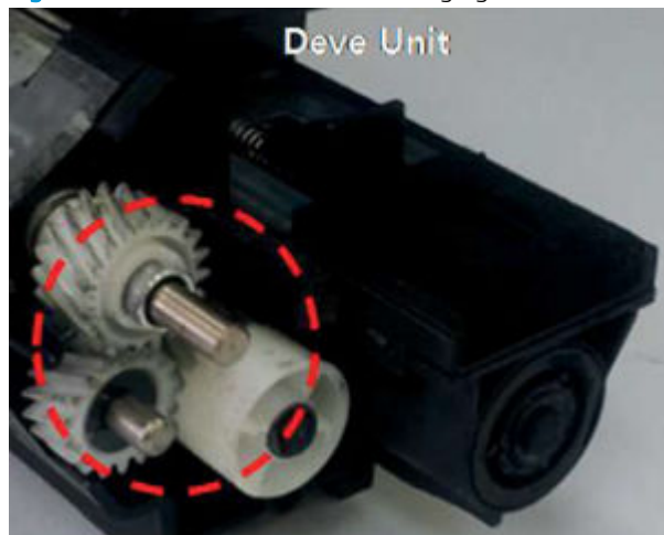
Figure 3-60 Grease the toner cartridge gears
