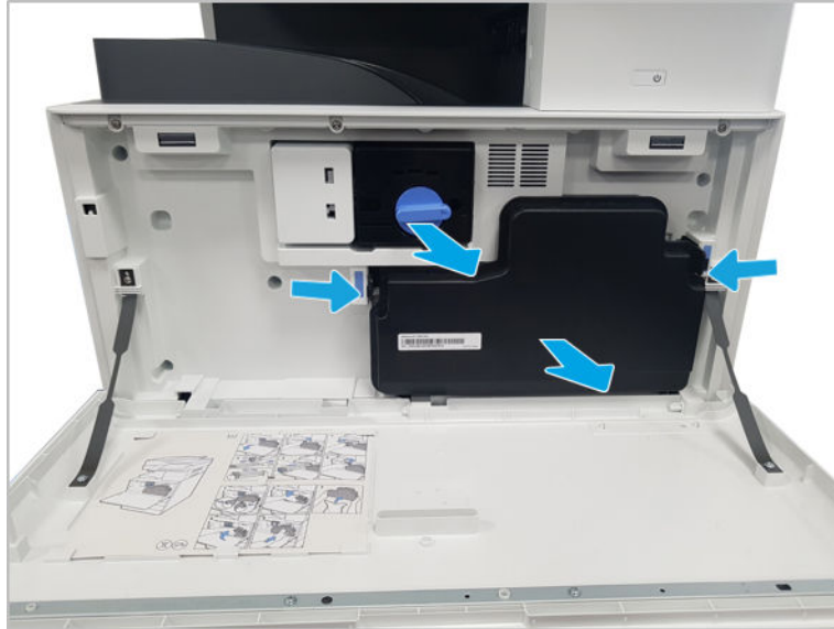
Figure 2-141 Remove the toner cartridge and TCU
