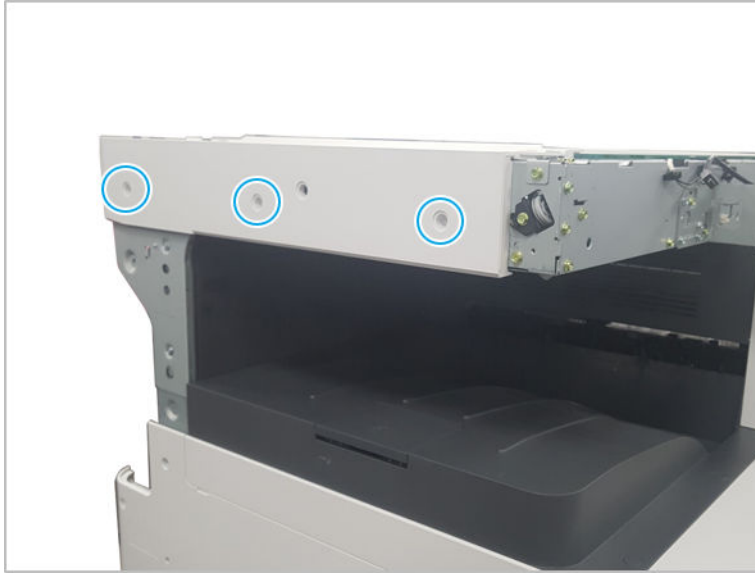
Figure 2-282 Release the left scanner cover
