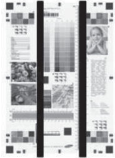
Figure 3-42 Black lines (feed direction)
