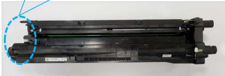
Figure 2-43 Remove the rear cover
