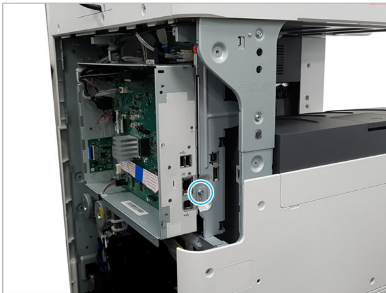
Figure 2-166 Remove the formatter cage side screw
