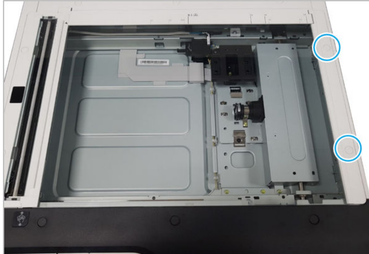
Figure 2-287 Remove scanner glass
