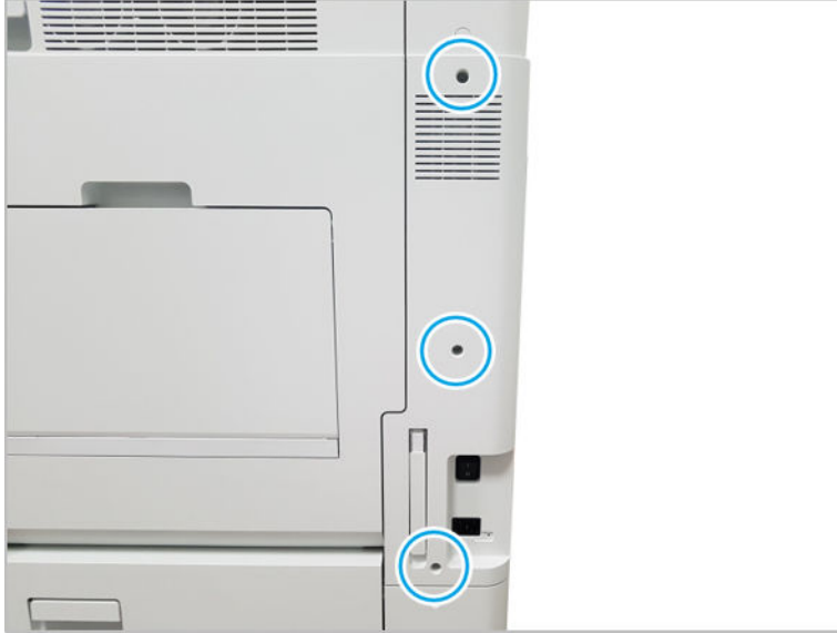
Figure 2-148 Remove the right-rear cover.
