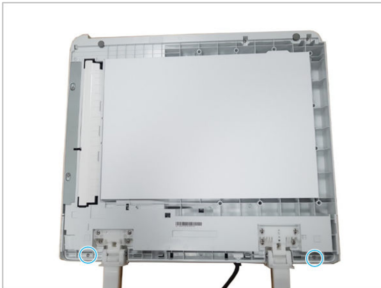
Figure 2-311 Remove two screws and release the hooks
