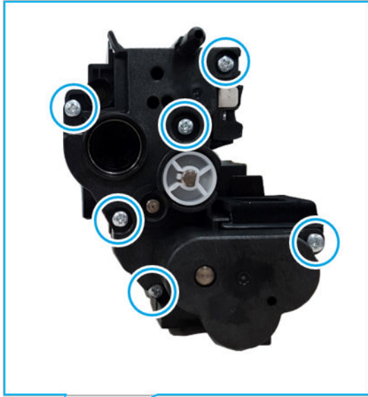
Figure 2-42 Remove six screws
