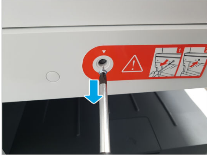
Figure 1-38 Remove the scan locking screw
