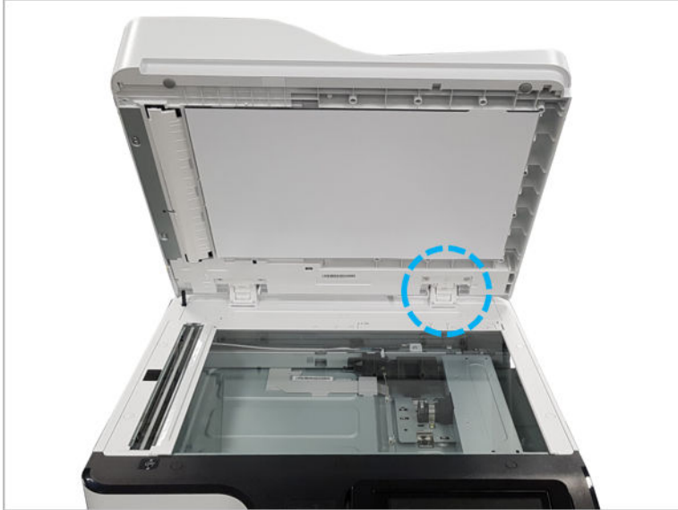
Figure 3-72 Open ADF and loosen screws
