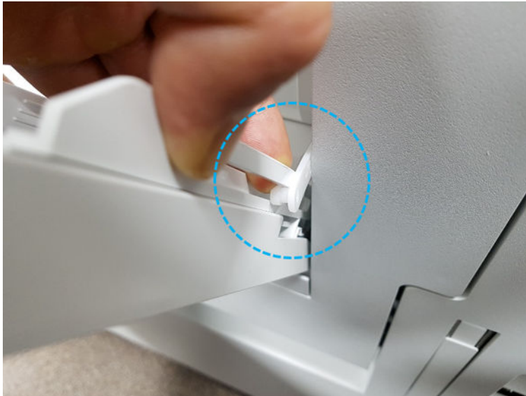
Figure 2-215 Open MP tray and release link
