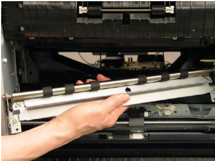
Figure 2-118 Remove the registration unit
