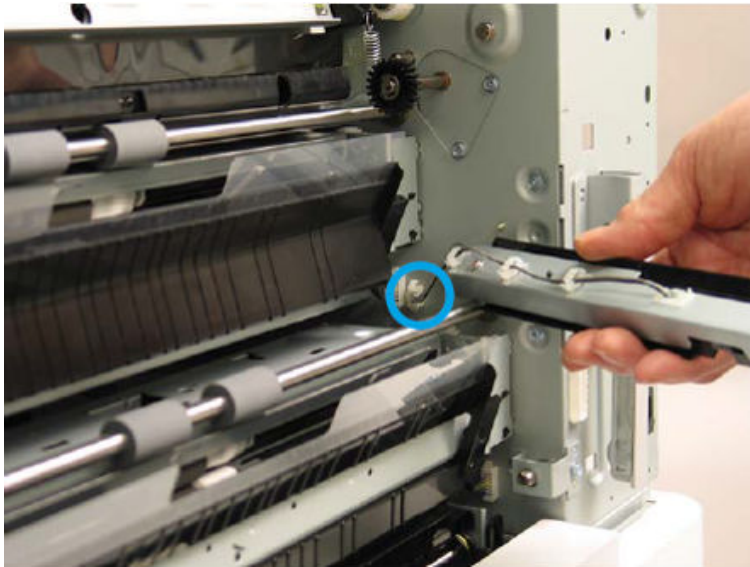
Figure 2-132 Disconnect one connector
