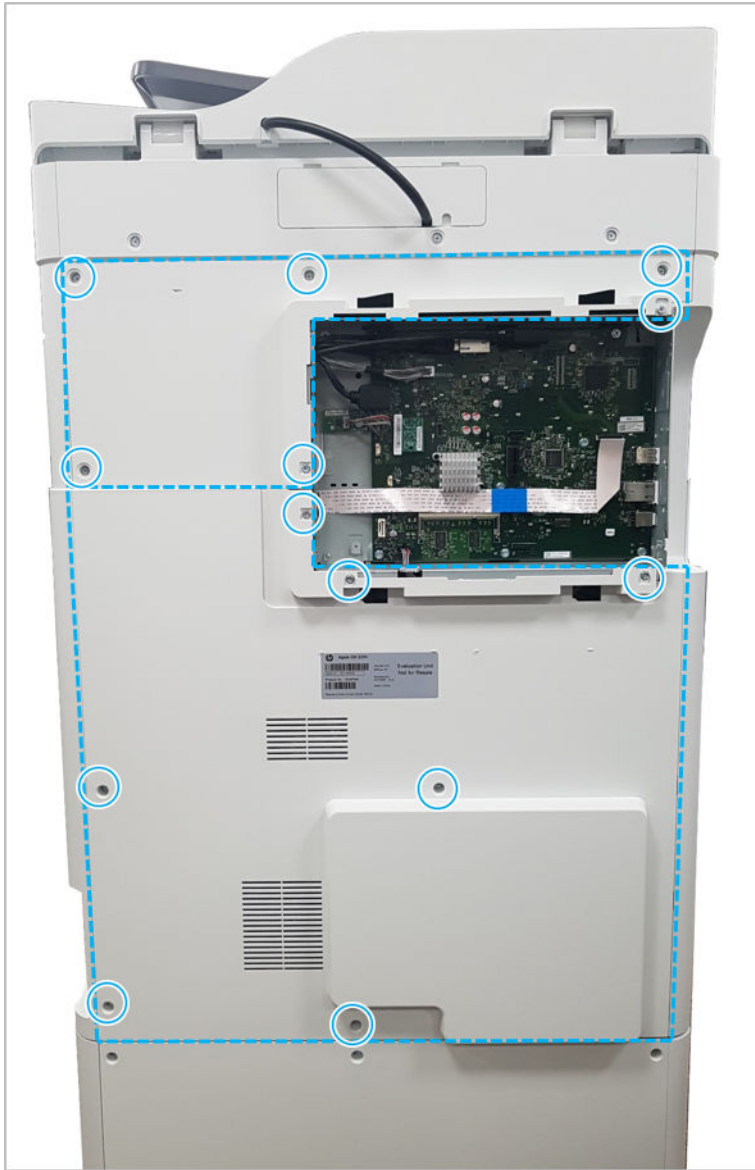
Figure 2-164 Remove the rear-bottom cover and rear-top cover
