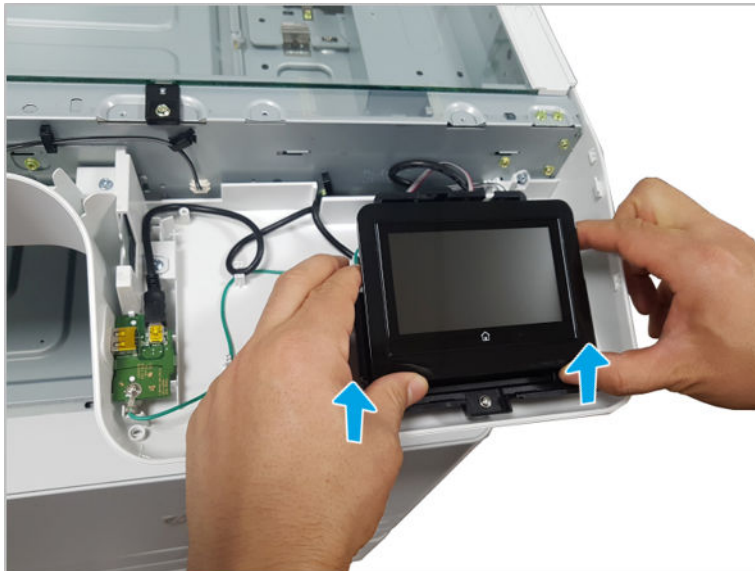
Figure 2-257 Release the control panel assembly
