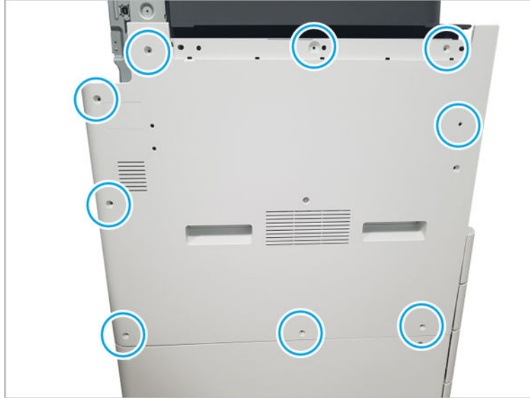
Figure 2-99 Remove the left cover
