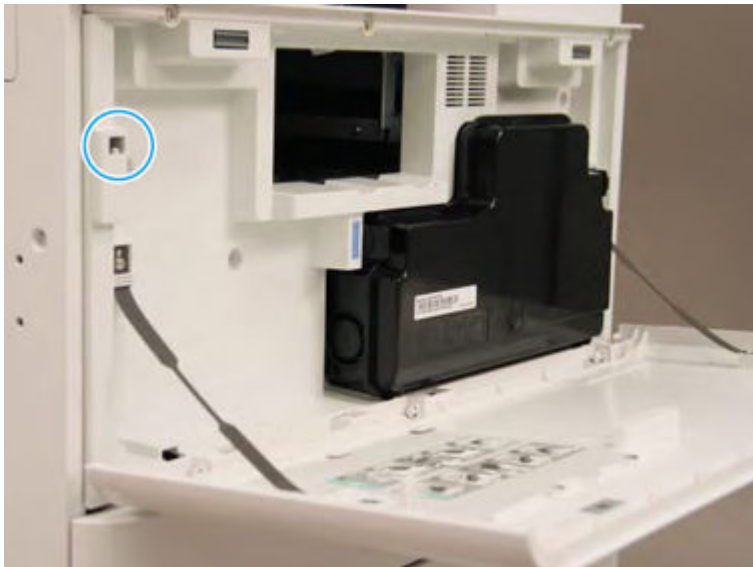
Figure 3-12 Defeat the toner cartridge door interlock
