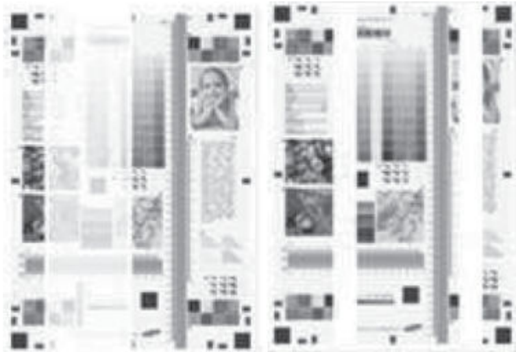
Figure 3-46 Light or White Lines (Feed direction)
