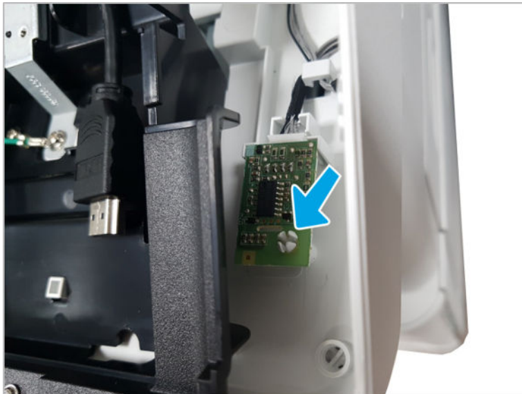
Figure 2-196 Release the latch
