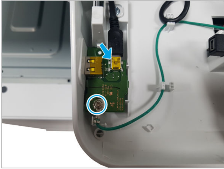
Figure 2-188 Remove the USB host PCA
