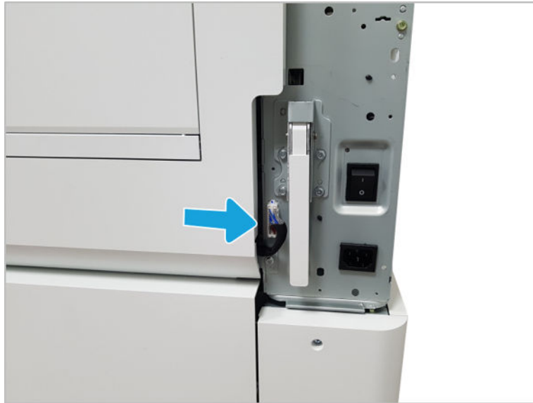
Figure 2-127 Disconnect right door connector
