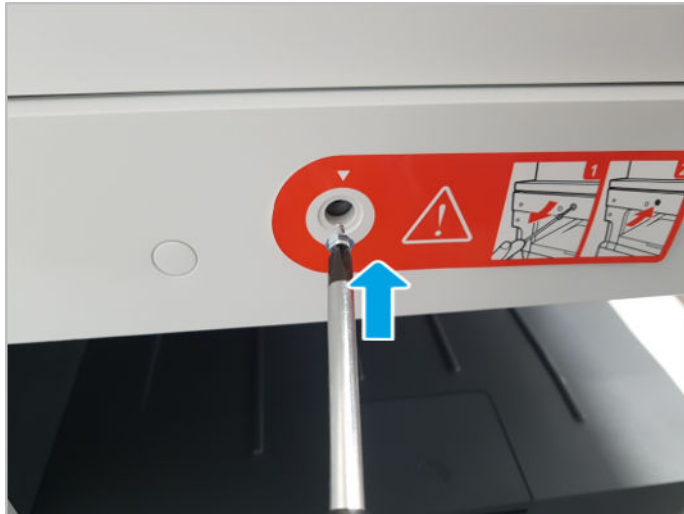
Figure 1-39 Install the scan locking screw
