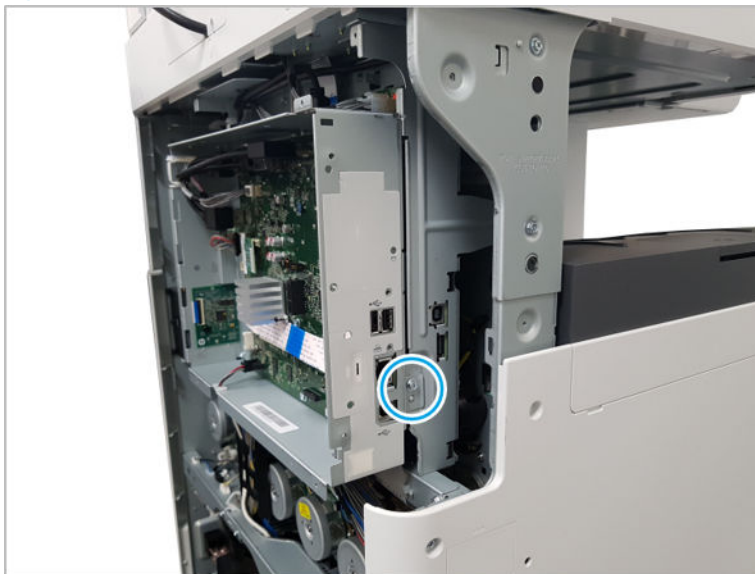
Figure 2-249 Remove the formatter cage side screw
