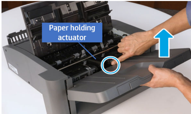
Figure 5-73 Remove the output tray.
