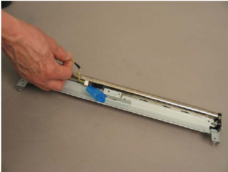
Figure 2-122 Remove the sensor and wire harness
