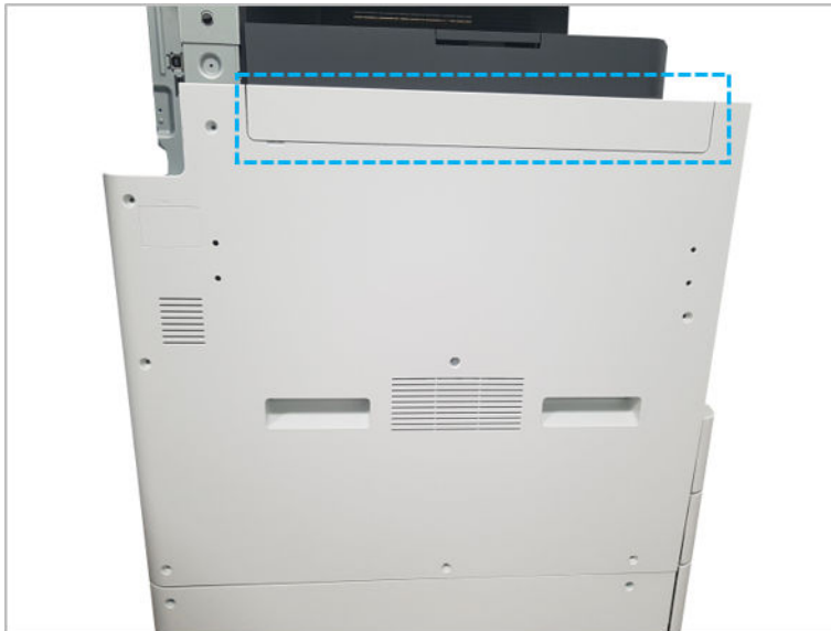
Figure 2-98 Remove the left trim cover
