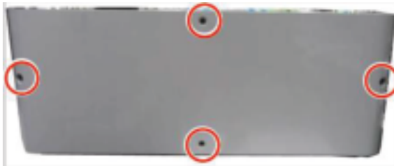
Figure 2-340 Remove the DCF rear cover
