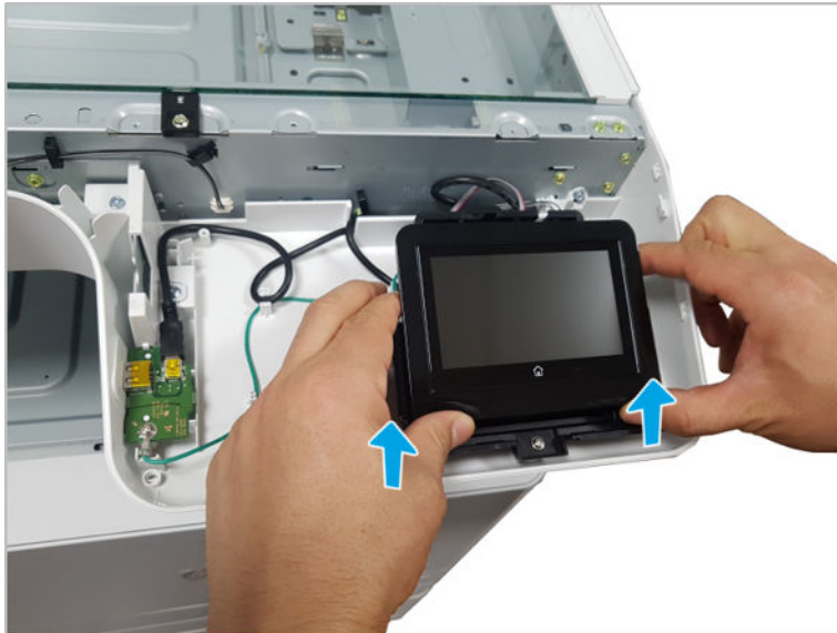
Figure 2-185 Release the control panel assembly
