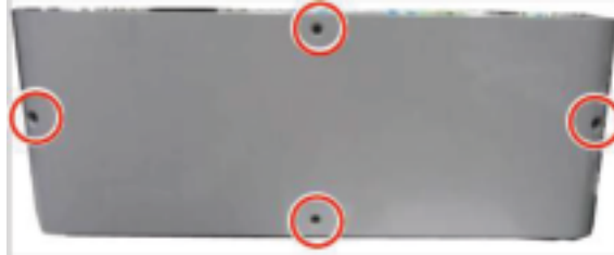
Figure 2-336 Remove the DCF rear cover
