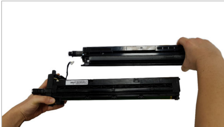
Figure 2-44 Separate developer and drum units
