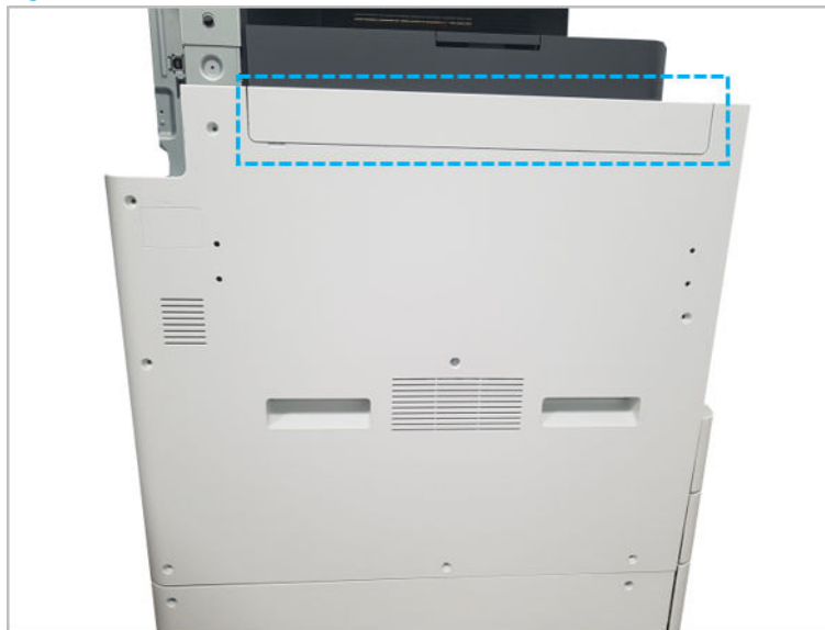
Figure 2-89 Remove the left trim cover
