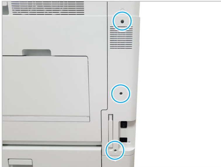
Figure 2-126 Remove the right-rear cover.
