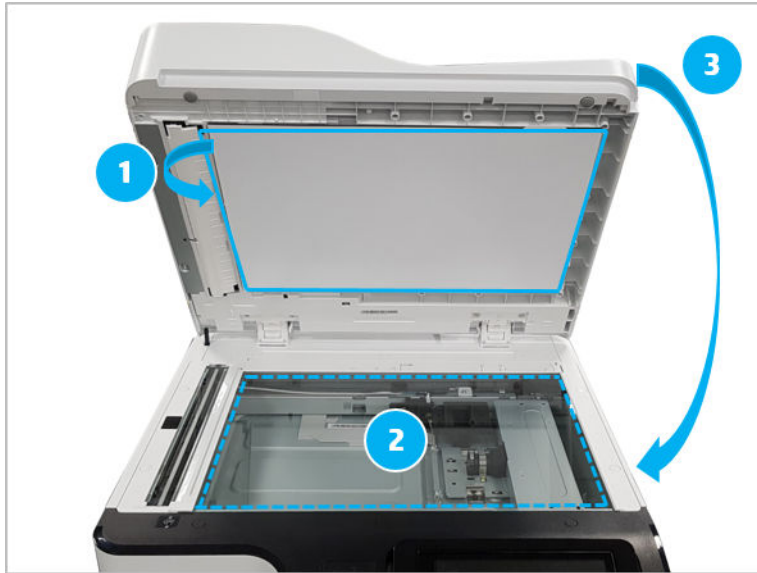
Figure 3-74 Detach and attach the sponge sheet
