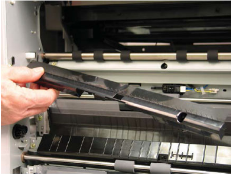
Figure 2-113 Remove the sensor cover
