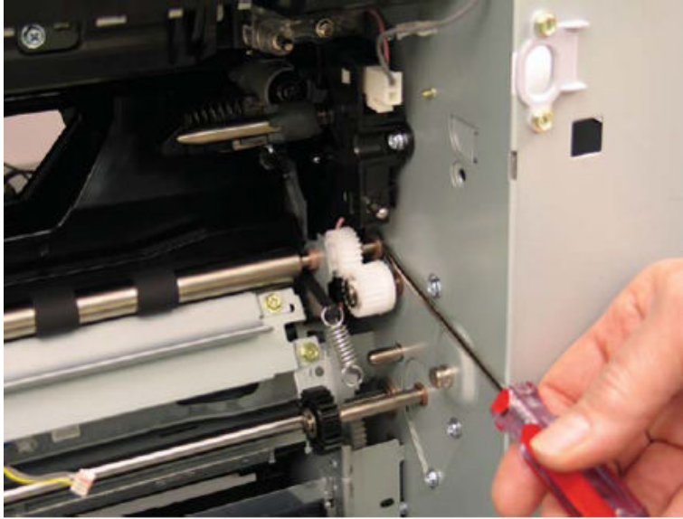
Figure 2-117 Remove two screws
