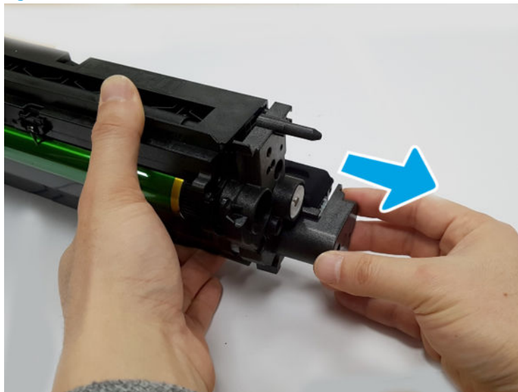
Figure 2-51 Remove the rear cover
