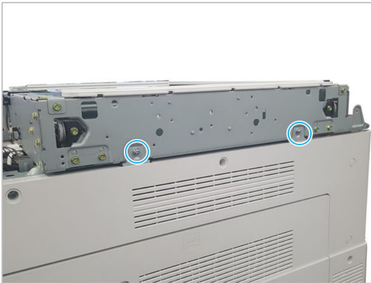
Figure 2-265 Remove two screws
