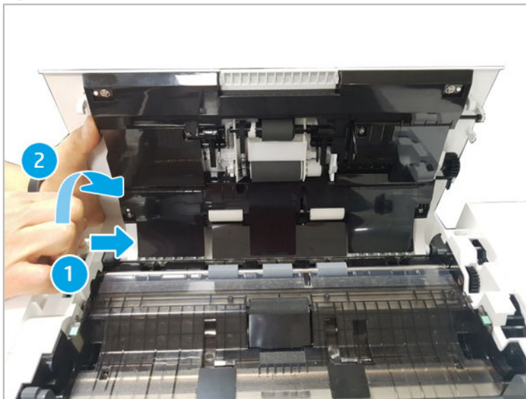
Figure 2-305 Remove the ADF open cover
