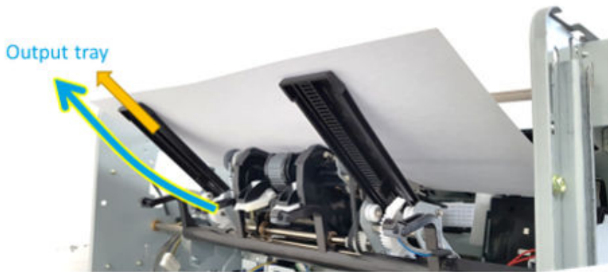
Figure 5-25 Inner finisher system - paper support unit operation
