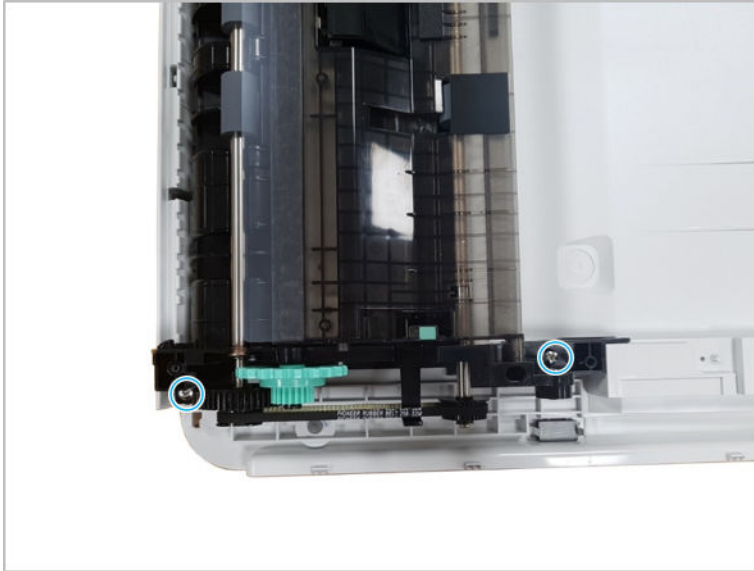
Figure 2-329 Remove two screws
