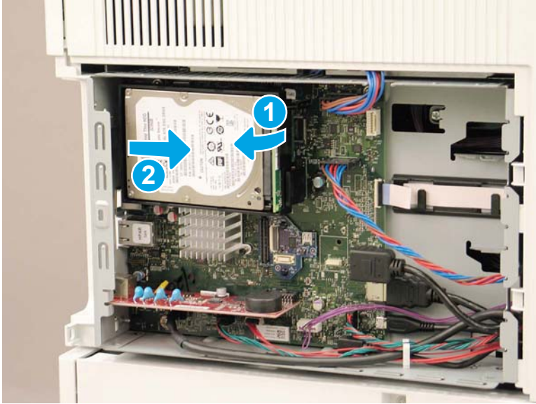
Figure 8-81 Rotate the HDD away from the formatter and remove the HDD
