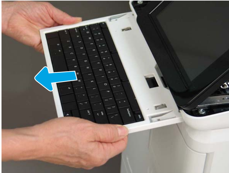
Figure 8-838 Remove the keyboard
