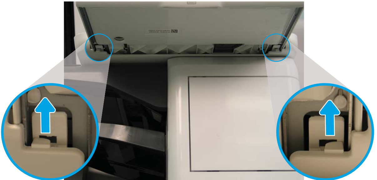
Figure 8-121 Release two tabs
