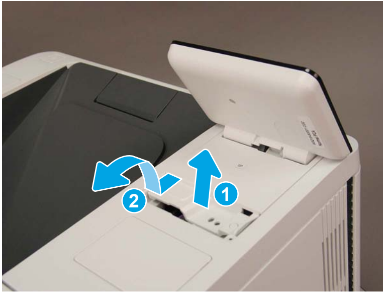
Figure 8-2333 Lift and release the control panel
