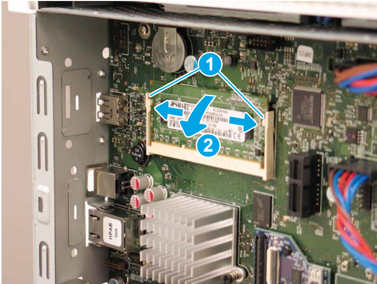
Figure 8-90 Release two locking arms and pivot the DIMM away from the holder
