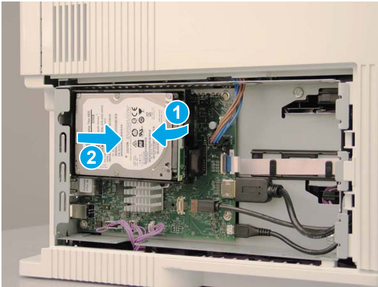
Figure 8-1690 Rotate the HDD away from the formatter and remove the HDD
