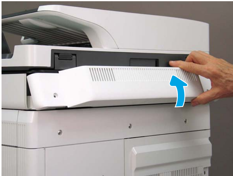
Figure 8-843 Remove the image scanner back cover
