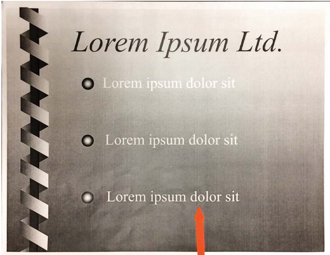
Figure 7-141 111 mm trailing edge blur
