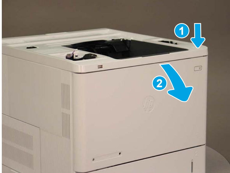
Figure 8-1863 Locate the tab and open the MP tray cover
