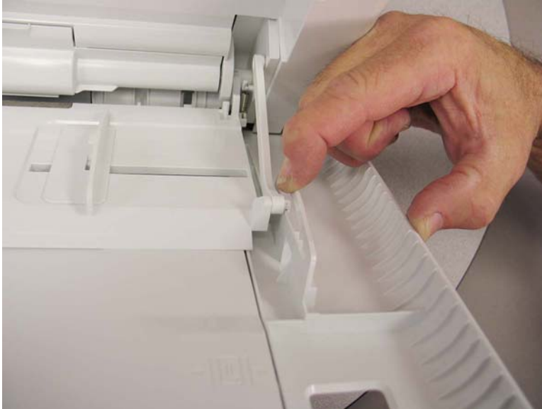
Figure 8-1842 Release the MP tray assembly lift arms from the MP cover
