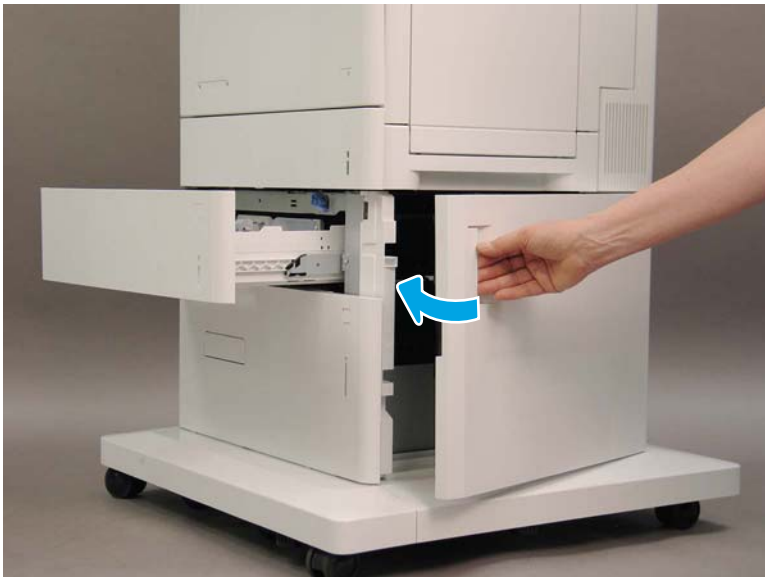
Figure 5-165 Close the right door of the paper feeder
