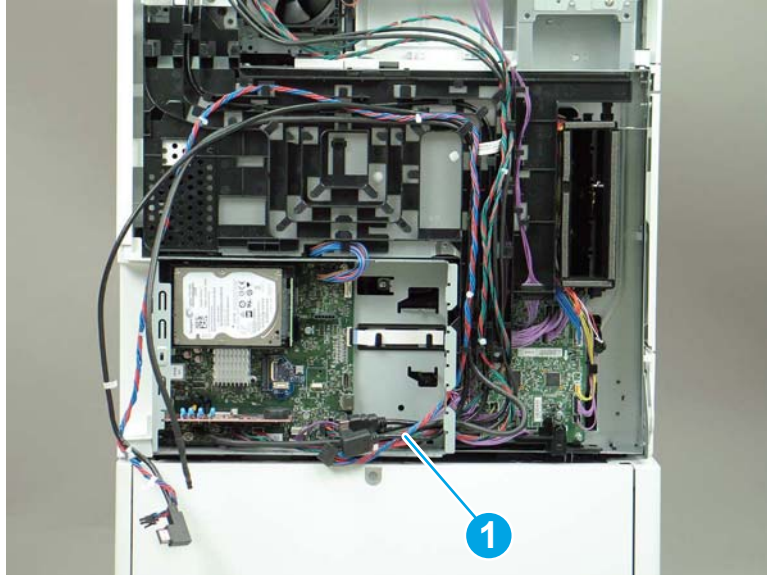
Figure 8-762 Thread the formatter cables through the formatter case
