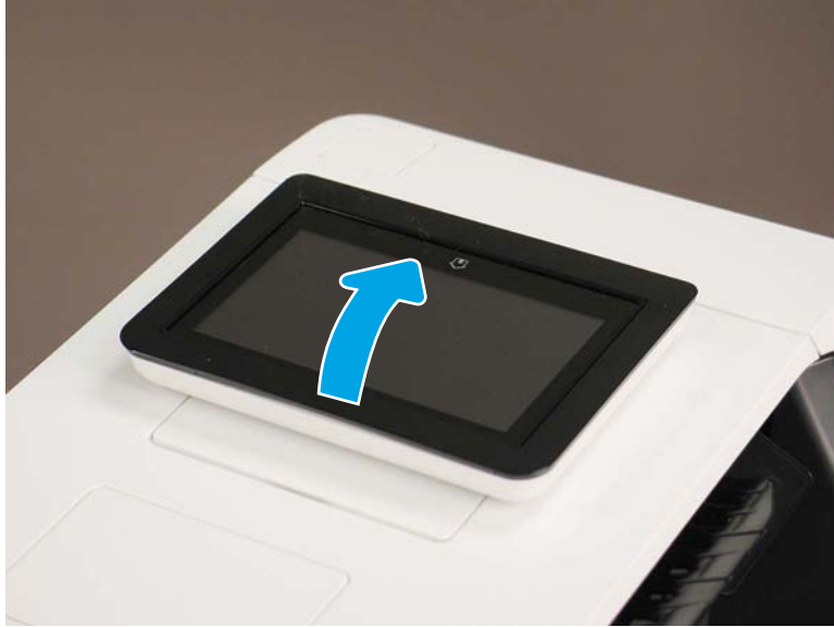
Figure 8-2084 Raise the control panel screen
