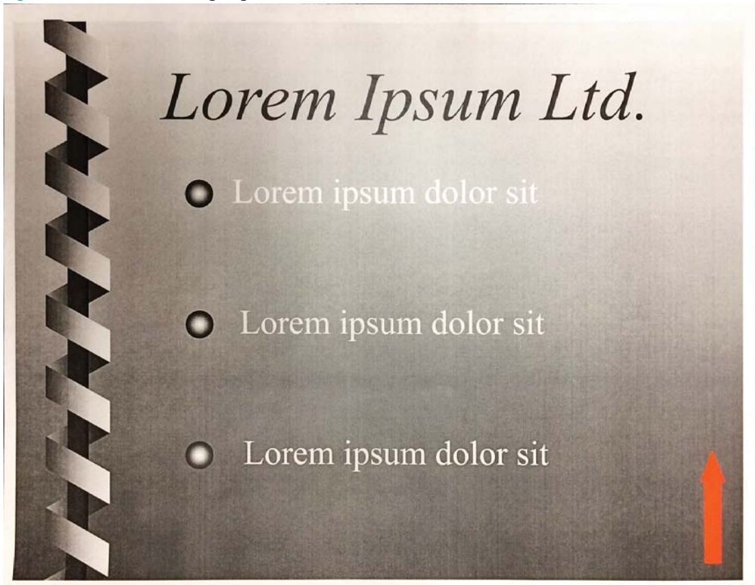
Figure 7-134 18 mm leading edge blur
