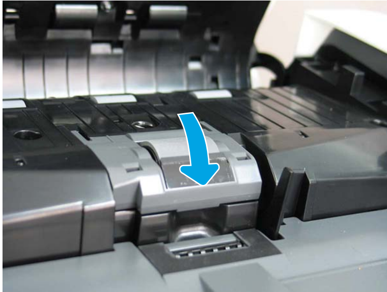
Figure 8-60 Close the separation roller cover
