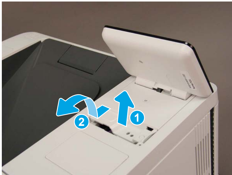
Figure 8-2087 Lift and release the control panel
