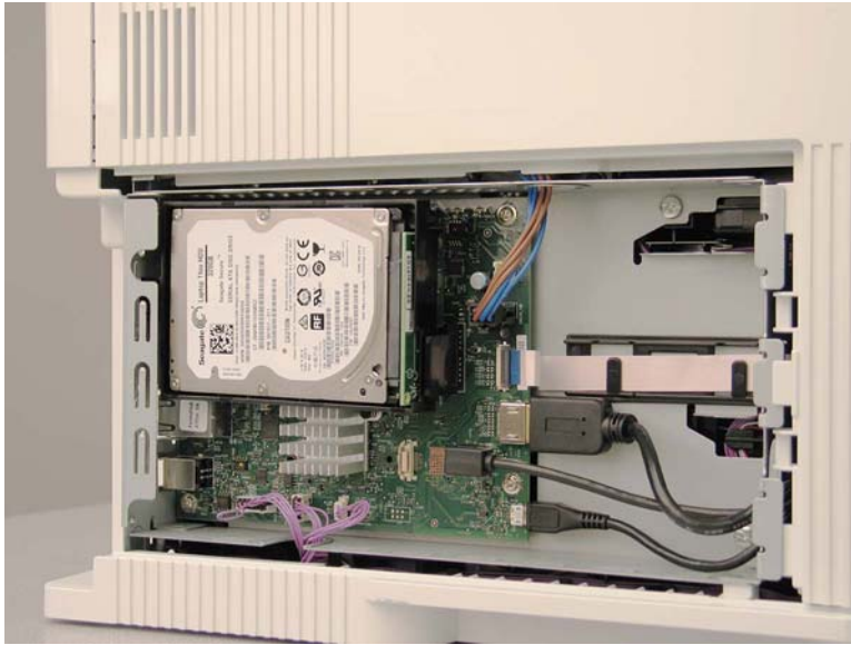
Figure 8-105 Locate the space for installing the internal USB ports/AA module
