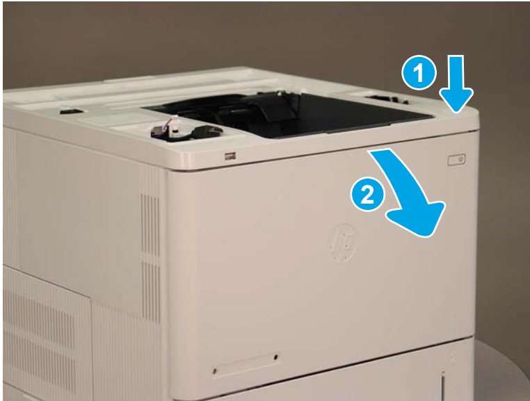
Figure 8-2337 Locate the tab and open the MP tray cover
