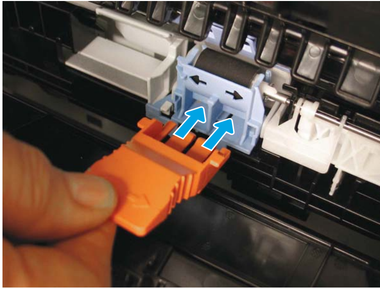
Figure 8-156 Install the orange tool in the separation roller
