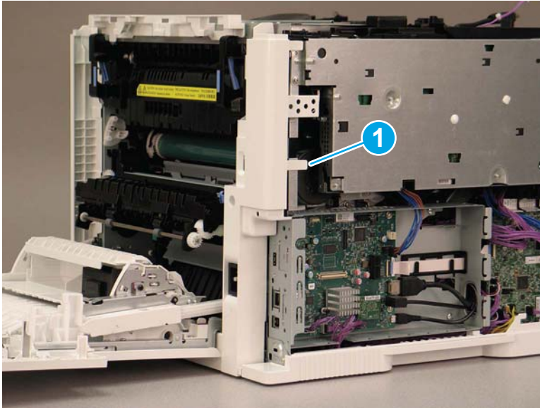
Figure 8-2139 Release the tab and remove the inlet cover
