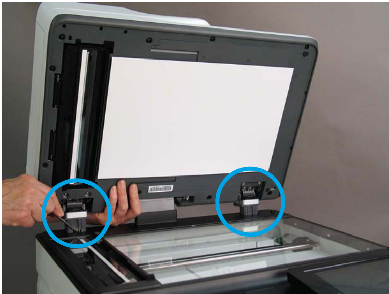
Figure 8-950 Release two tabs on the ADF
