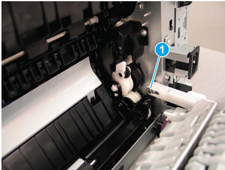
Figure 8-2225 Remove the e-ring
