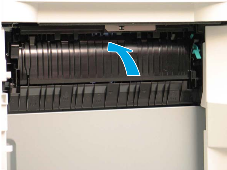
Figure 5-85 Raise the feed assembly
