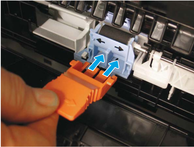
Figure 5-140 Install the orange tool in the separation roller
