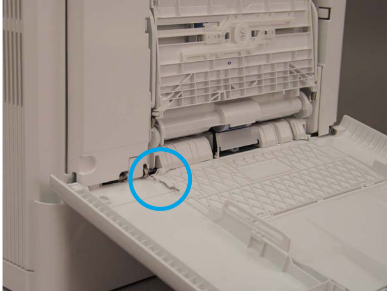
Figure 8-1829 Flex and slide to release the MP cover
