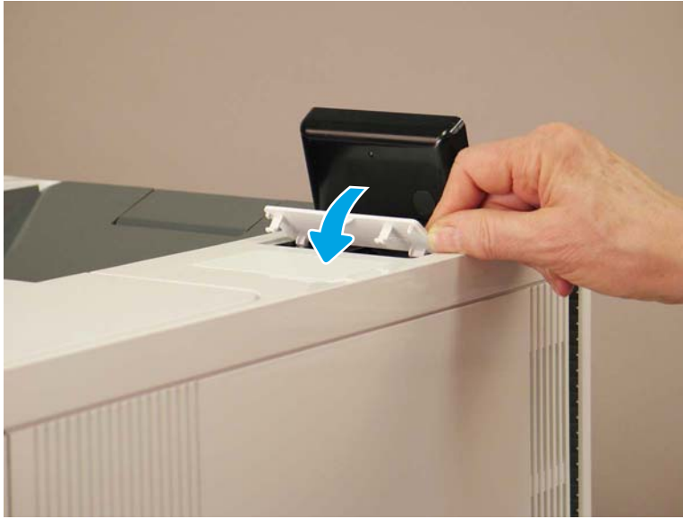
Figure 8-1665 Align the control panel cover and pivot down to install it
