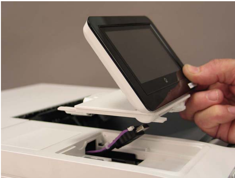
Figure 8-1816 Remove the control panel
