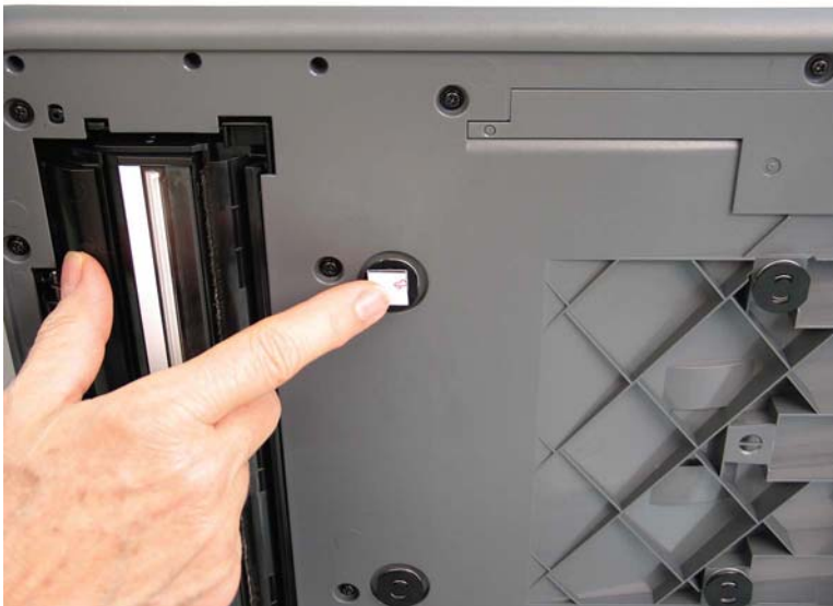
Figure 8-72 Attach the adhesive squares on each retention clip
