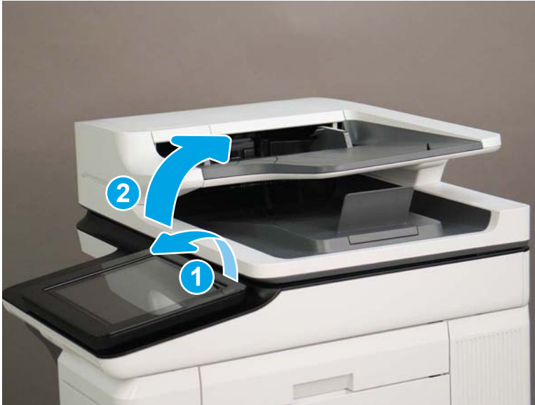
Figure 8-116 Tilt the control panel and open the document feeder
