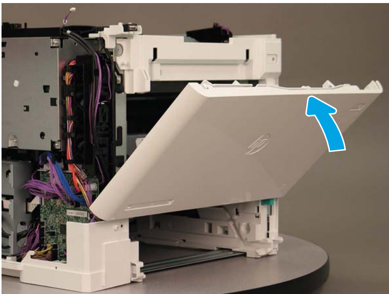
Figure 8-2266 Partially close the cartridge door
