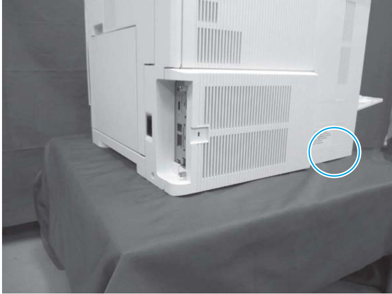
Figure 7-6 Engine test button (2 of 2)
