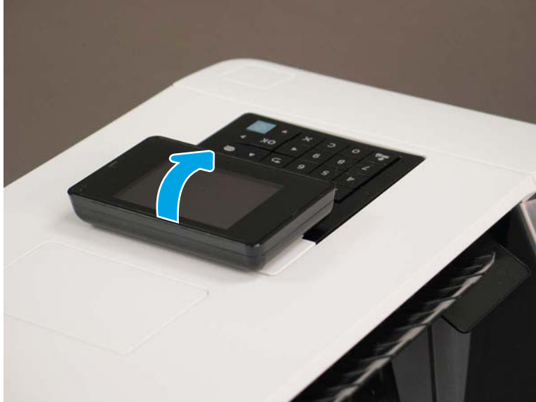
Figure 8-1656 Raise the control panel screen
