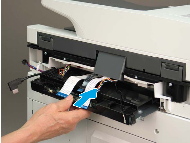
Figure 8-591 Check the cables when installing the SCB
