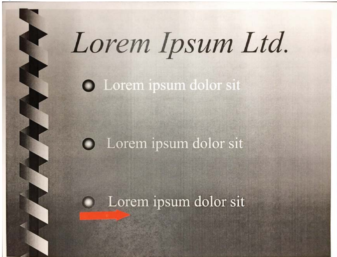
Figure 7-140 104 mm trailing edge blur
