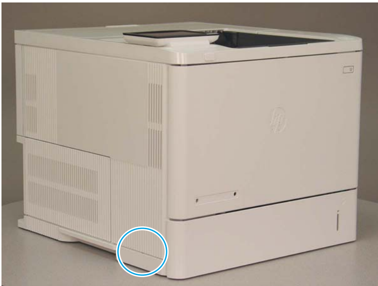
Figure 7-89 Engine test button (1 of 2)
