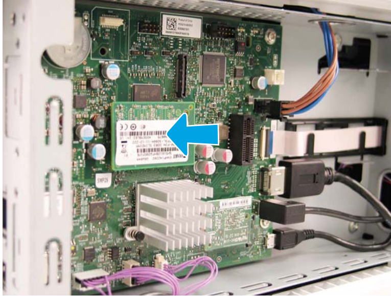
Figure 8-1705 Push the DIMM onto the formatter connector
