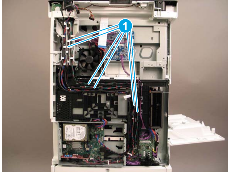
Figure 8-959 Release the formatter cables
