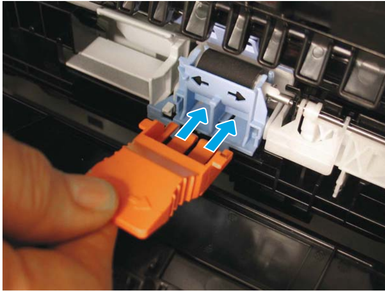
Figure 5-61 Install the orange tool in the separation roller
