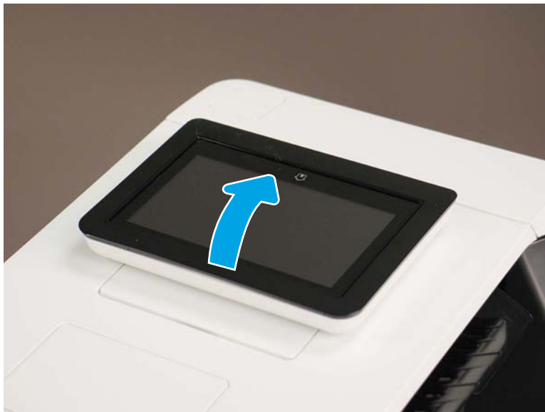
Figure 8-2126 Raise the control panel screen
