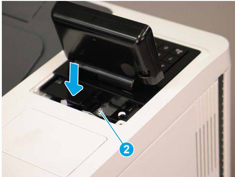
Figure 8-1664 Lower the control panel and install one thumbscrew
