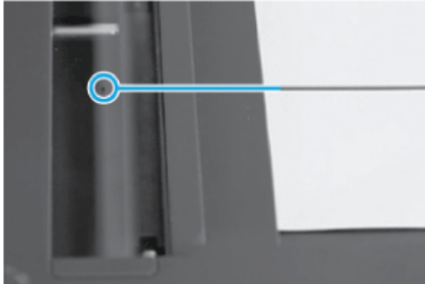
Figure 7-128 Identify the CQ defect location
