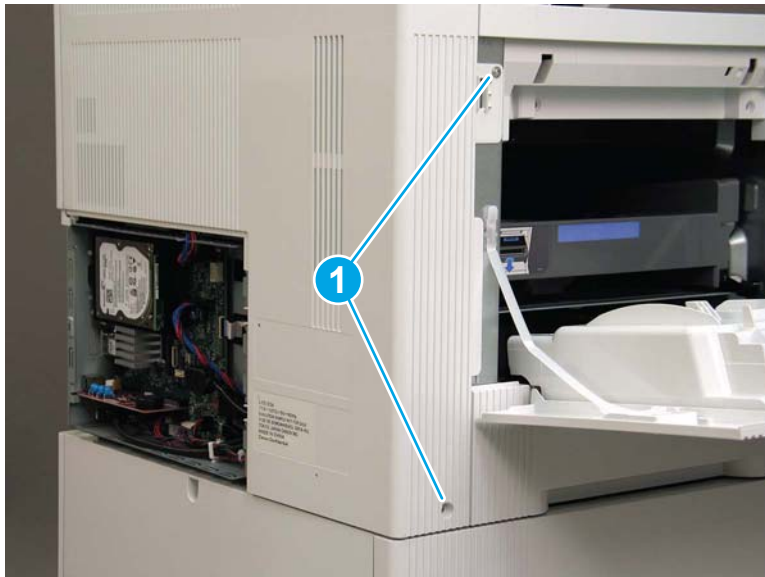
Figure 8-624 Remove two screws
