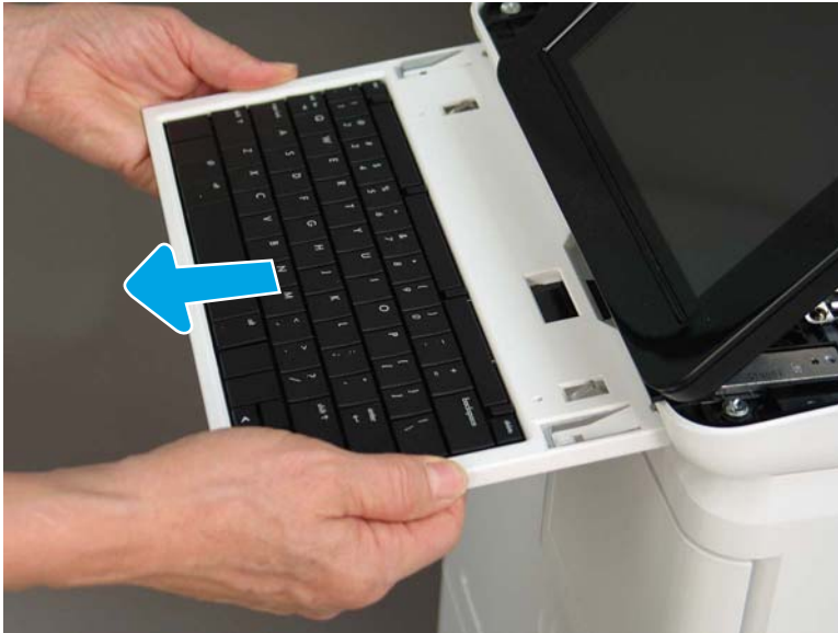
Figure 8-894 Remove the keyboard
