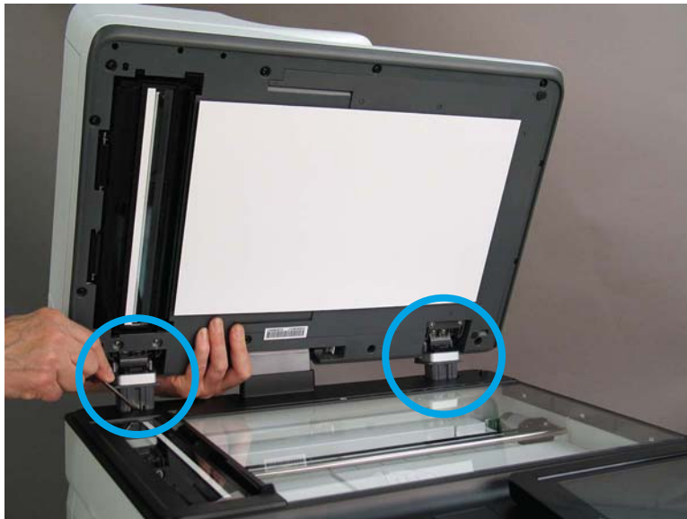
Figure 8-1168 Release two tabs on the ADF
