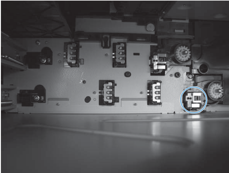
Figure 2-16 Tray 3 paper surface sensor
