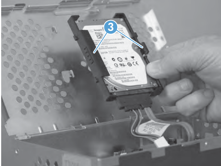
Figure 2-20 Remove the encrypted HDD (3 of 4)
