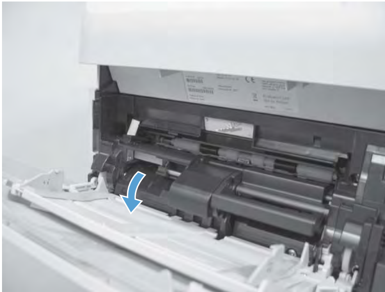
Figure 2-29 Remove the Tray 1 separation roller (1 of 3)
