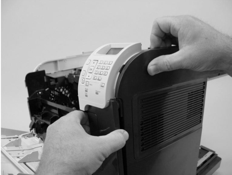
Figure 2-46 Remove the right-side cover (2 of 3)
