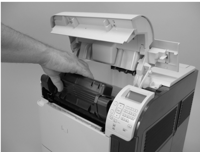
Figure 2-3 Remove the print cartridge (2 of 2)
