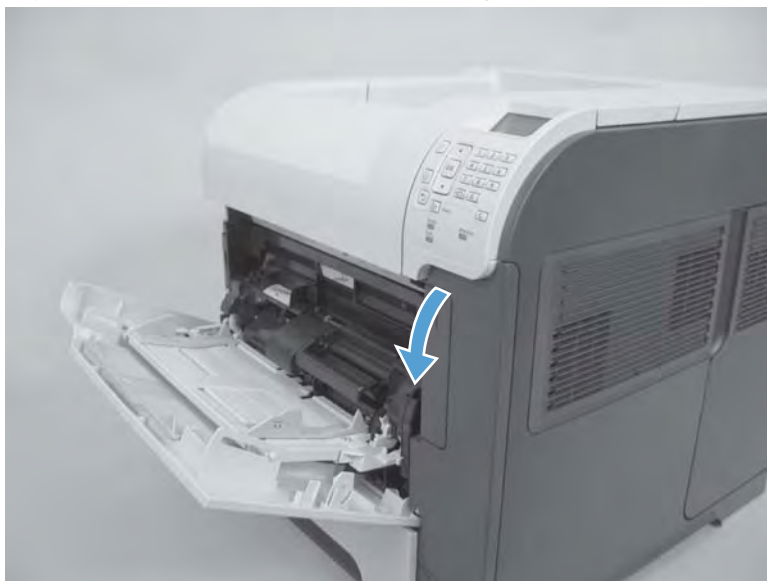
Figure 2-36 Remove the front accessory covers (2 of 2)
