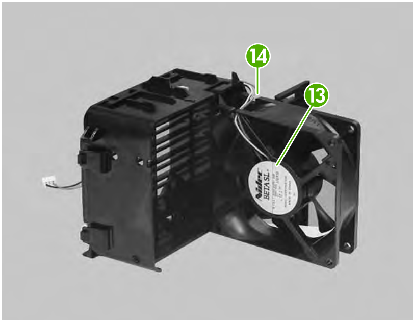
Figure 5-111 Removing the main fan (5 of 5)
