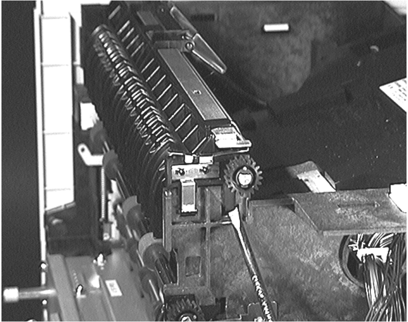
Figure 6-55 Upper Delivery Assembly Tabs
