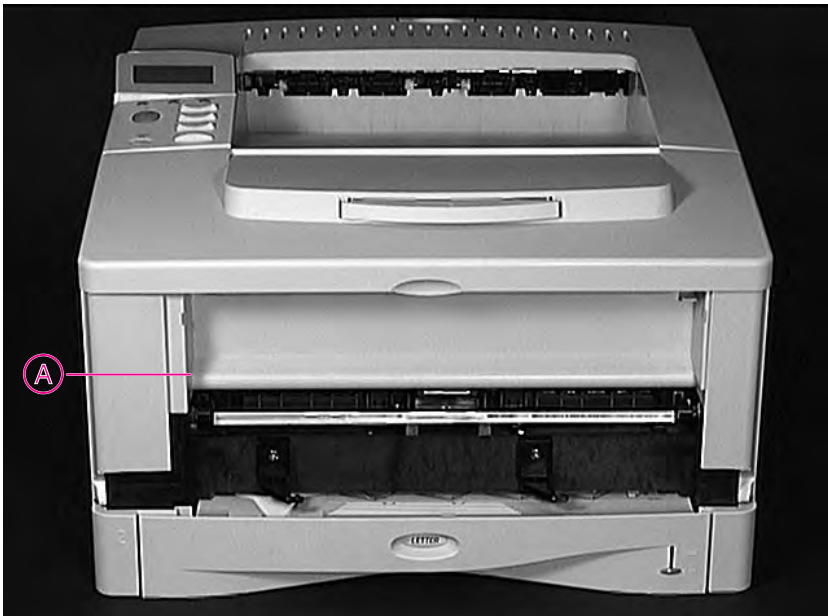
Figure 7-1 Location of the Engine Test Button
