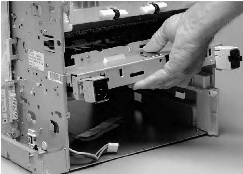
Figure 143. Power supply (5 of 5)
