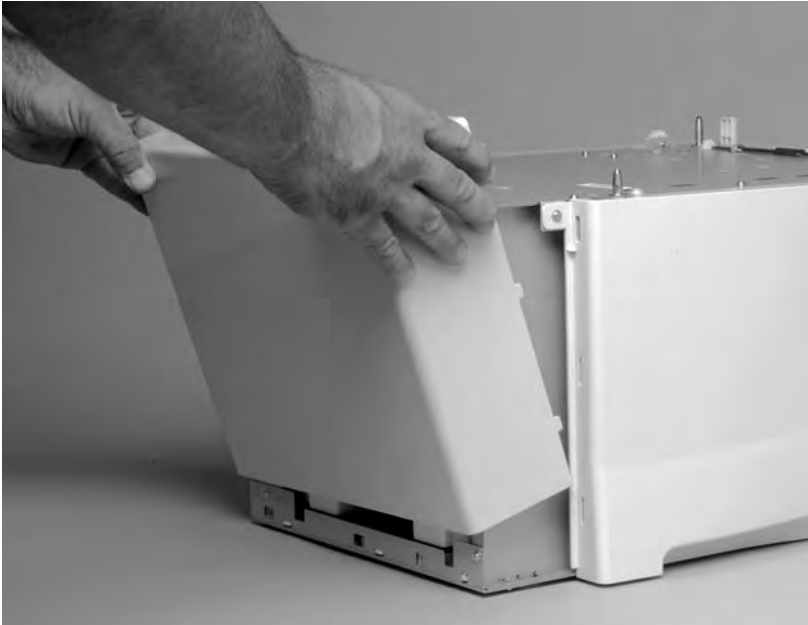
Figure 6-121 1,500-sheet feeder rear cover (2 of 2)
