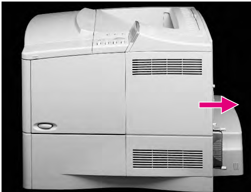
Figure 40. Removing the rear right side cover
