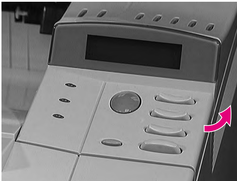
Figure 41. Removing the control panel overlay
