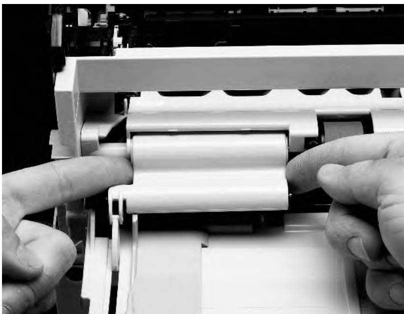
Figure 50. Removing the tray 1 sensor arm cover
