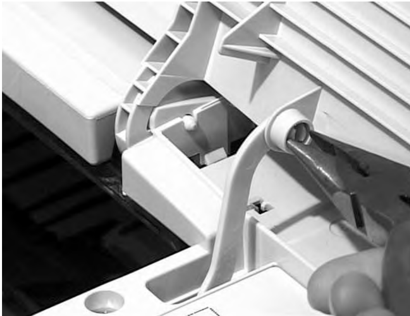
Figure 43. Disconnecting the toner cartridge drive arm
