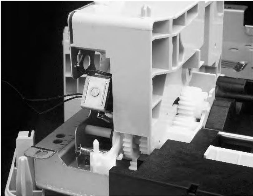
Figure 90. Location of spring and lever (the paper feeder is inverted)
