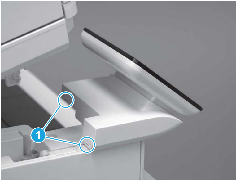
Figure 5-336 Release two tabs
