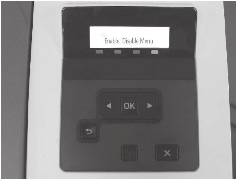
Figure 4-37 2-line control panel
