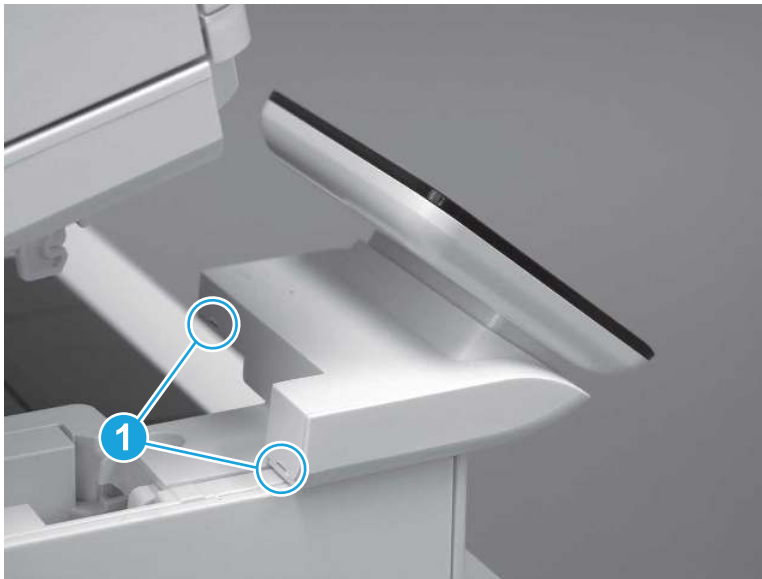
Figure 5-617 Release two tabs
