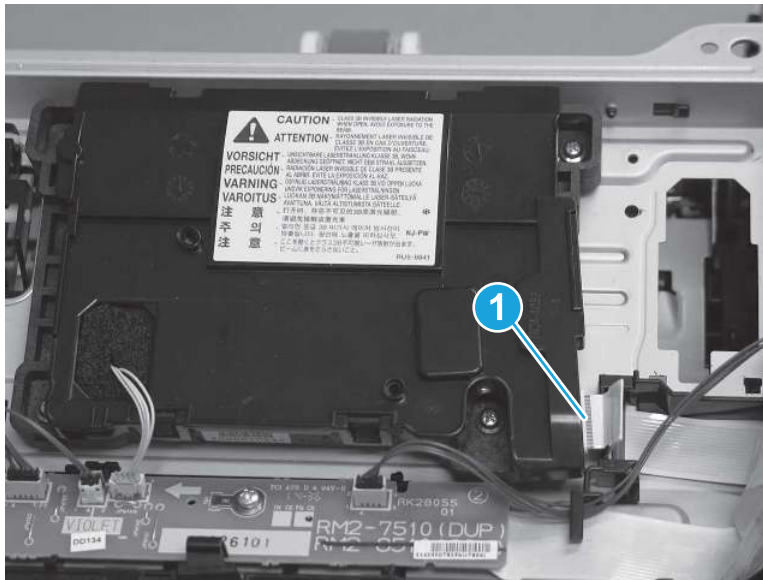
Figure 5-860 Disconnect one FFC
