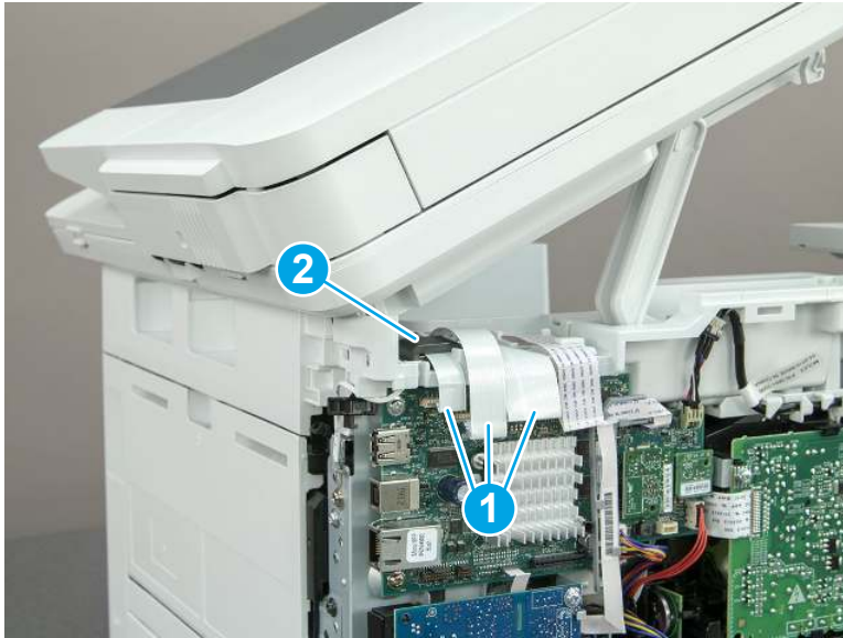
Figure 5-264 Disconnect three FFCs
