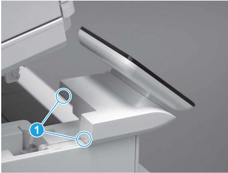
Figure 5-727 Release two tabs
