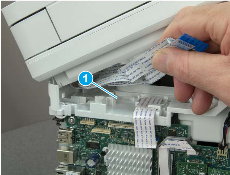
Figure 5-769 Release the tape
