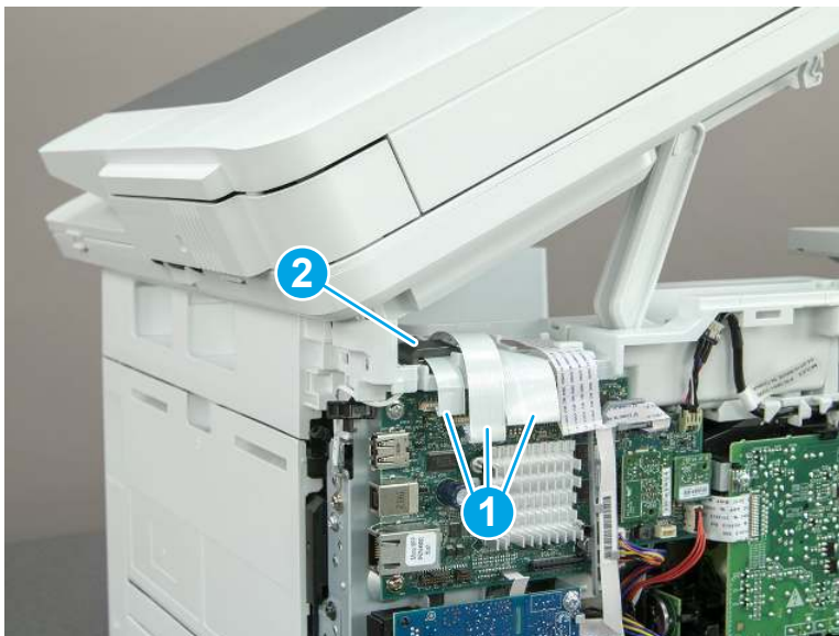
Figure 5-716 Disconnect three FFCs
