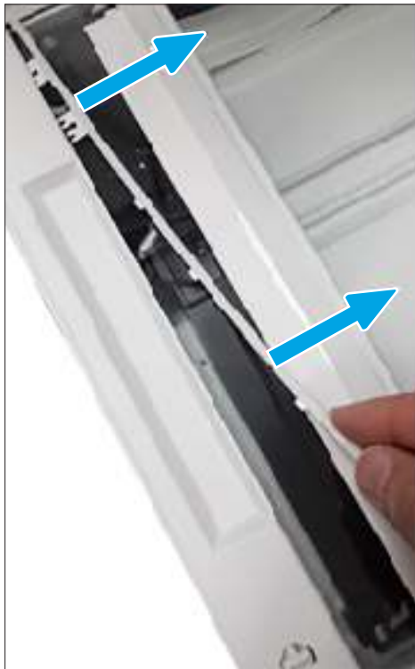
Figure 5-61 Remove the Mylar holder
