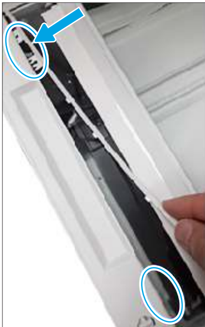
Figure 5-70 Reinstall the Mylar holder
