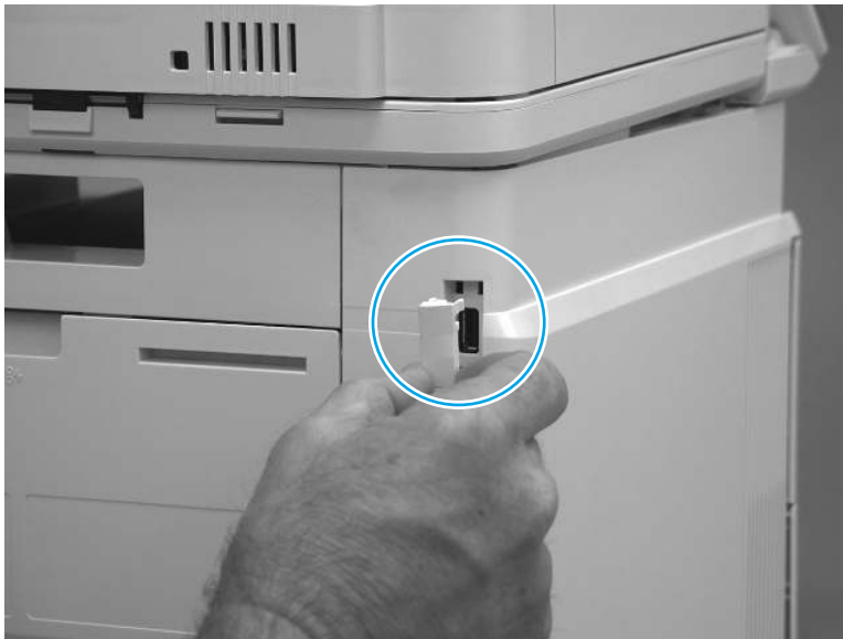
Figure 5-104 Remove the rear USB cover
