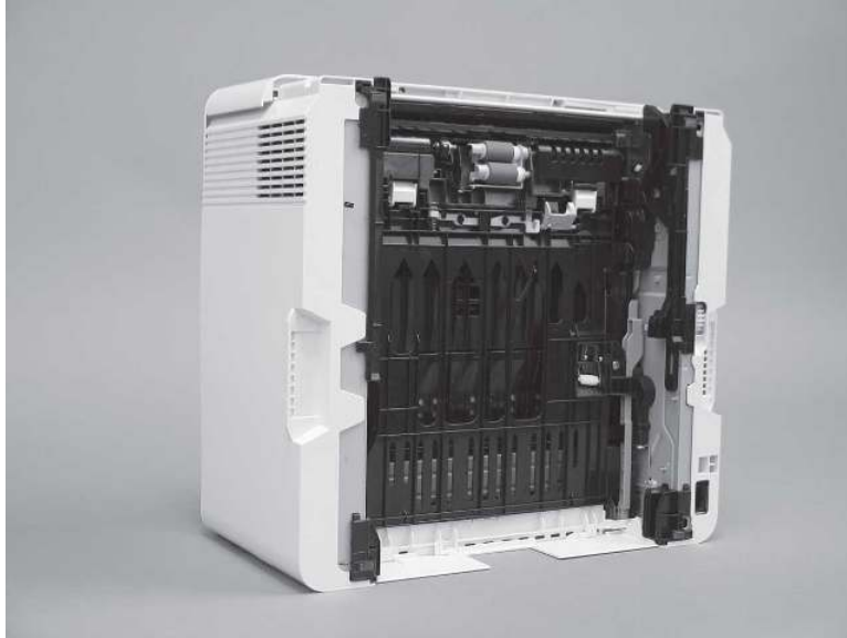
Figure 4-65 Place the printer bottom-side face forward
