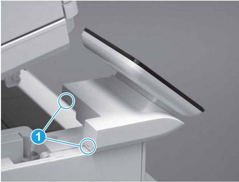
Figure 5-779 Release two tabs
