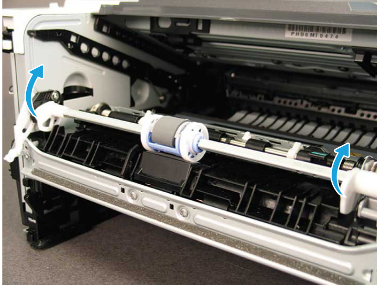
Figure 5-1041 Rotate the Tray 1 pickup roller shaft
