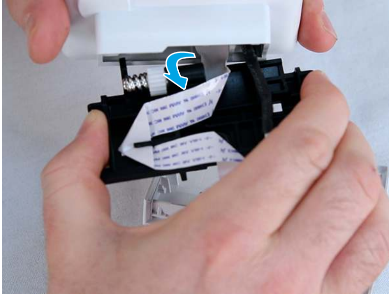
Figure 5-1024 Separate the control panel and mount chassis
