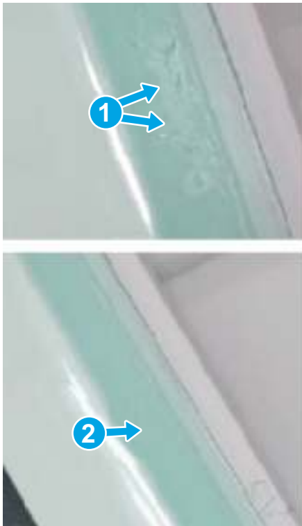
Figure 5-75 Incorrect/correct Mylar installation
