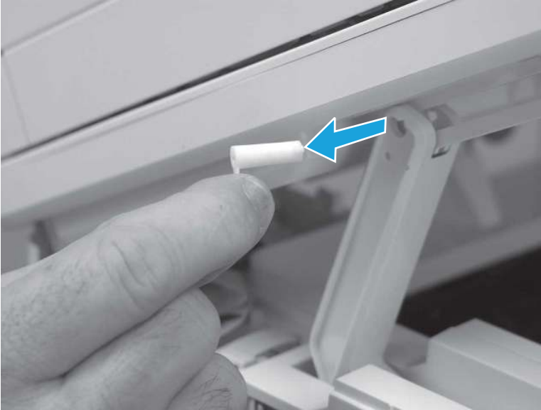
Figure 5-501 Remove the slider pin
