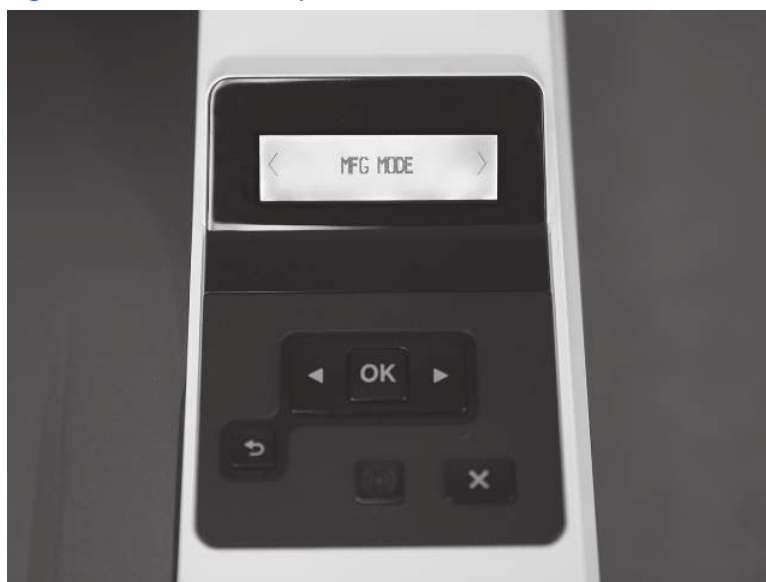
Figure 4-41 2-line control panel
