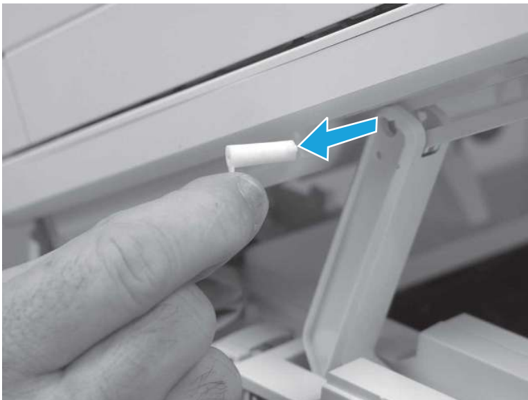
Figure 5-269 Remove the slider pin
