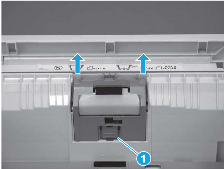
Figure 5-43 Release the assembly
