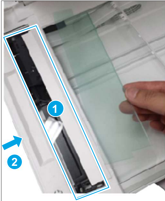
Figure 5-62 Remove adhesive residue
