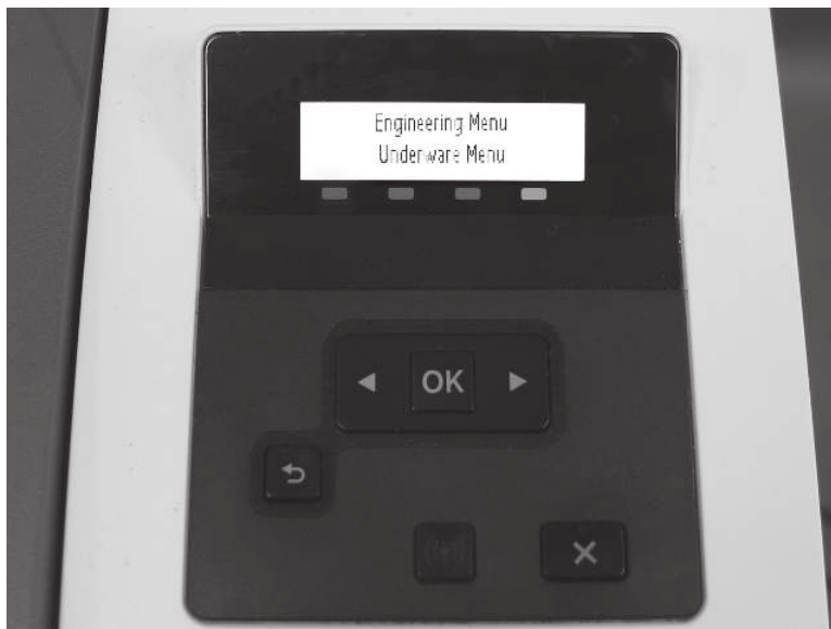
Figure 4-39 2-line control panel
