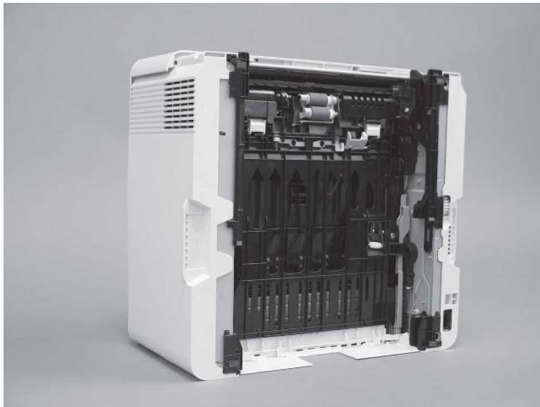
Figure 4-76 Place the printer bottom-side face forward
