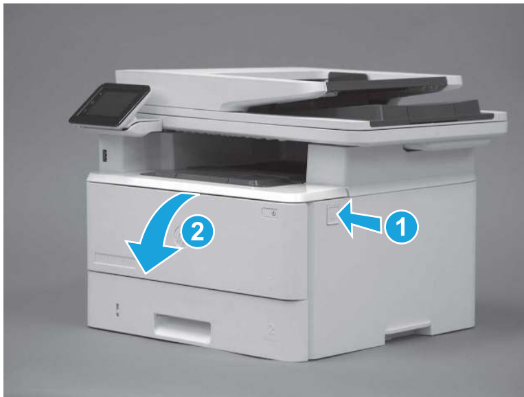
Figure 2-10 Open the toner-cartridge door
