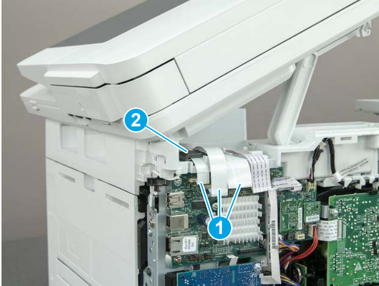
Figure 5-606 Disconnect three FFCs
