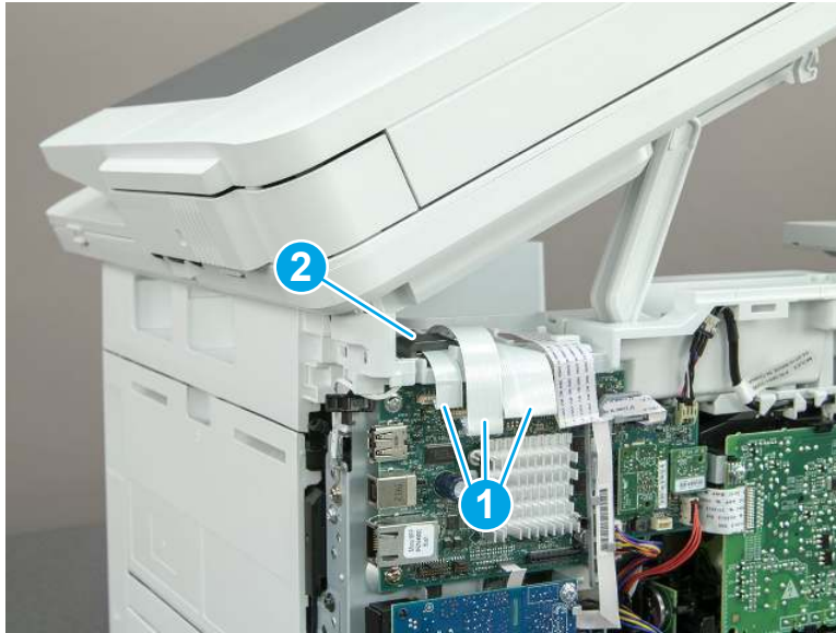
Figure 5-93 Disconnect three FFCs
