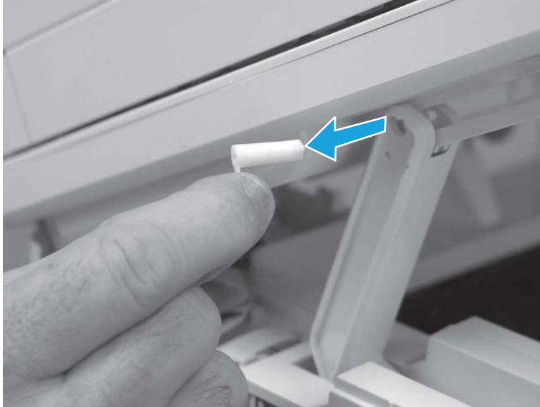
Figure 5-773 Remove the slider pin
