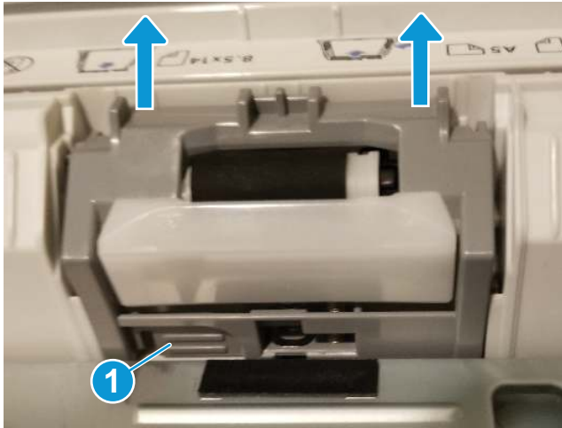
Figure 5-25 Release the assembly
