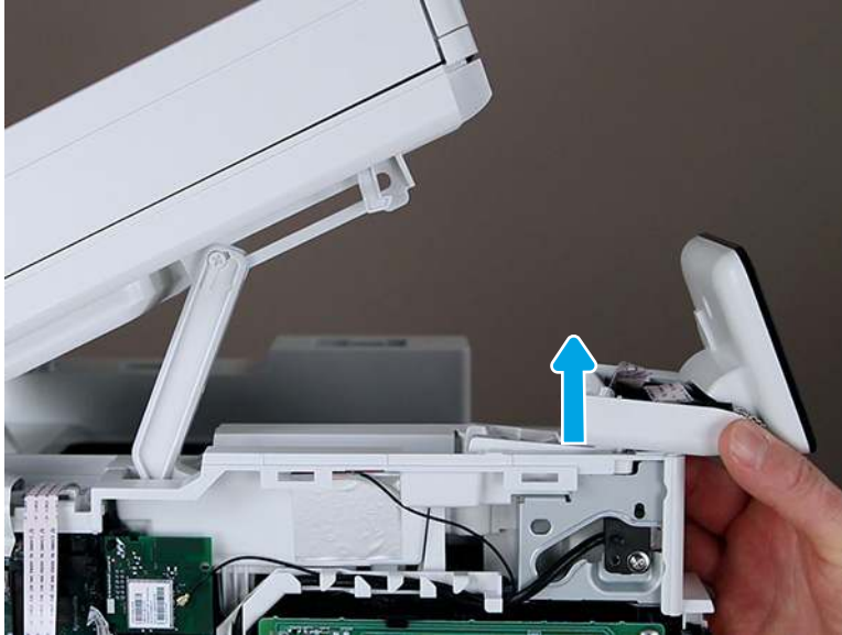
Figure 5-554 Lift up the control-panel assembly
