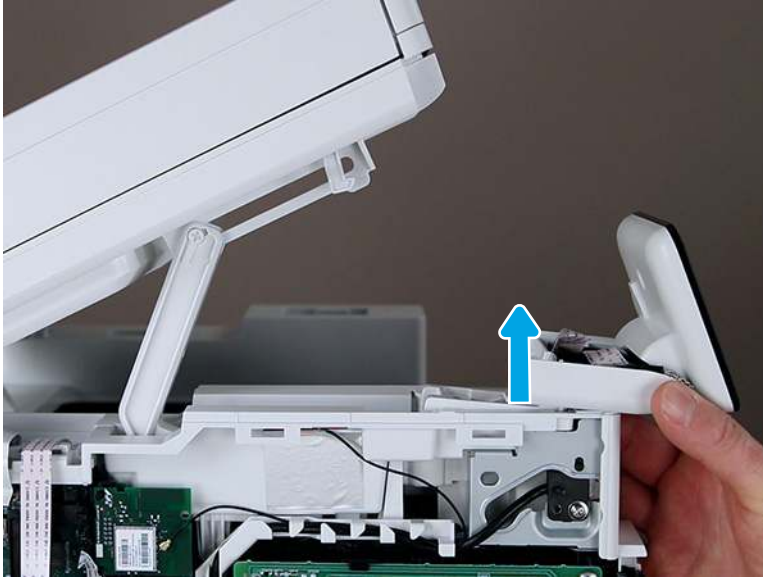
Figure 5-622 Lift up the control-panel assembly
