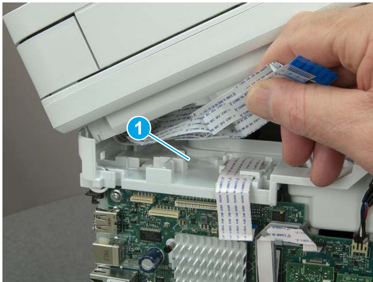
Figure 5-94 Release the tape
