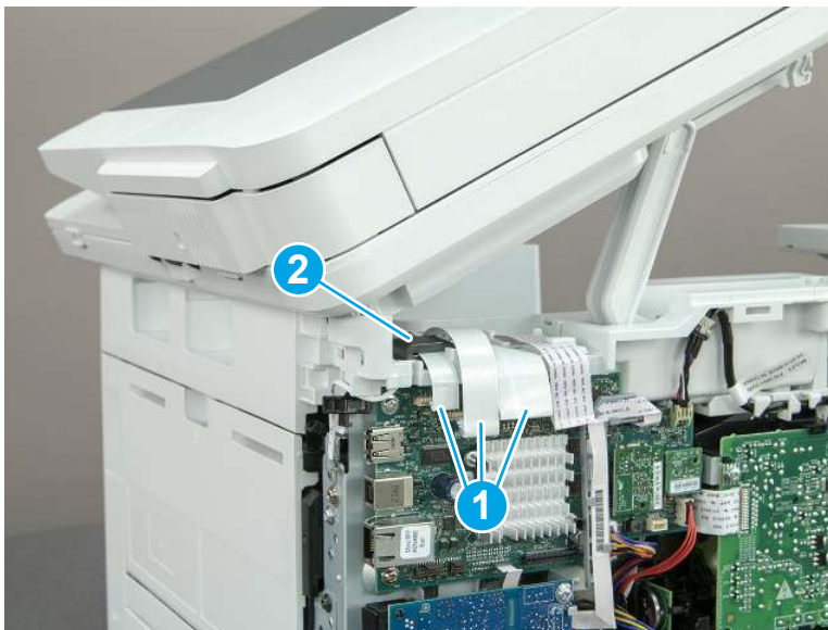
Figure 5-878 Disconnect three FFCs
