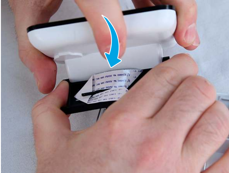
Figure 5-1022 Tilt the control panel
