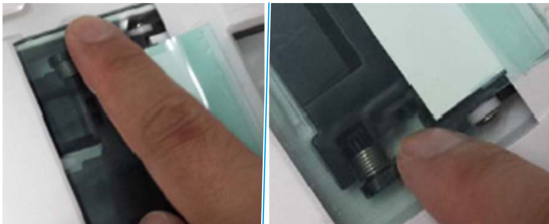
Figure 5-66 Check the install of the Mylar
