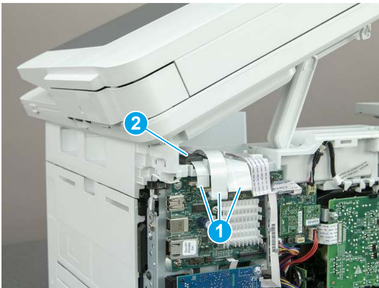
Figure 5-768 Disconnect three FFCs
