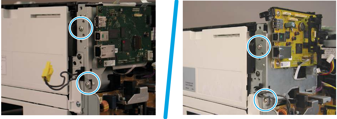
Figure 5-851 Remove two screws
