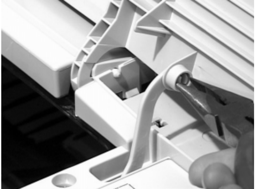
Figure 6-5 Removing the Toner Cartridge Drive Arm
