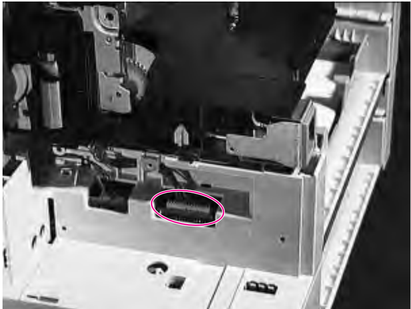
Figure 6-39 Unplugging the connector to the Paper Feed Module
