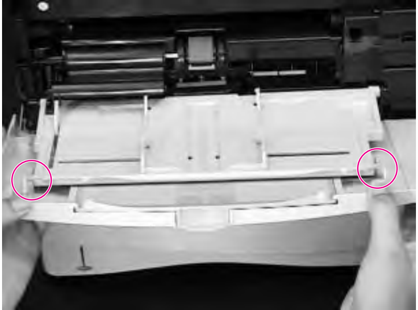
Figure 6-11 Removing Tray 1 from the Front Cover
