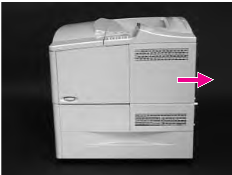
Figure 6-2 Removing the Rear Right Side Cover
