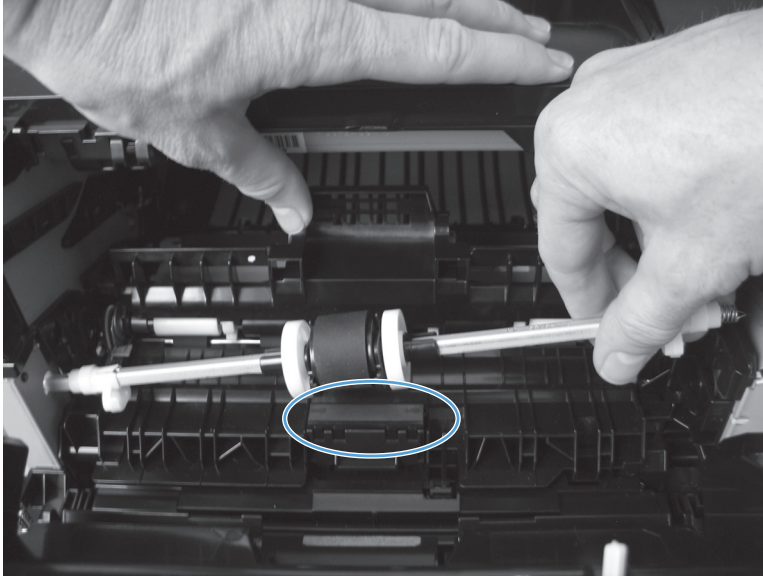
Figure 1-6 Remove the MP tray separation pad (3 of 5)
