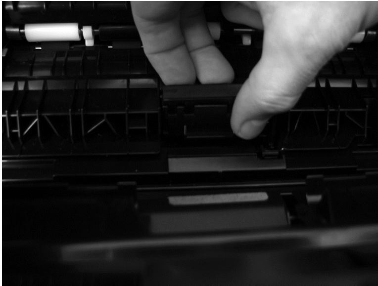
Figure 1-8 Remove the MP tray separation pad (5 of 5)
