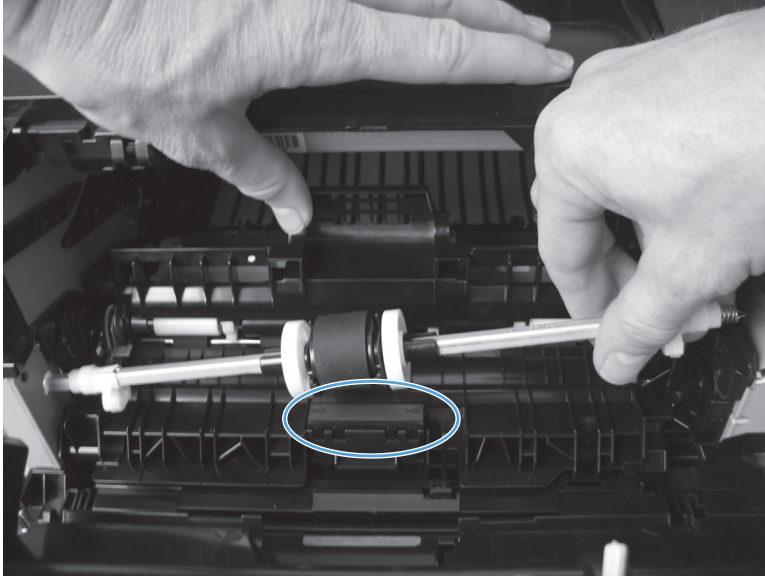
Figure 1-6 Remove the MP tray separation pad (3 of 5)
