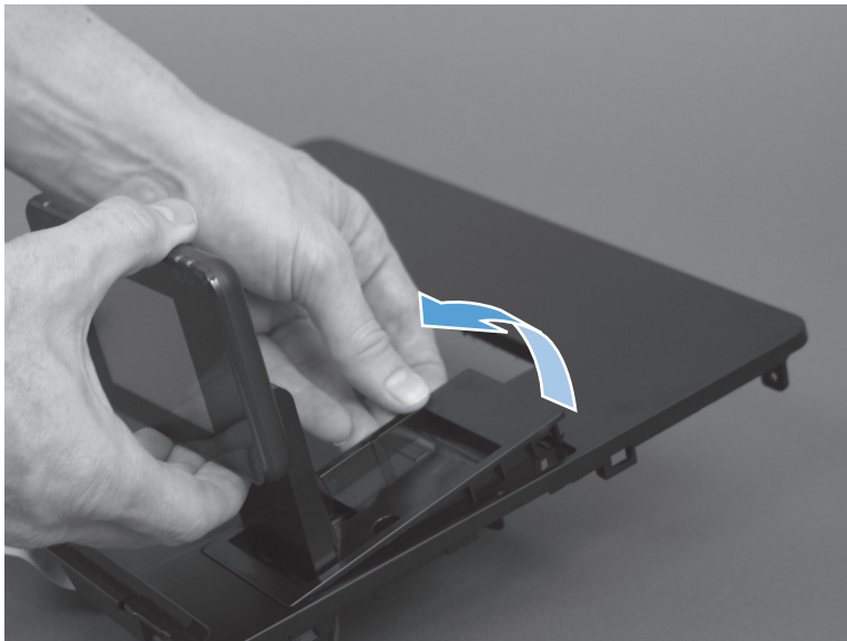
Figure 1-24 Remove the touchscreen control panel (3 of 3)
