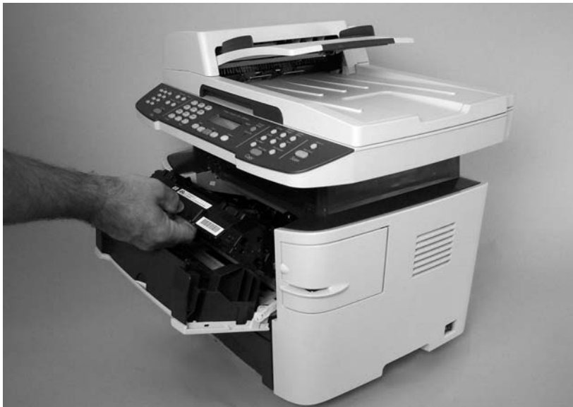
Figure 5-4 Remove the print cartridge (2 of 2)
