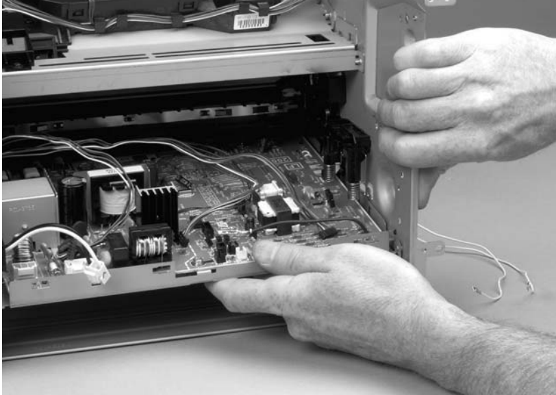
Figure 5-78 Remove the ECU (7 of 8)
