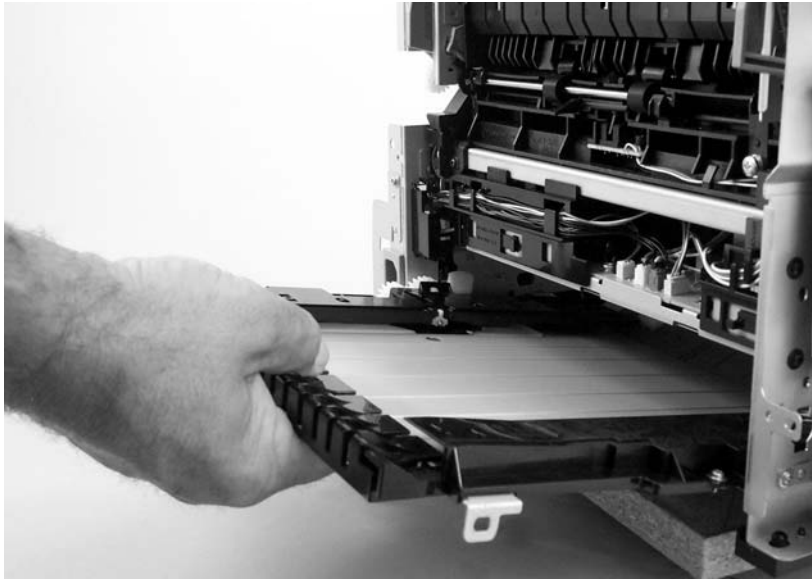
Figure 5-50 Remove the duplex assembly (3 of 3)
