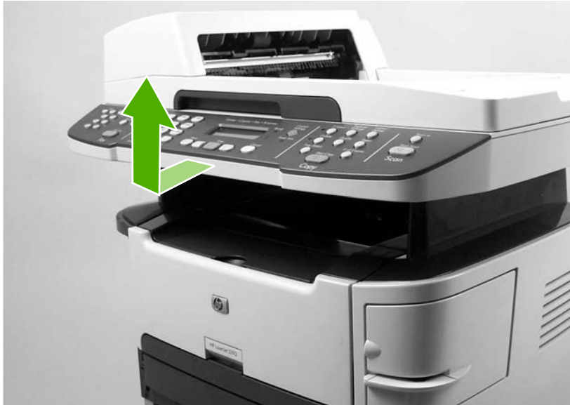
Figure 5-30 Remove the scanner/ADF assembly (3 of 3)
