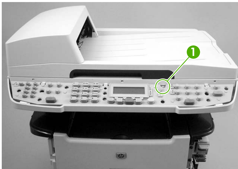
Figure 5-32 Remove the bezel and control panel (2 of 4)
