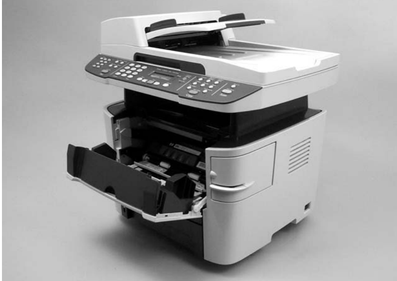
Figure 5-3 Remove the print cartridge (1 of 2)
