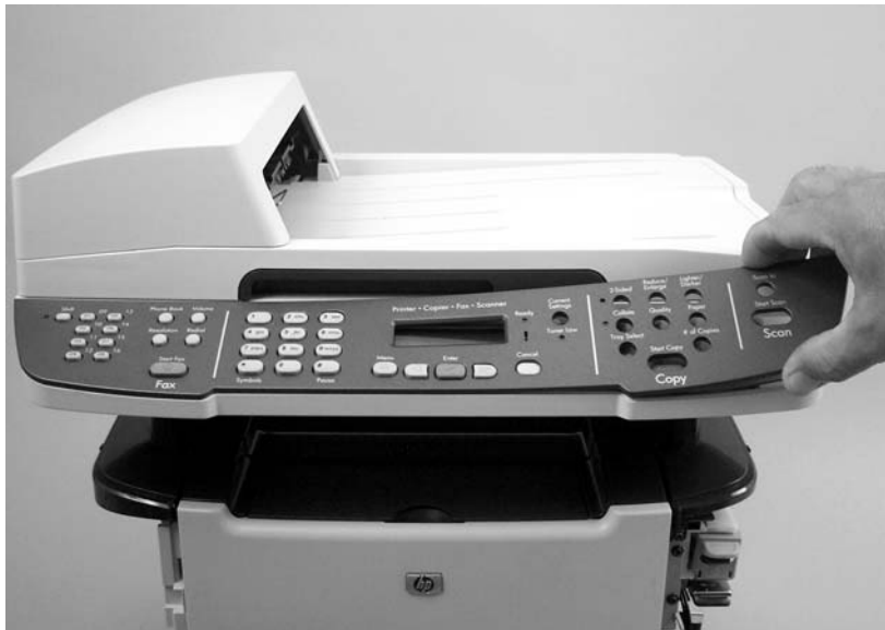
Figure 5-31 Remove the bezel and control panel (1 of 4)
