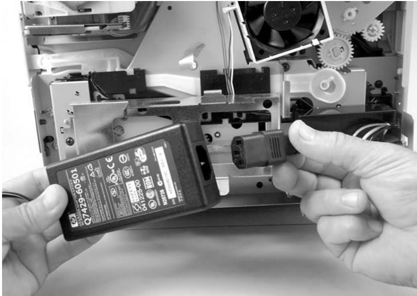
Figure 5-39 Remove the convenience-stapler power assembly (3 of 3)
