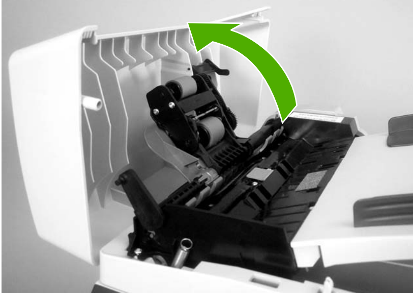
Figure 5-21 Replacing the ADF pickup-roller assembly (3 of 6)
