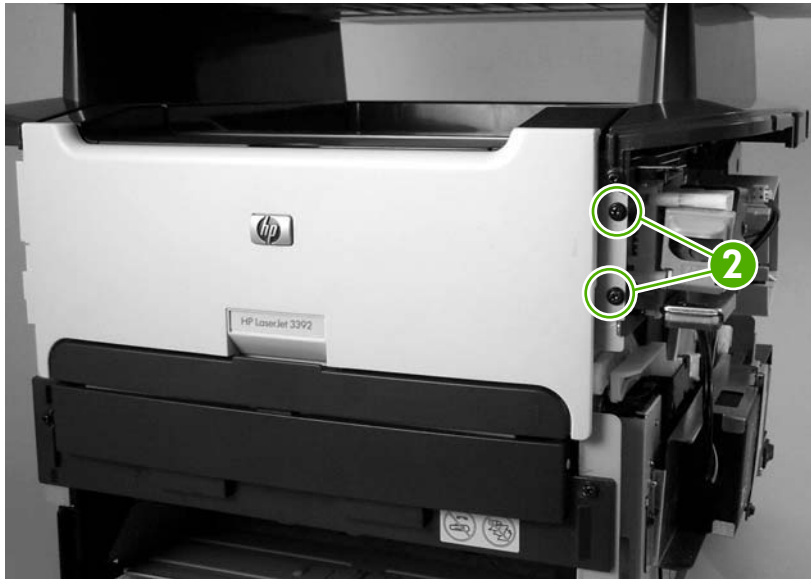
Figure 5-36 Remove the convenience-stapler assembly (2 of 2)
