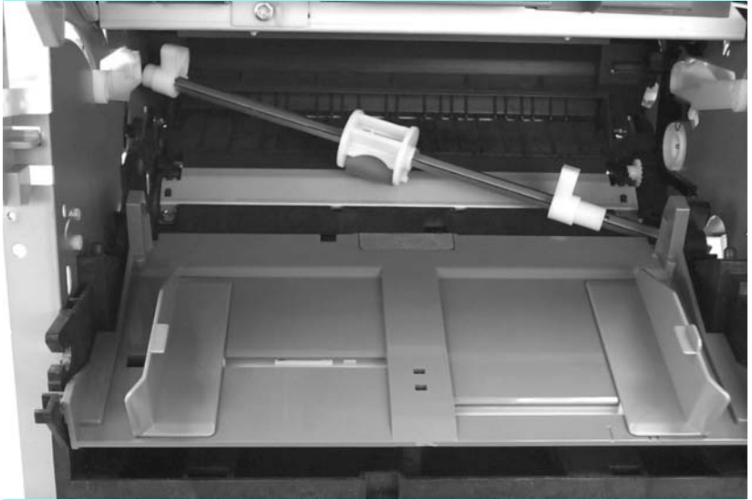
Figure 77. Removing the paper lift-plate assembly (2 of 3)
