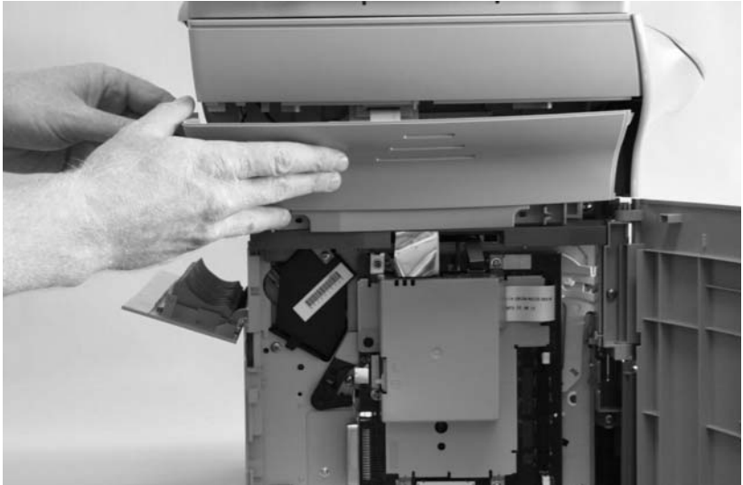
Figure 26. Removing the left scanner cover
