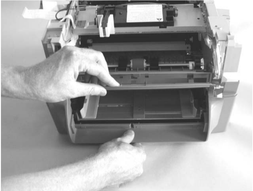
Figure 52. Removing the front cover (2 of 2)
