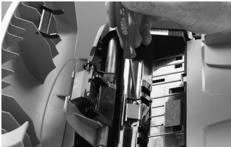
Figure 34. Removing the ADF separation pad
