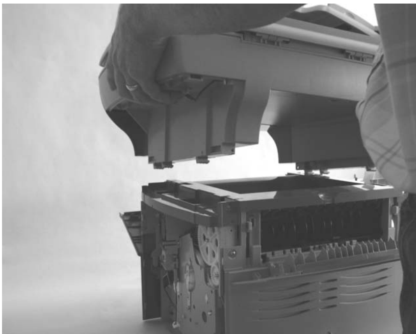
Figure 30. Separating the scanner from the printer (4 of 4)
