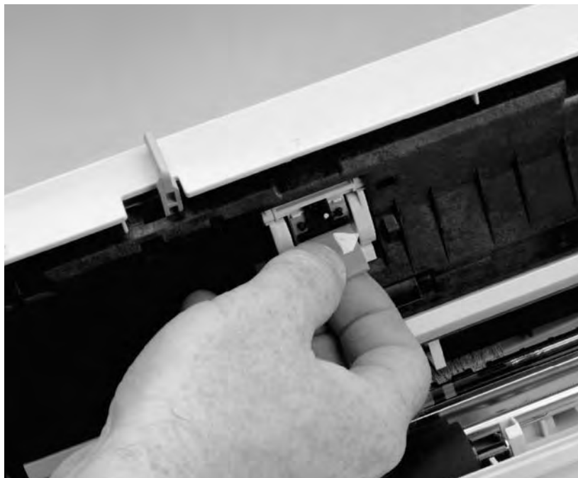
Figure 34. Document scanner separation pad removal
