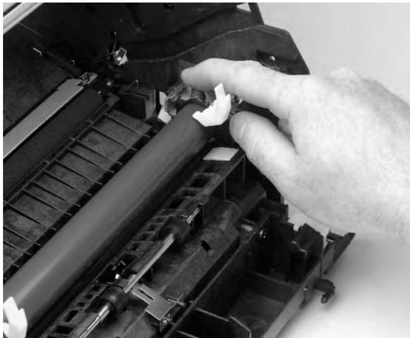
Figure 48. Fusing element metal clips reinstallation
