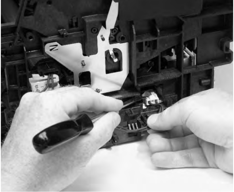
Figure 50. Fusing element removal (3 of 4)
