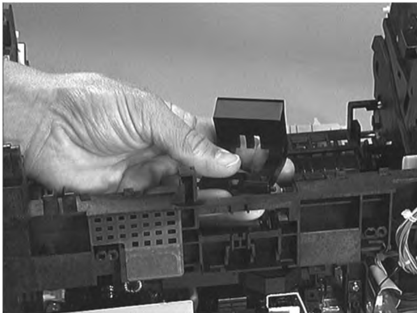
Figure 63. Separation pad removal (2 of 2)
