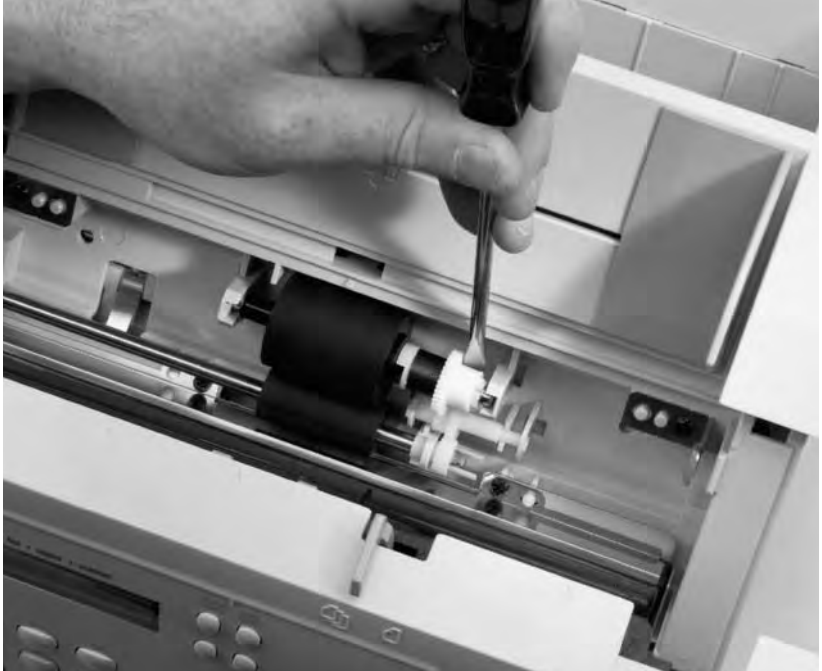
Figure 33. Document scanner pickup roller removal
