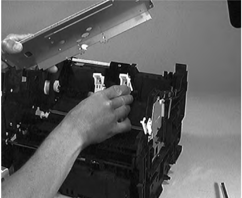
Figure 60. Paper-pickup assembly removal (2 of 2)
