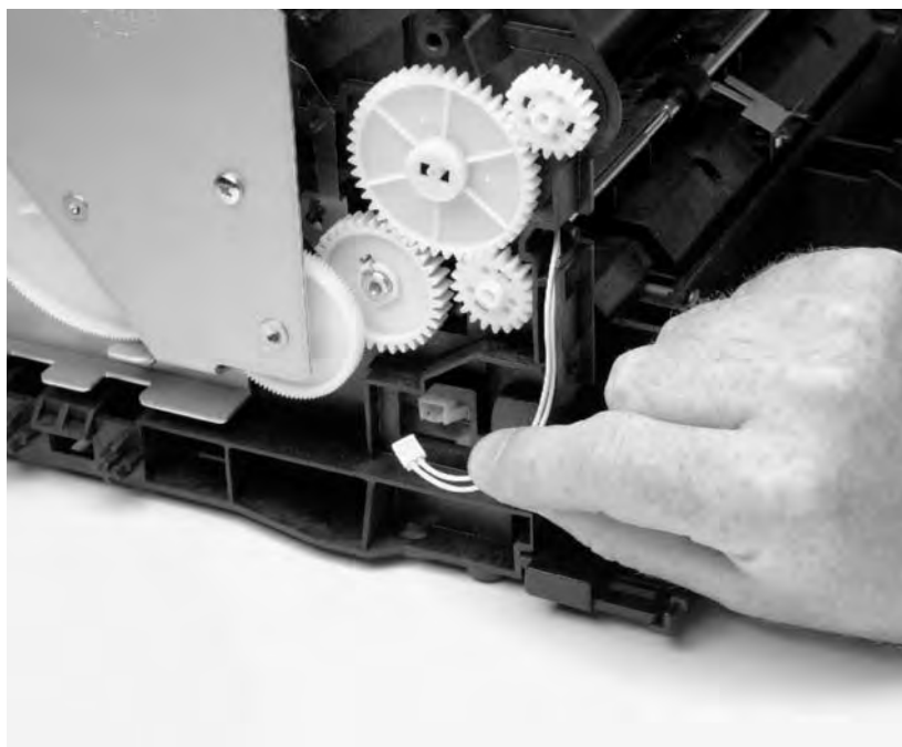
Figure 49. Fusing element removal (2 of 4)
