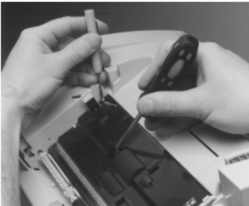
Figure 30. Contact image sensor removal (1 of 2)
