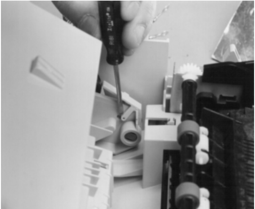
Figure 25. Printer door removal (3 of 3)
