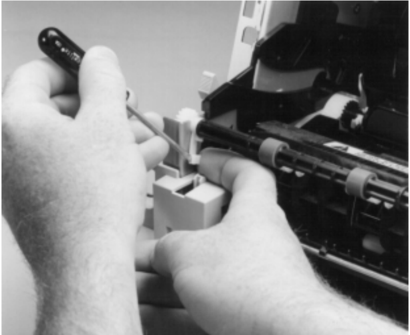
Figure 39. Exit roller removal
