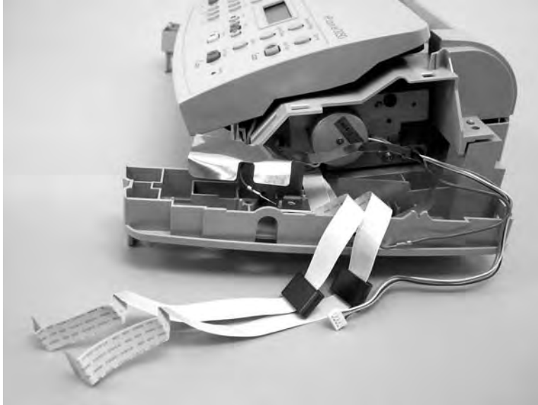
Figure 5-37 Removing the scanner assembly top cover (2 of 4)
