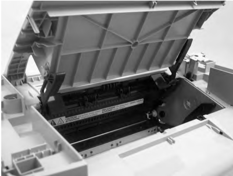
Figure 5-106 Removing the print-cartridge door (1 of 2)
