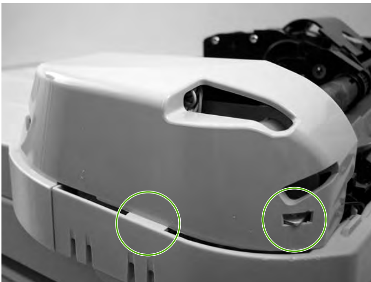
Figure 5-49 ADF cover correctly installed
