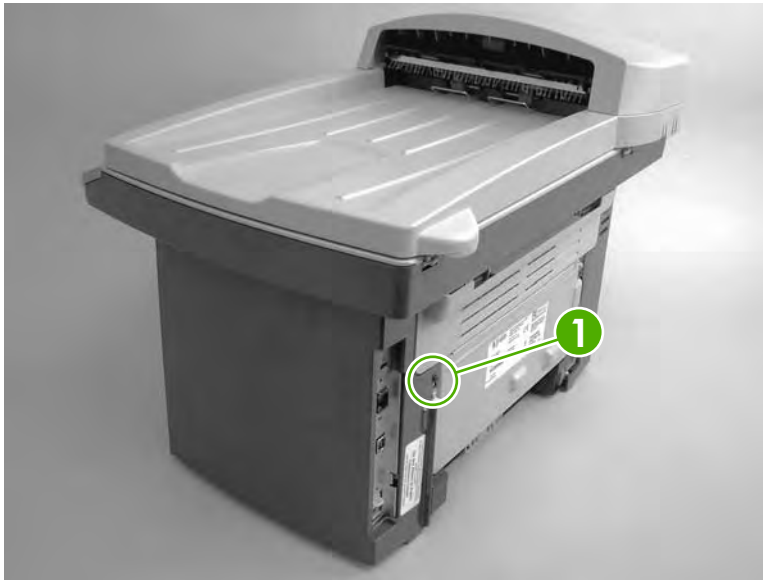
Figure 5-72 Removing the scanner assembly (1 of 13)
