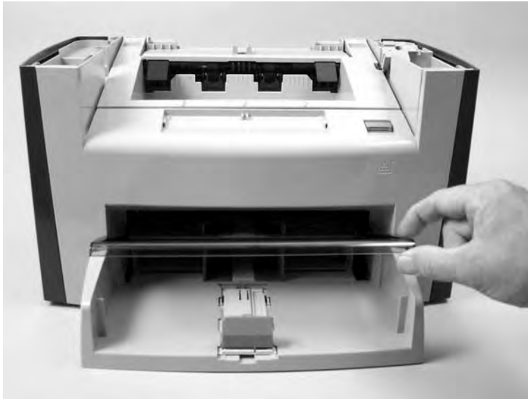
Figure 5-96 Removing the media input tray (1 of 3)
