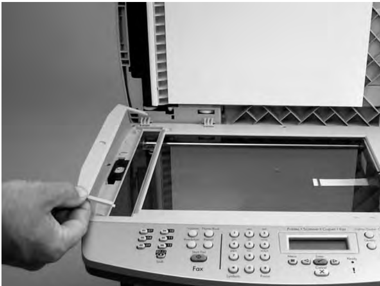
Figure 5-70 Removing the ADF scanner glass (2 of 3)
