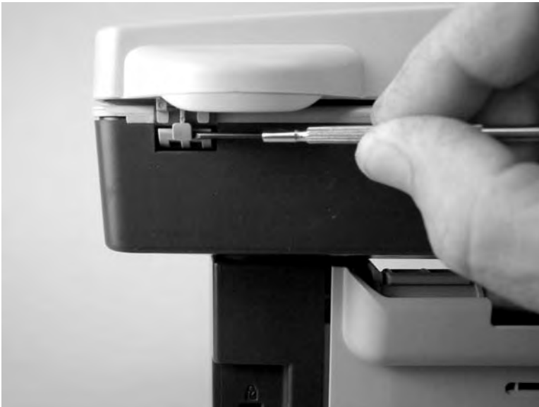
Figure 5-51 Removing the flatbed lid (3 of 5)
