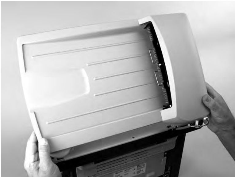
Figure 5-53 Removing the flatbed lid (5 of 5)
