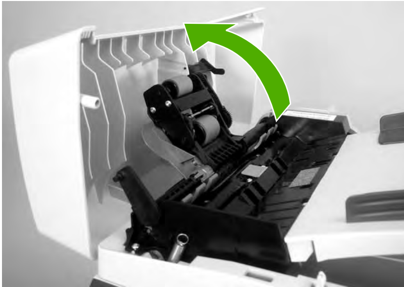
Figure 5-65 Replacing the ADF pickup roller and load-arm assembly (3 of 6)
