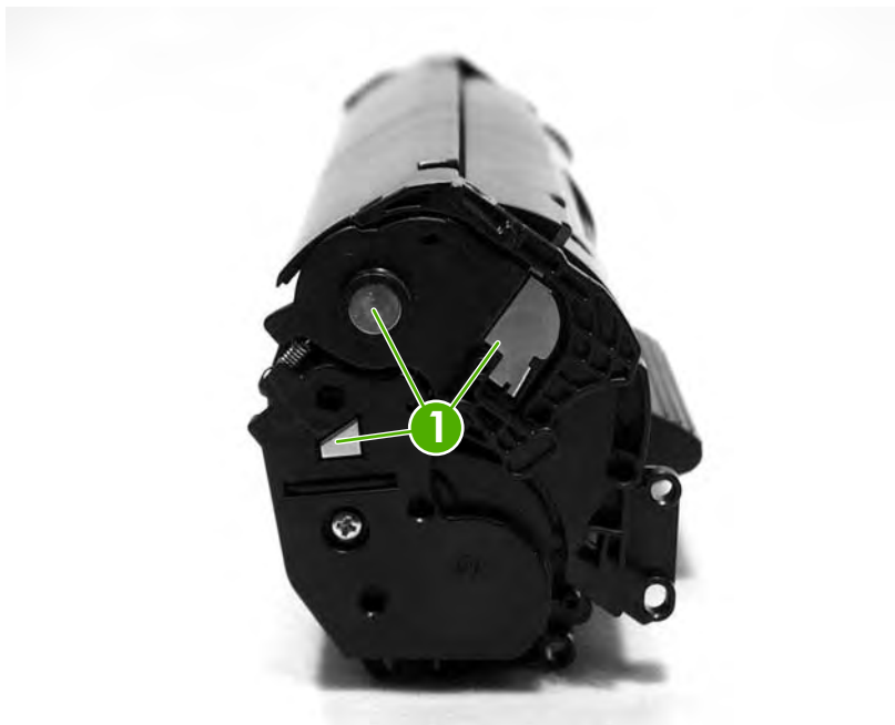
Figure 6-1 Print-cartridge high-voltage contacts
