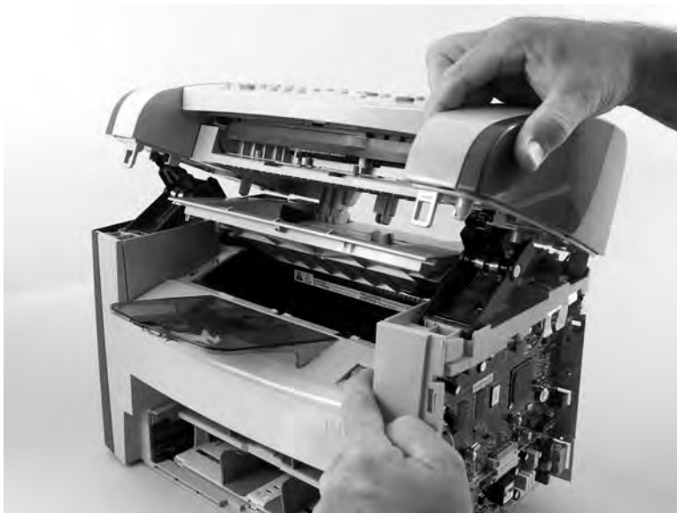
Figure 5-29 Removing the scanner assembly (8 of 14)
