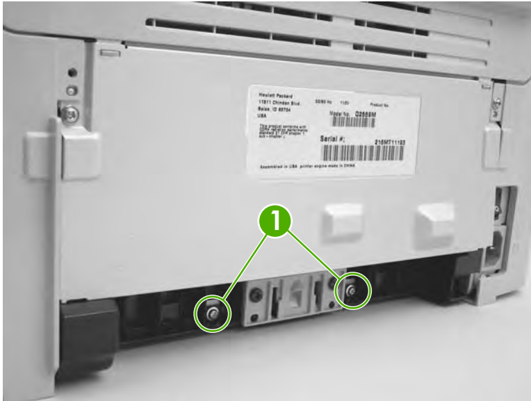
Figure 5-86 Removing the printer separation pad (1 of 2)
