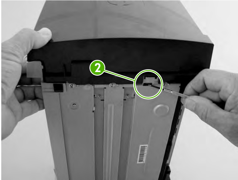
Figure 5-26 Removing the scanner assembly (5 of 14)
