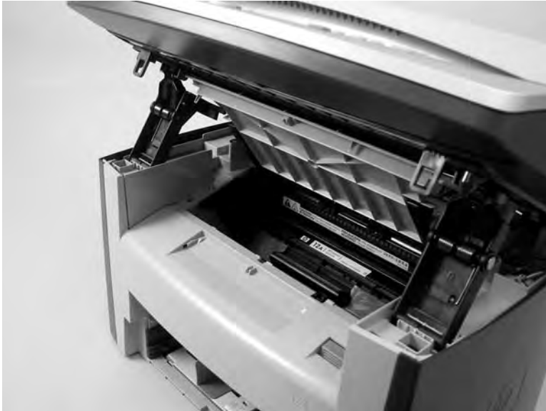
Figure 5-88 Removing the print cartridge (1 of 2)
