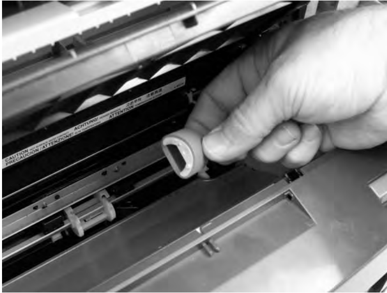
Figure 5-92 Removing the printer pickup roller (3 of 5)
