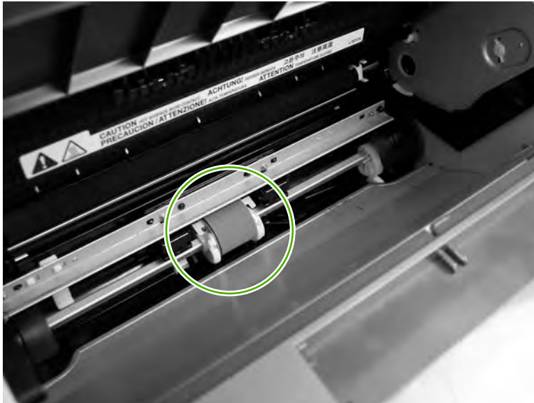
Figure 5-90 Removing the printer pickup roller (1 of 5)
