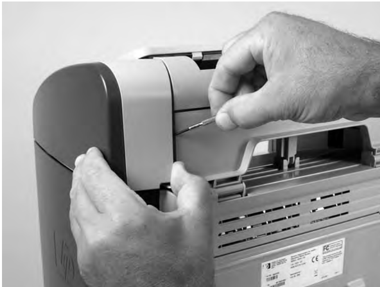
Figure 5-10 Removing the scanner side covers (1 of 2)
