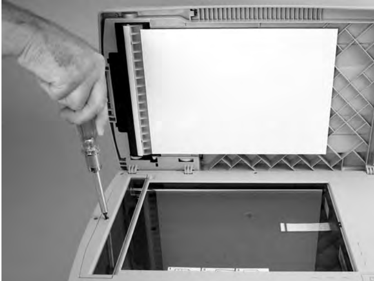
Figure 5-69 Removing the ADF scanner glass (1 of 3)
