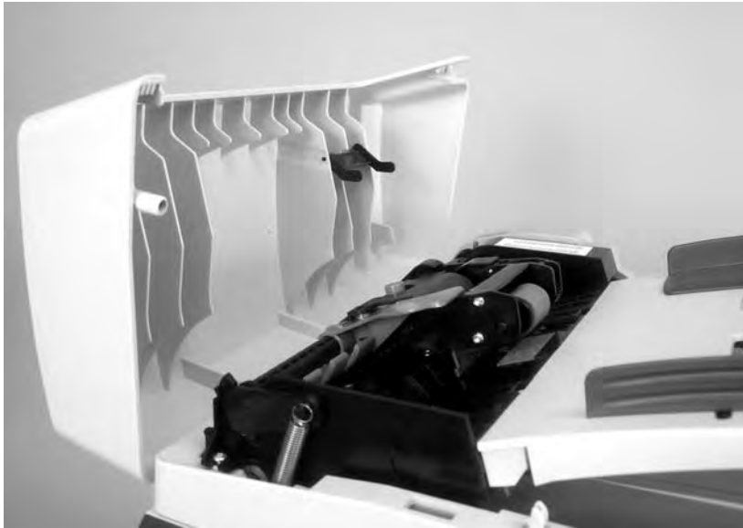
Figure 5-63 Replacing the ADF pickup roller and load-arm assembly (1 of 6)
