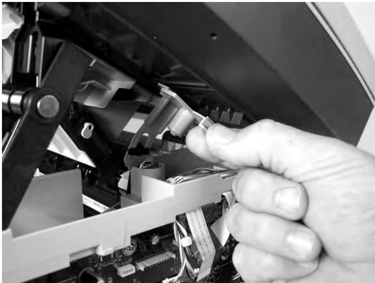
Figure 5-79 Removing the scanner assembly (8 of 13)
