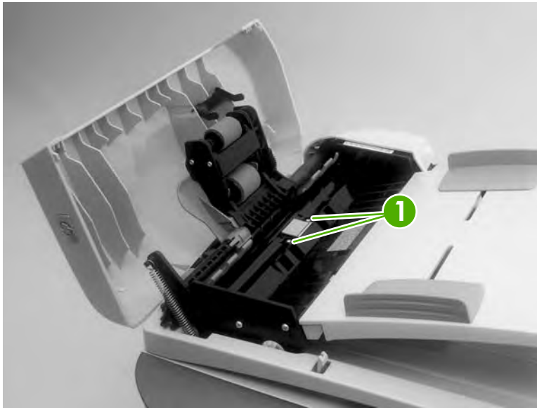
Figure 5-61 Removing the ADF separation pad
