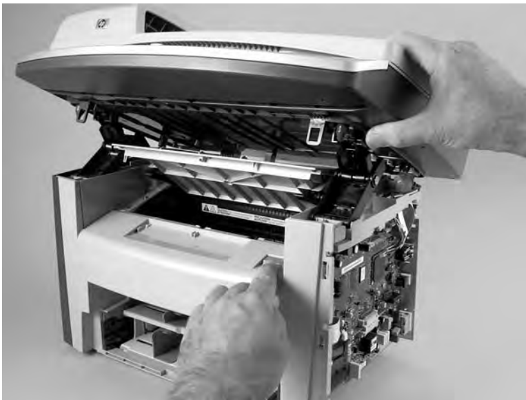
Figure 5-77 Removing the scanner assembly (6 of 13)
