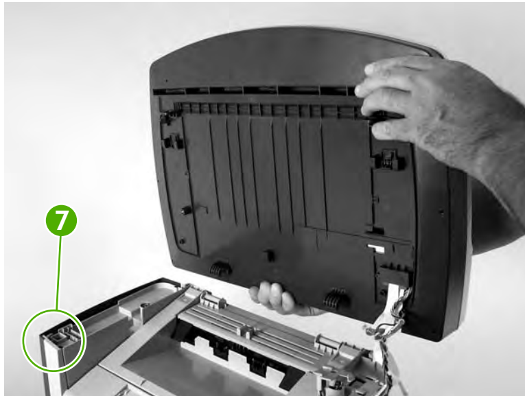
Figure 5-84 Removing the scanner assembly (13 of 13)
