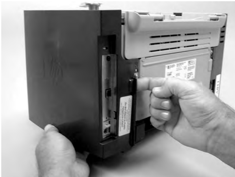
Figure 5-103 Removing the side covers (2 of 4)
