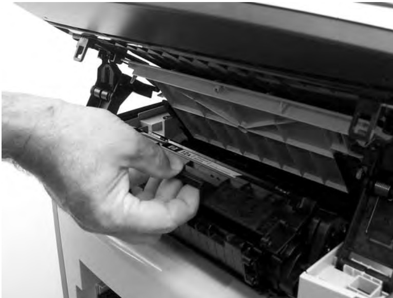
Figure 5-89 Removing the print cartridge (2 of 2)
