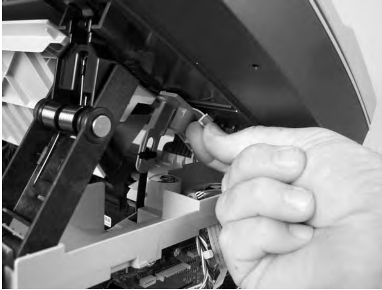
Figure 5-78 Removing the scanner assembly (7 of 13)
