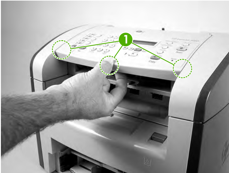
Figure 5-13 Removing the control-panel bezel (1 of 3)
