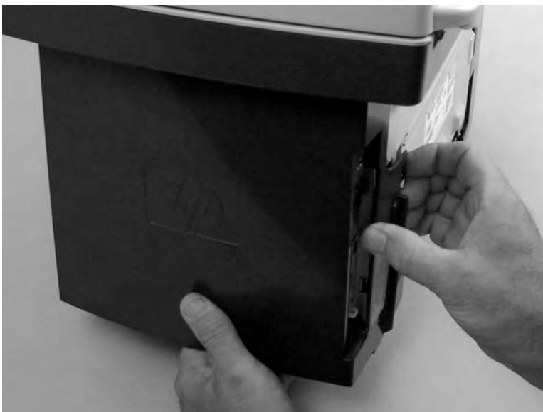
Figure 5-73 Removing the scanner assembly (2 of 13)
