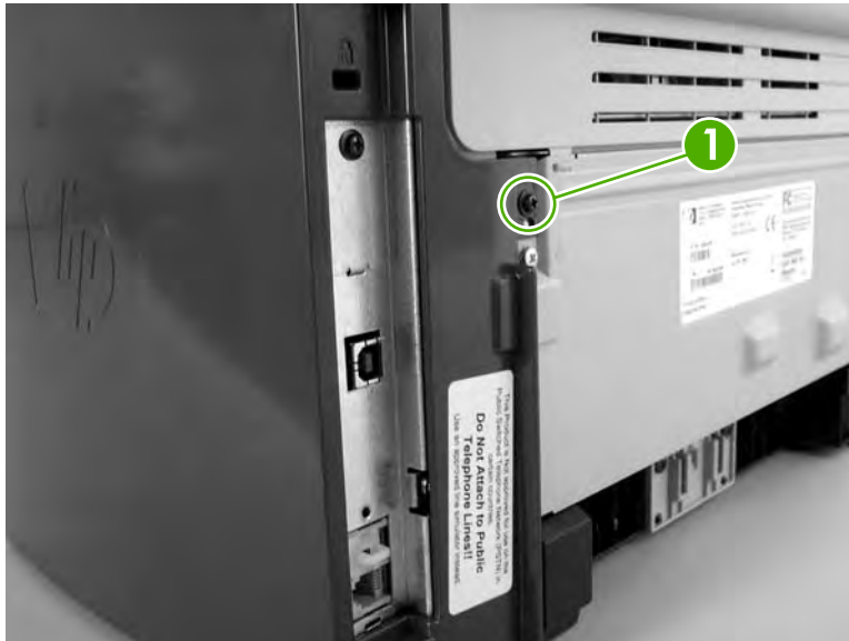
Figure 5-24 Removing the scanner assembly (3 of 14)
