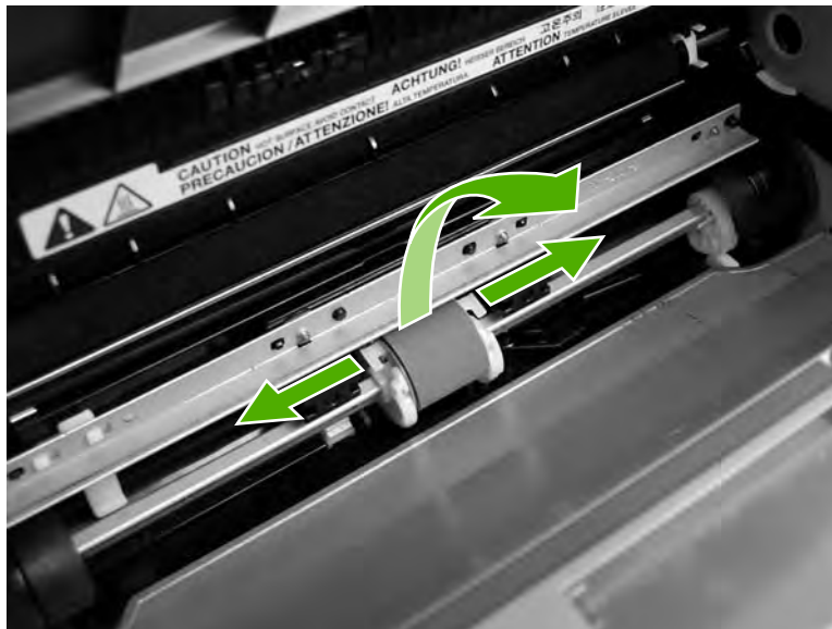
Figure 5-91 Removing the printer pickup roller (2 of 5)
