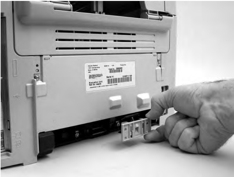
Figure 5-87 Removing the printer separation pad (2 of 2)
