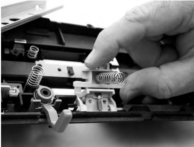
Figure 5-20 Removing the separation-pad assembly (2 of 3)
