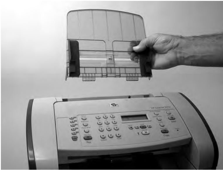
Figure 5-22 Removing the scanner assembly (1 of 14)
