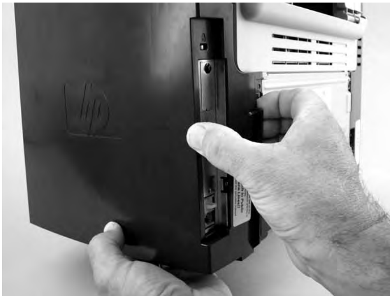
Figure 5-25 Removing the scanner assembly (4 of 14)
