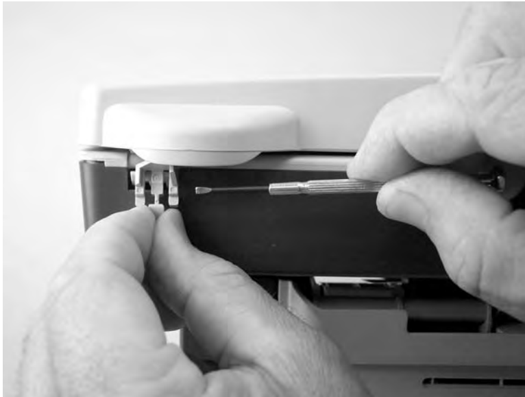
Figure 5-52 Removing the flatbed lid (4 of 5)
