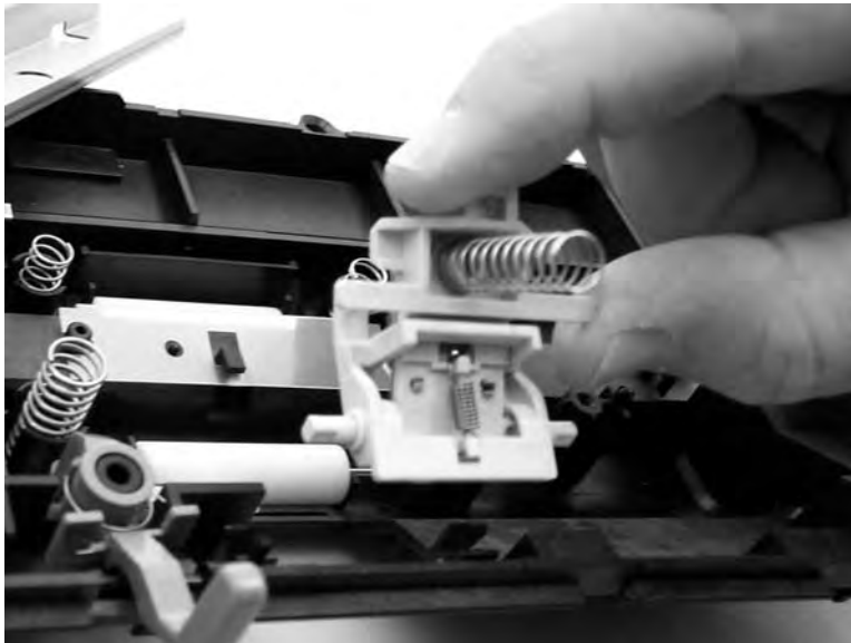
Figure 5-21 Removing the separation-pad assembly (3 of 3)
