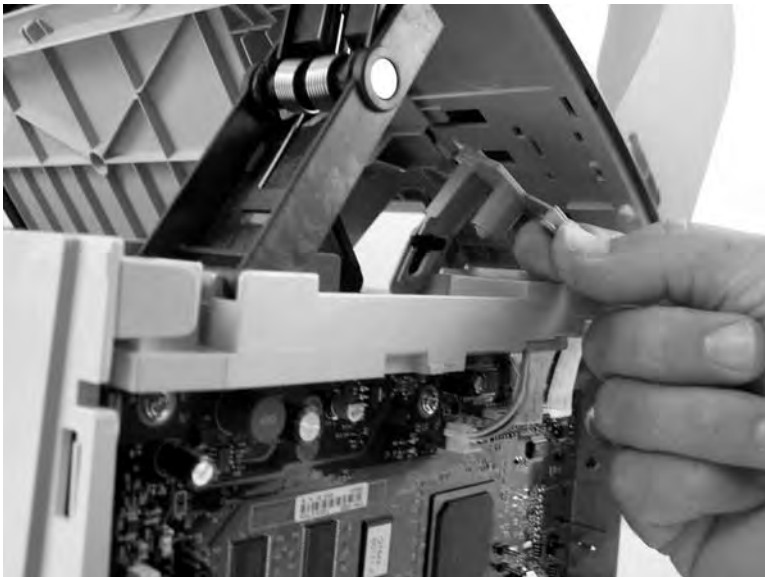
Figure 5-31 Removing the scanner assembly (10 of 14)
