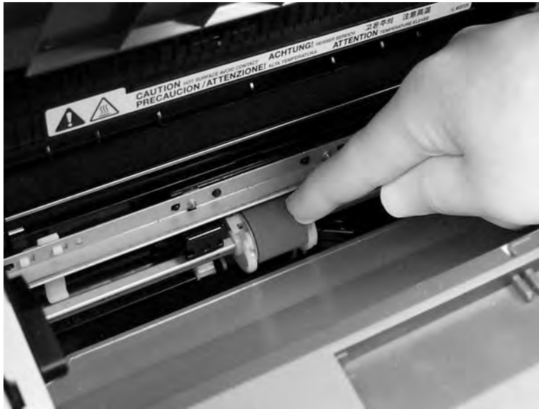
Figure 5-94 Removing the printer pickup roller (5 of 5)
