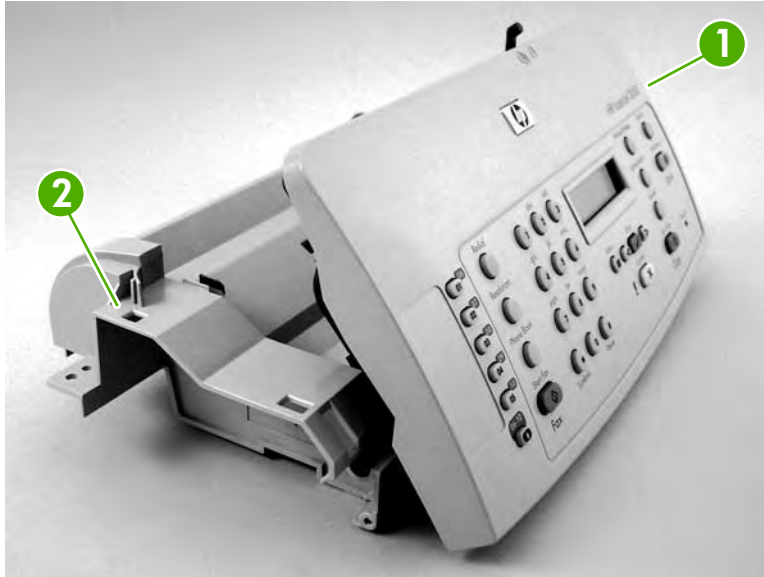
Figure 5-40 Removing the top-cover assembly (1 of 2)
