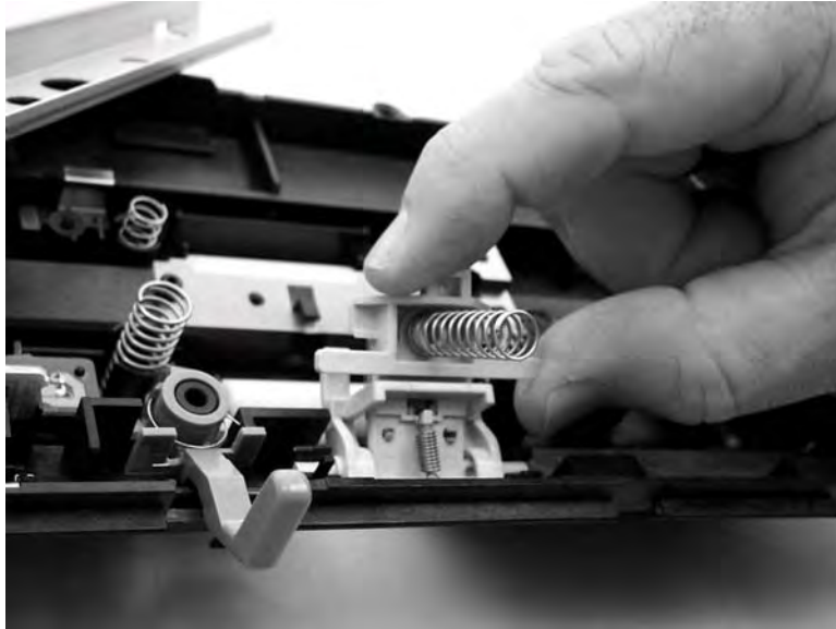
Figure 5-22. Remove the separation pad assembly (2 of 3)
