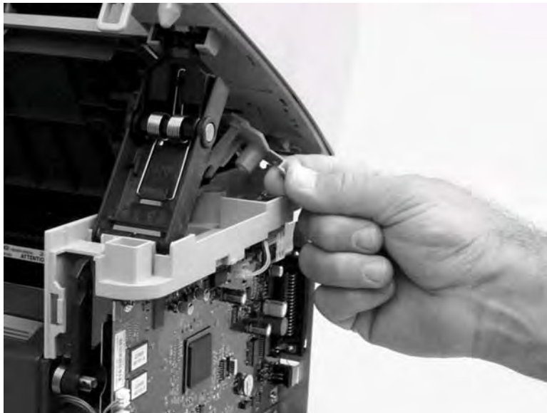
Figure 5-33. Remove the scanner assembly (10 of 15)
