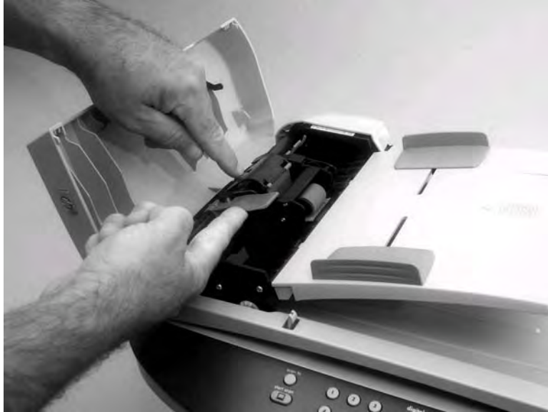
Figure 5-69. Remove the ADF pickup roller (1 of 2)
