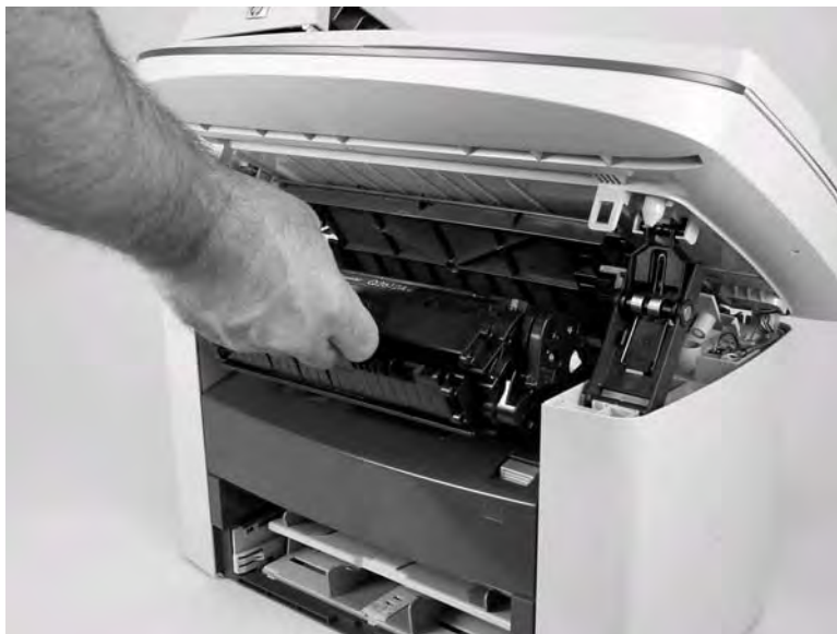
Figure 5-92. Remove the print cartridge (2 of 2)
