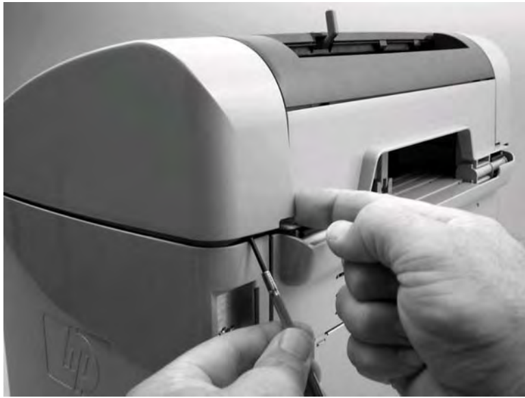
Figure 5-10. Remove the scanner side covers (1 of 3)
