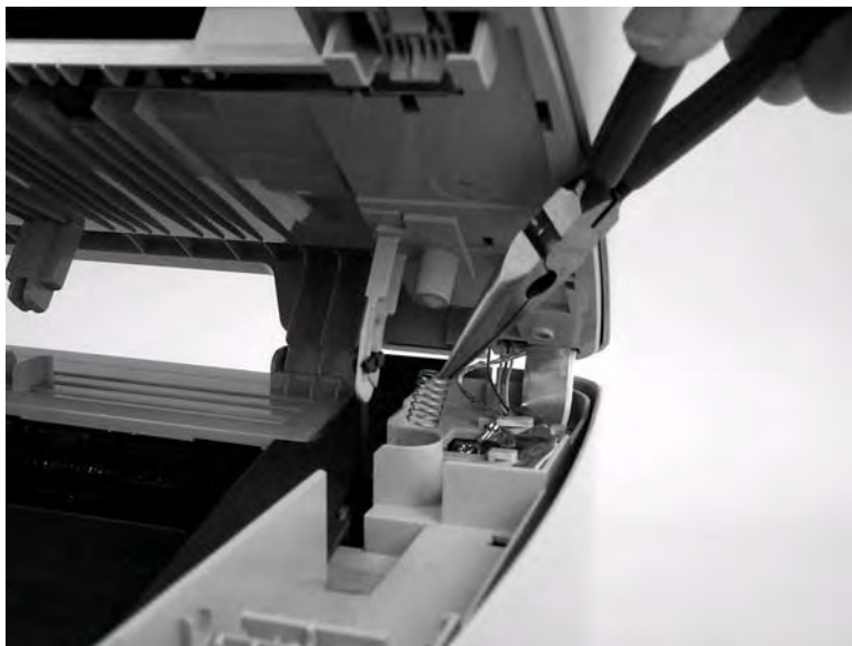
Figure 5-9. Remove the link assemblies and scanner support frame springs (4 of 4)
