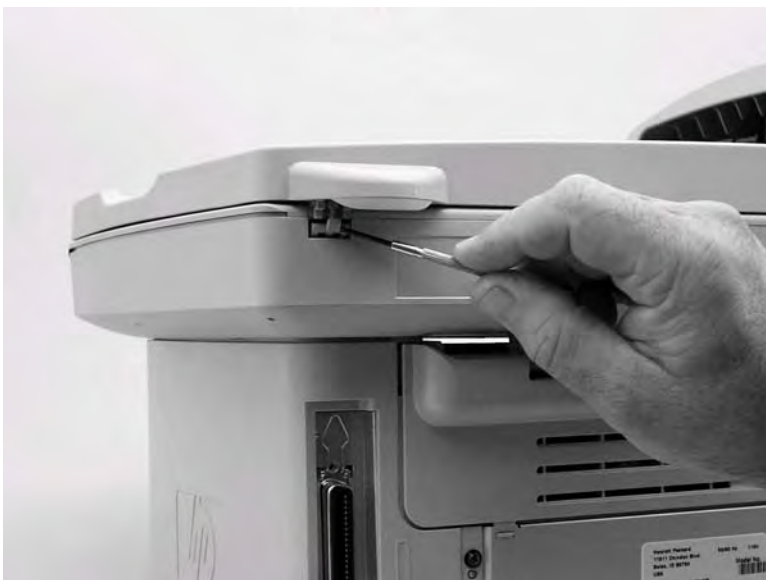
Figure 5-56. Remove the flatbed lid (3 of 5)
