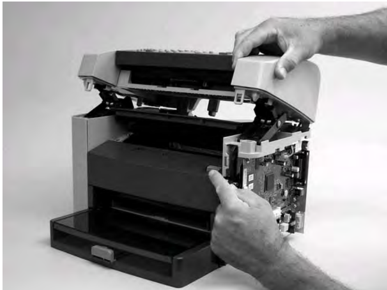
Figure 5-31. Remove the scanner assembly (8 of 15)
