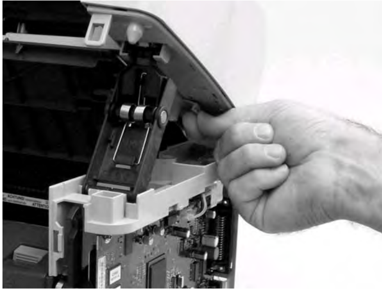
Figure 5-32. Remove the scanner assembly (9 of 15)
