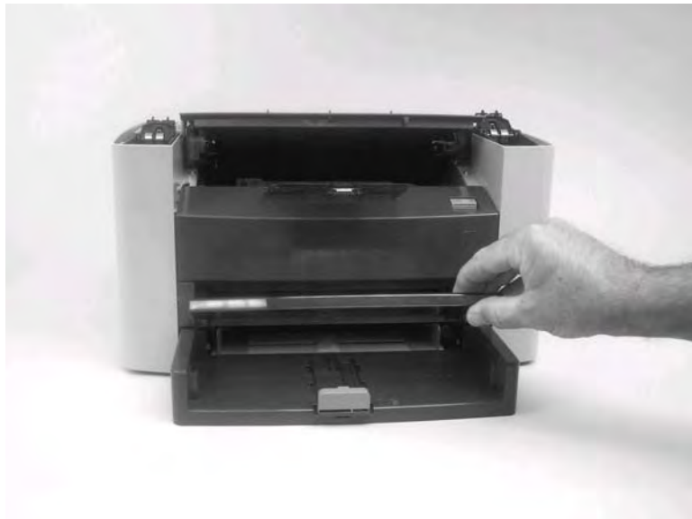
Figure 5-98. Remove the media input tray (1 of 3)
