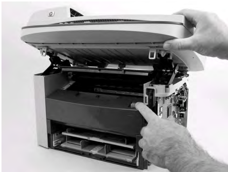
Figure 5-80. Remove the scanner assembly (6 of 13)
