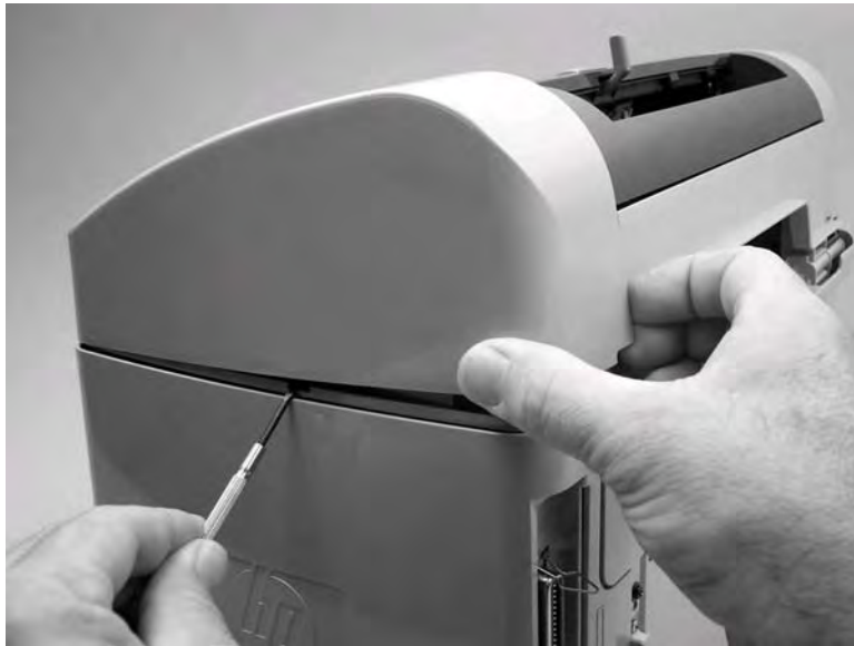
Figure 5-11. Remove the scanner side covers (2 of 3)
