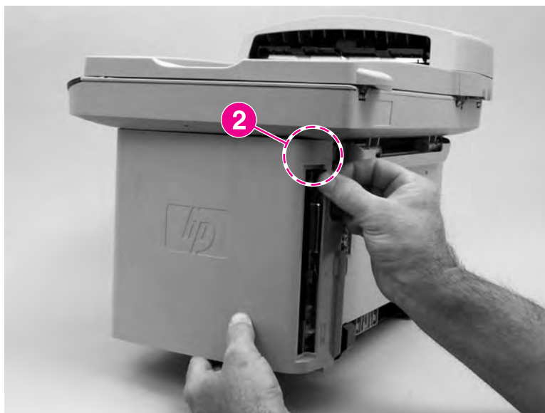
Figure 5-76. Remove the scanner assembly (2 of 13)
