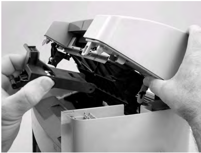
Figure 5-8. Remove the link assemblies and scanner support frame springs (3 of 4)
