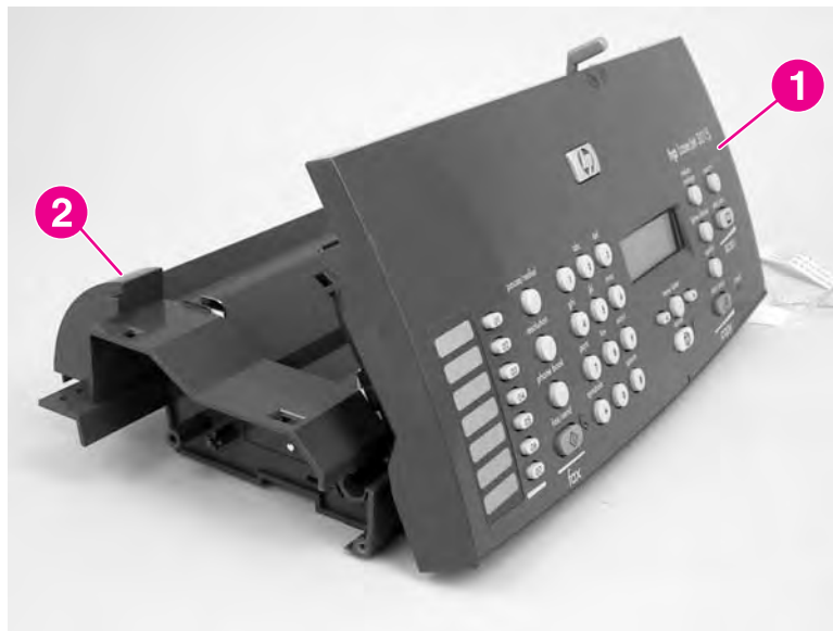
Figure 5-45. Remove the top-cover assembly (1 of 2)
