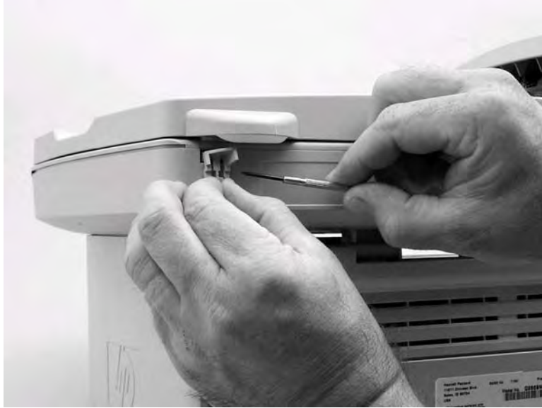
Figure 5-57. Remove the flatbed lid (4 of 5)
