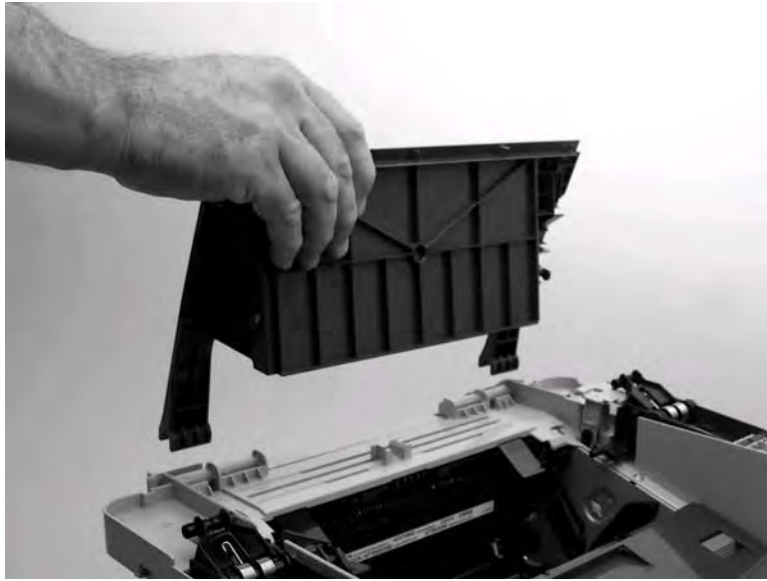
Figure 5-109. Remove the print-cartridge door (2 of 2)
