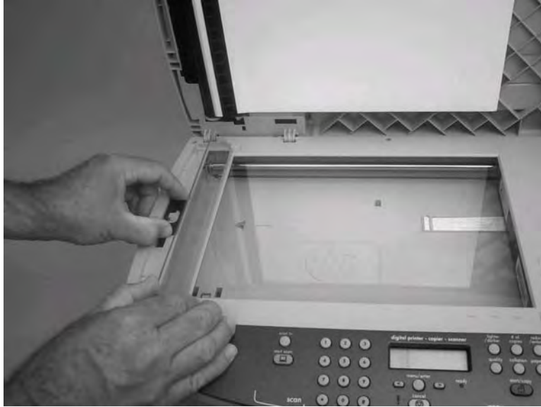
Figure 5-73. Remove the ADF scanner glass (3 of 3)
