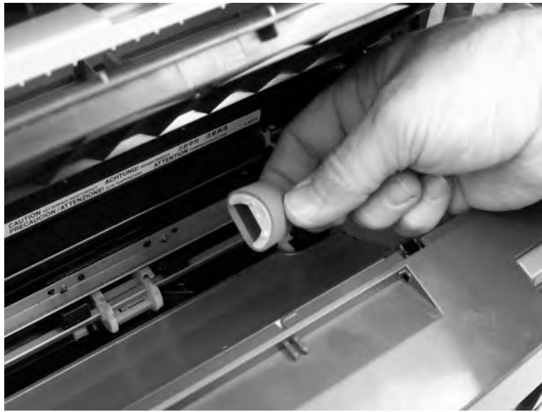
Figure 5-95. Remove the printer pickup roller (3 of 5)
