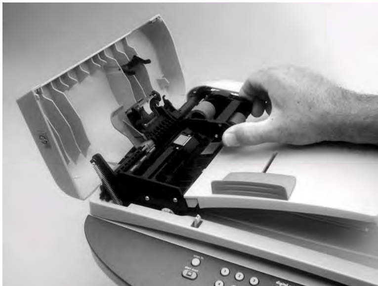
Figure 5-70. Remove the ADF pickup roller (2 of 2)
