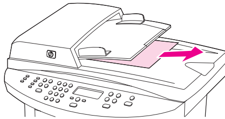
Figure 6-7. Clearing output bin jams (HP LaserJet 3020 and 3030)
