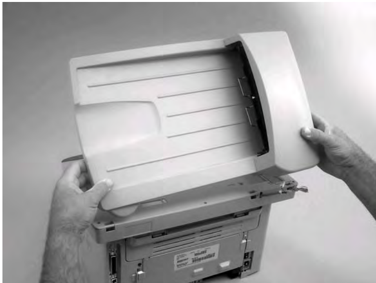
Figure 5-58. Remove the flatbed lid (5 of 5)
