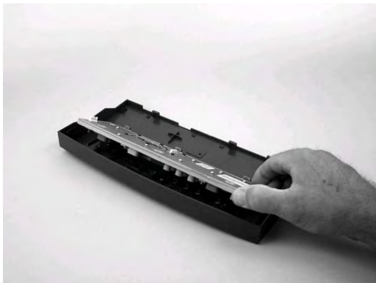
Figure 5-18. Remove the control-panel assembly (2 of 2)
