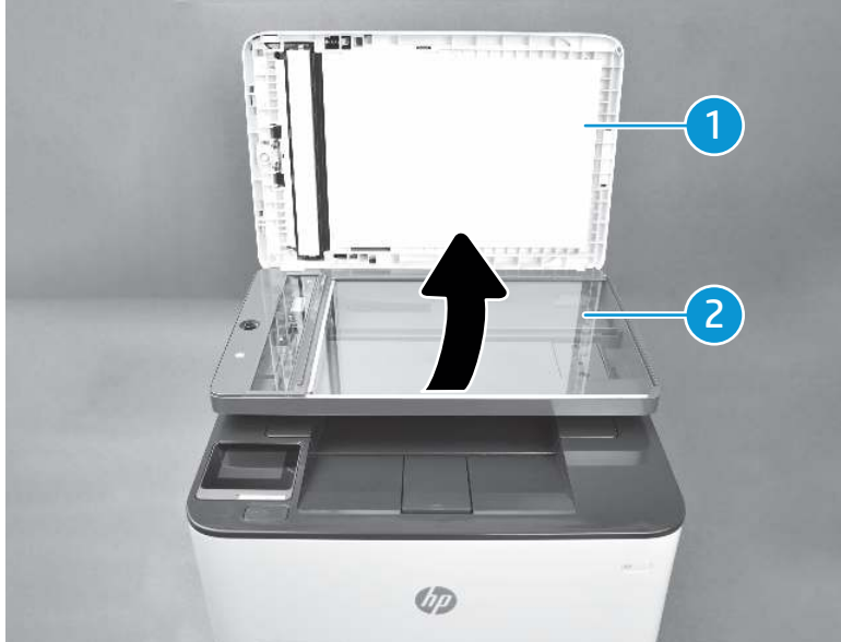
Figure 2-22 Clean the white plastic backing and the scanner glass
