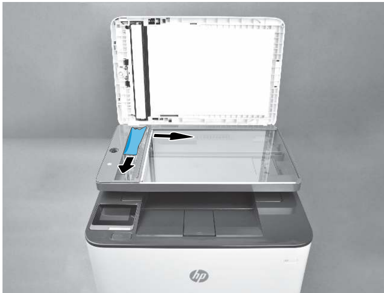
Figure 2-23 Dry the white plastic backing and the scanner glass
