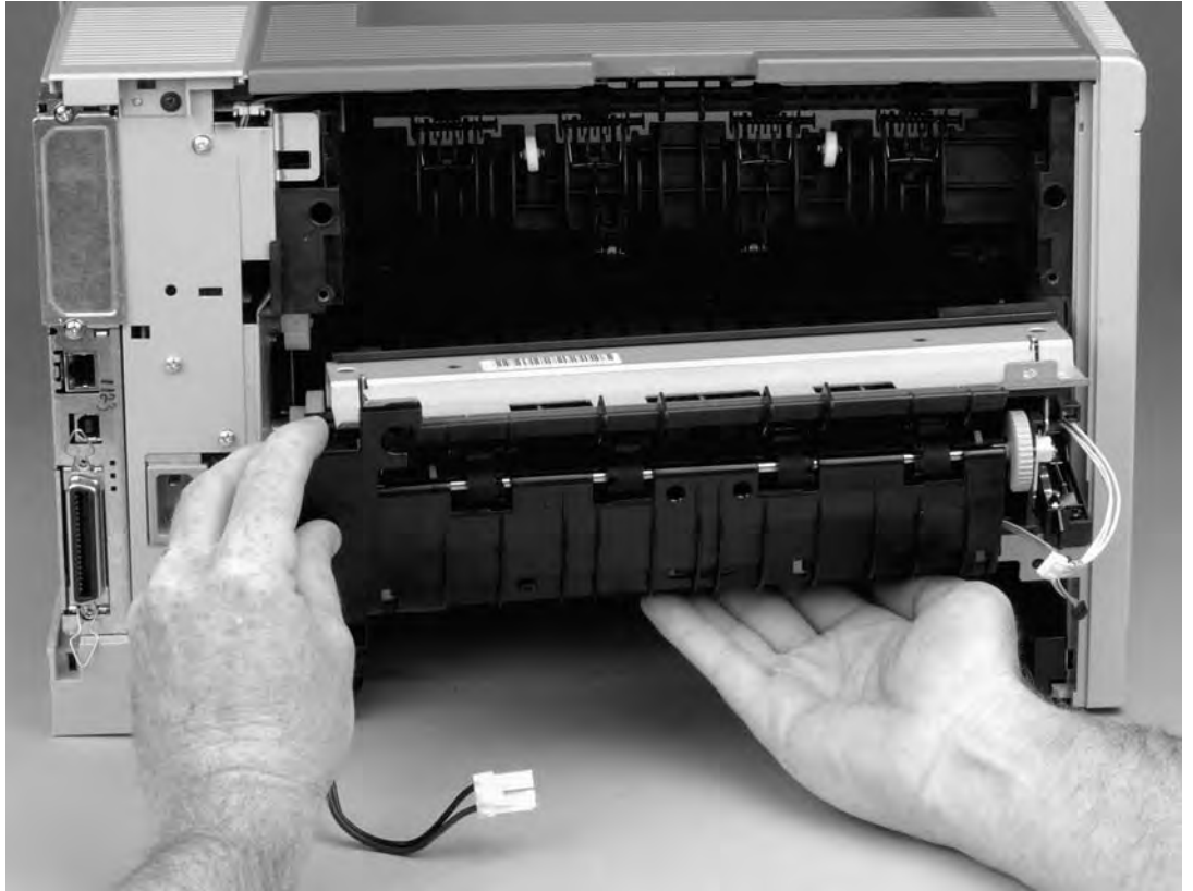
Figure 6-23. Removing the fuser (5 of 5)
