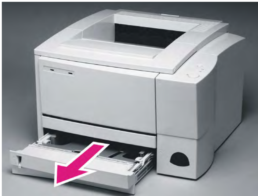
Figure 55. Remove cassette from tray 2
