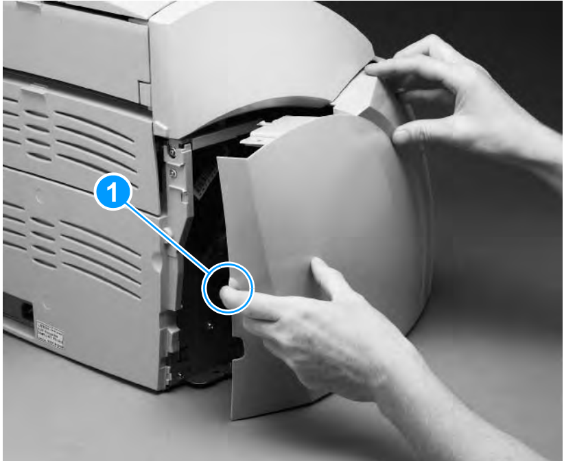
Figure 24. Removing the left side cover
