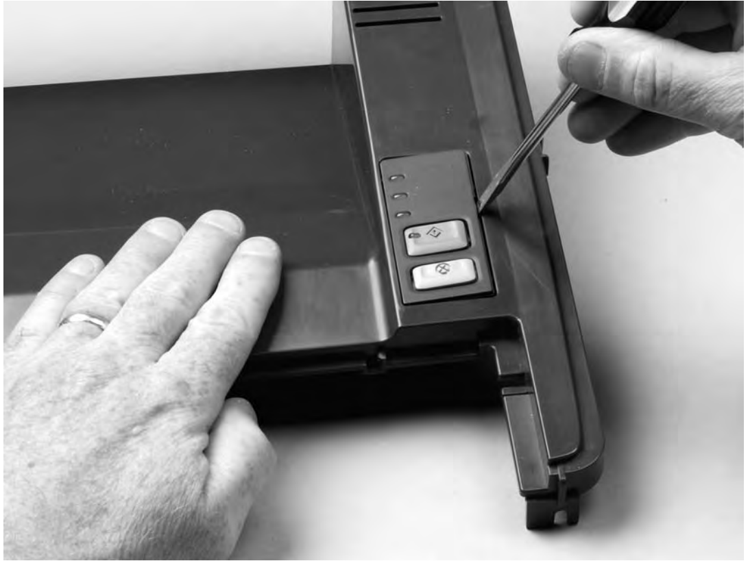
Figure 6-12. Removing the control panel (1 of 2)
