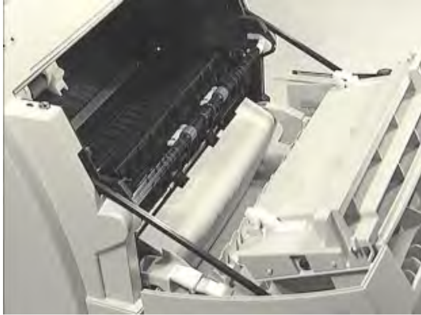
Figure 4-7 Opening the printer door
