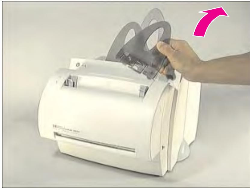
Figure 4-1 Removing the paper guides
