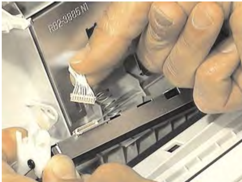
Figure 4-6 Disconnecting the CIS wire connector
