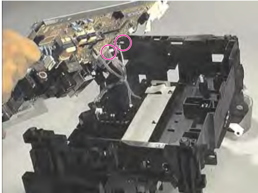
Figure 4-50 Removing the ECU pan (continued on next page)
