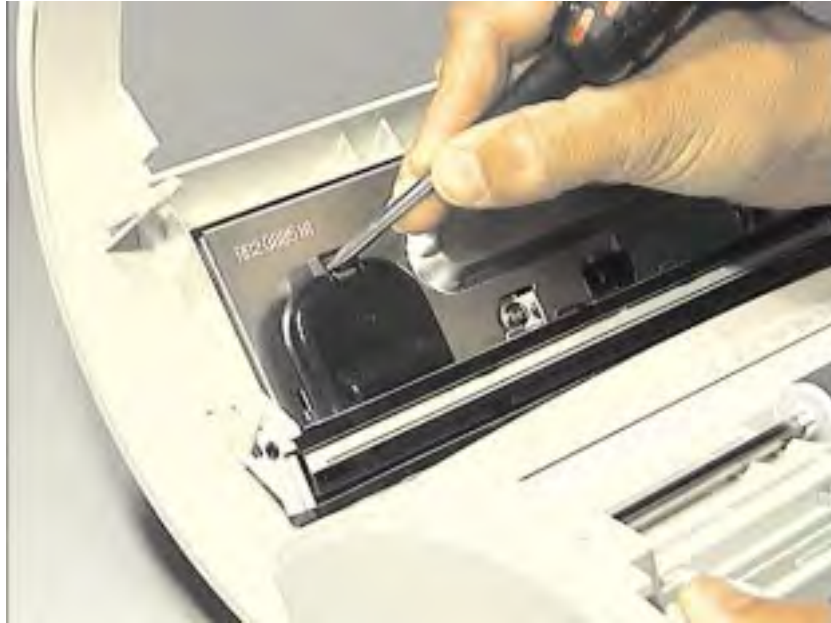
Figure 4-4 Removing the Contact Image Sensor (continued on next page)
