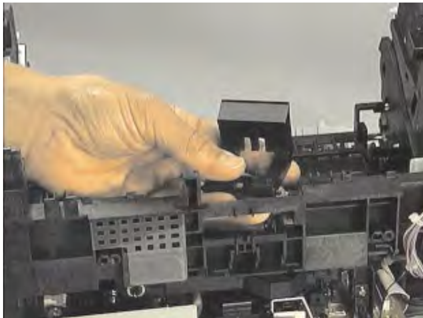
Figure 4-43 Removing the separation pad
