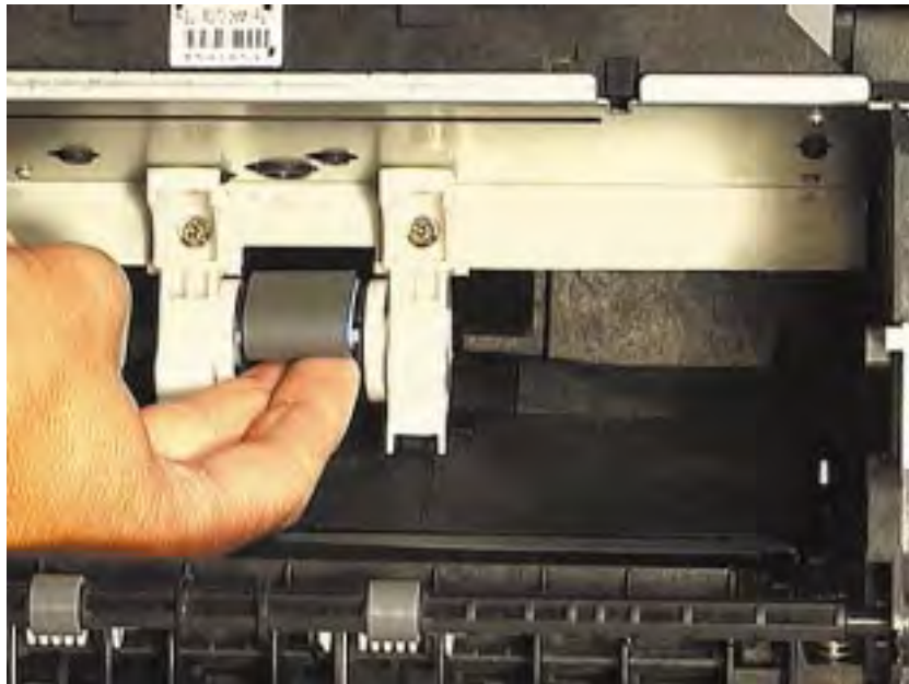
Figure 4-38 Changing the pickup roller
