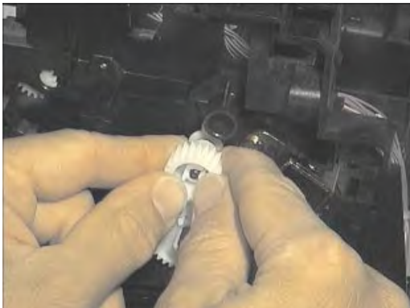
Figure 4-52 Removing the paper feed assembly (continued)
