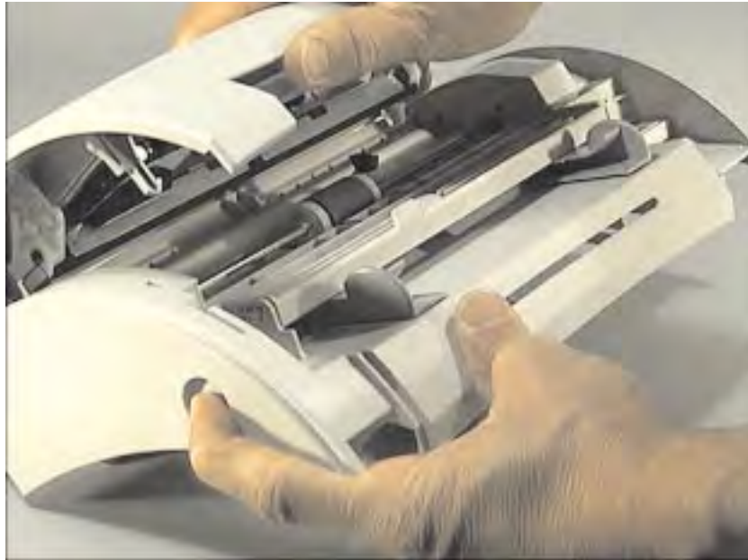
Figure 4-3 Opening the scanner unit
