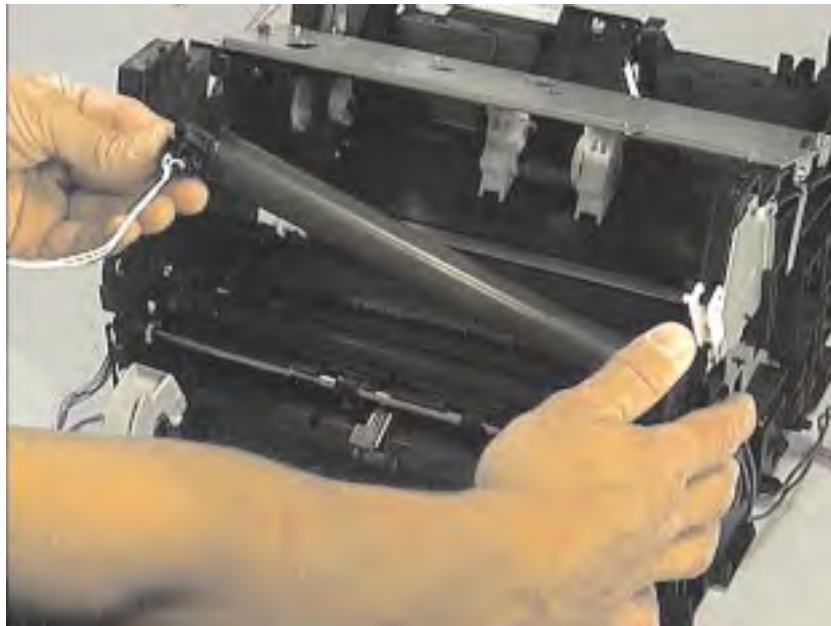
Figure 4-31 Removing the fusing element
