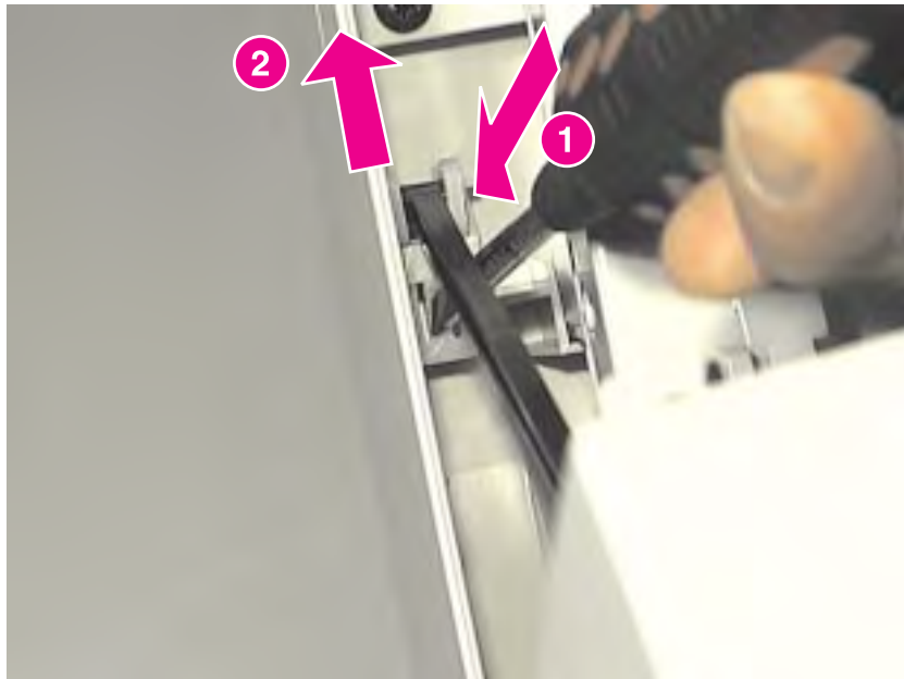
Figure 4-8 Disconnecting the stabilizer bars
