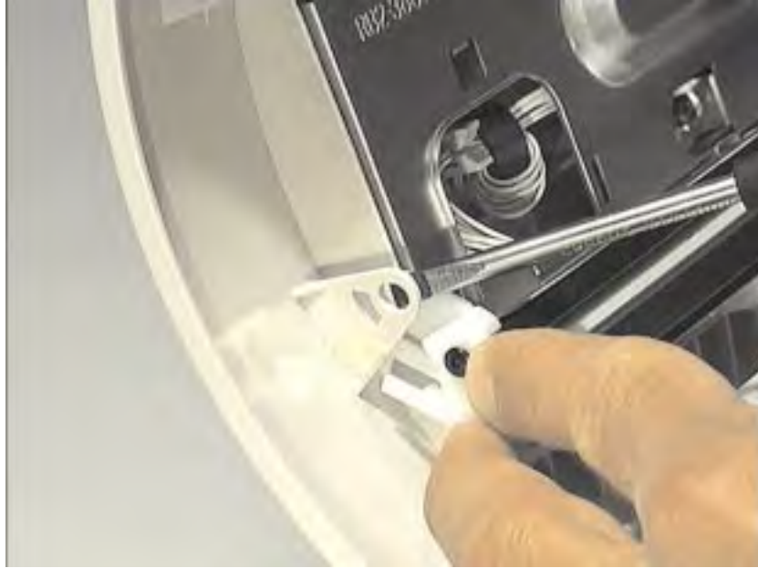
Figure 4-5 Removing the Contact Image Sensor (continued)
