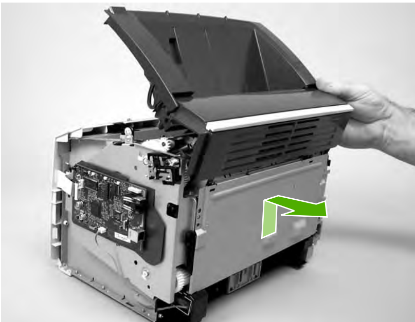
Figure 5-13 Remove the rear panel and top-cover assembly (5 of 6)
