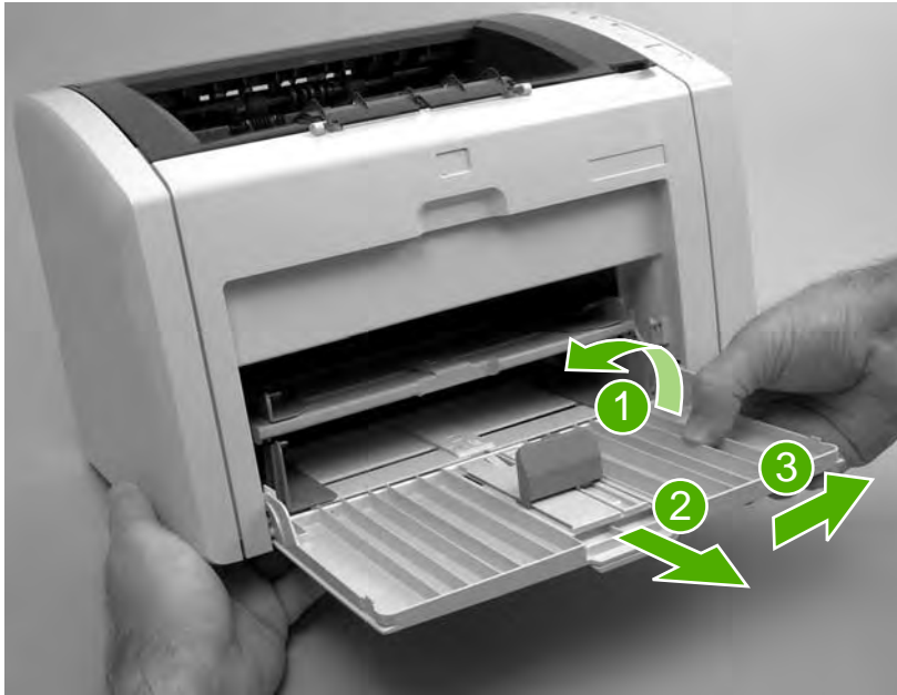
Figure 5-3 Remove the main input tray
