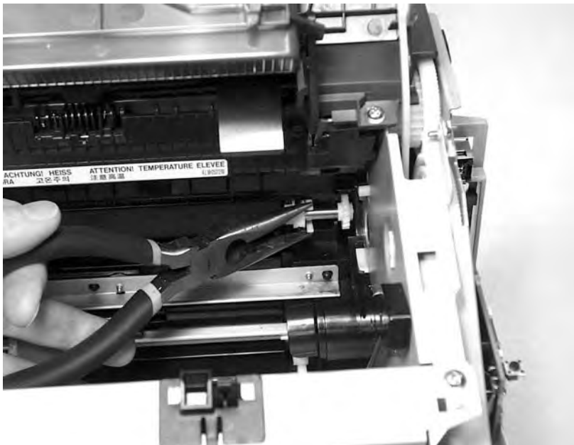
Figure 5-22 Remove the transfer roller (3 of 3)
