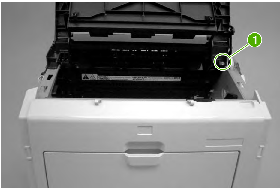
Figure 5-9 Remove the rear panel and top-cover assembly (1 of 6)
