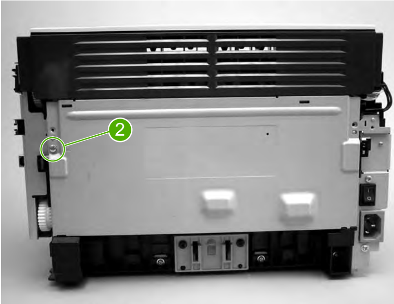
Figure 5-12 Remove the rear panel and top-cover assembly (4 of 6)
