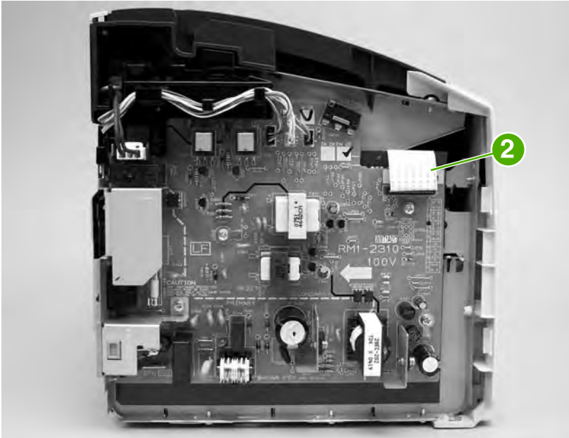
Figure 5-29 Remove the ECU assembly (2 of 6)
