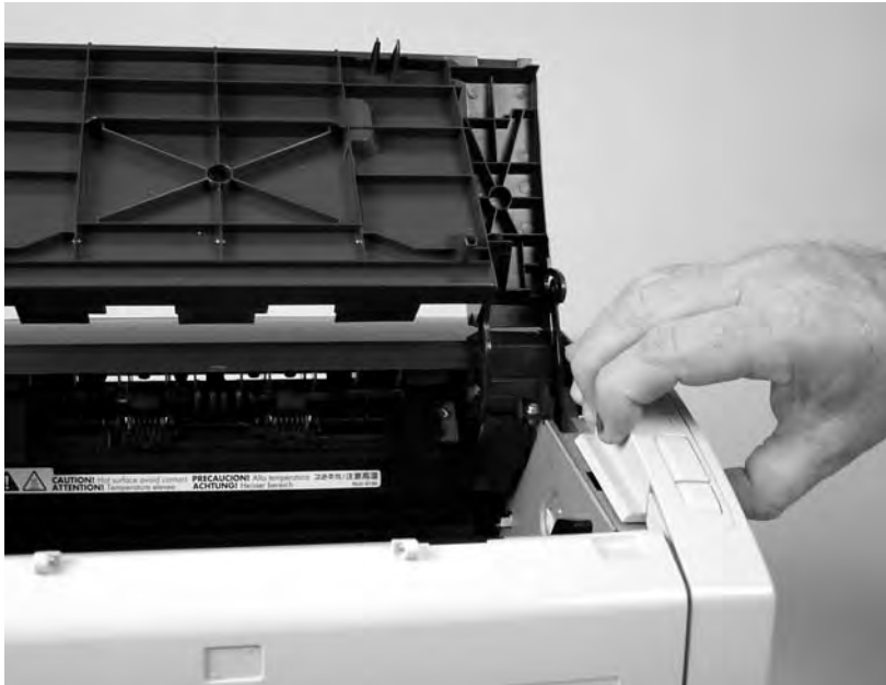
Figure 5-7 Remove the right-side cover (3 of 4)
