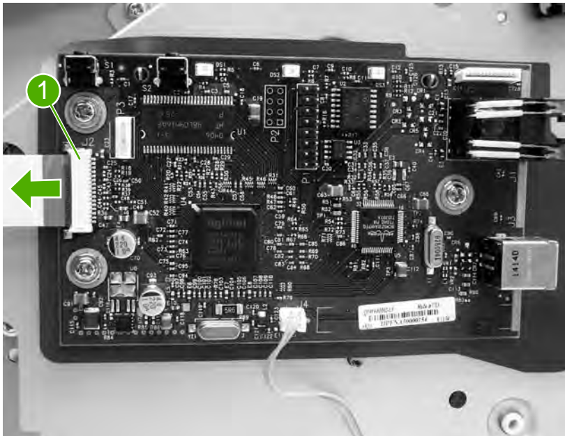
Figure 5-28 Remove the ECU assembly (1 of 6)
