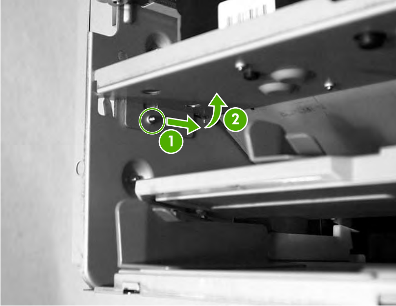
Figure 5-32 Remove the ECU assembly (4 of 6)
