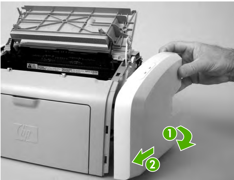
Figure 5-9 Remove the right-side cover (4 of 4; HP LJ 1020 printer shown)
