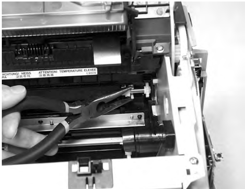
Figure 5-23 Remove the transfer roller (3 of 3)
