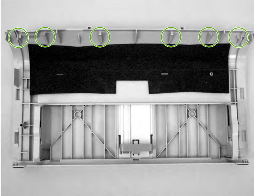
Figure 5-18 Remove the front cover (1 of 3)
