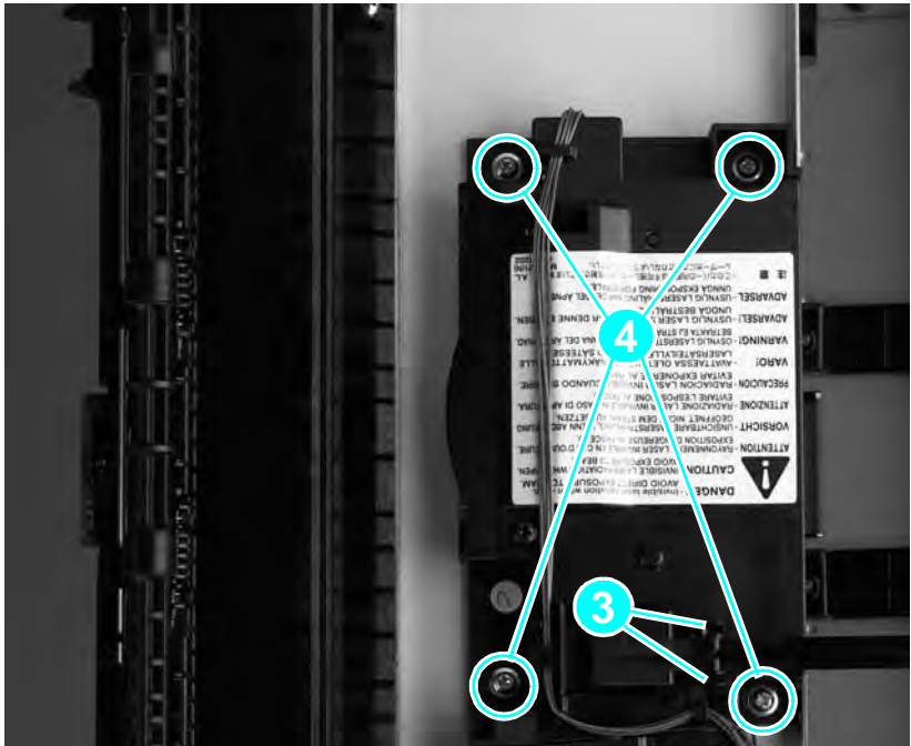
Figure 30. Remove the laser/scanner
