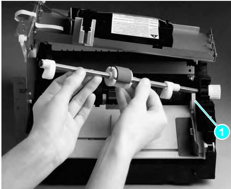
Figure 42. Remove the pickup roller assembly
