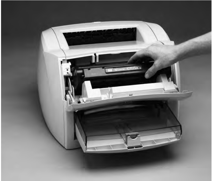
Figure 4. Remove the toner cartridge
