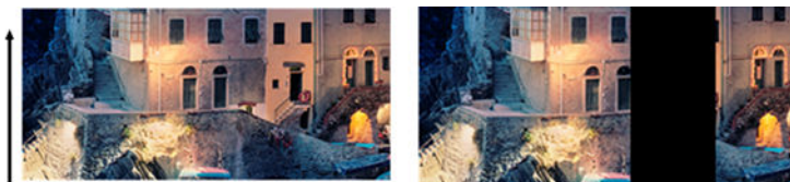
Original Scan affected by a CIS failing module
