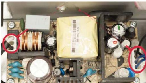
5. Remove the screws (x4, Torx 10), and lift the Power Supply out.
