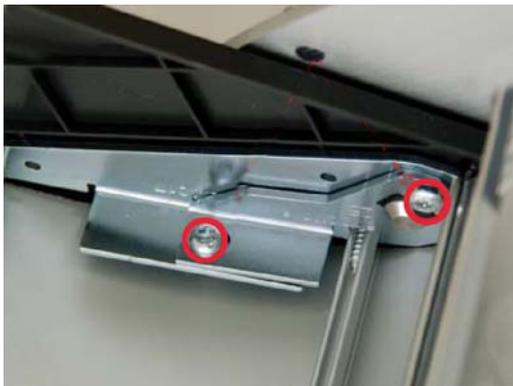
3. Remove the screws (x3, Torx 15) (A), and pull out the assembly (B).
