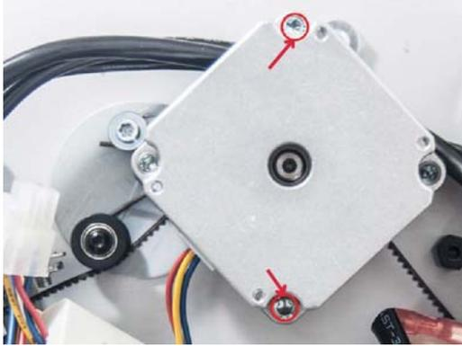
6. Remove the Stepper Motor Assembly.
