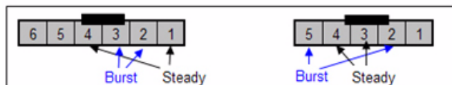
Resistance values as seen in P1 and P2 connectors on the Power Control PCA
