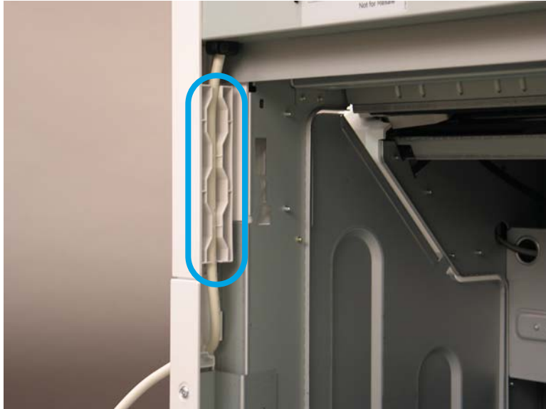
Figure 1-3197 Release the power cord
