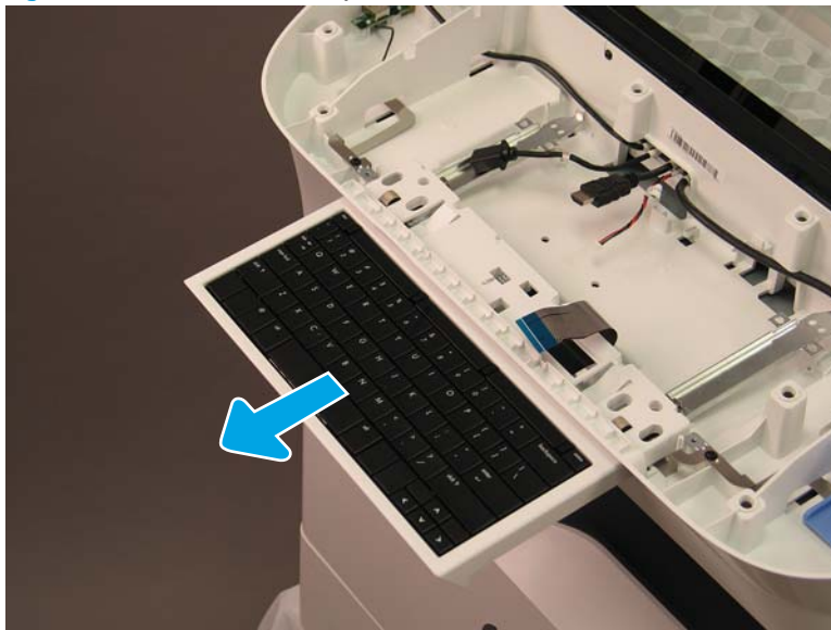
Figure 1-244 Remove the keyboard and rails
