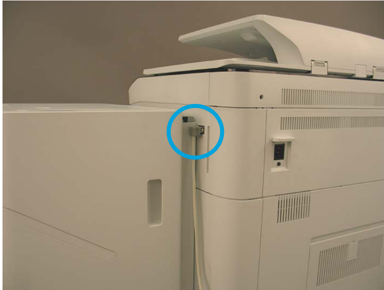
Figure 1-3201 Disconnect finisher connector
