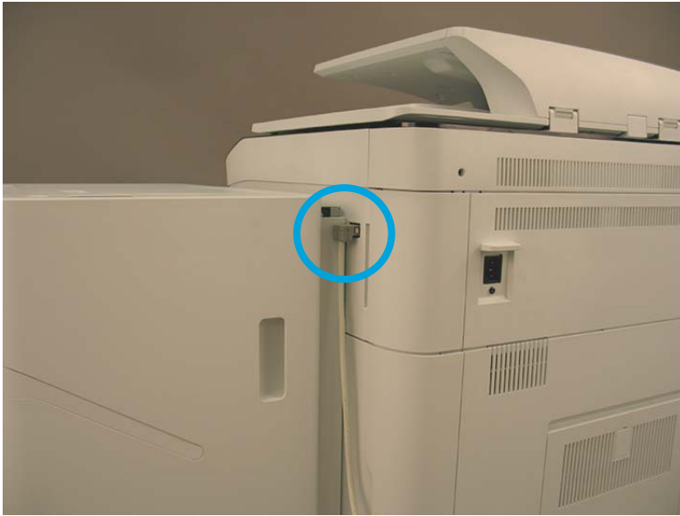
Figure 1-3724 Disconnect finisher connector
