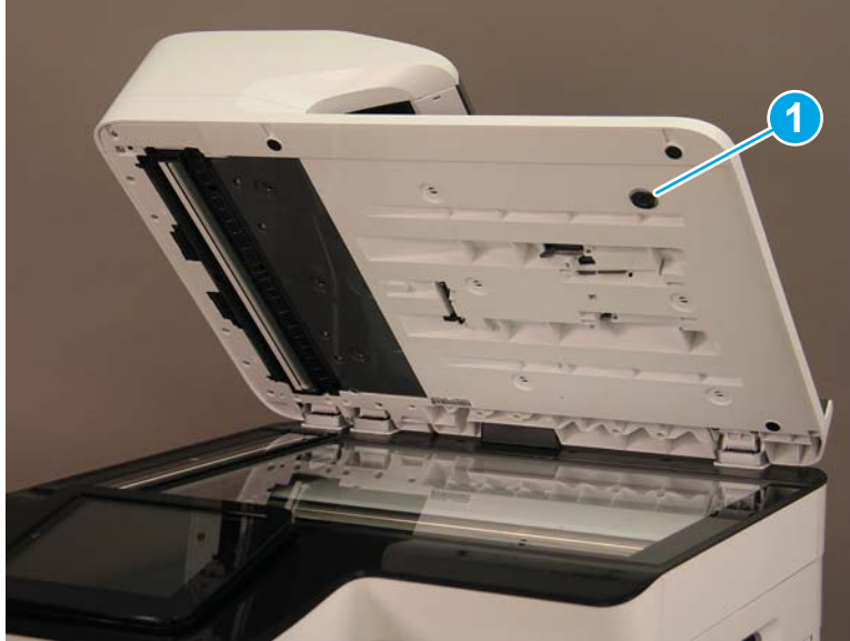
Figure 1-152 Check the document feeder left over reflector tabs
