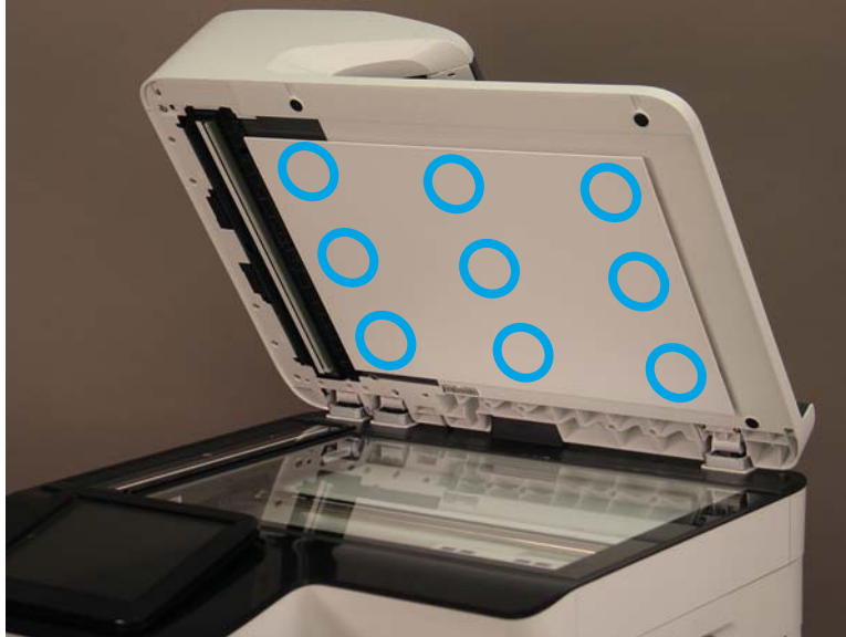
Figure 1-158 Check the reflector install
