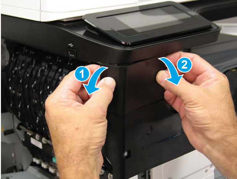
Figure 1-284 Release the front tower cover
