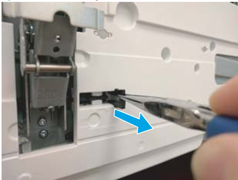
Figure 1-981 Pull the locking lever out
