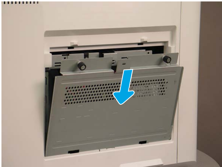
Figure 1-1345 Install the formatter cage cover
