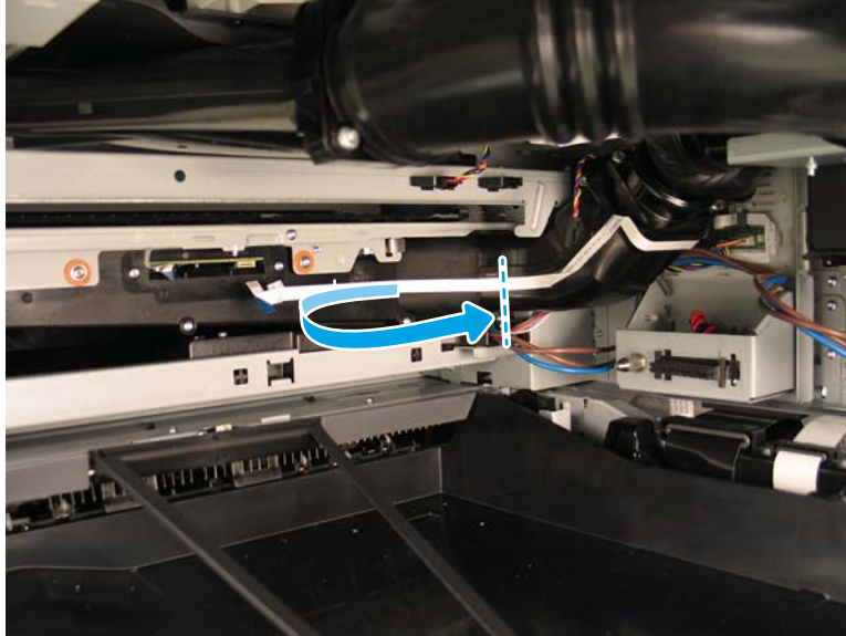
Figure 1-842 Release the FFC
