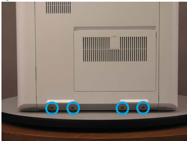
Figure 1-1654 Remove four screws
