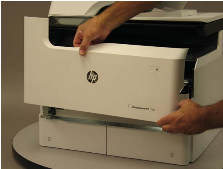
Figure 1-2350 Remove the cartridge door
