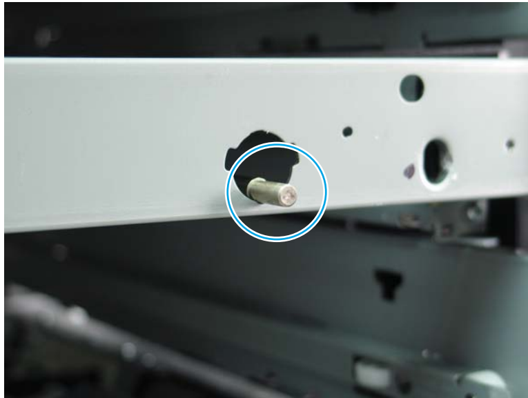
Figure 1-2547 Correct shaft install
