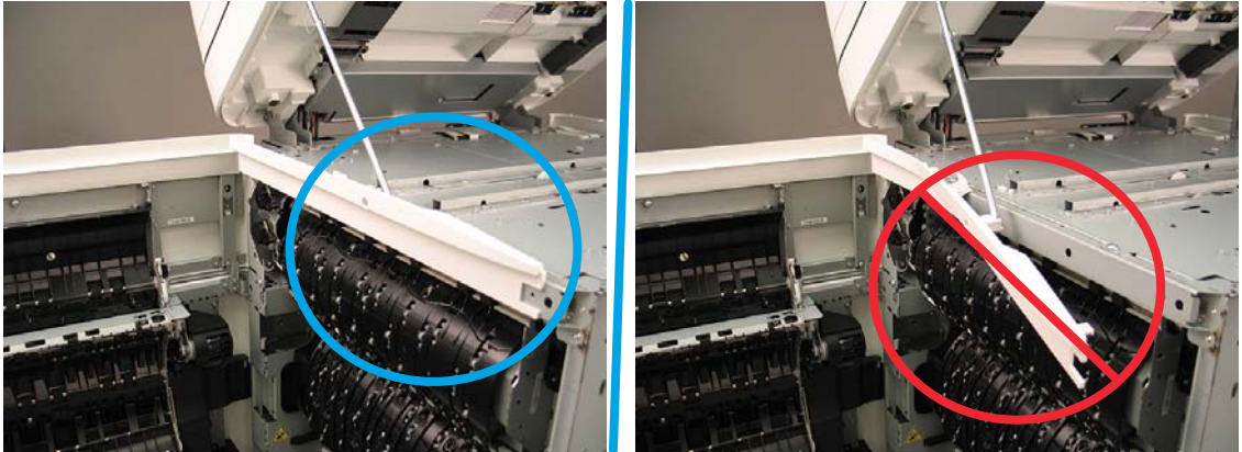
Figure 1-2770 Do not use the left-side cover as a hand hold
