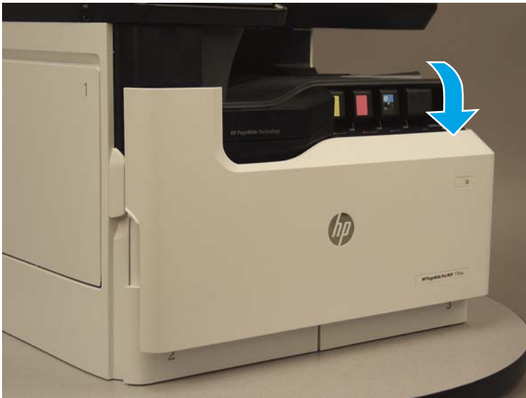
Figure 1-1124 Open the cartridge door
