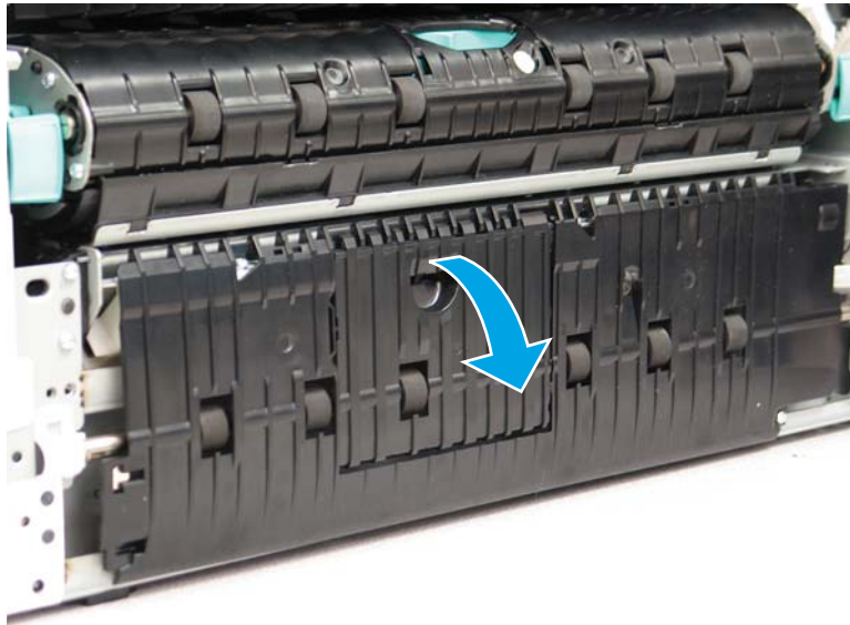
Figure 1-122 Open the separation roller door (A3 Tray 2 or A4 tandem Tray 3)
