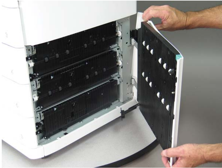
Figure 1-2495 Flex the top inner corner right door
