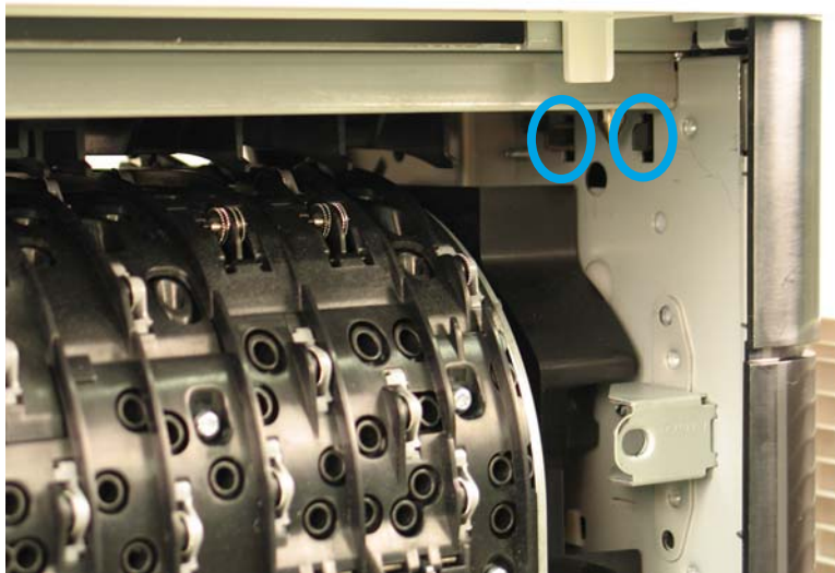
Figure 1-1734 Release two tabs
