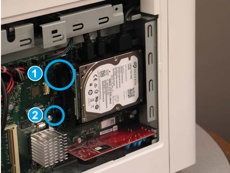
Figure 1-50 Check the HDD connector
