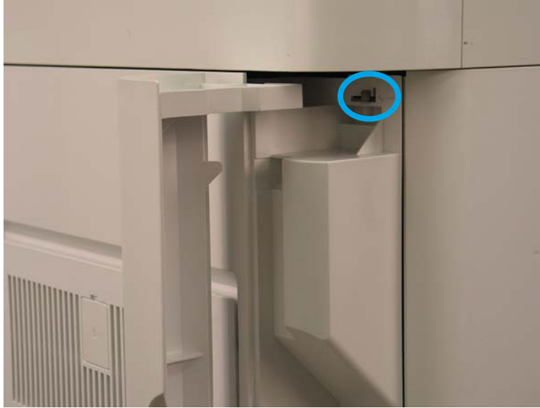
Figure 1-425 Release the latches
