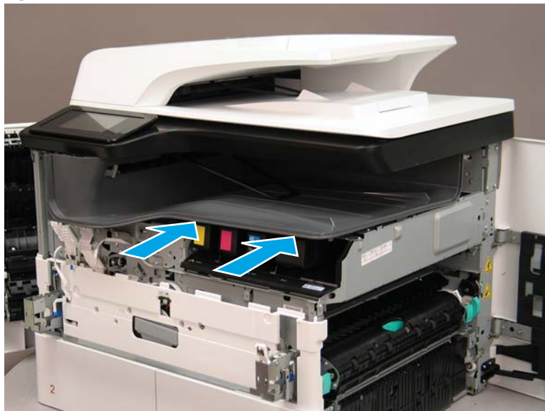
Figure 1-2312 Install the output bin
