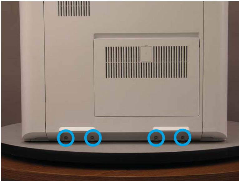
Figure 1-1458 Remove four screws
