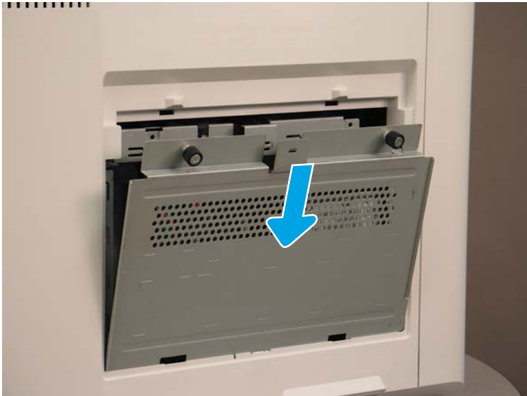
Figure 1-51 Install the formatter cage cover
