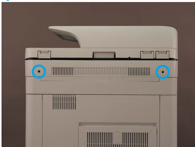
Figure 1-400 Remove two screws
