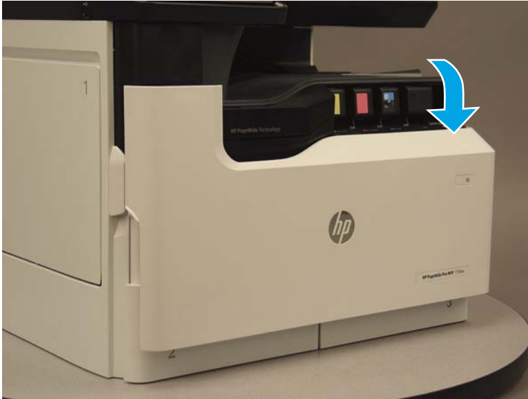
Figure 1-267 Open the cartridge door
