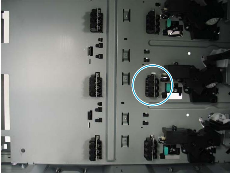
Figure 1-2531 Locate the sheet feeder width detect sensor
