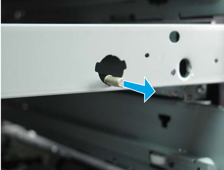
Figure 1-2544 Pull the shaft out
