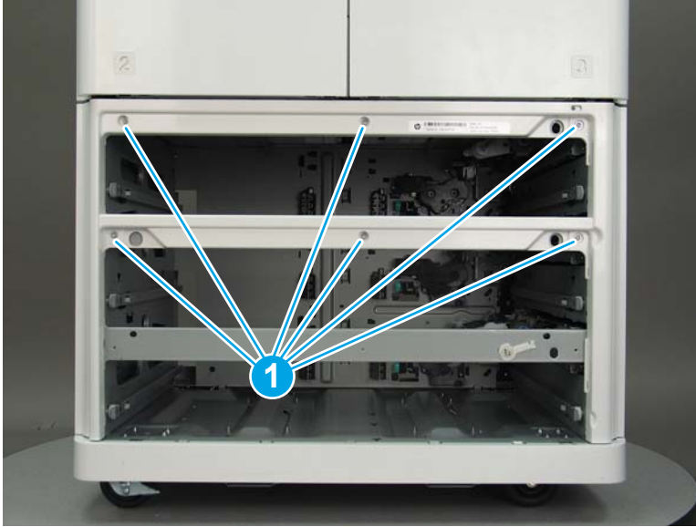
Figure 1-2555 Remove six screws
