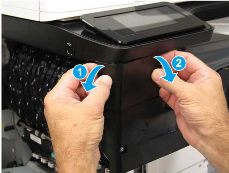
Figure 1-918 Release the front tower cover
