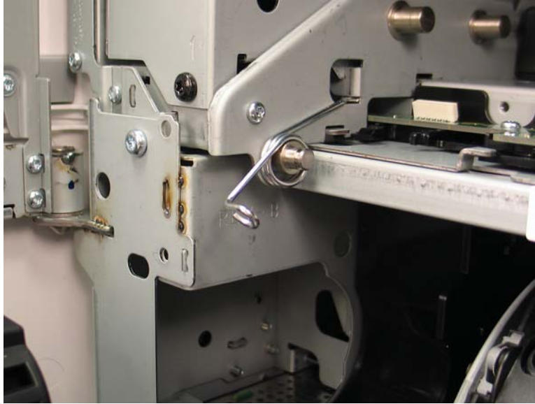
Figure 1-1182 Correctly install the spring
