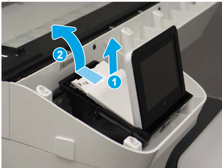
Figure 1-505 Release the control panel
