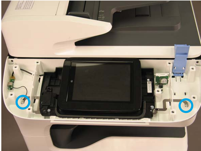
Figure 1-2873 Remove two screws
