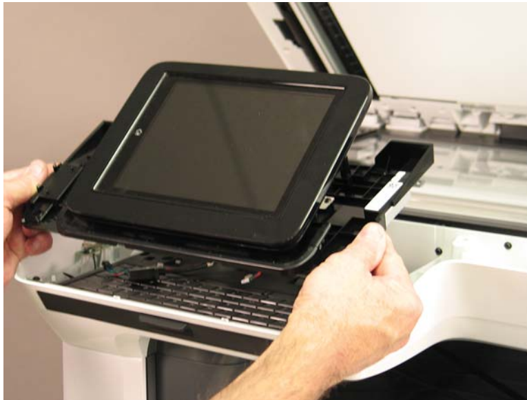
Figure 1-513 Remove the control panel
