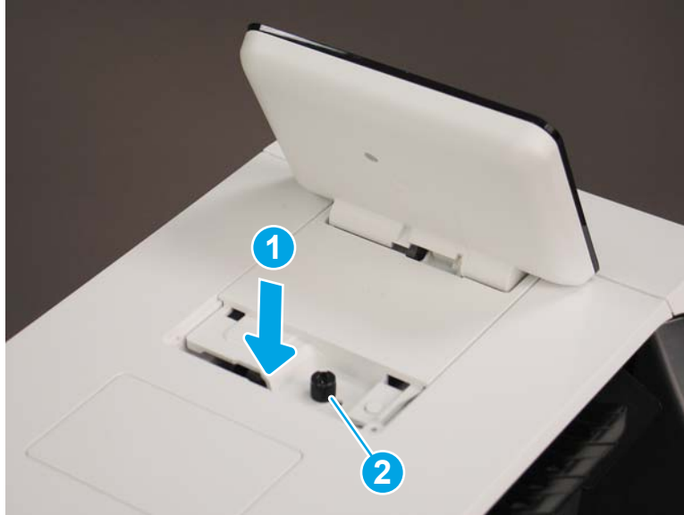
Figure 1-98 Install one thumbscrew (1 of 2) (765/E751/P752)
