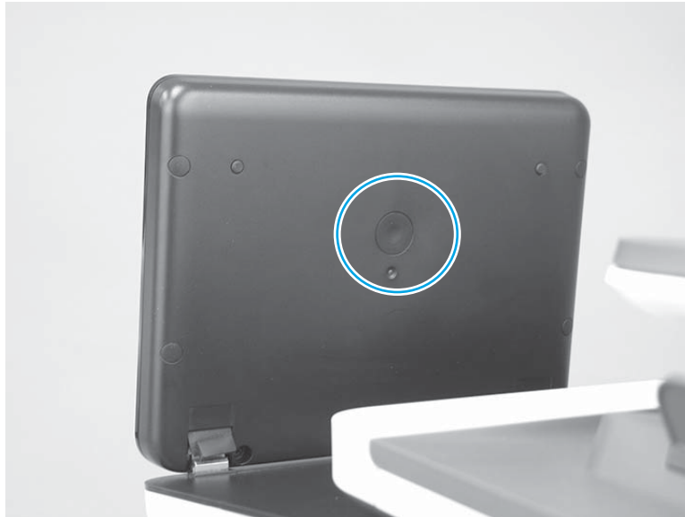
Figure 2-5 Press the diagnostics-access button (780/785 printers)
