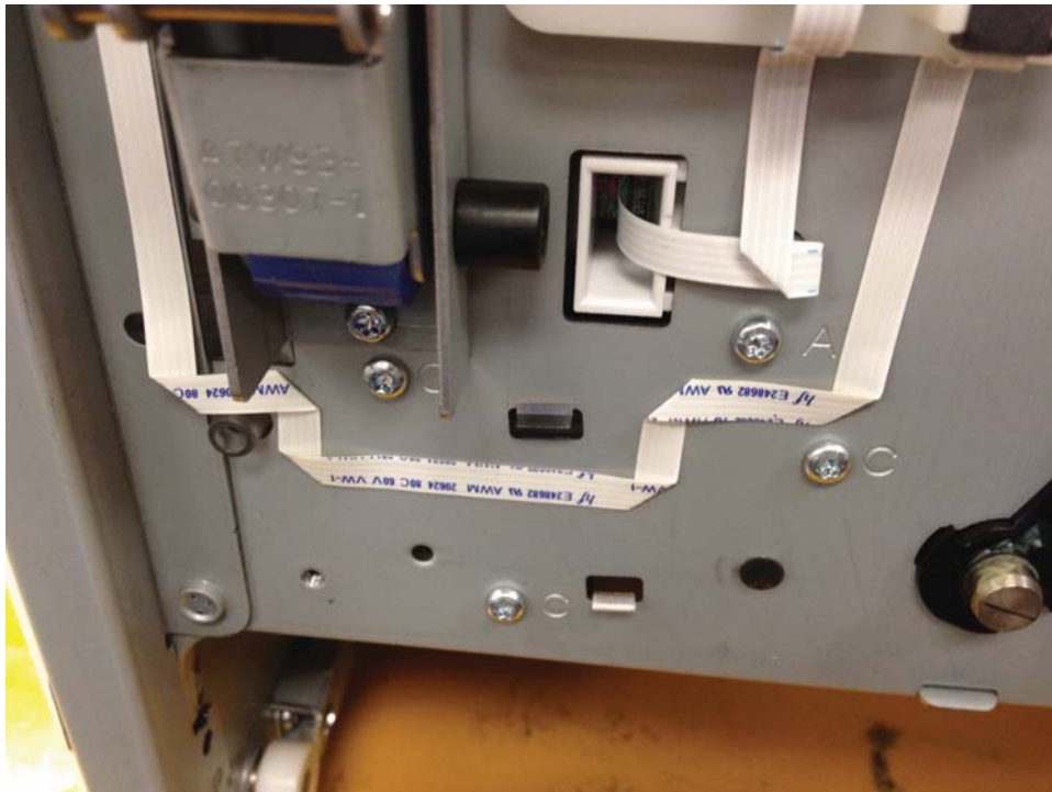
Figure 1-44 FFC double-sided tape retainer
