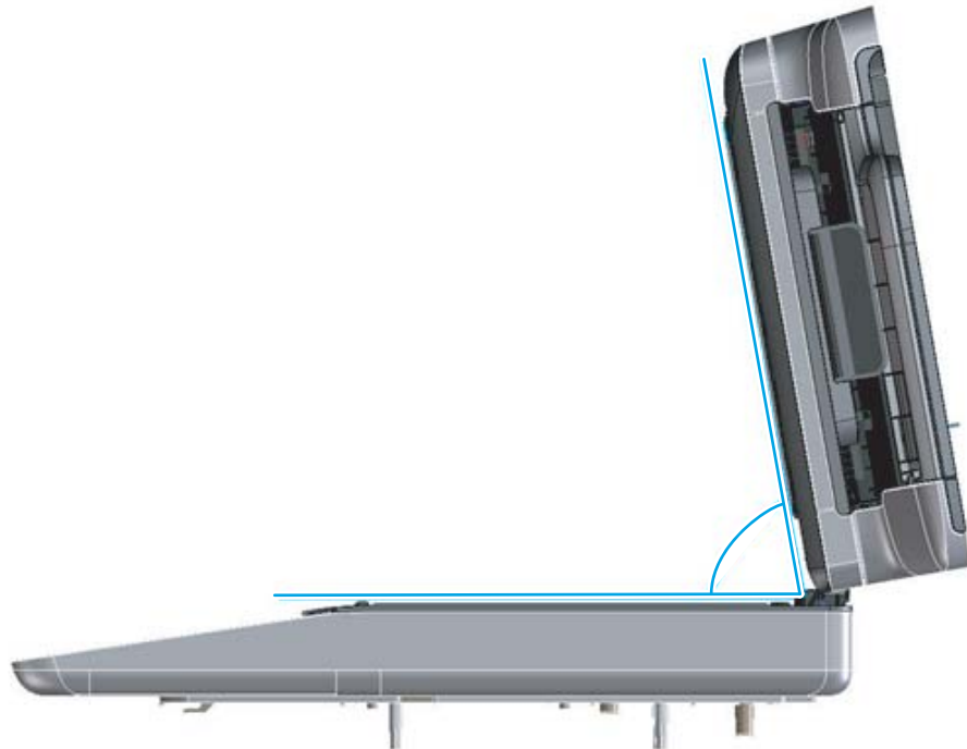
Figure 1-37 Document feeder open (60° to 80°)
