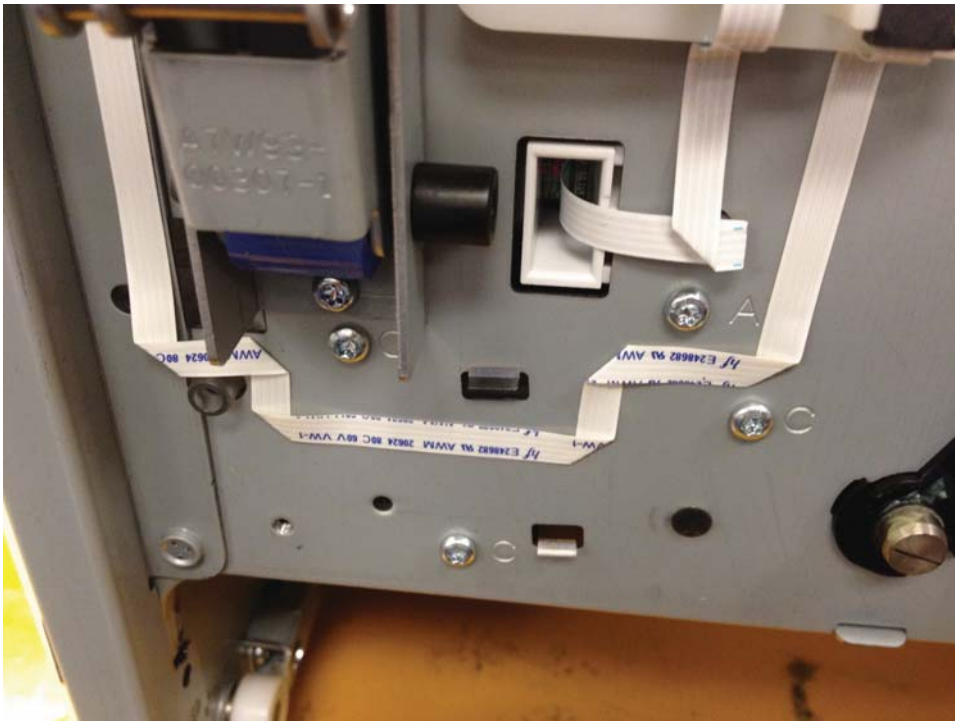
Figure 1-11 FFC double-sided tape retainer
