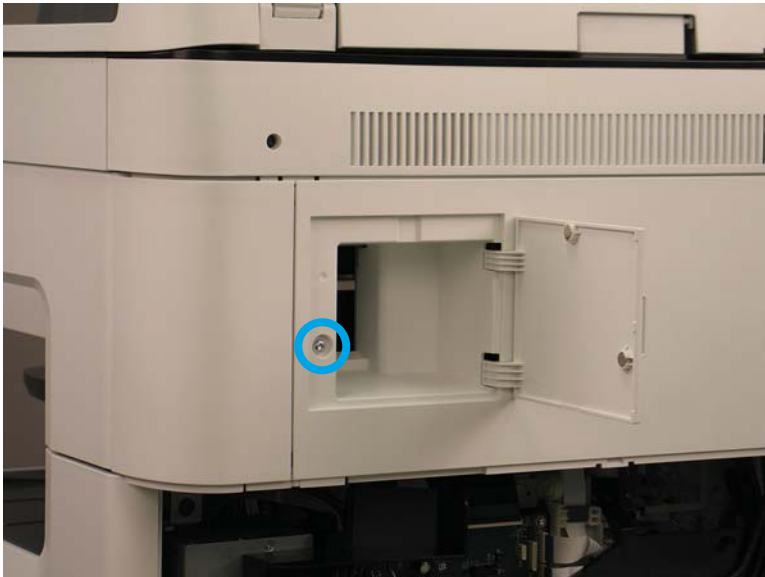
Figure 1-1978 Remove one screw
