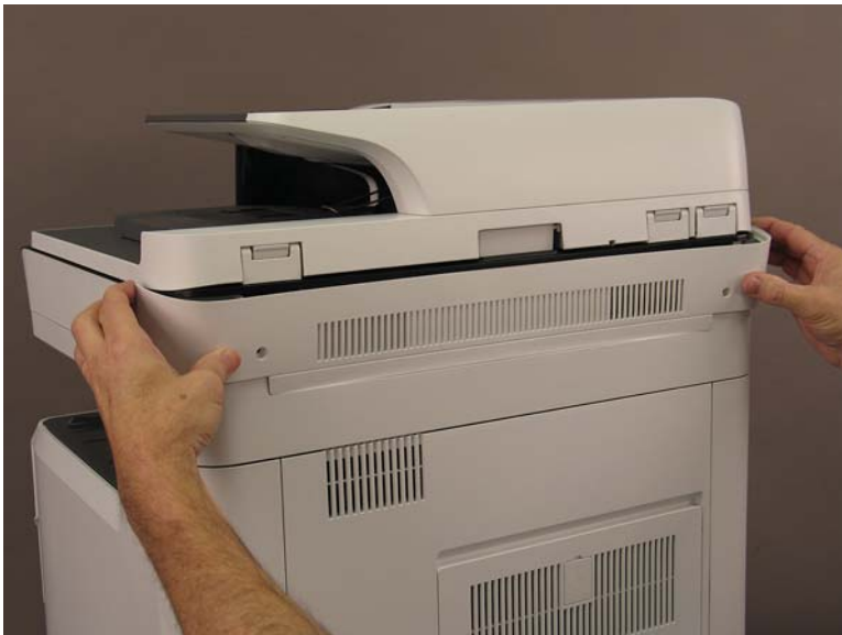
Figure 1-390 Release the cover
