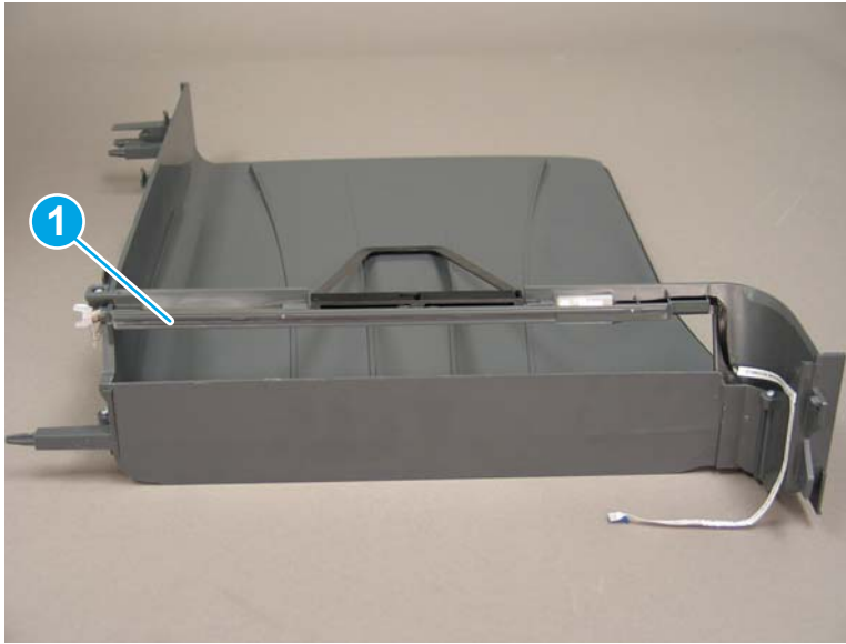
Figure 1-1555 Locate the mounting rail (output bin)
