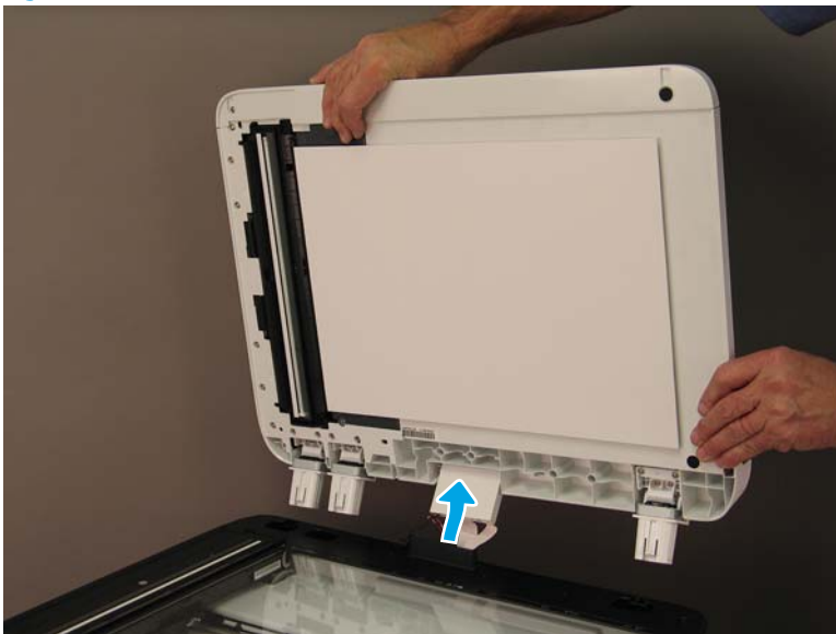
Figure 1-394 Remove the document feeder
