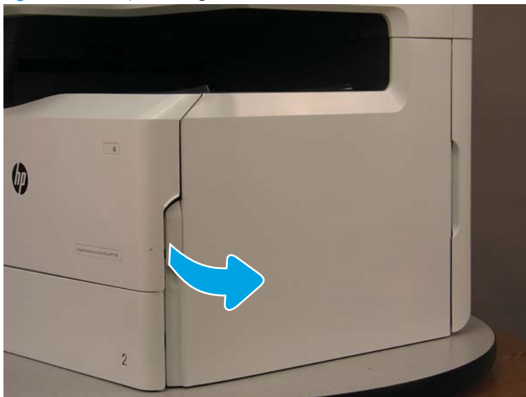
Figure 1-1312 Open the right door
