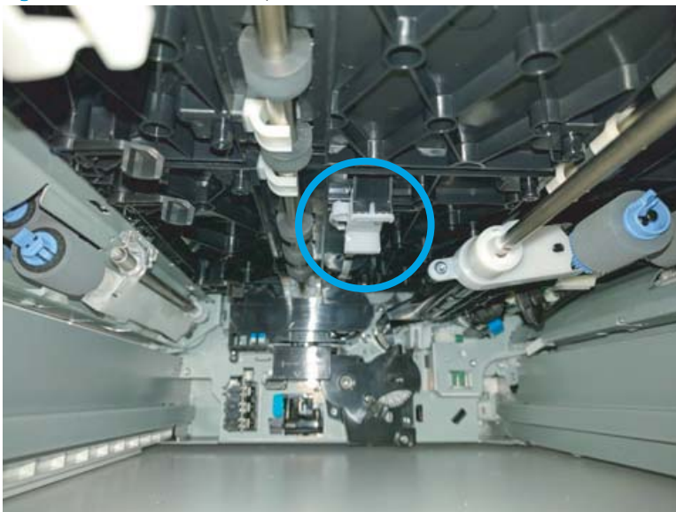
Figure 1-723 Locate the duplex exit REDI sensor and holder
