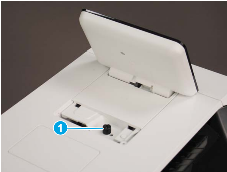
Figure 1-93 Remove one thumbscrew
