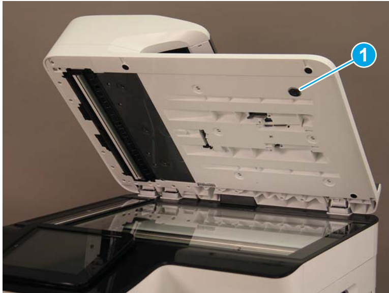
Figure 1-151 Check the document feeder left over reflector tabs
