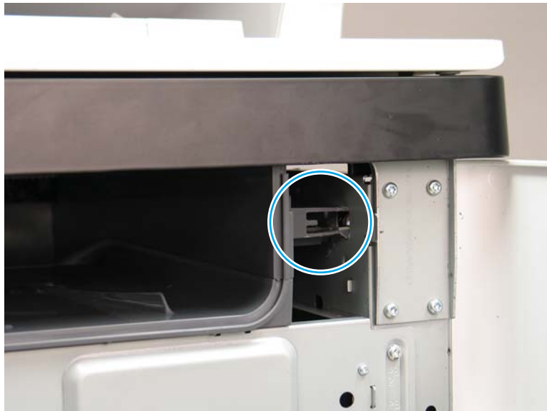
Figure 1-1391 Check the output bin installation
