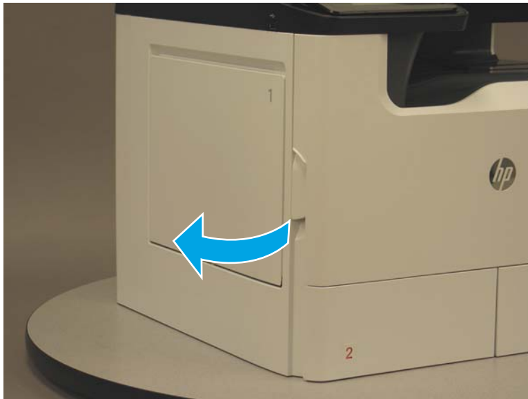
Figure 1-1256 Open the left door
