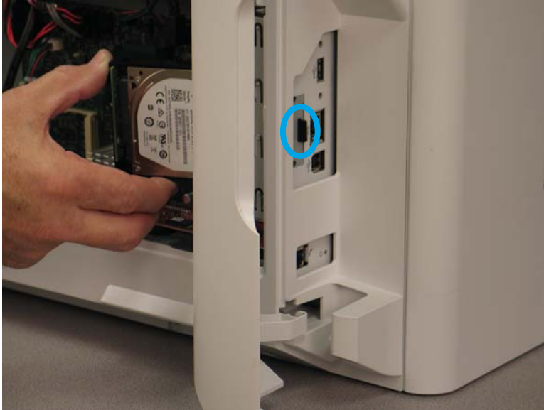
Figure 1-38 Locate the slot in the sheet metal
