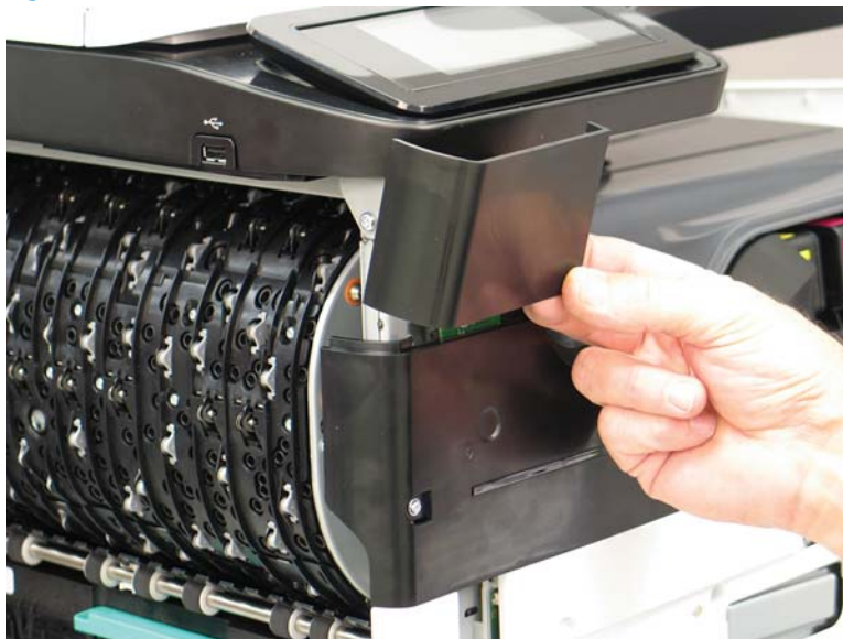
Figure 1-240 Remove the cover
