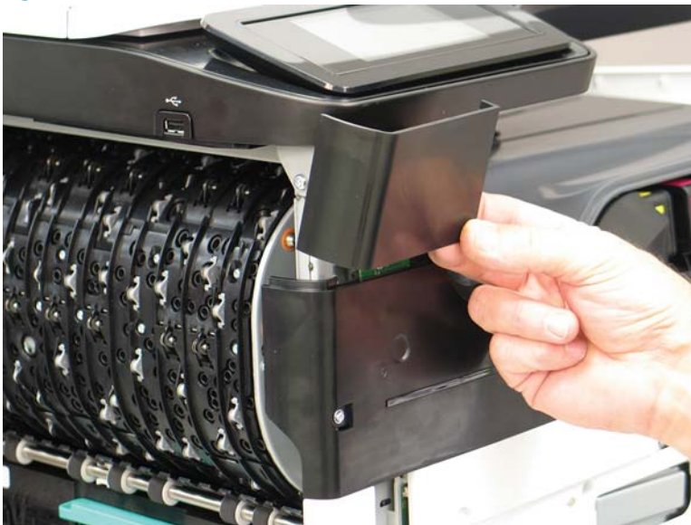
Figure 1-592 Remove the cover
