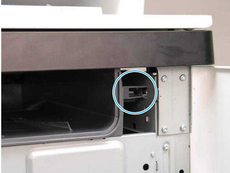
Figure 1-1438 Check the output bin installation
