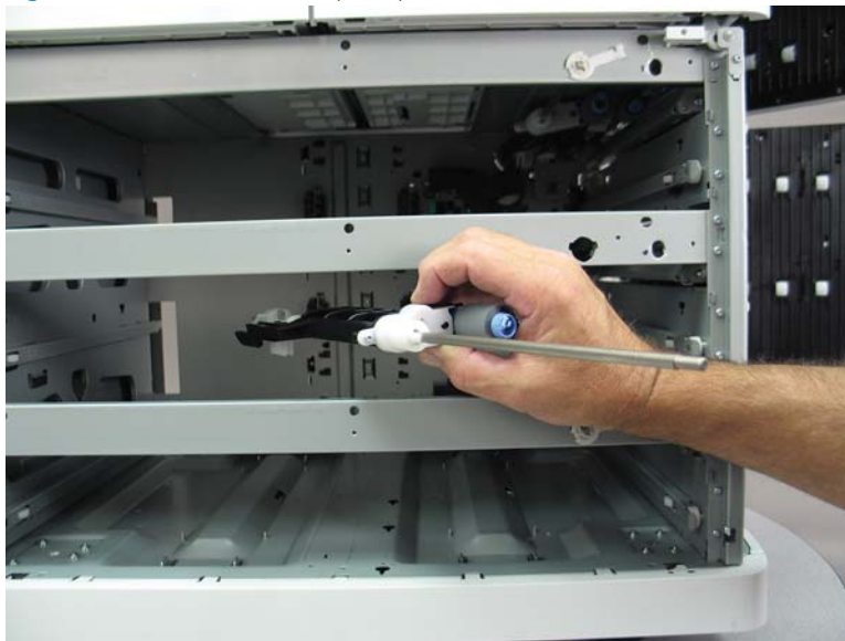
Figure 1-1800 Remove the pickup roller arm
