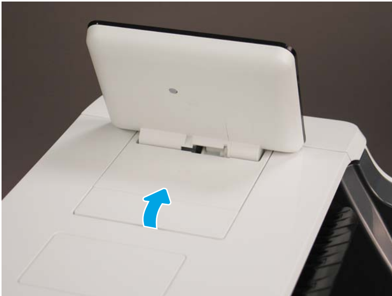
Figure 1-1190 Remove the cover
