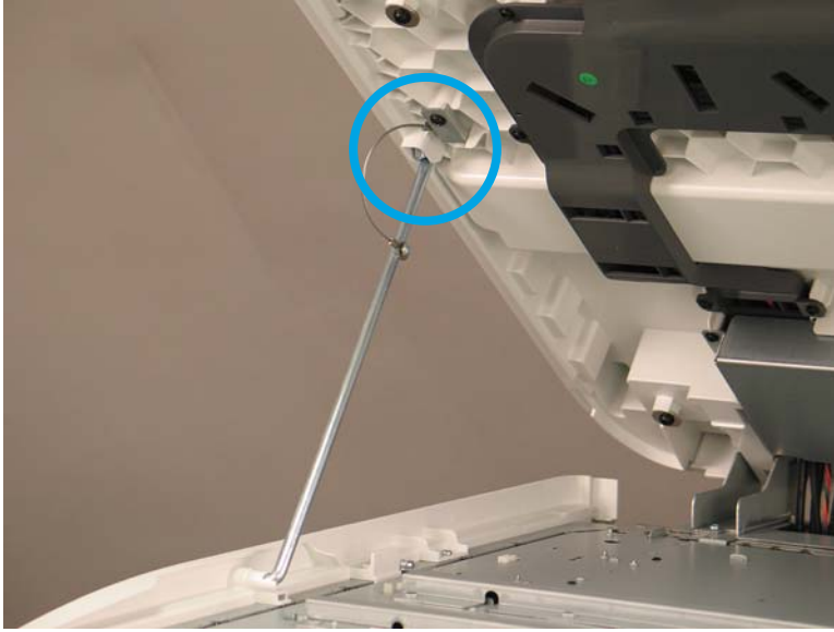
Figure 1-2361 Secure the ISA
