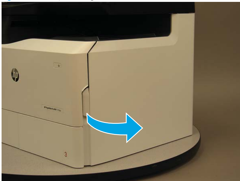
Figure 1-1588 Open the right door
