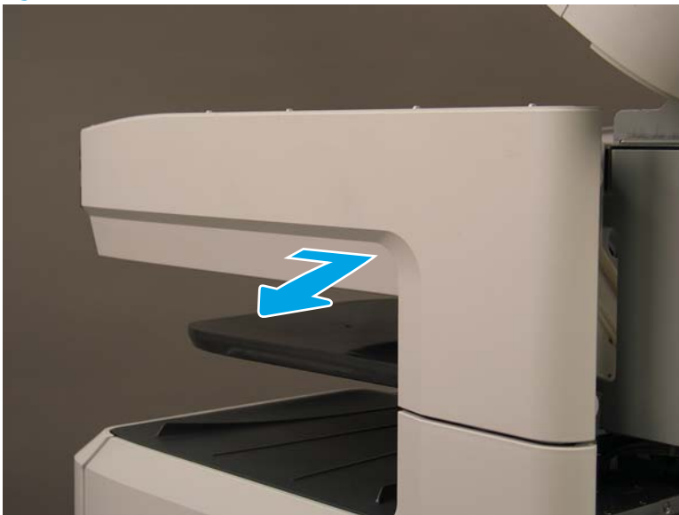
Figure 1-1174 Remove the cover
