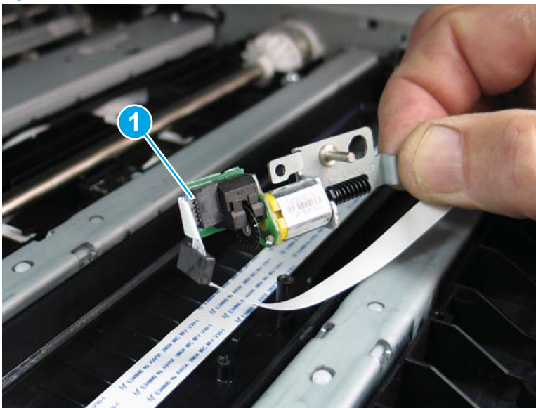
Figure 1-1640 Remove the image sensor motor
