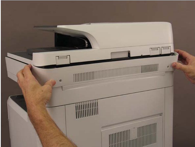
Figure 1-432 Release the cover
