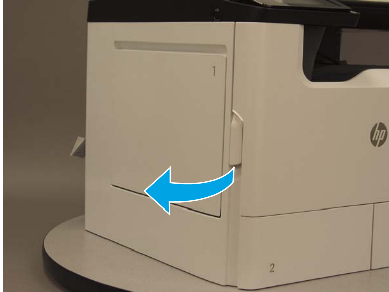
Figure 1-726 Open the left door
