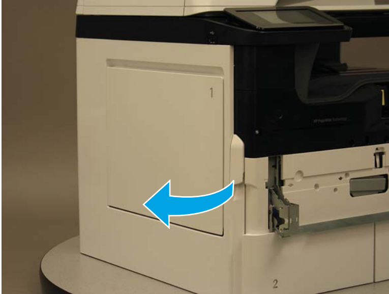
Figure 1-729 Open the left door
