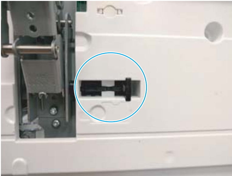
Figure 1-627 Locate the cover lock feature
