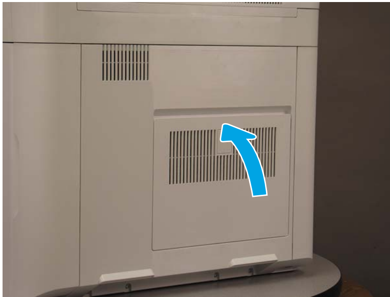
Figure 1-44 Install the formatter cover
