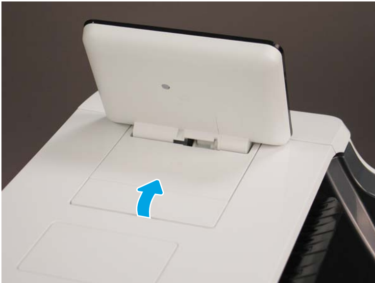
Figure 1-353 Remove the cover
