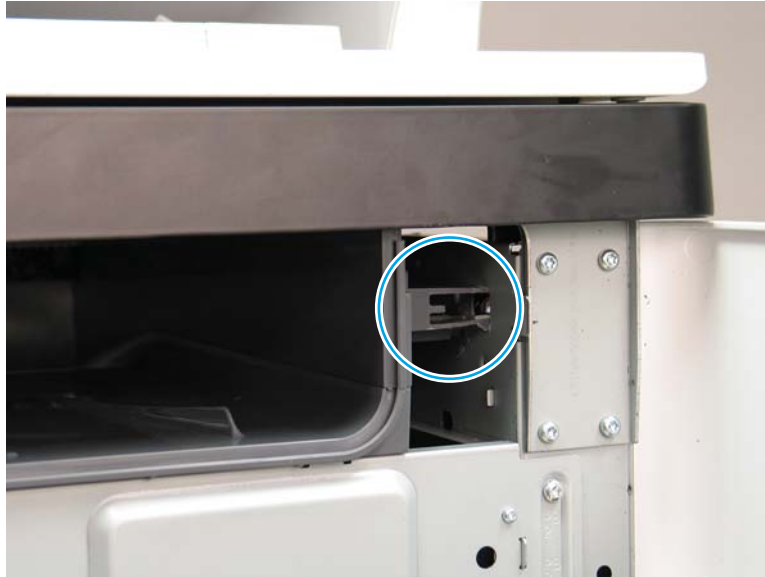
Figure 1-1337 Check the output bin installation
