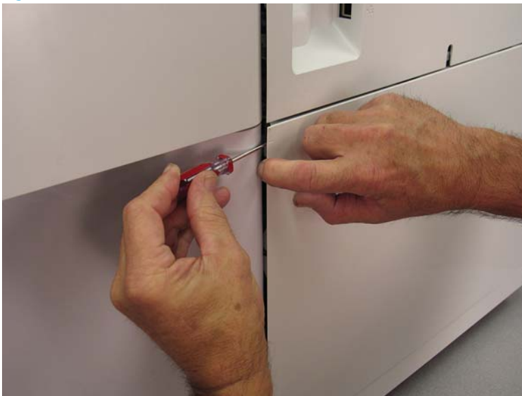
Figure 1-1805 Release the rear cover
