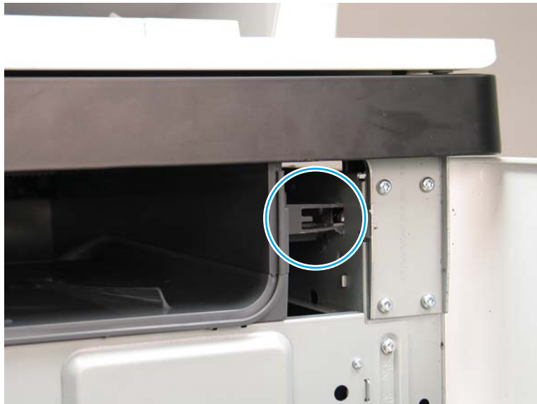
Figure 1-338 Check the output bin installation
