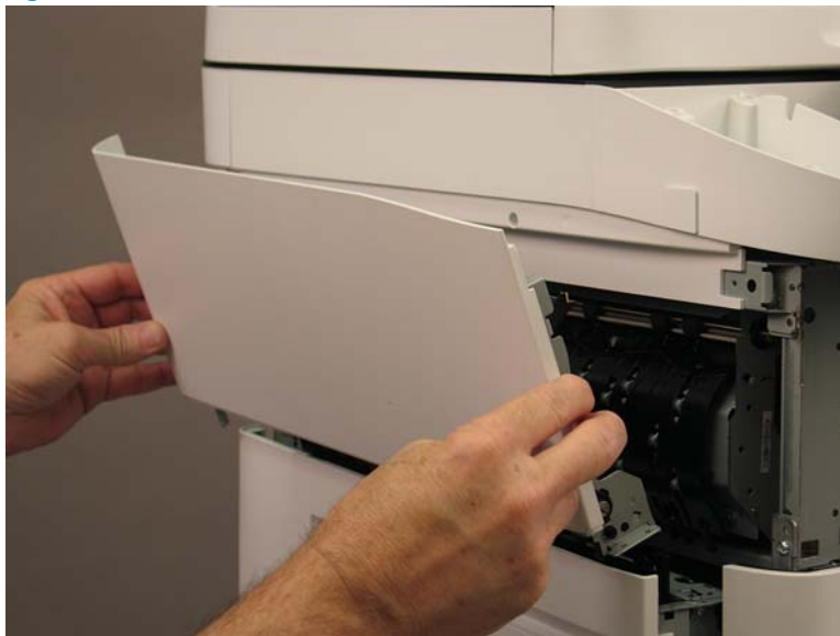
Figure 1-2047 Remove the cover
