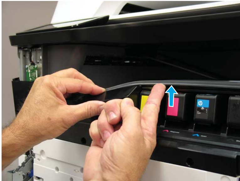
Figure 1-655 Release one tab
