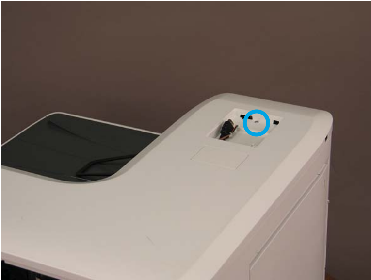
Figure 1-365 Remove one screw
