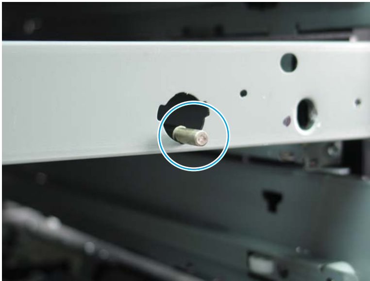
Figure 1-1802 Correct shaft install
