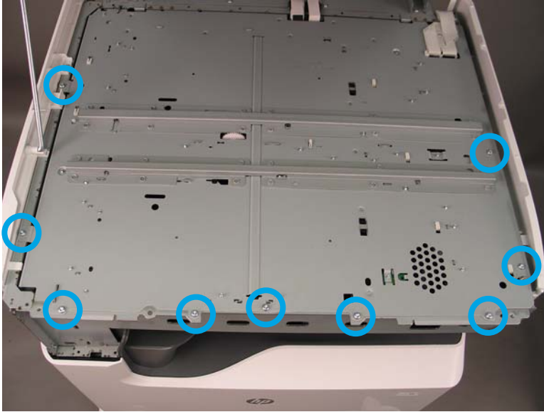
Figure 1-2326 Remove nine screws
