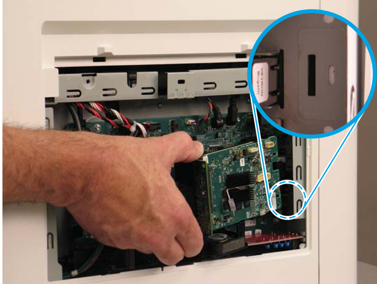
Figure 1-52 Locate the slot in the sheet metal
