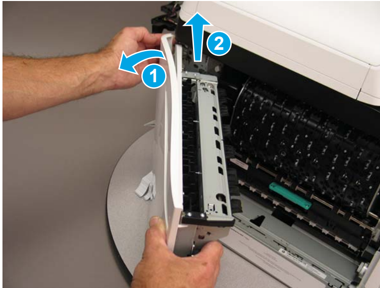
Figure 1-300 Remove the left door
