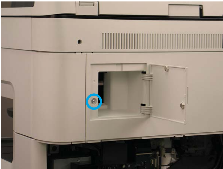
Figure 1-2061 Remove one screw
