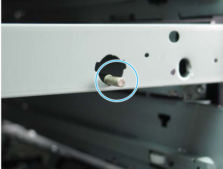
Figure 1-1816 Correct shaft install
