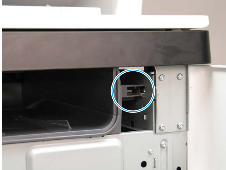
Figure 1-1613 Check the output bin installation
