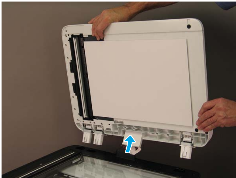
Figure 1-350 Remove the document feeder
