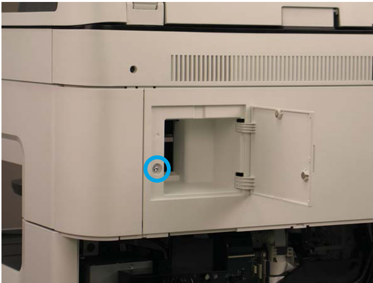
Figure 1-873 Remove one screw
