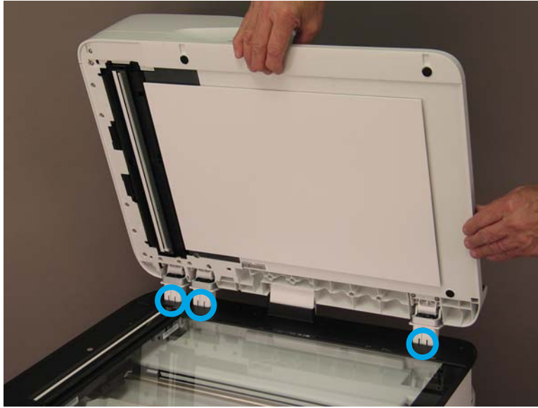
Figure 1-1113 Release the document feeder
