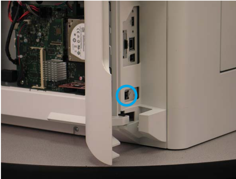
Figure 1-834 Locate the slot in the sheet metal
