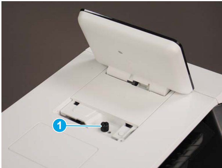
Figure 1-1191 Remove one thumbscrew
