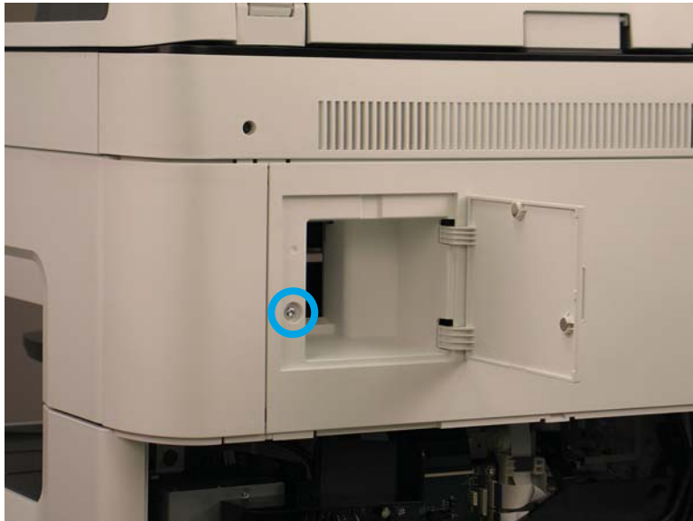
Figure 1-2015 Remove one screw
