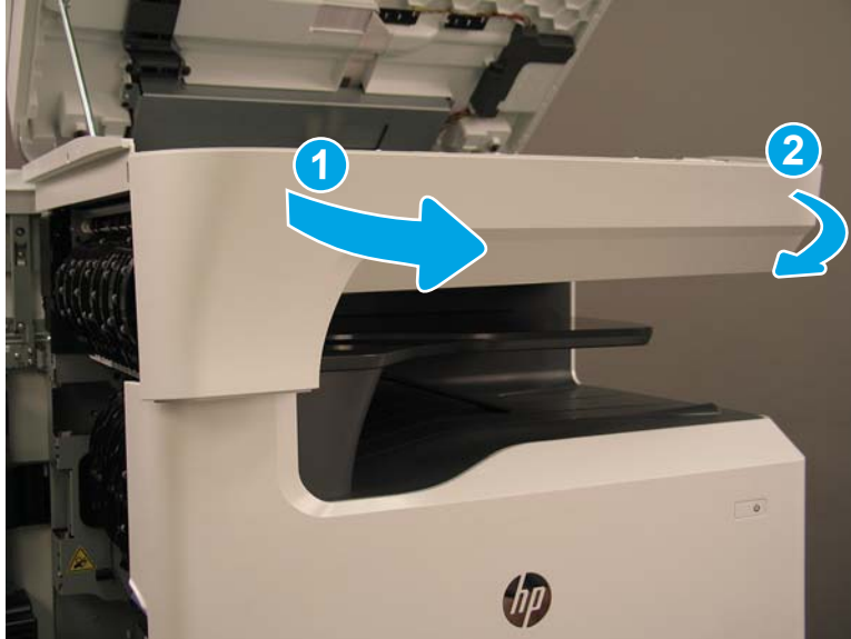
Figure 1-1167 Release the cover
