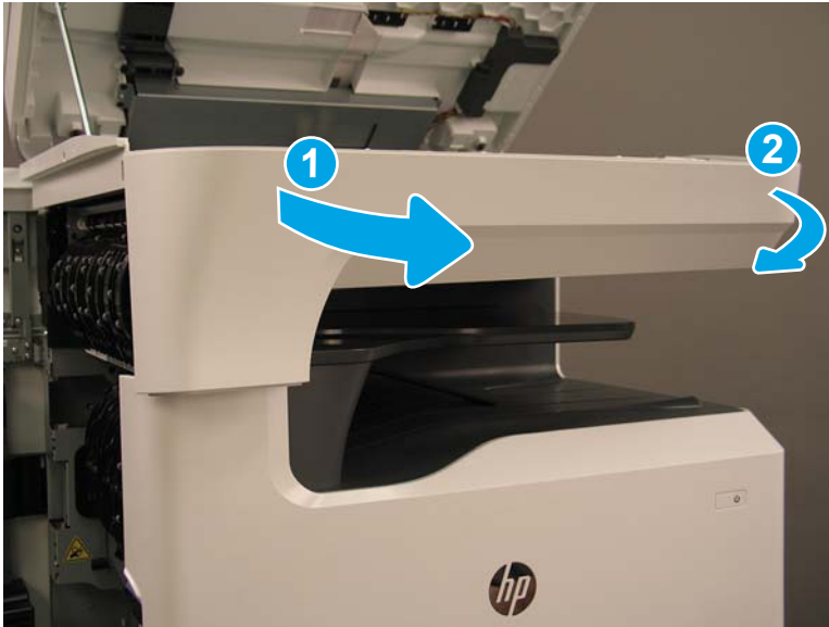
Figure 1-2365 Release the cover
