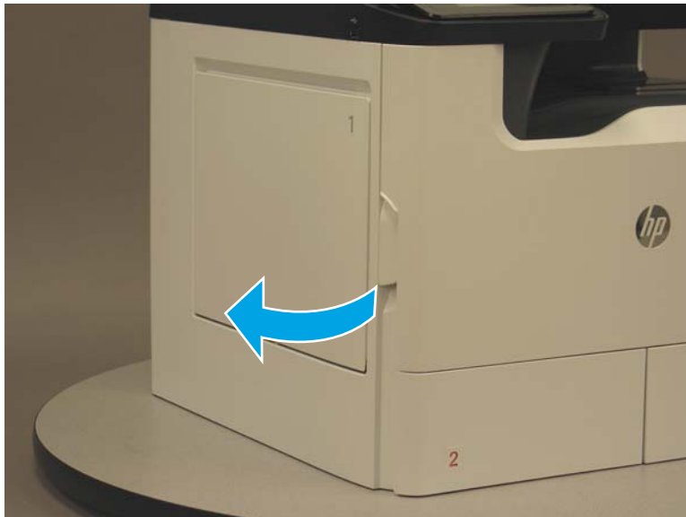
Figure 1-1209 Open the left door
