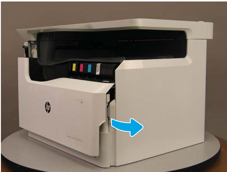
Figure 1-456 Open the door
