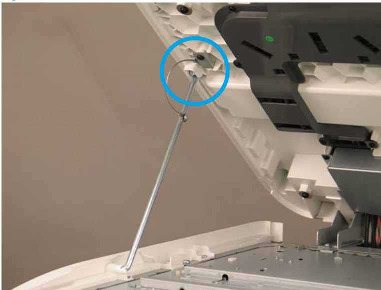
Figure 1-2181 Secure the ISA
