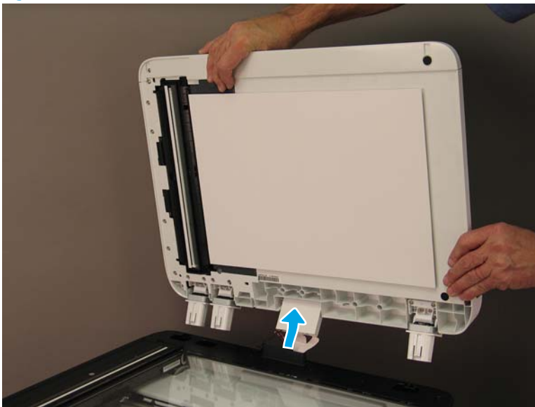
Figure 1-344 Remove the document feeder
