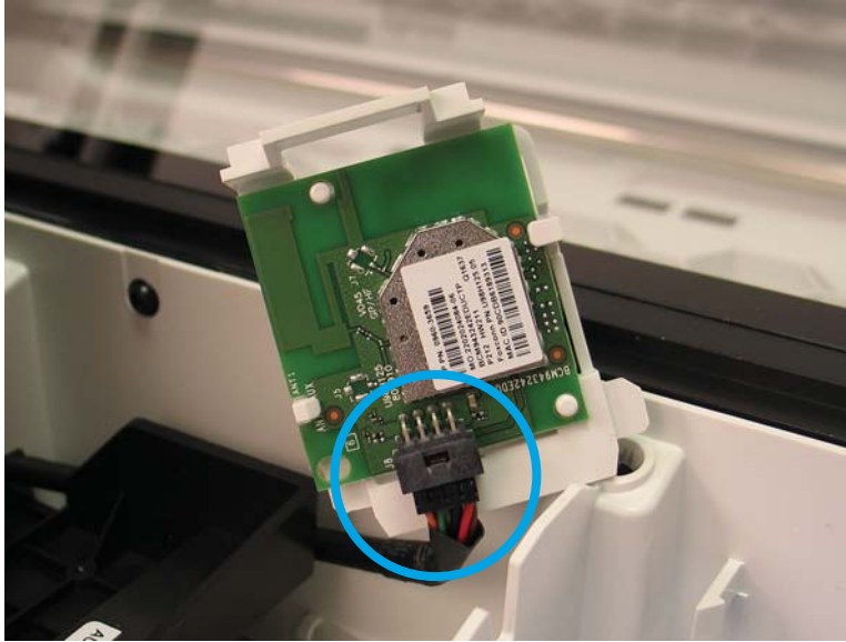
Figure 1-218 Remove the WiFi PCA
