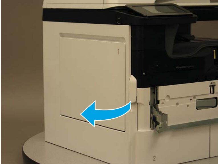
Figure 1-249 Open the left door
