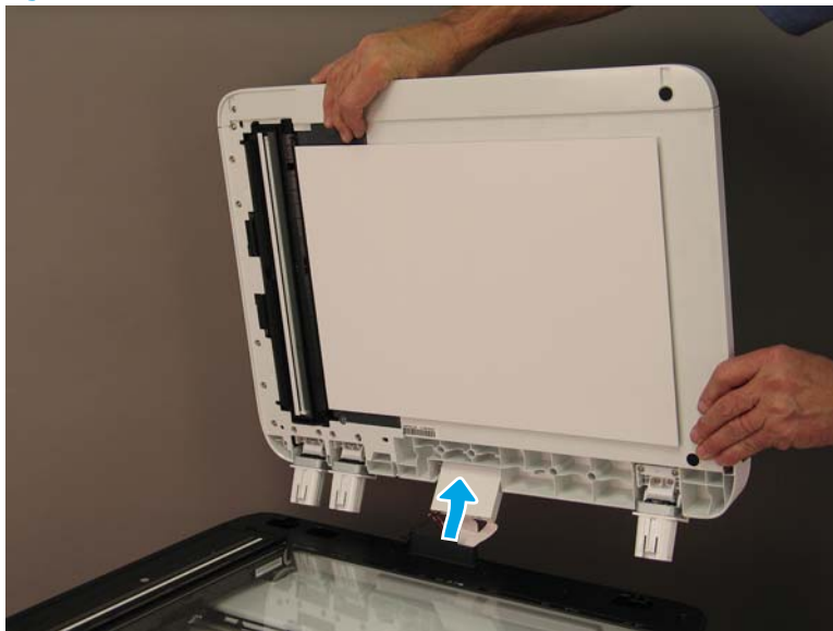
Figure 1-1114 Remove the document feeder
