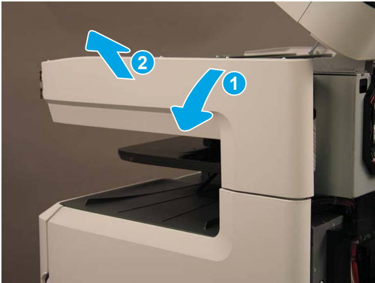
Figure 1-2033 Remove the cover
