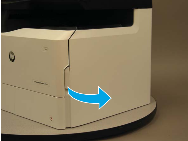
Figure 1-801 Open the right door
