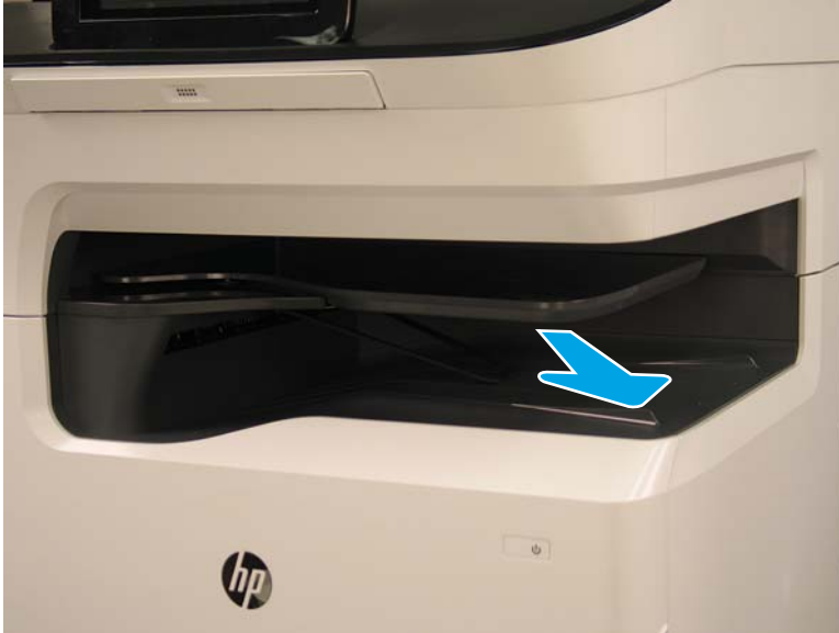
Figure 1-182 Pull the tray out
