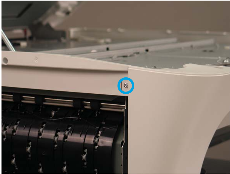
Figure 1-2026 Remove one screw
