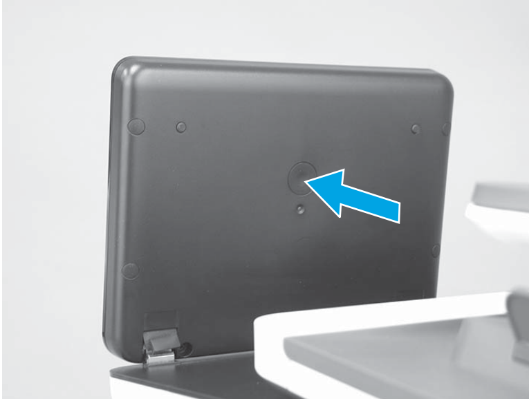
Figure 2-54 Press the diagnostics-access button (586)
