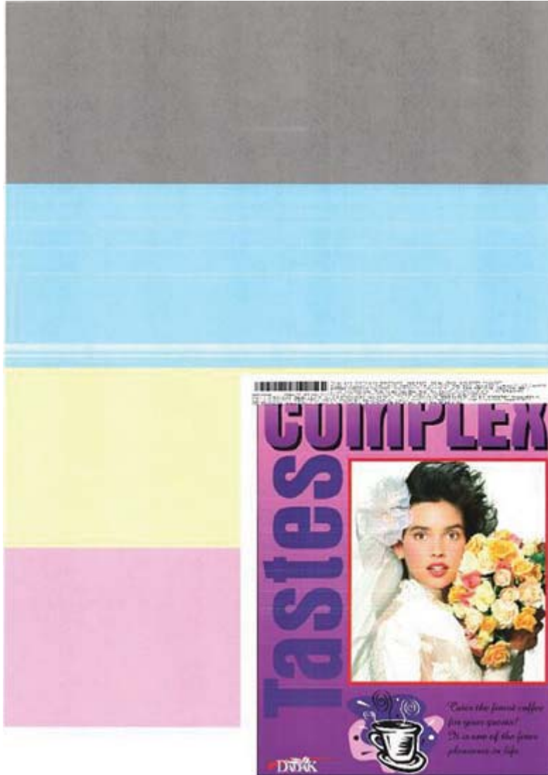
Figure 2-126 C-roller contamination streaks
