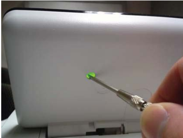
Figure 2-28 Press the diagnostics-access button (M856/E85055)
