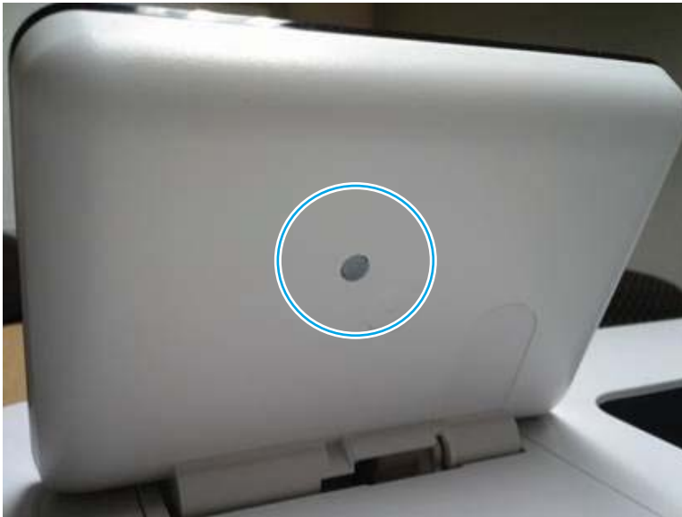
Figure 2-27 Diagnostic-tests access button (M856/E85055)
