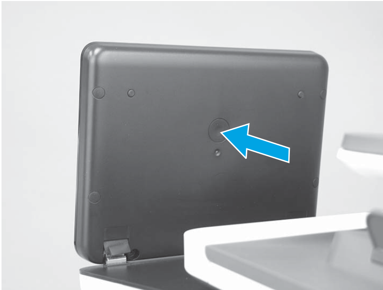
Figure 2-30 Press the diagnostics-access button (M776)
