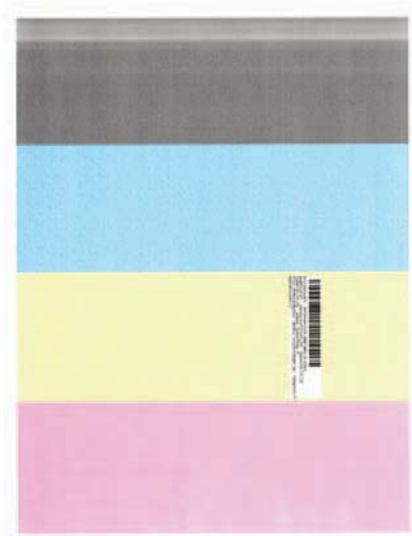
Figure 2-128 Laser path blockage streaks
