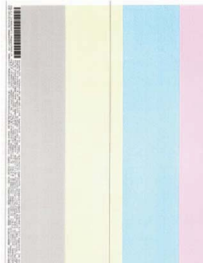
Figure 2-129 OPC grounding bands
