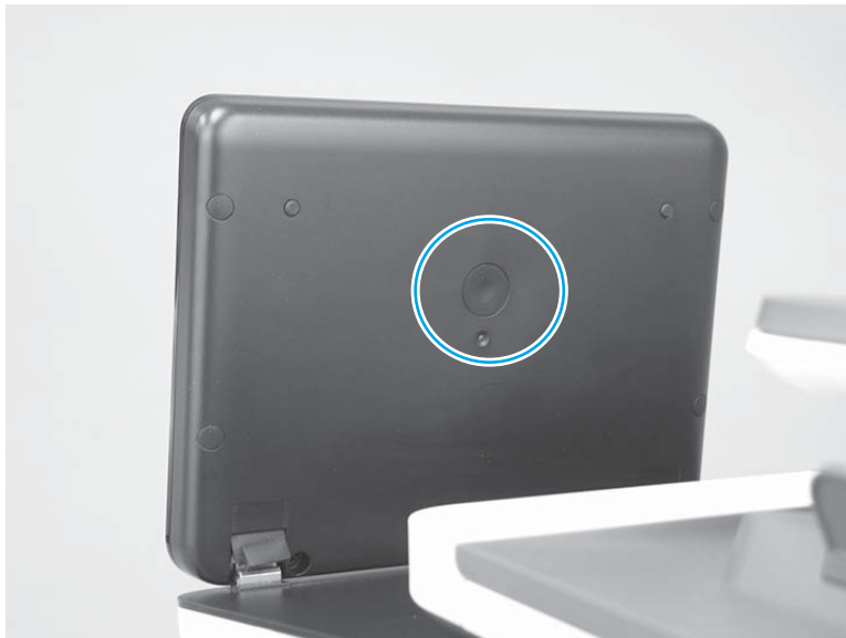
Figure 2-29 Diagnostic-tests access button (M776)
