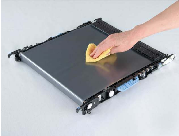
Figure 1-1203 Clean the ITB
