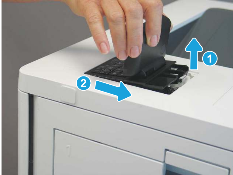
Figure 1-993 Slide the control panel back
