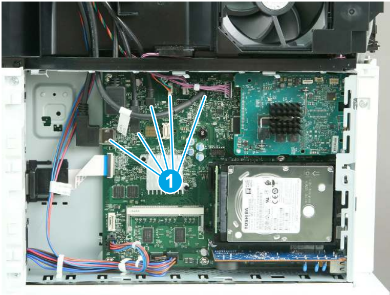
Figure 1-318 Disconnect five connectors
