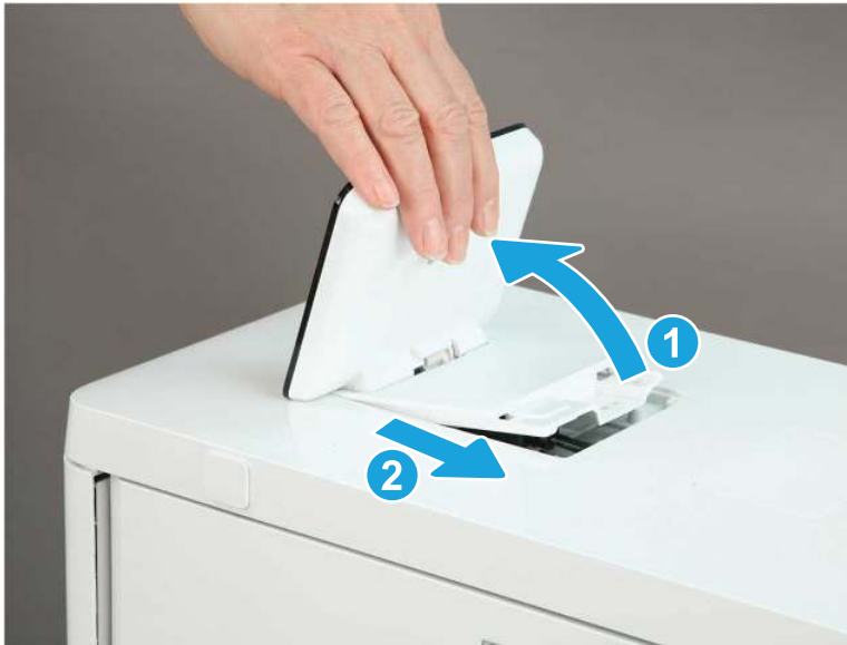
Figure 1-951 Slide the control panel back
