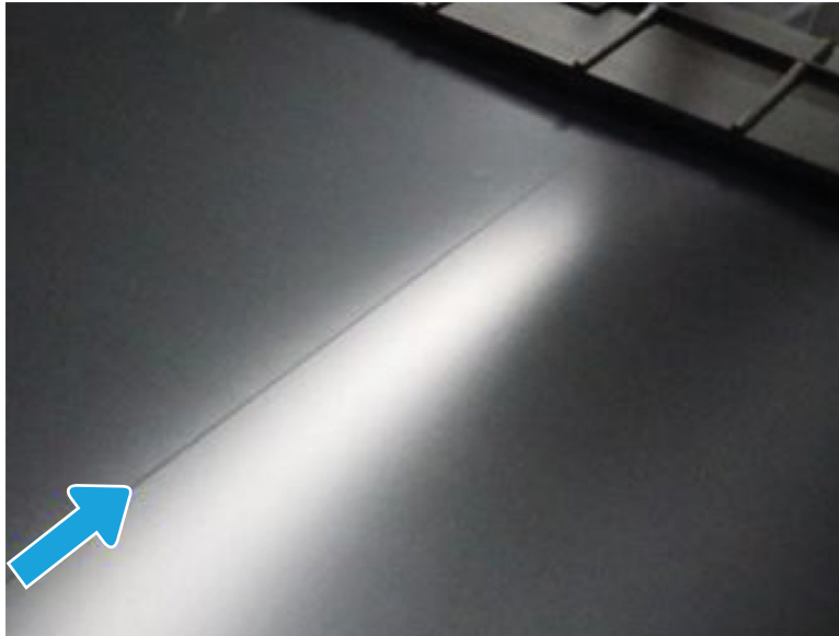
Figure 1-1197 Check for convex streak
