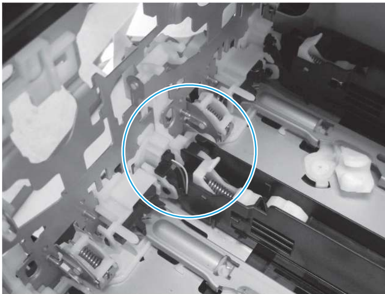
Figure 1-1084 Link arm correct installation (M751/E75245/M856/E85055/M776dn/M776z/M776zs)
