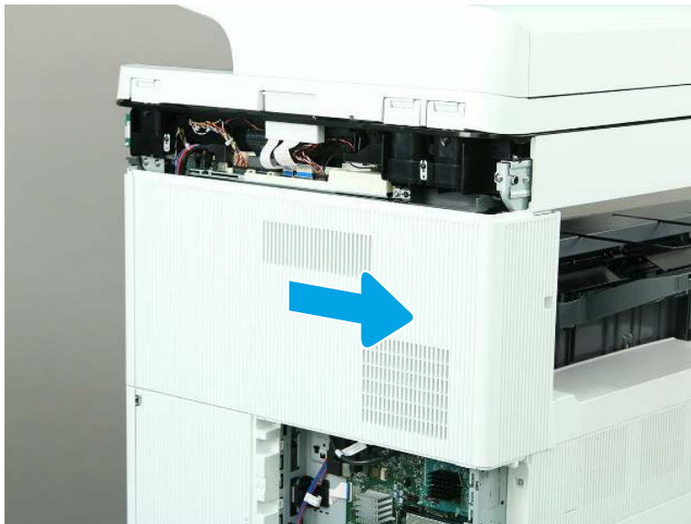
Figure 1-1263 Remove the rear upper and left rear upper cover
