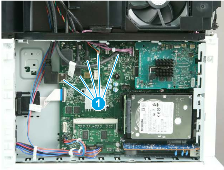
Figure 1-473 Disconnect five connectors
