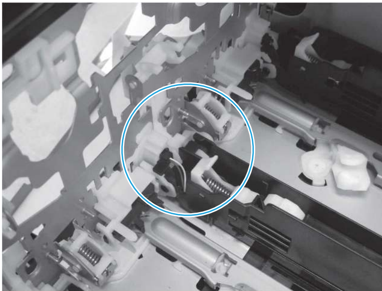
Figure 1-1016 Link arm correct installation (M751/E75245/M856/E85055/M776dn/M776z/M776zs)
