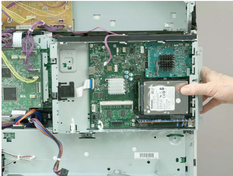
Figure 1-1251 Remove the formatter and case
