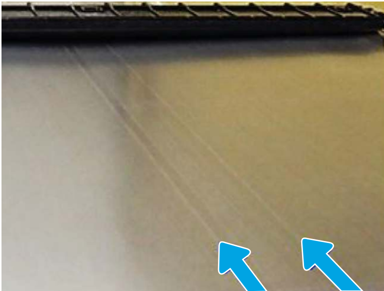
Figure 1-1204 Look for debris or toner streaks on the ITB
