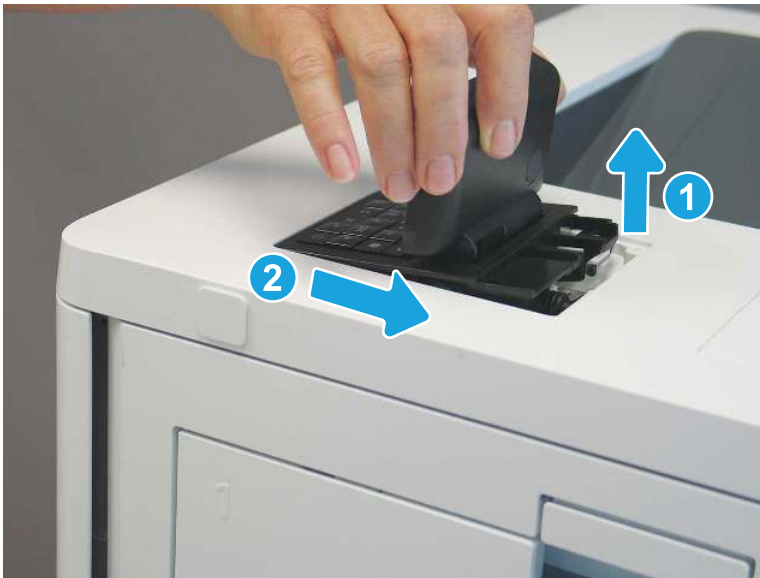
Figure 1-1902 Slide the control panel back
