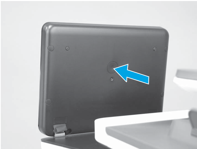
Figure 2-23 Press the diagnostics-access button
