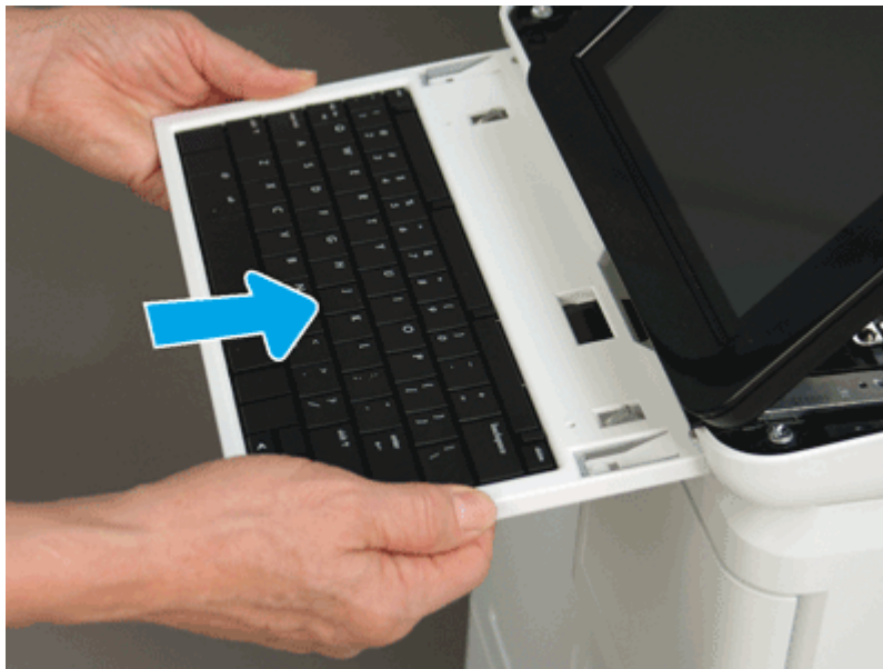
Figure 5-196 Slide the keyboard tray into the slot
