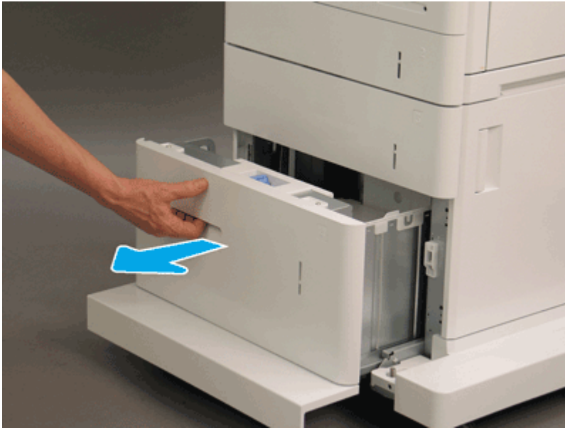
Figure 2-71 Open the high-capacity paper tray
