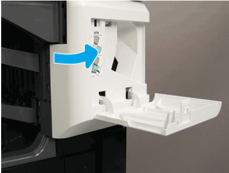
Figure 5-873 Remove the stapler cover
