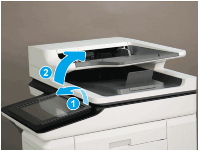
Figure 5-1488 Tilt the control panel and open the document feeder
