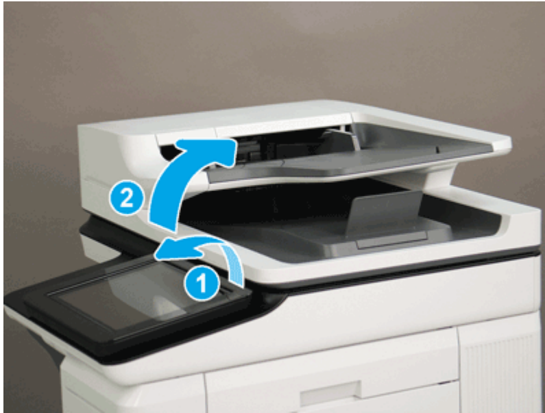
Figure 5-1069 Tilt the control panel forward and open the document feeder
