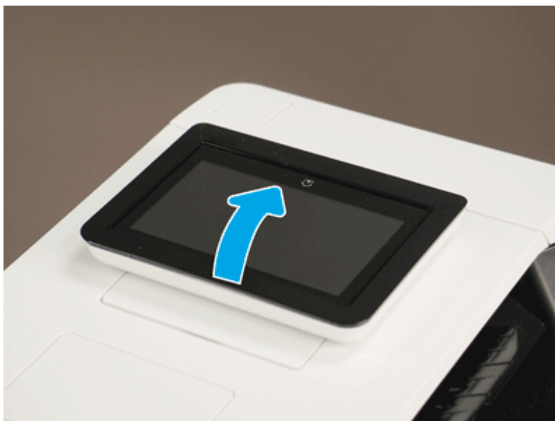
Figure 5-150 Tilt the control panel up
