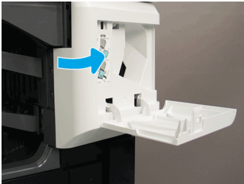
Figure 5-2316 Remove the stapler cover
