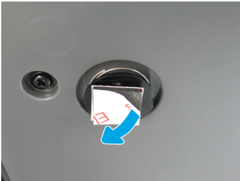
Figure 5-171 Remove the protective film
