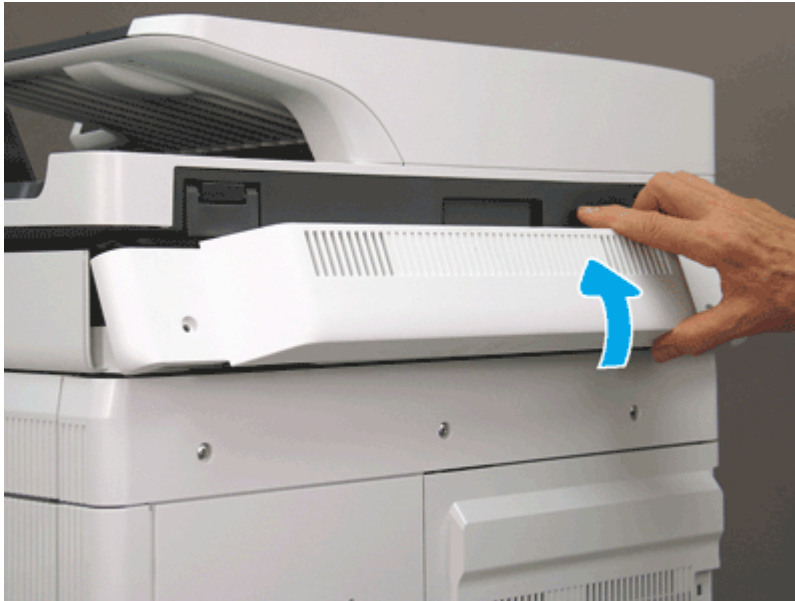
Figure 5-458 Remove the image scanner back cover
