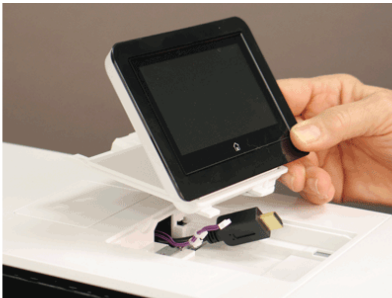
Figure 5-587 Remove the control panel
