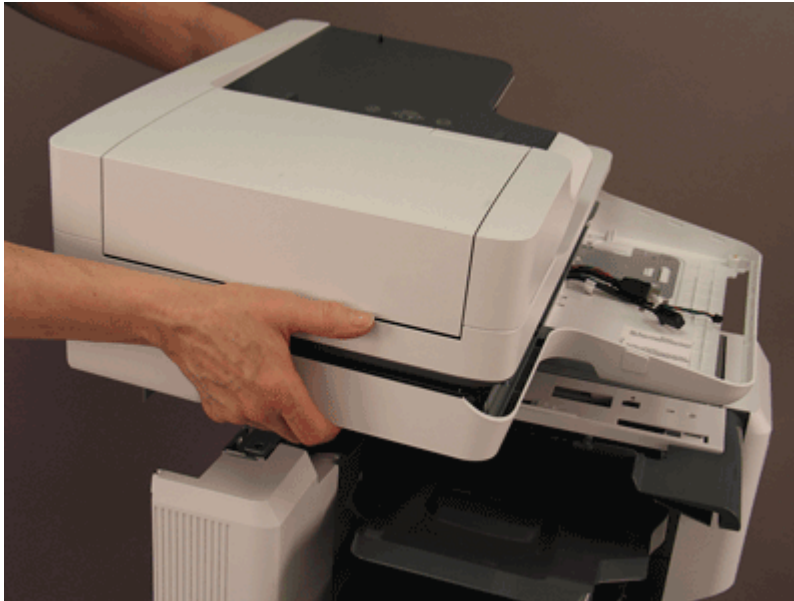
Figure 5-2212 Remove the document feeder and image scanner
