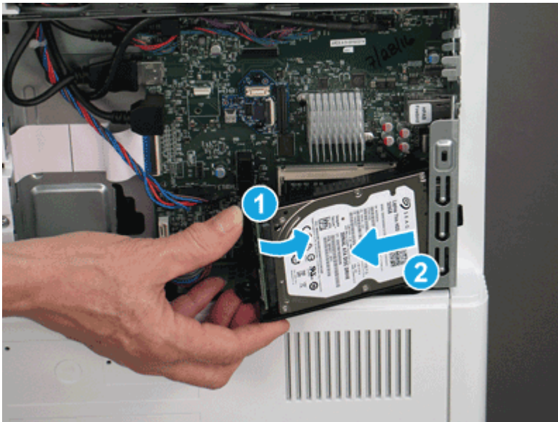
Figure 5-1333 Remove the HDD
