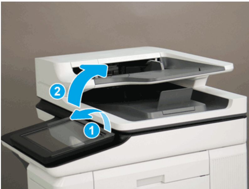
Figure 5-776 Tilt the control panel forward and open the document feeder
