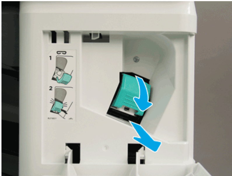
Figure 5-1395 Remove the staple cartridge
