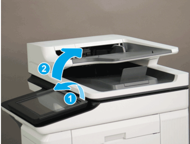
Figure 5-2271 Tilt the control panel and open the document feeder
