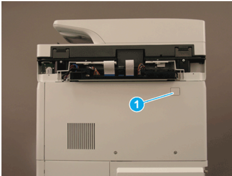
Figure 5-2337 Remove one screw cover
