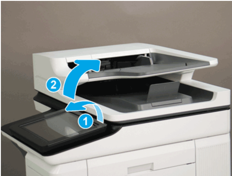
Figure 5-460 Tilt the control panel and open the document feeder
