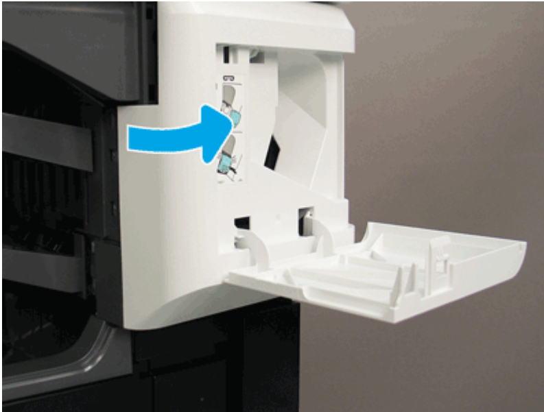
Figure 5-2377 Remove the stapler cover
