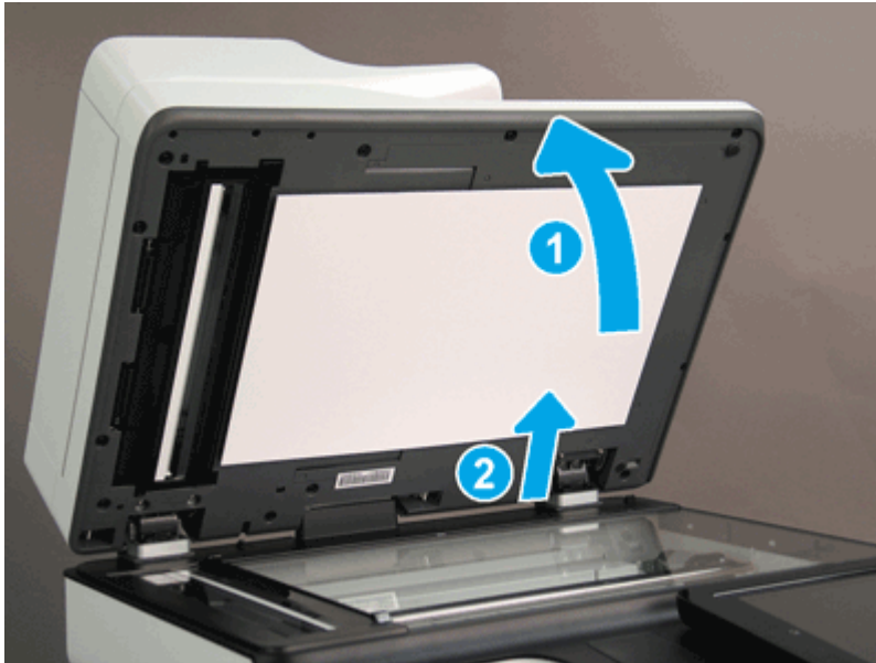
Figure 5-645 Tilt and lift the document feeder
