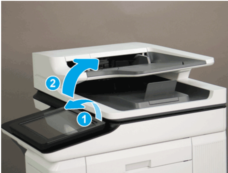
Figure 5-283 Tilt the control panel and open the document feeder
