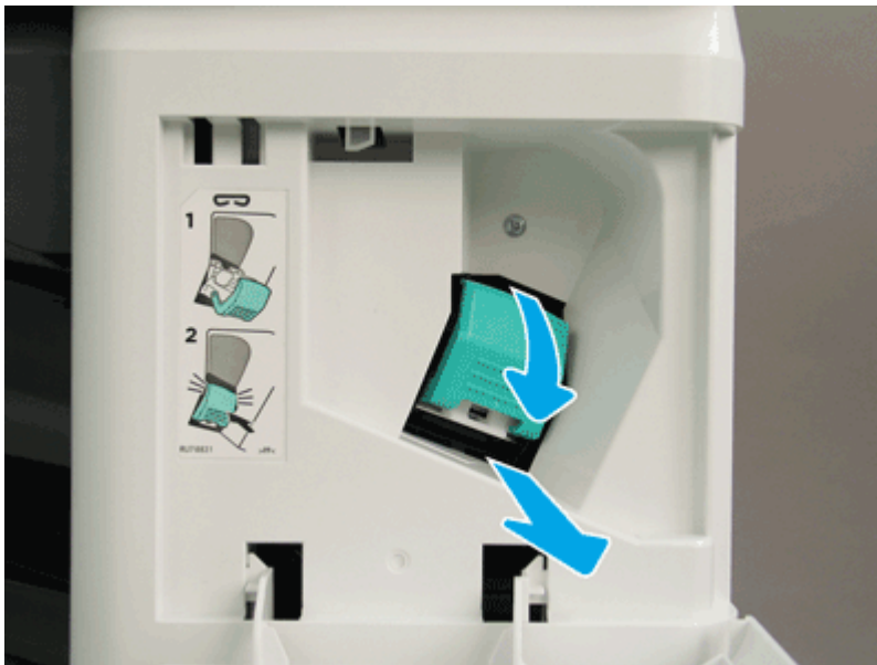
Figure 5-1282 Remove the staple cartridge
