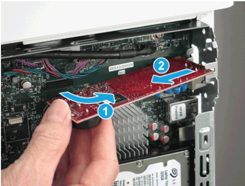
Figure 5-111 Remove the fax PCA
