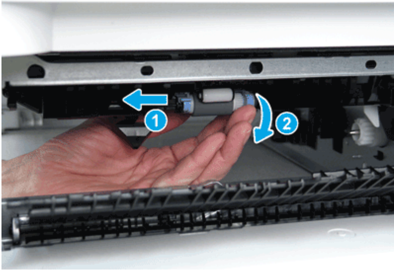
Figure 2-25 Remove the pickup roller assembly
