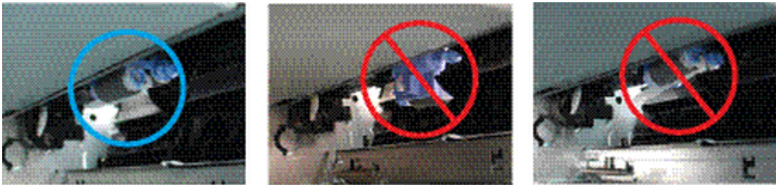
Figure 2-69 Roller correct and incorrect installation
