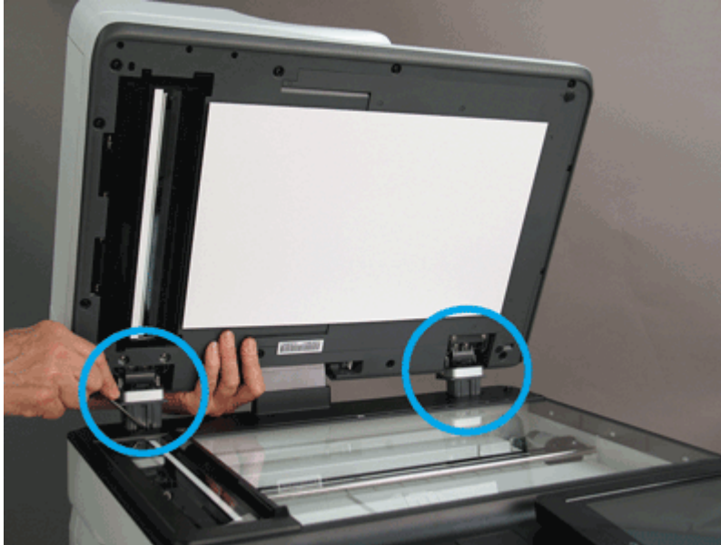
Figure 5-636 Release two tabs
