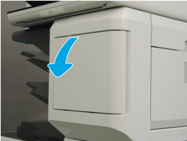
Figure 5-1394 Open the stapler door
