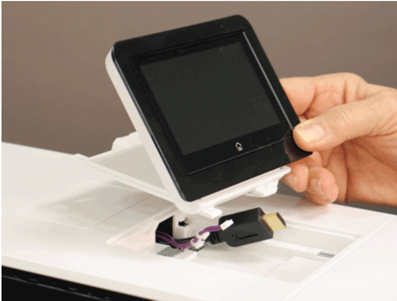
Figure 5-1542 Remove the control panel
