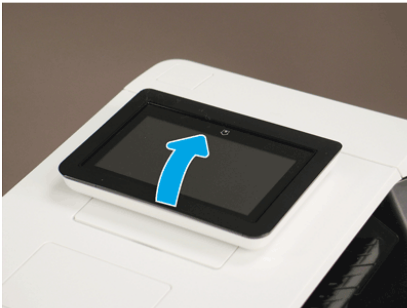
Figure 5-968 Tilt the control panel up
