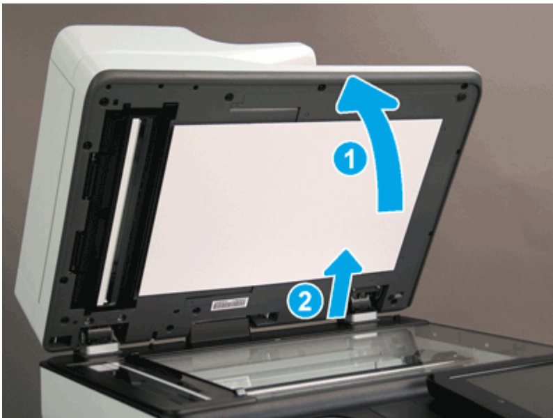
Figure 5-635 Tilt and lift the document feeder
