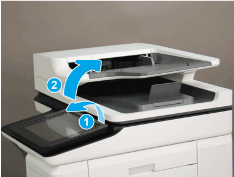
Figure 5-926 Tilt the control panel forward and open the document feeder
