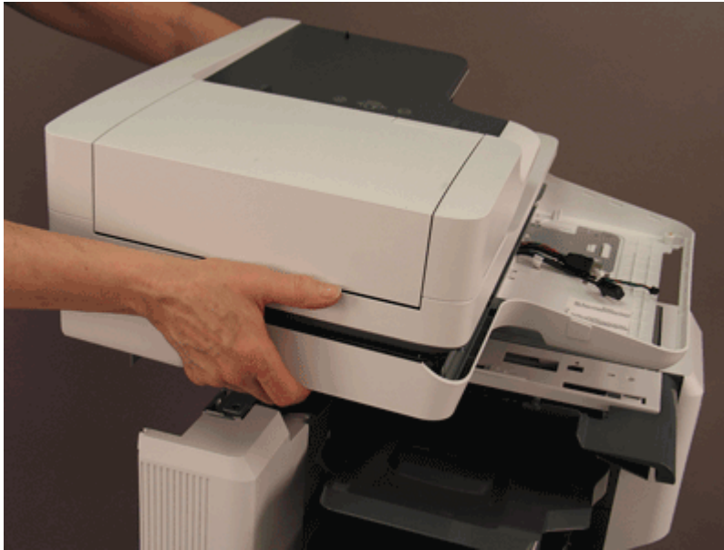
Figure 5-445 Remove the document feeder and image scanner
