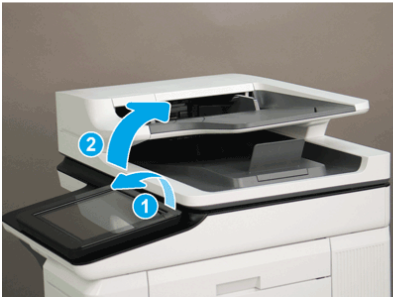
Figure 5-2405 Tilt the control panel and open the document feeder
