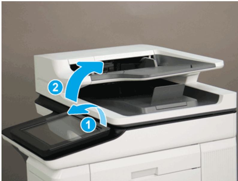
Figure 5-532 Tilt the control panel and open the document feeder
