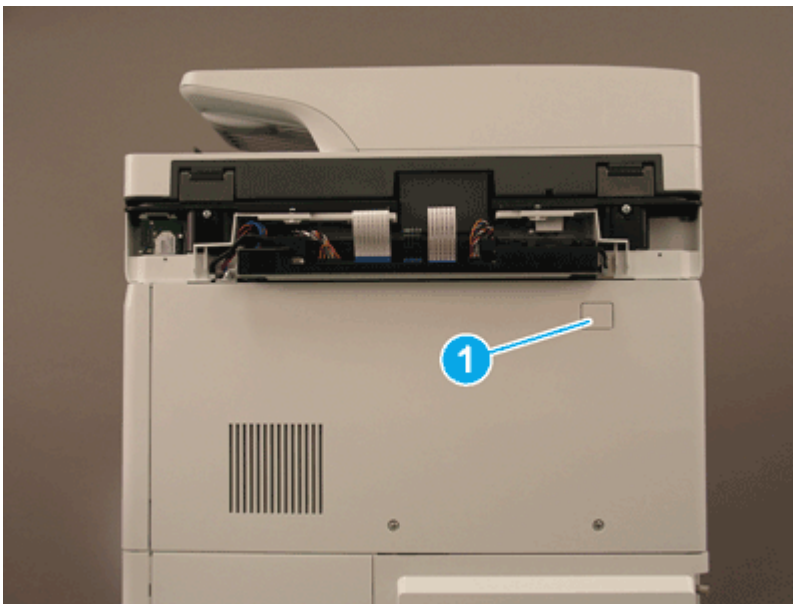
Figure 5-2232 Remove one screw cover
