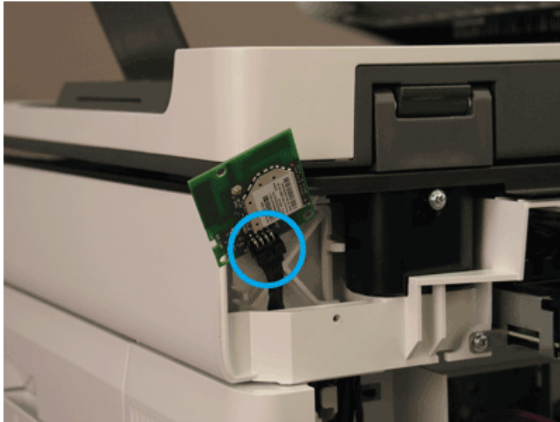
Figure 5-988 Connect the wireless card connector
