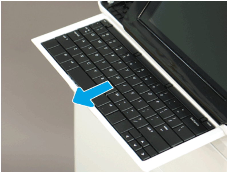
Figure 5-1066 Slide the keyboard tray out
