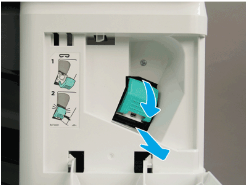
Figure 5-2215 Remove the staple cartridge
