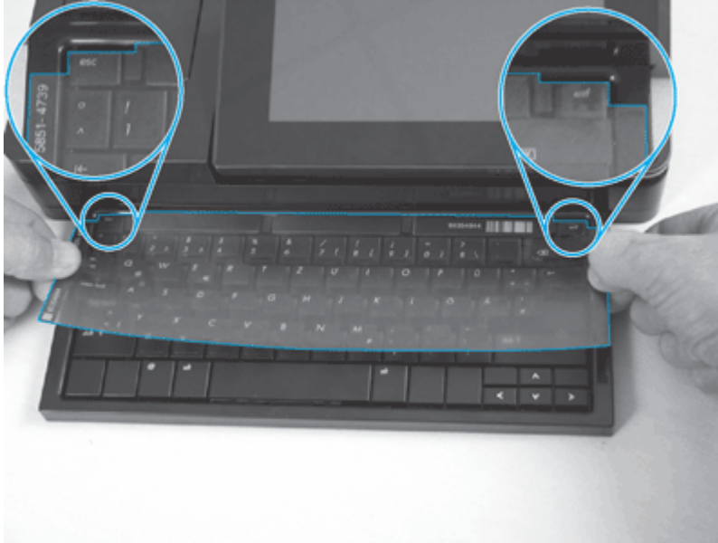
Figure 5-204 Position the keyboard overlay
