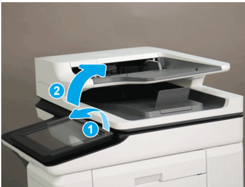
Figure 5-316 Tilt the control panel and open the document feeder
