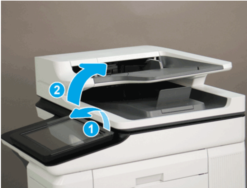
Figure 5-2317 Tilt the control panel and open the document feeder
