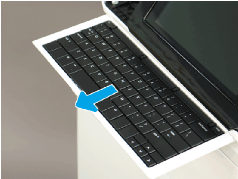
Figure 5-1370 Slide the keyboard tray out
