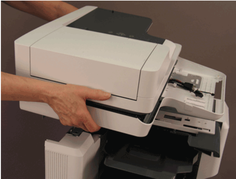
Figure 5-795 Remove the document feeder and image scanner
