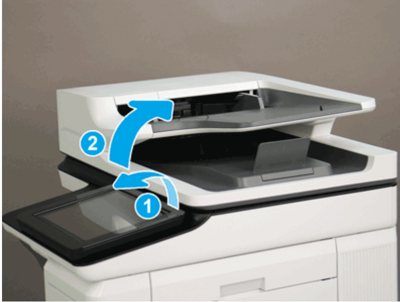
Figure 5-2193 Tilt the control panel forward and open the document feeder
