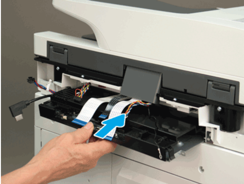
Figure 5-690 Check the cables when installing the SCB
