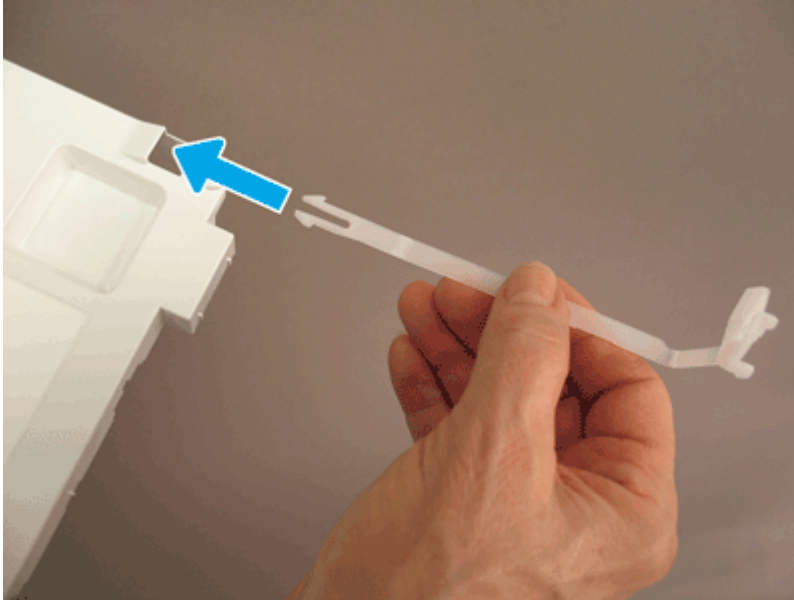
Figure 5-745 Reinstall the link arm
