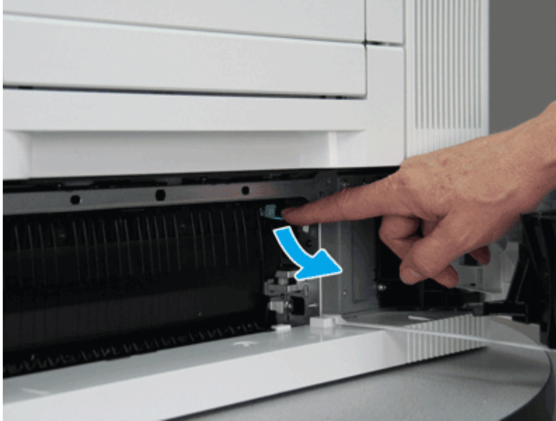
Figure 2-23 Lower the assembly cover
