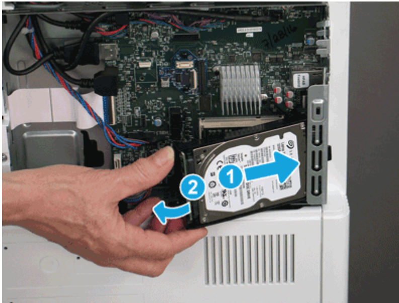
Figure 5-106 Install the HDD
