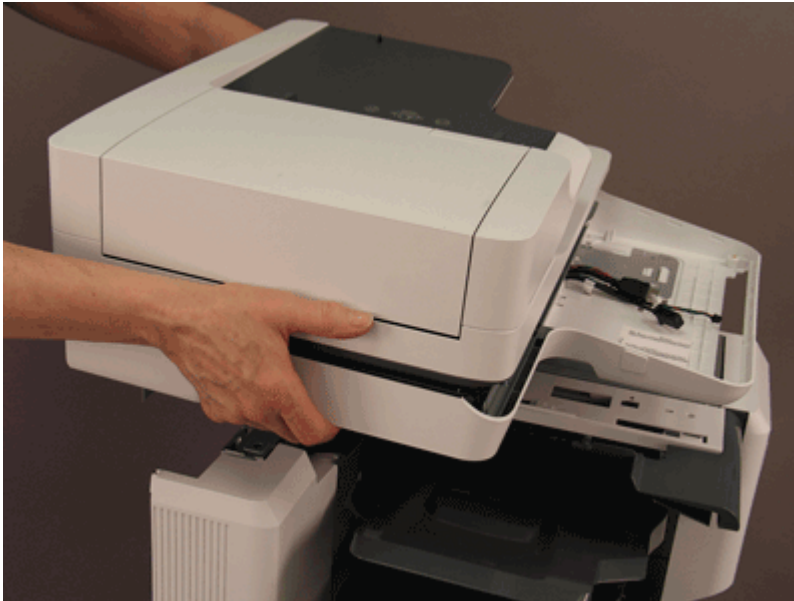
Figure 5-1642 Remove the document feeder and image scanner
