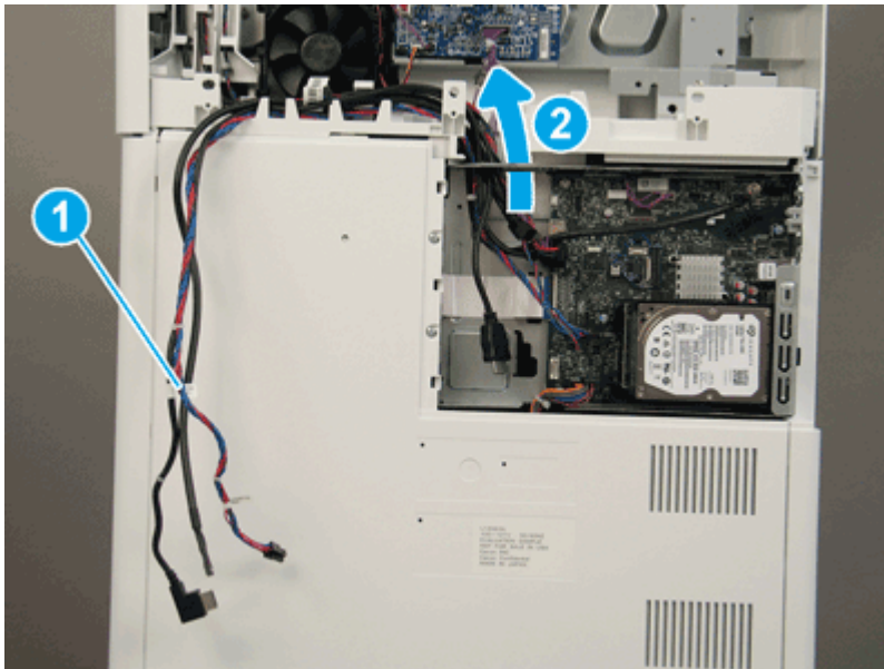
Figure 5-674 Thread the cables
