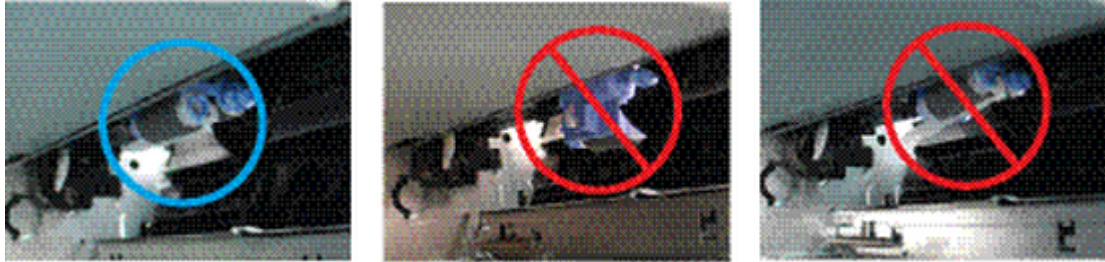
Figure 5-244 Roller correct and incorrect installation
