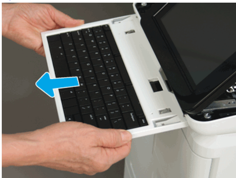
Figure 5-538 Remove the keyboard
