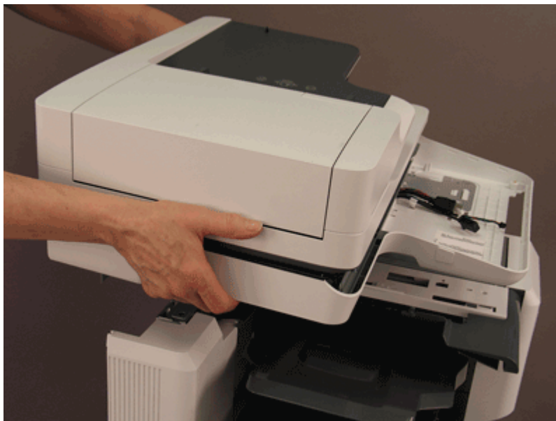
Figure 5-342 Remove the document feeder and image scanner
