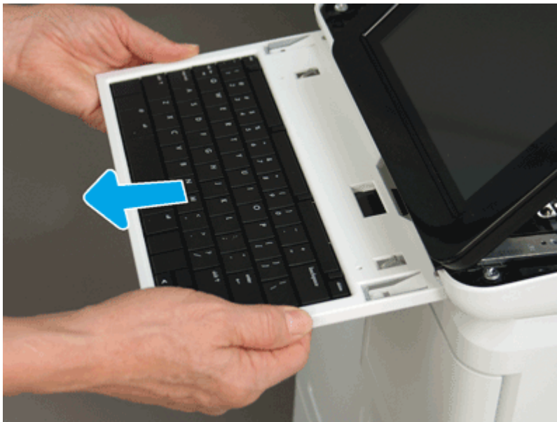
Figure 5-925 Remove the keyboard
