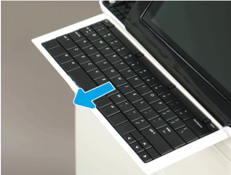
Figure 5-423 Slide the keyboard tray out
