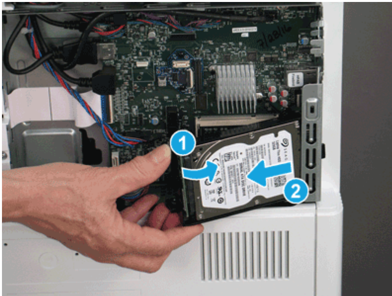
Figure 5-1315 Remove the HDD
