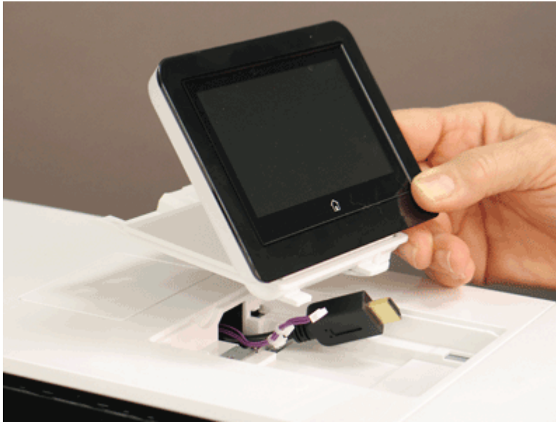
Figure 5-1116 Remove the control panel
