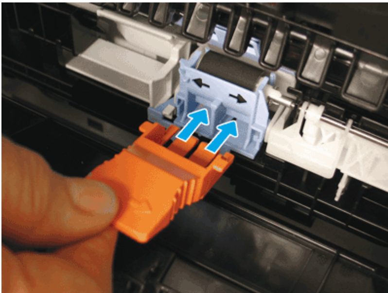
Figure 2-76 Install the orange tool
