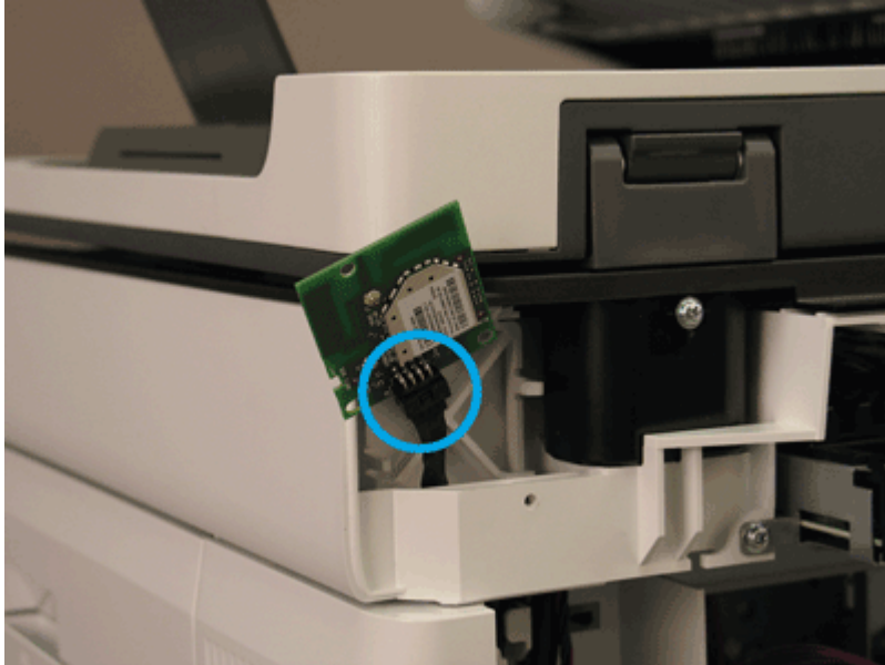
Figure 5-347 Connect the wireless card connector
