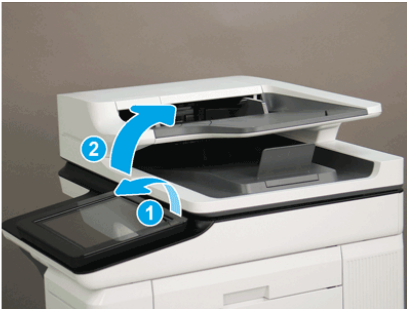
Figure 5-648 Tilt the control panel and open the document feeder
