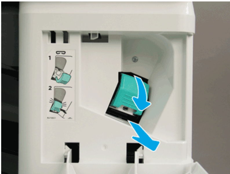
Figure 5-798 Remove the staple cartridge
