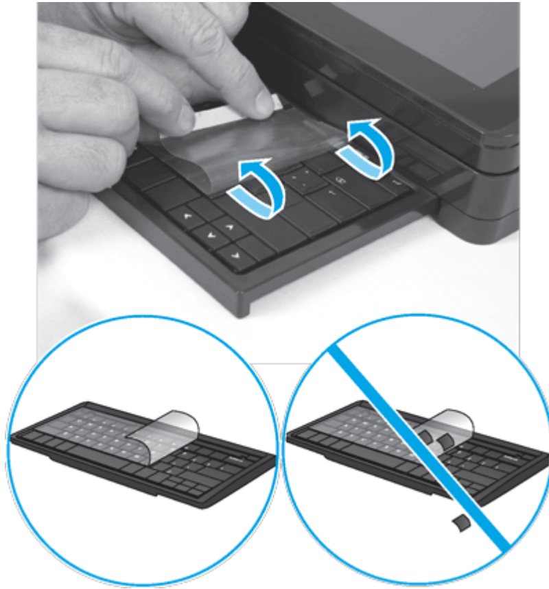
Figure 5-206 Apply the keyboard overlay
