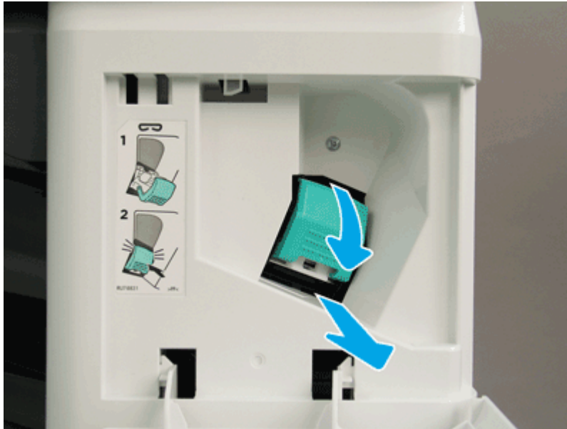
Figure 5-1517 Remove the staple cartridge
