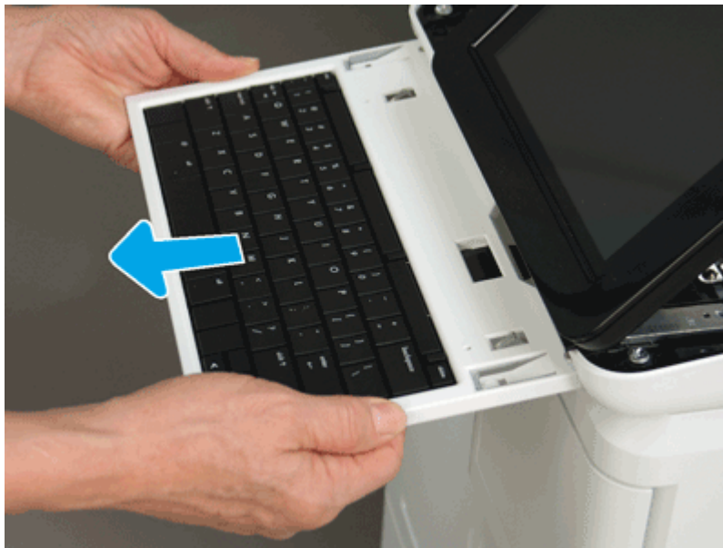
Figure 5-1494 Remove the keyboard
