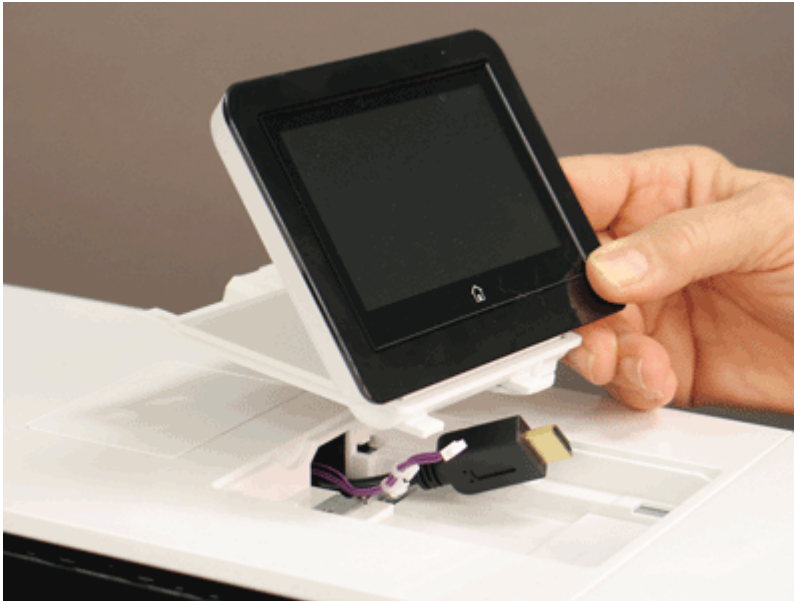
Figure 5-155 Remove the control panel
