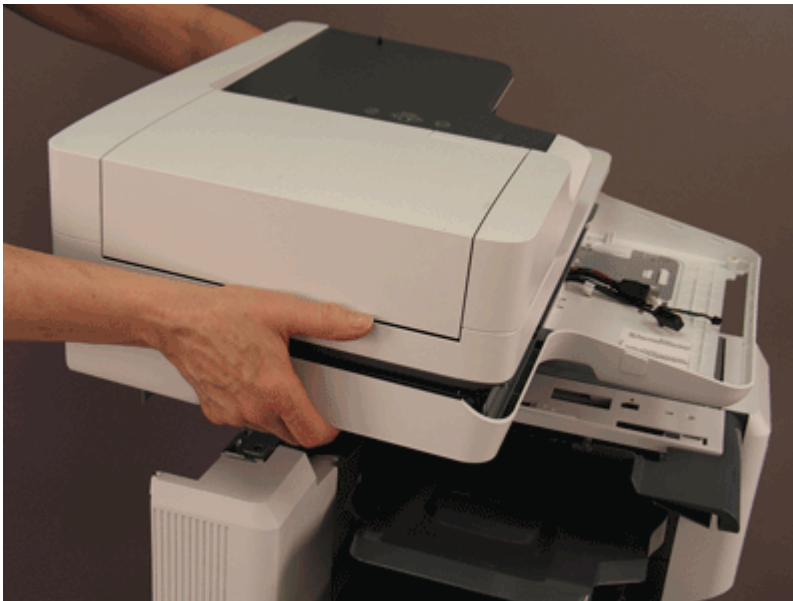
Figure 5-868 Remove the document feeder and image scanner
