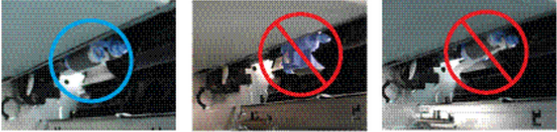
Figure 2-64 Roller correct and incorrect installation
