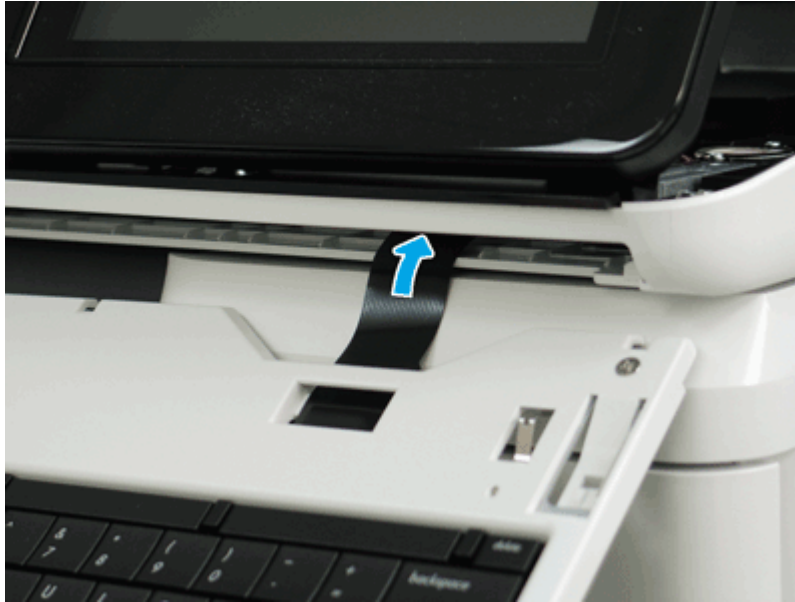
Figure 5-195 Position the flat cable in the slot
