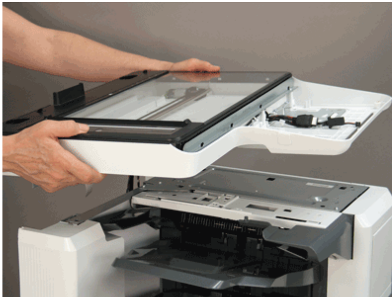
Figure 5-678 Remove the image scanner assembly
