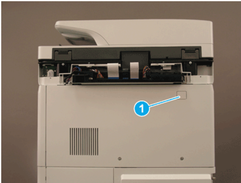
Figure 5-2389 Remove one screw cover
