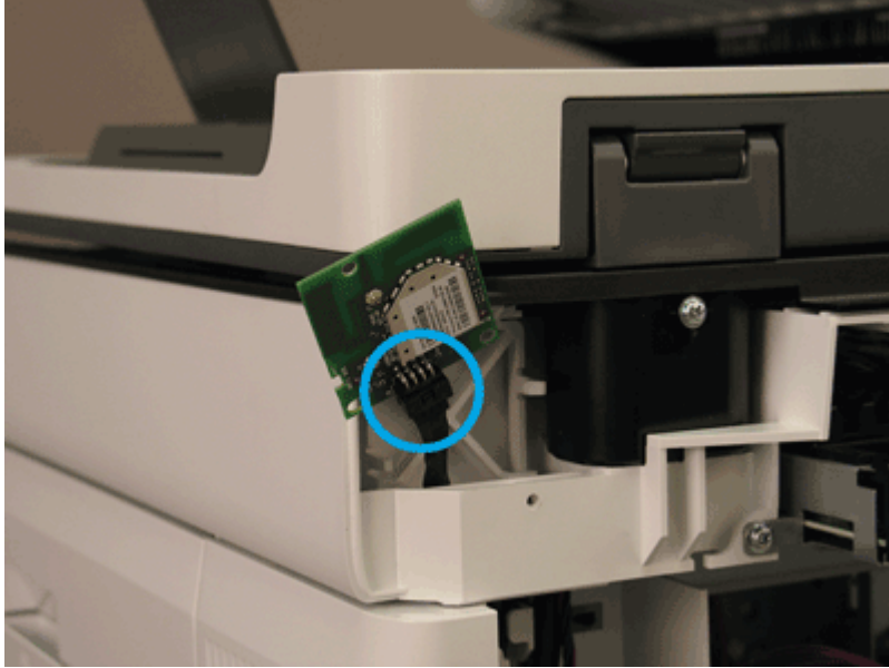
Figure 5-1230 Connect the wireless card connector
