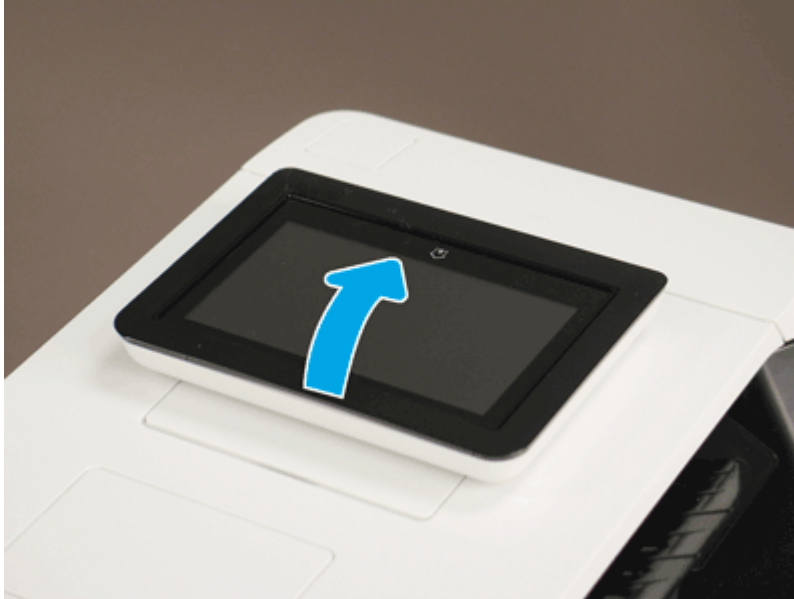
Figure 5-582 Tilt the control panel up
