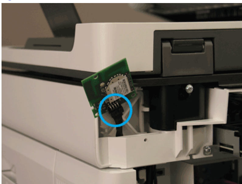
Figure 5-496 Connect the wireless card connector
