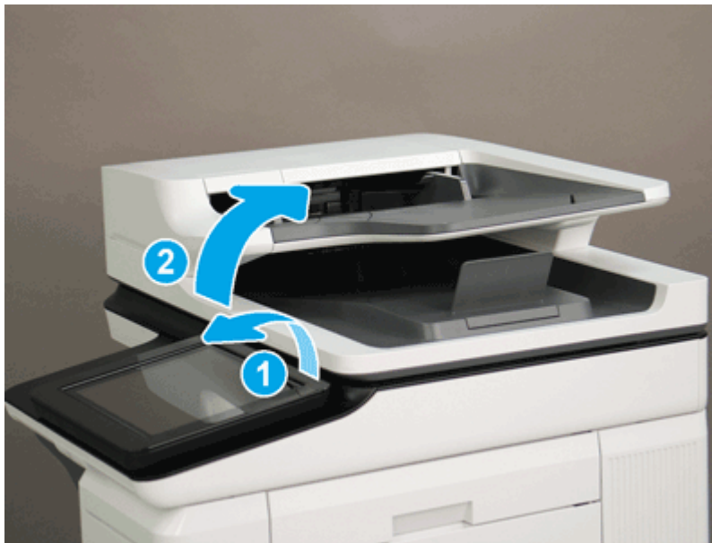
Figure 5-1062 Tilt the control panel and open the document feeder
