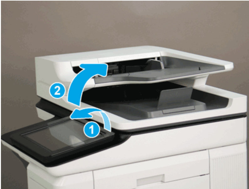
Figure 5-1495 Tilt the control panel forward and open the document feeder
