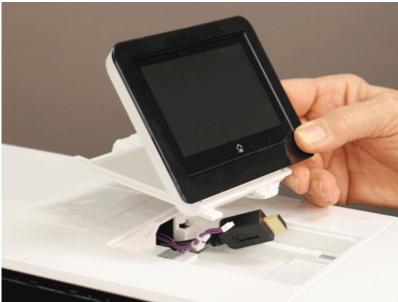
Figure 5-1306 Remove the control panel
