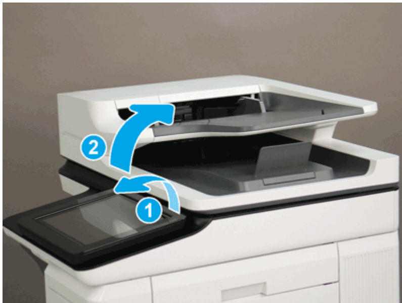
Figure 5-2427 Tilt the control panel and open the document feeder
