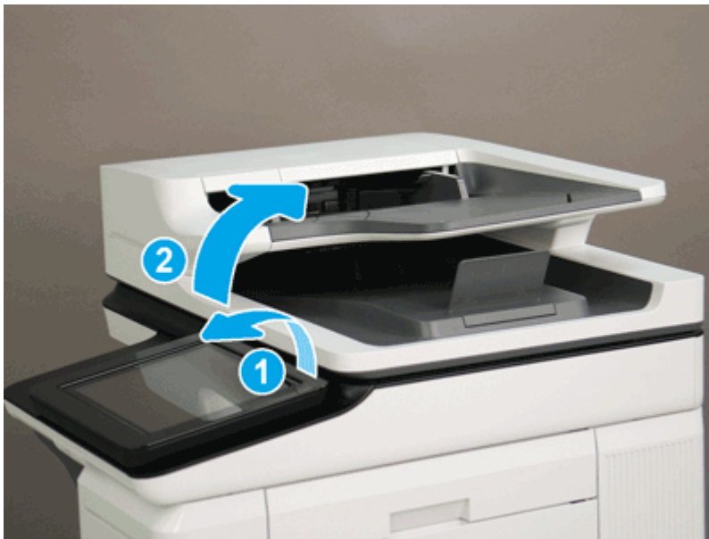
Figure 5-426 Tilt the control panel forward and open the document feeder
