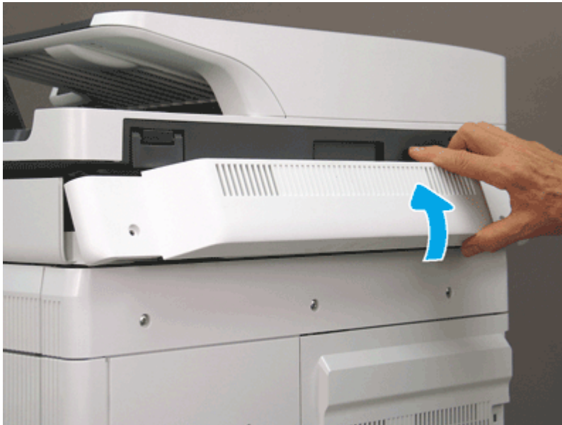
Figure 5-687 Remove the image scanner back cover
