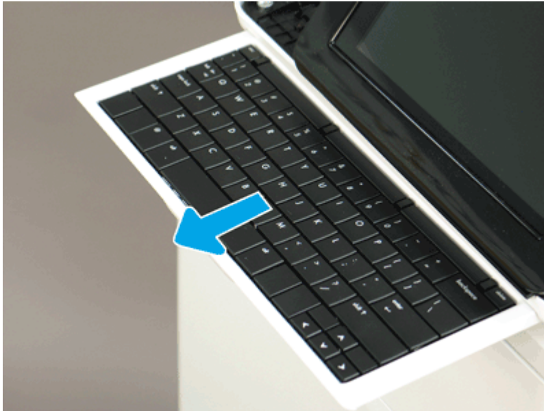
Figure 5-853 Slide the keyboard tray out
