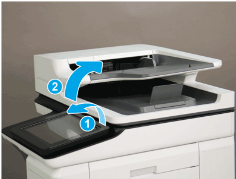
Figure 5-350 Tilt the control panel and open the document feeder
