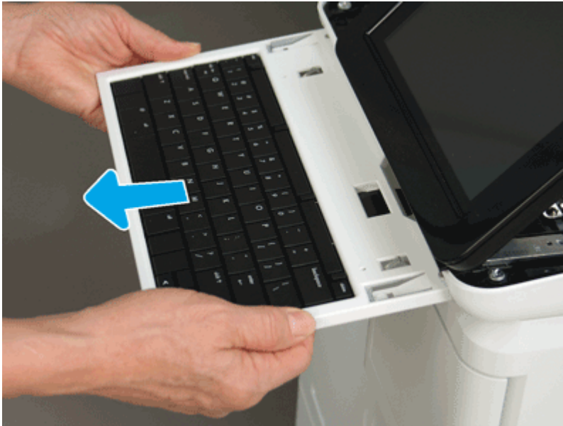
Figure 5-775 Remove the keyboard
