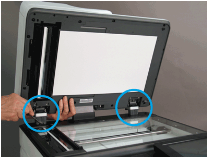
Figure 5-628 Release two tabs
