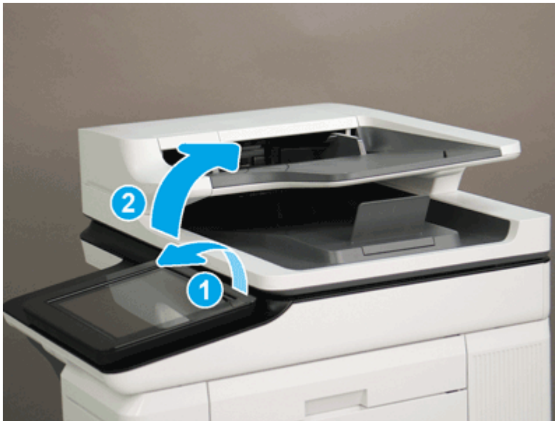
Figure 5-207 Tilt the control panel forward and open the document feeder
