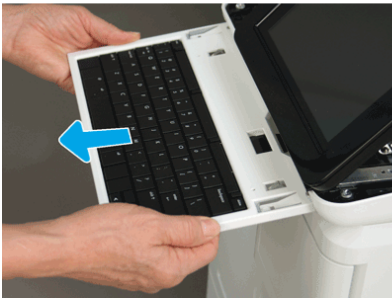
Figure 5-1068 Remove the keyboard
