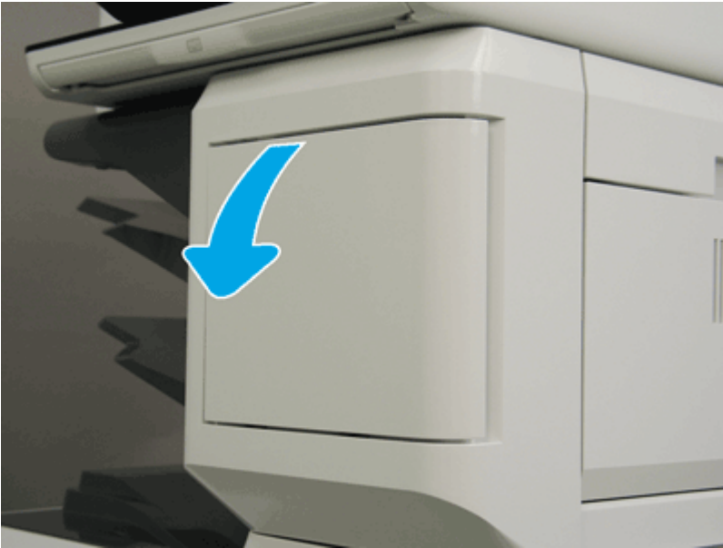
Figure 5-2290 Open the stapler door
