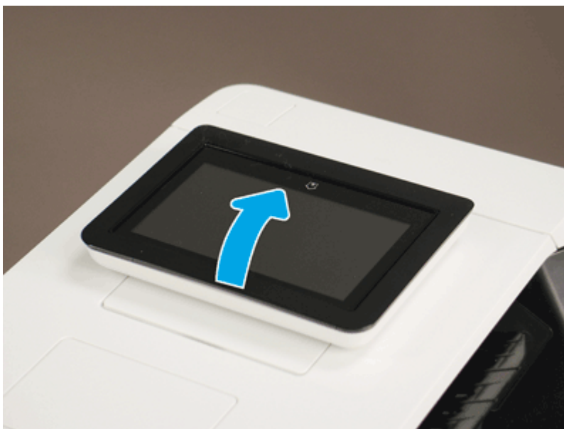
Figure 5-891 Tilt the control panel up
