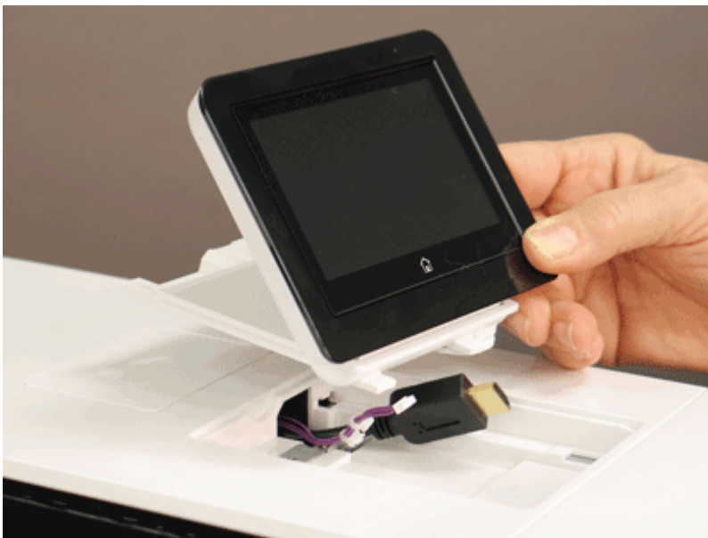
Figure 5-823 Remove the control panel
