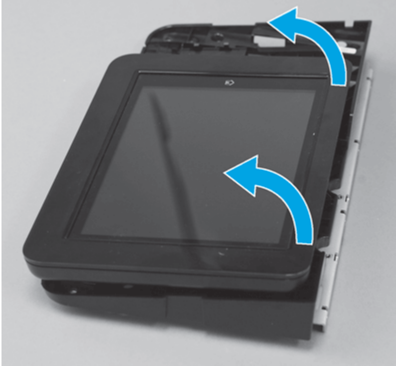
Figure 5-214 Tilt the control panel
