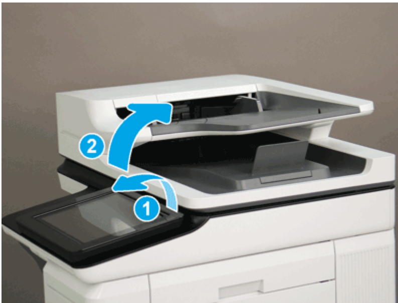
Figure 5-384 Tilt the control panel and open the document feeder
