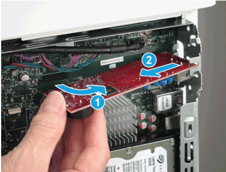
Figure 5-1126 Remove the fax PCA
