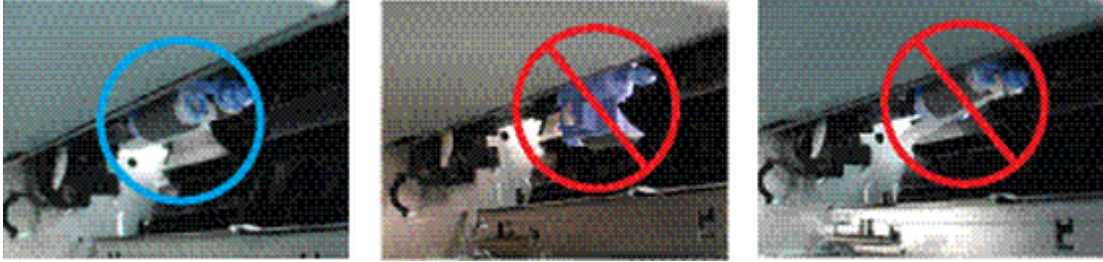
Figure 2-41 Roller correct and incorrect installation
