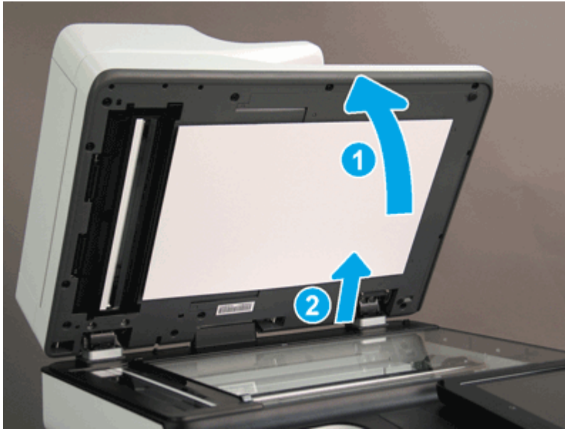
Figure 5-627 Tilt and lift the document feeder
