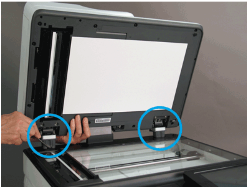
Figure 5-646 Release two tabs
