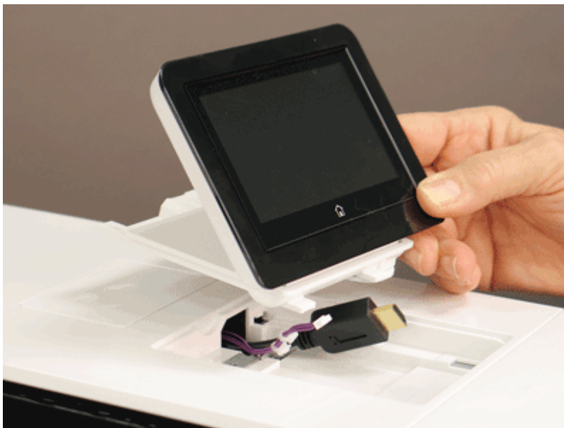
Figure 5-1594 Remove the control panel
