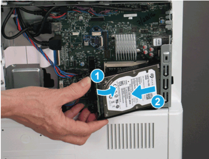
Figure 5-1128 Remove the HDD
