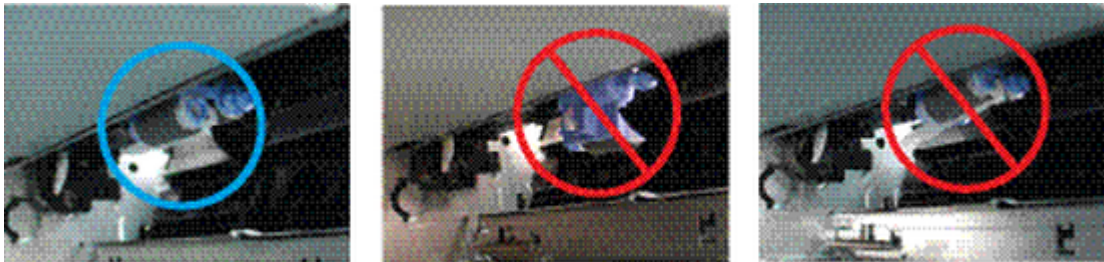
Figure 5-249 Roller correct and incorrect installation
