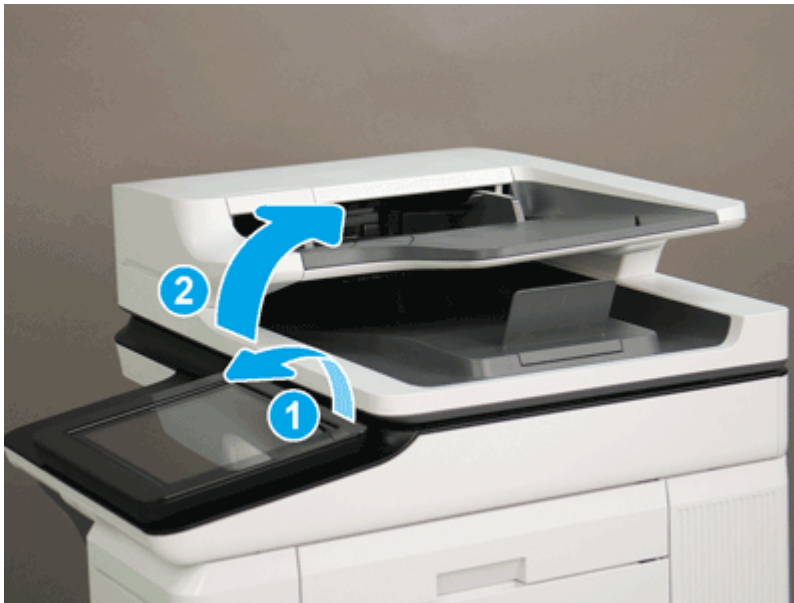
Figure 5-467 Tilt the control panel forward and open the document feeder
