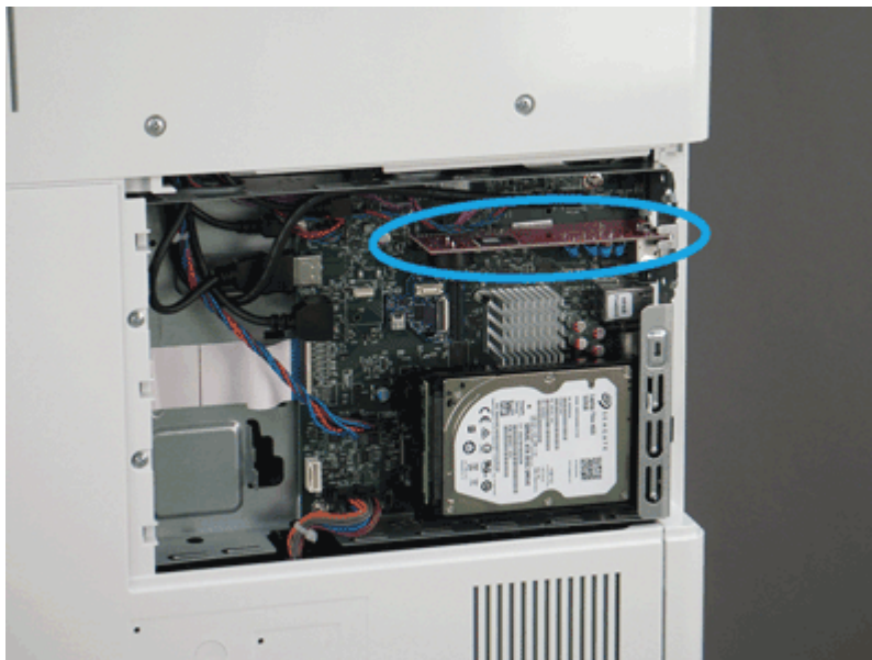
Figure 5-1209 Locate the fax PCA
