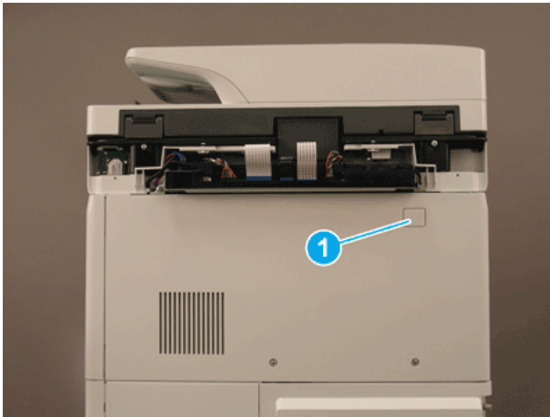
Figure 5-2263 Remove one screw cover
