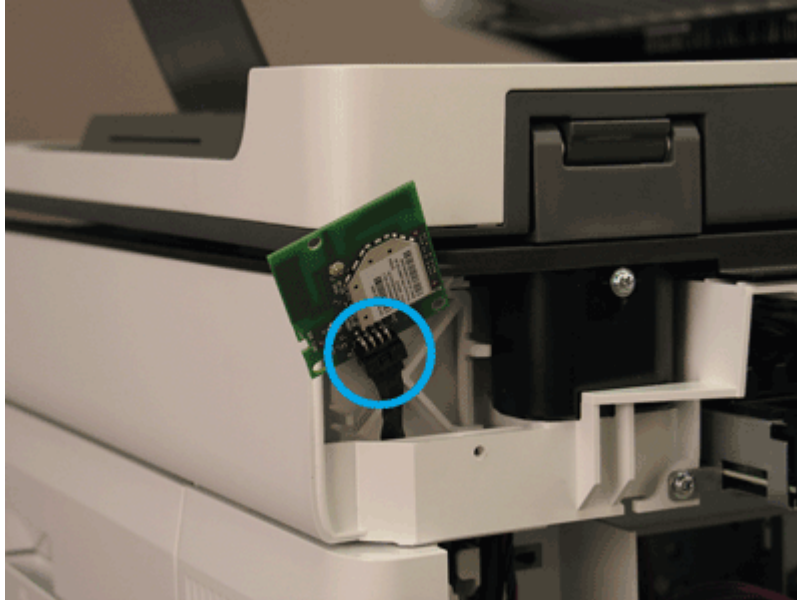
Figure 5-1683 Connect the wireless card connector
