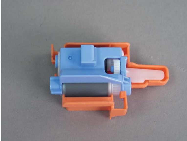
Figure 1-240 Do not remove the orange installation tray
