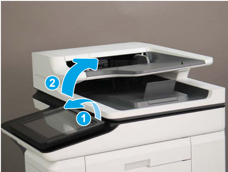
Figure 1-1340 Tilt the control panel forward and open the document feeder
