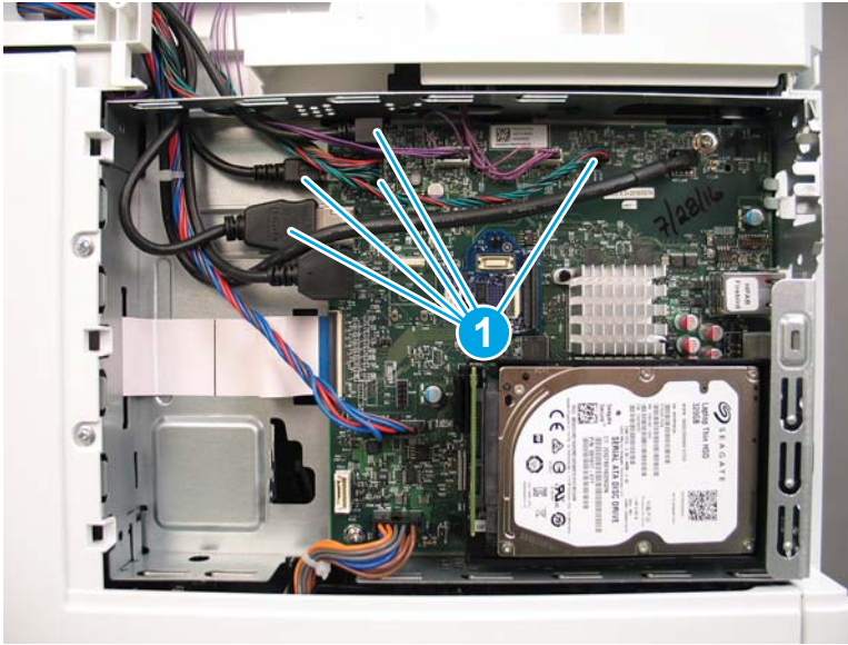
Figure 1-705 Disconnect five connectors
