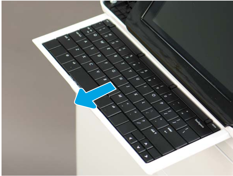
Figure 1-1421 Slide the keyboard tray out
