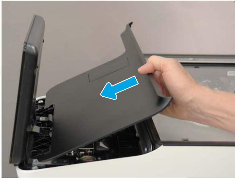
Figure 1-220 Position the cover on the printer
