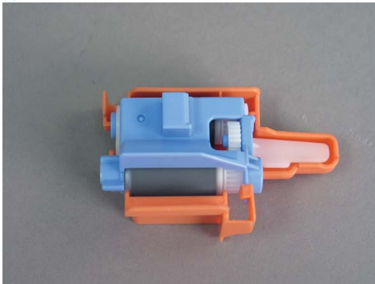
Figure 1-245 Do not remove the orange installation tray
