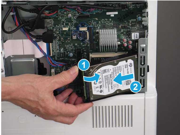
Figure 1-98 Remove the HDD
