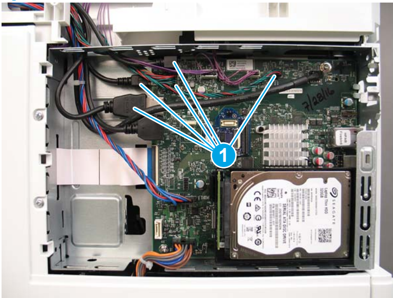
Figure 1-337 Disconnect five connectors
