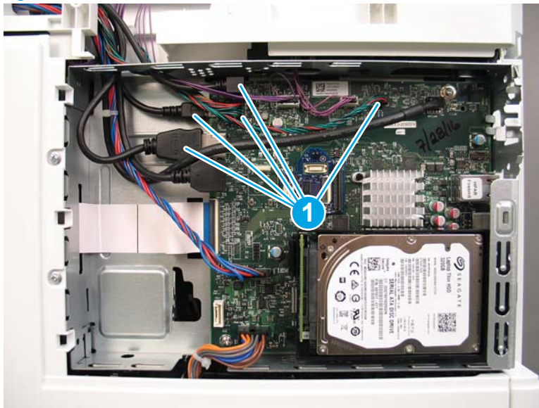
Figure 1-371 Disconnect five connectors
