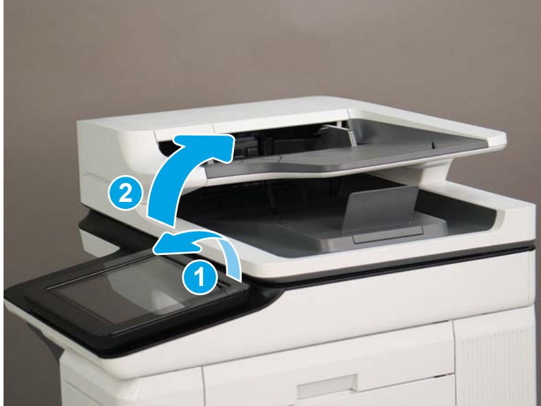
Figure 1-1417 Tilt the control panel and open the document feeder
