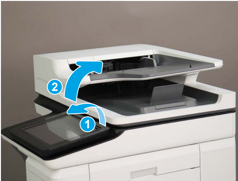
Figure 1-188 Tilt the control panel and open the document feeder
