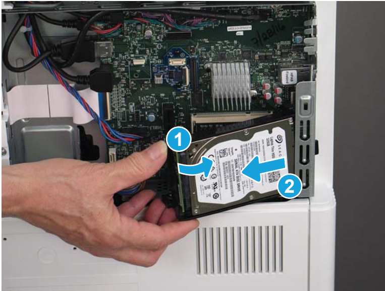
Figure 1-1405 Remove the HDD
