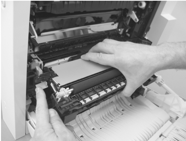
Figure 1-239 Reinstall the secondary transfer assembly
