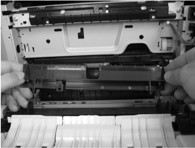
Figure 1-347 Remove the paper-pickup assembly (7 of 11)
