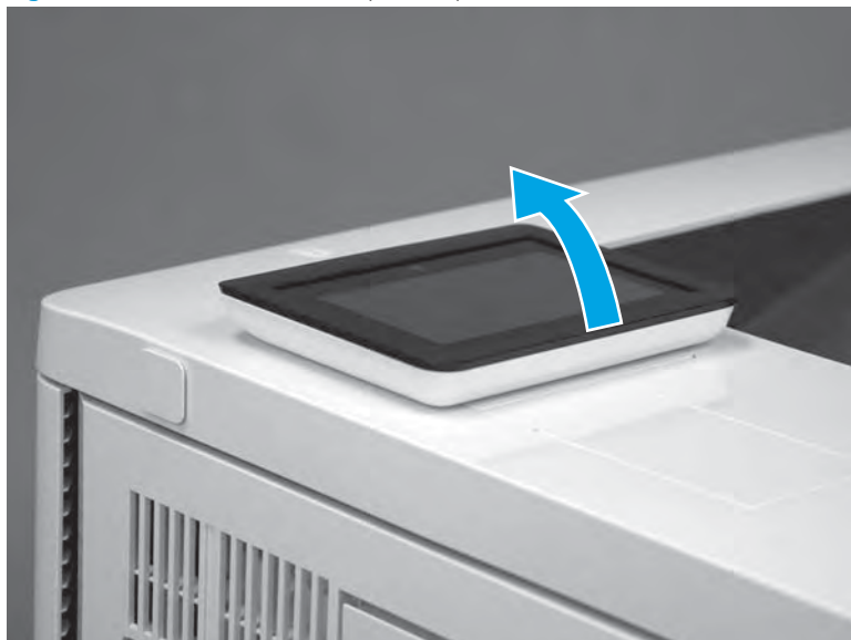
Figure 1-4662 Tilt the control panel up
