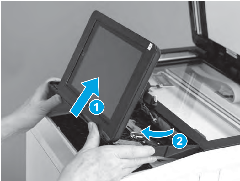
Figure 1-4998 Remove the control panel
