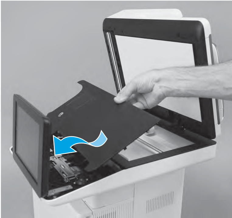
Figure 1-159 Position the control-panel cover on the printer
