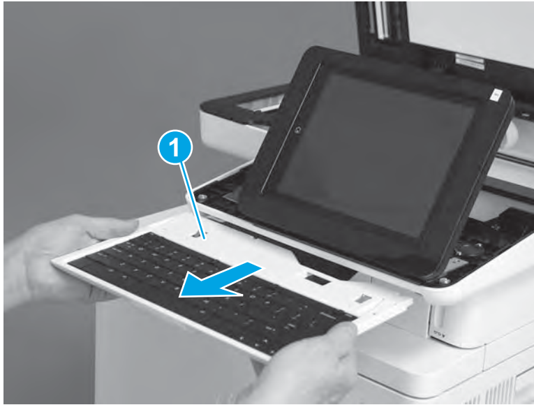
Figure 1-153 Remove the keyboard
