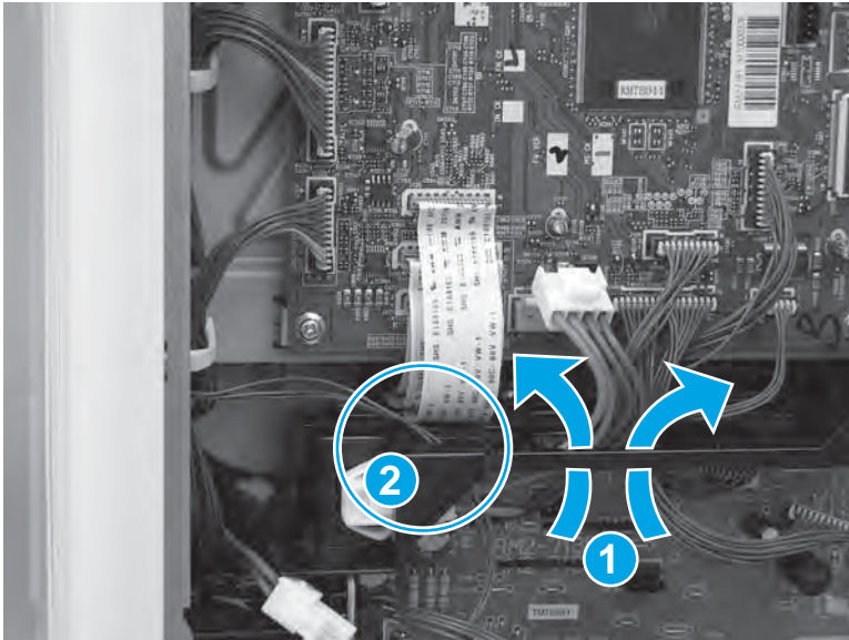
Figure 1-1746 Pass the wire harnesses through the opening
