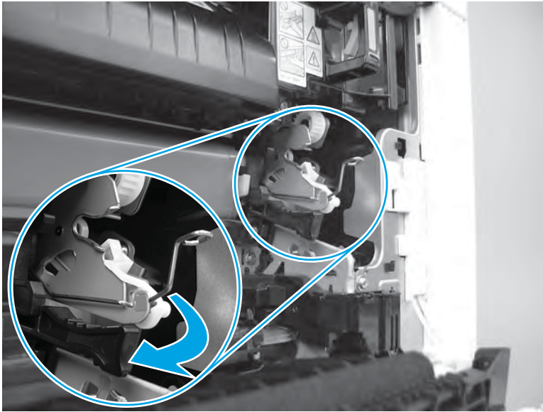
Figure 1-4137 Remove the spring from the holder
