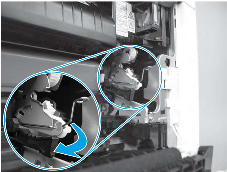
Figure 1-1527 Remove the spring from the holder
