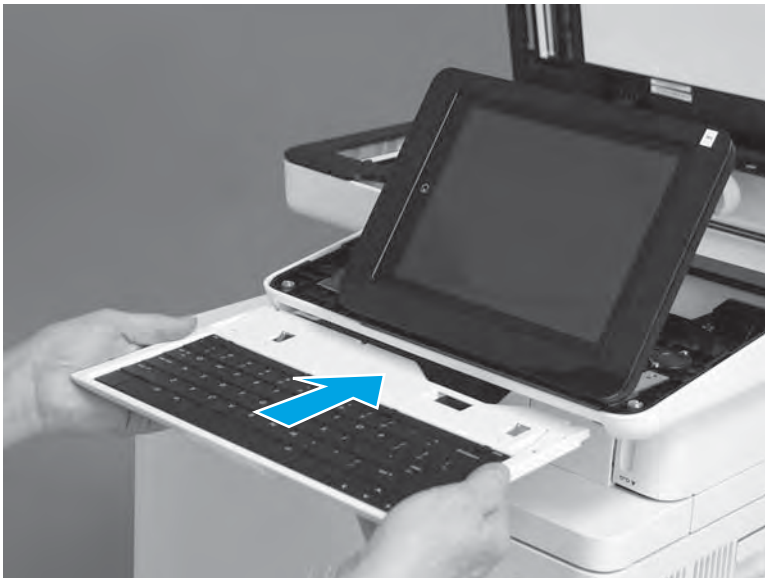
Figure 1-156 Slide the keyboard into the slot
