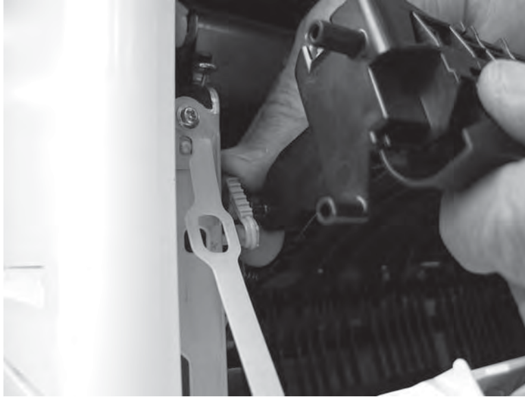
Figure 1-4413 Disengage the blue arm and pin
