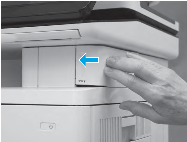
Figure 1-346 Install the cover assembly
