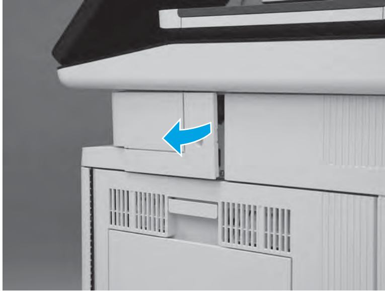
Figure 1-2494 Release the back edge of the cover
