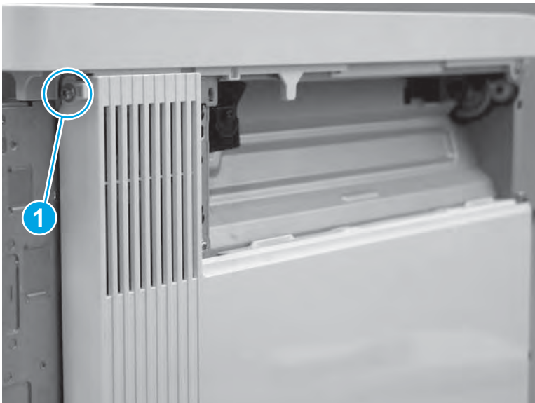
Figure 1-2054 Install one screw
