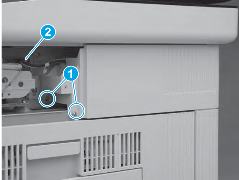
Figure 1-1976 Remove two screws and one connector
