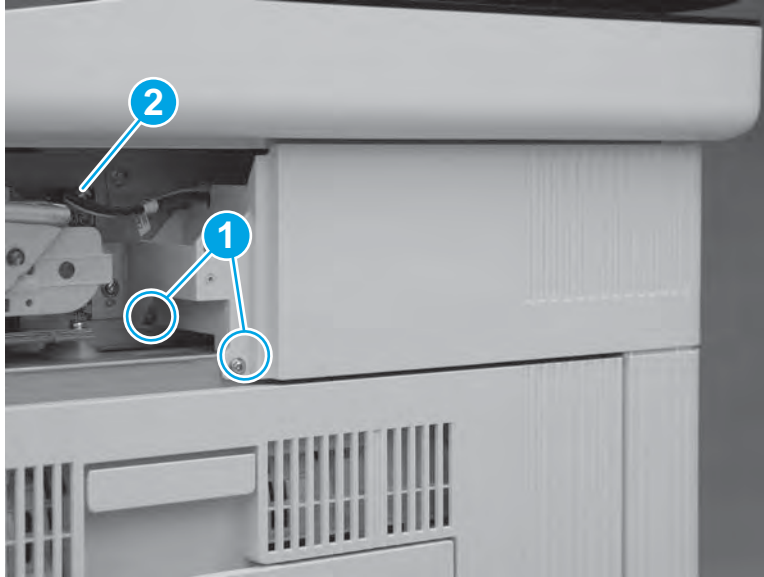
Figure 1-2502 Remove two screws and one connector
