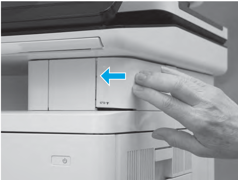
Figure 1-2043 Install the cover assembly
