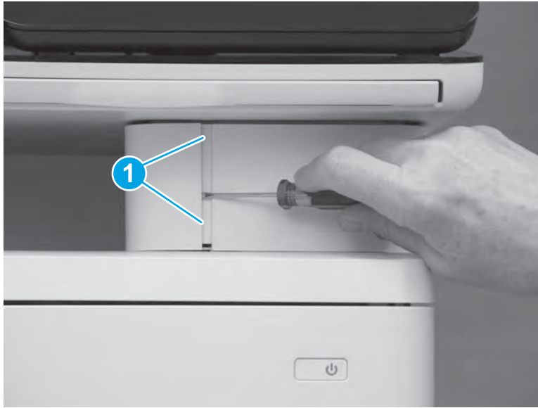
Figure 1-741 Release two tabs
