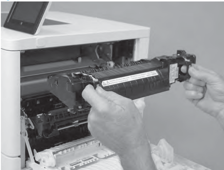
Figure 1-3486 Remove the fuser
