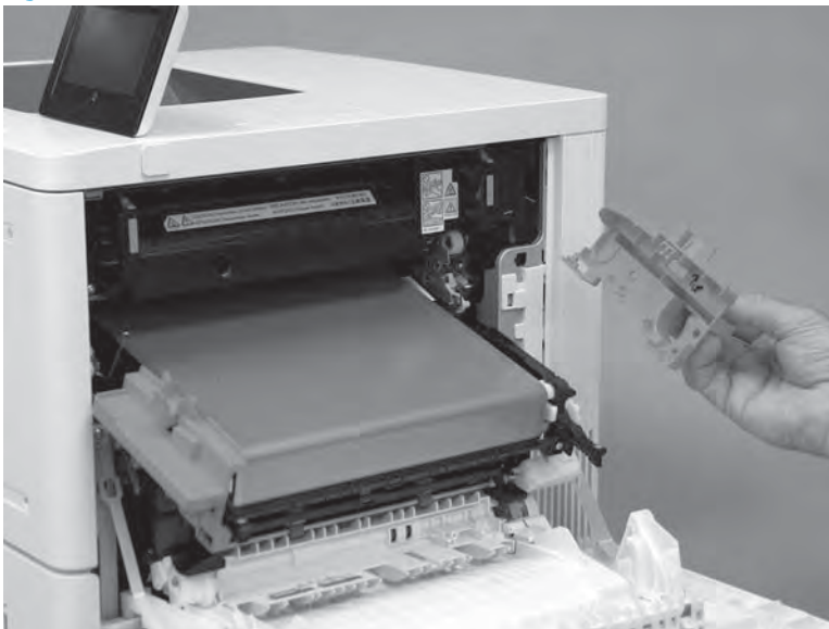
Figure 1-241 Remove the orange handle
