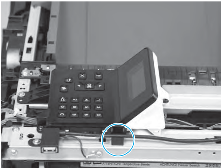
Figure 1-953 Place one cable in the guide
