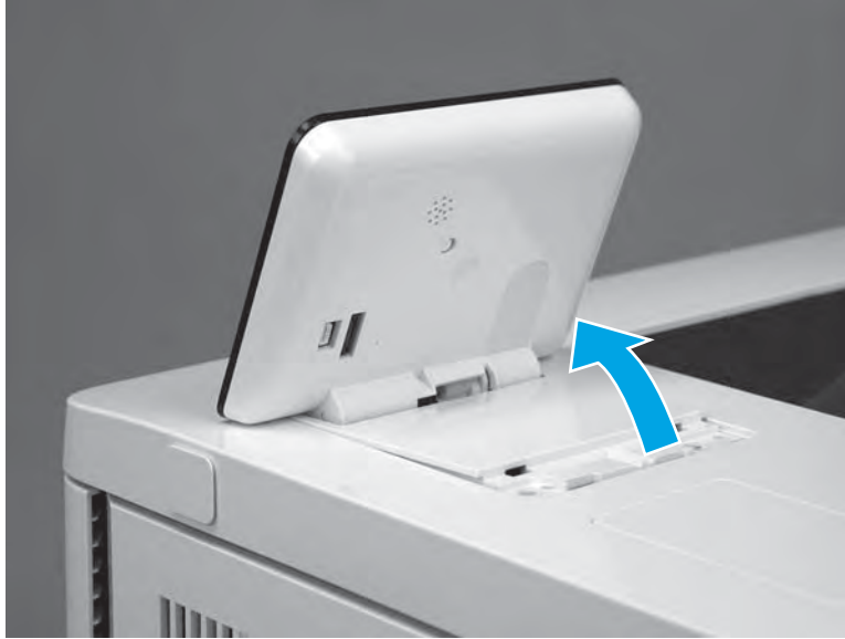
Figure 1-1009 Rotate the control-panel base up
