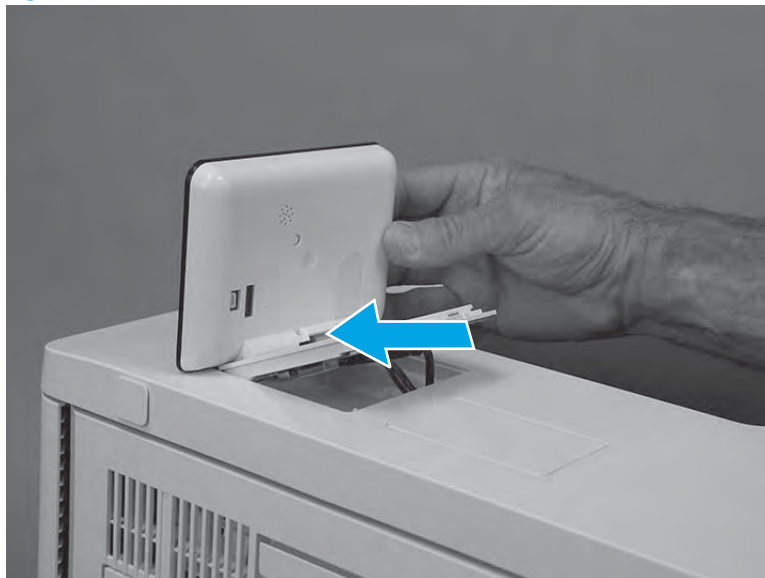
Figure 1-1044 Turn the control panel over
