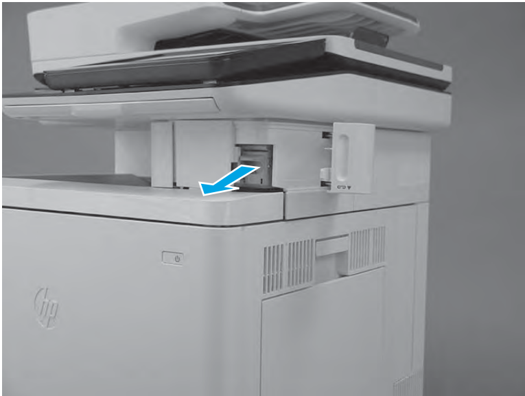
Figure 1-18 Remove the staple cartridge
