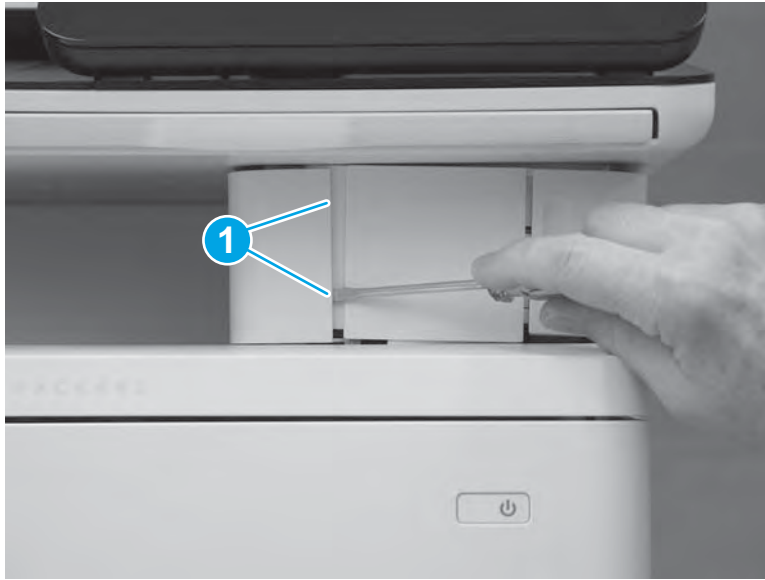
Figure 1-1413 Release two tabs
