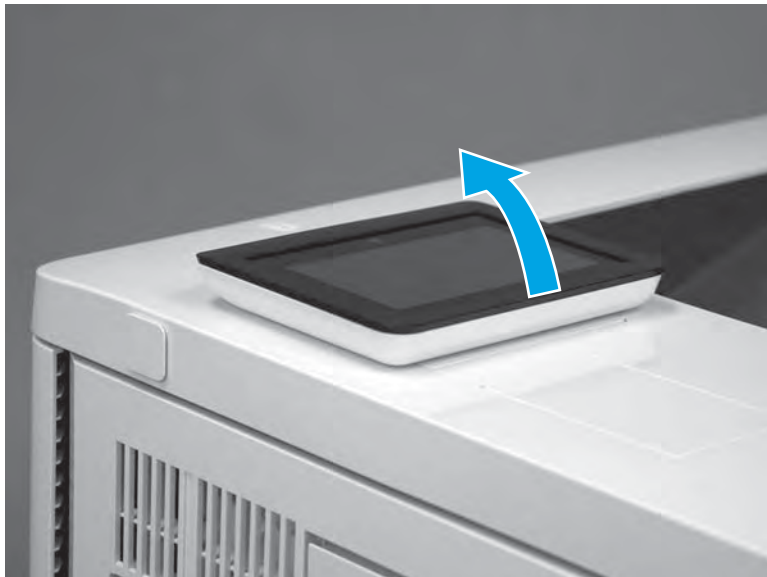
Figure 1-113 Tilt the control panel up
