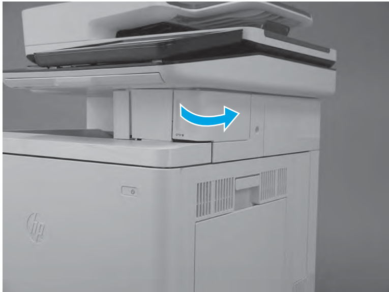
Figure 1-1333 Open the stapler door
