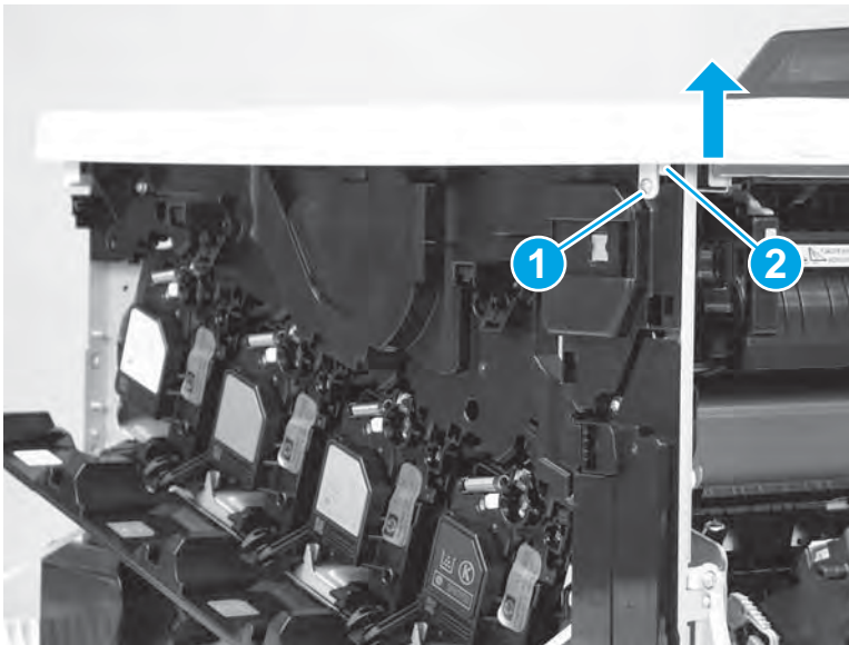
Figure 1-2992 Remove one screw and release one tab
