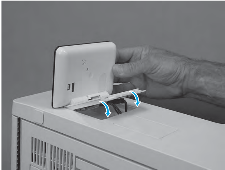
Figure 1-3907 Rotate the control-panel base down
