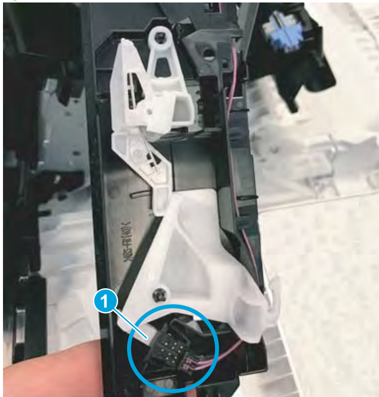
Figure 1-1251 Remove the switch
