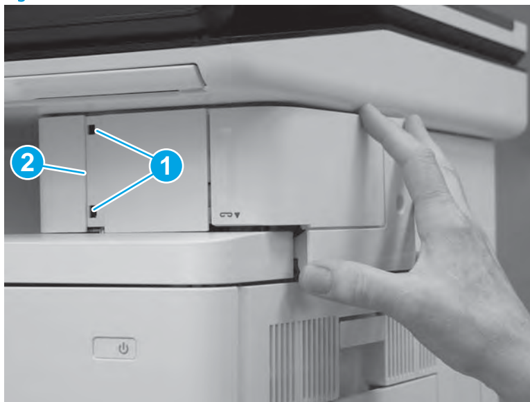
Figure 1-1284 Install two tabs
