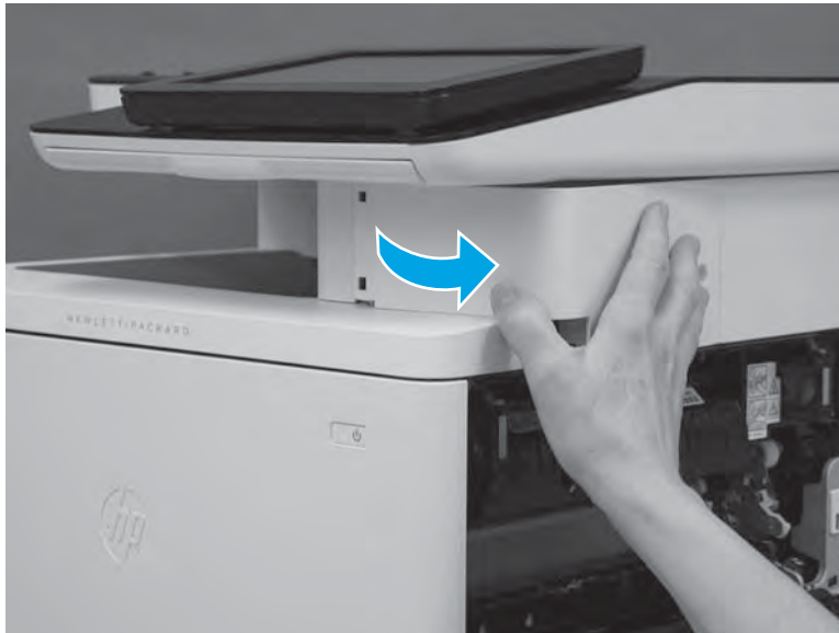
Figure 1-3970 Rotate the cover
