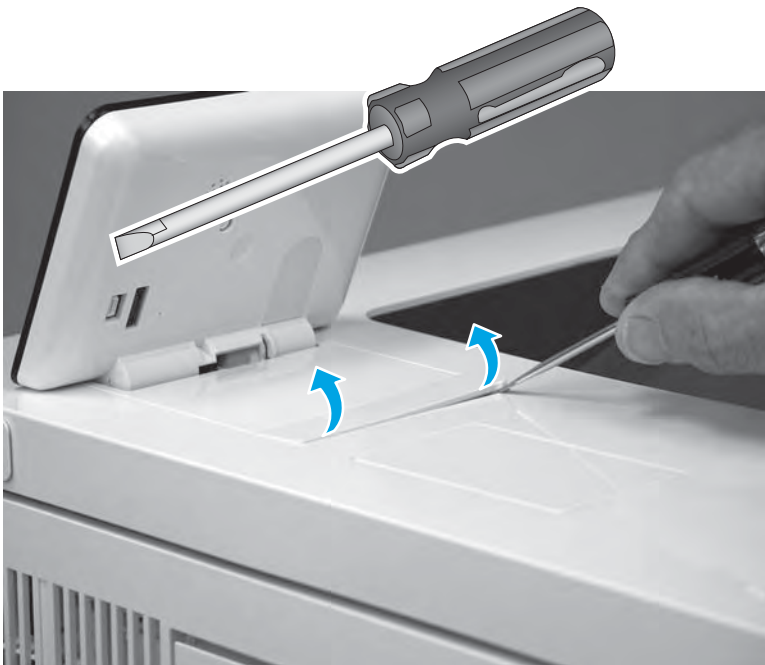
Figure 1-4434 Release the control-panel screws cover tabs
