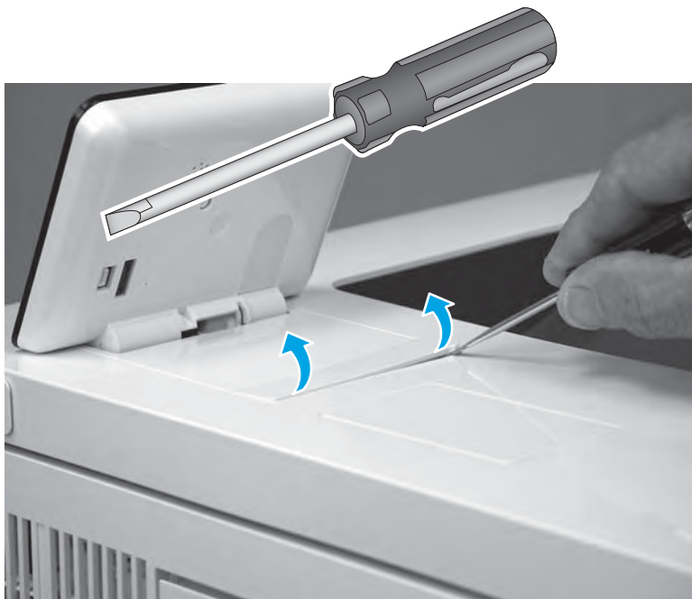
Figure 1-1006 Release the control-panel screws cover tabs
