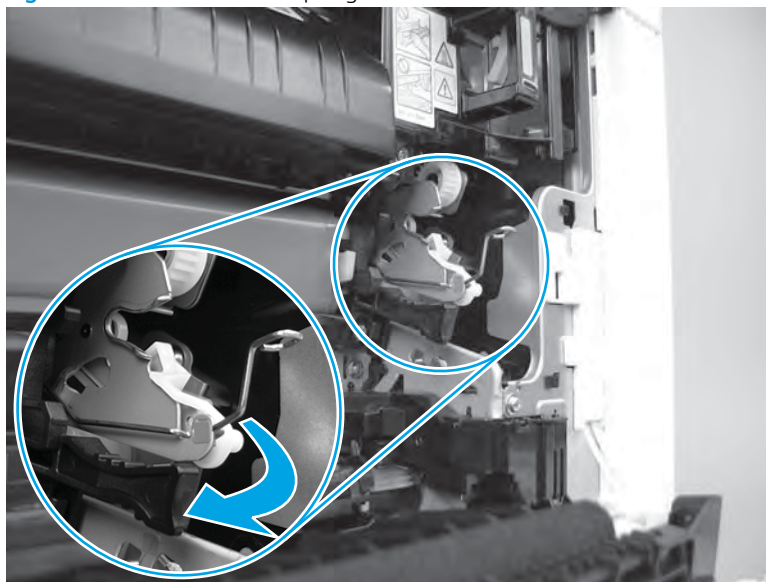
Figure 1-243 Remove the spring from the holder
