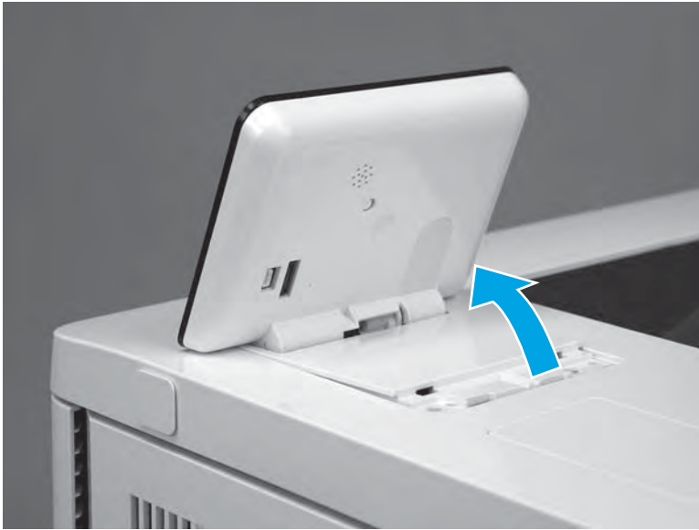
Figure 1-2936 Rotate the control-panel base up
