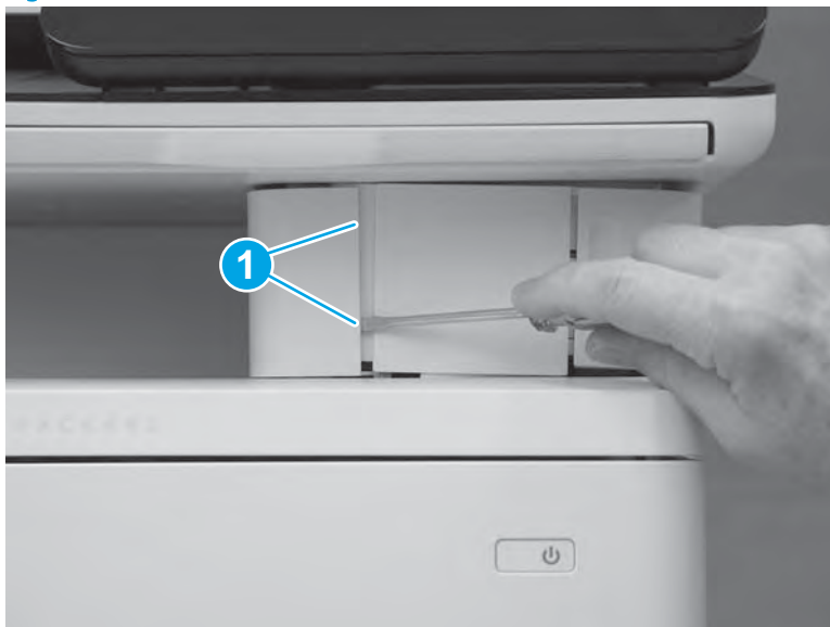
Figure 1-3775 Release two tabs
