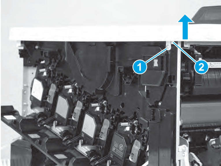
Figure 1-681 Remove one screw and release one tab
