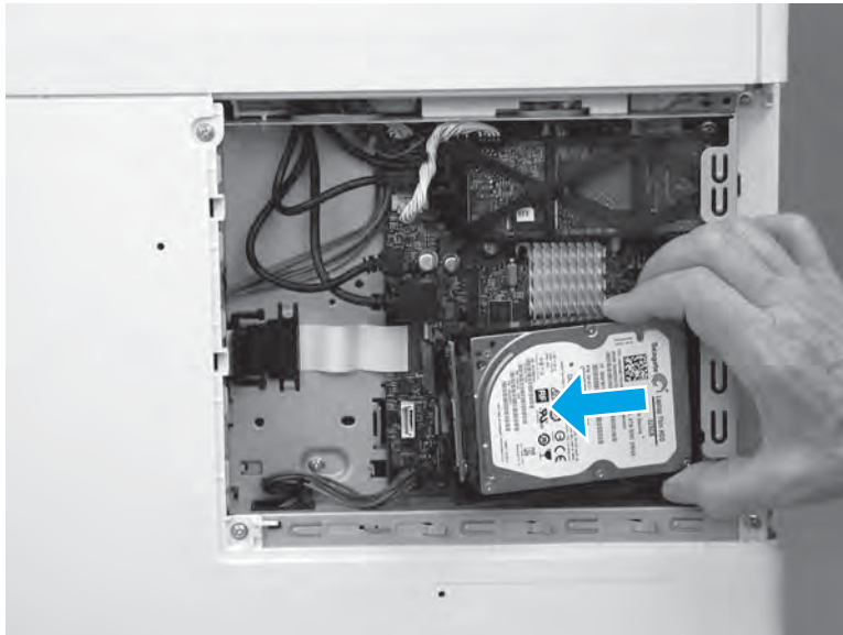
Figure 1-4679 Remove the HDD
