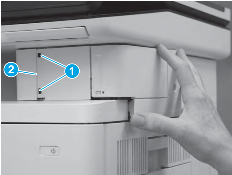
Figure 1-2042 Install two tabs
