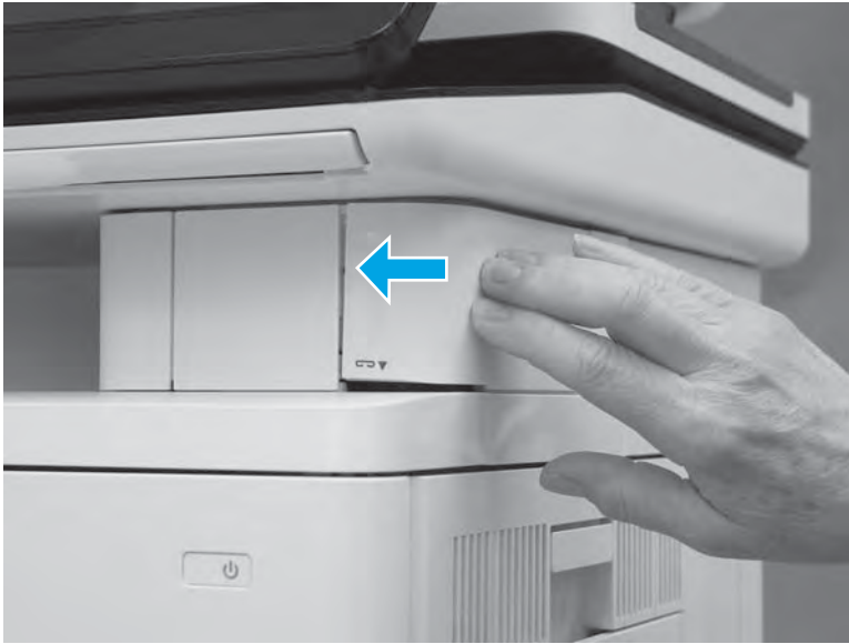
Figure 1-4356 Install the cover assembly
