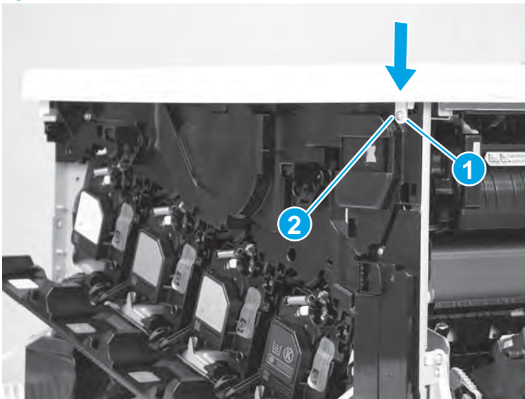
Figure 1-1511 Engage one tab and install one screw
