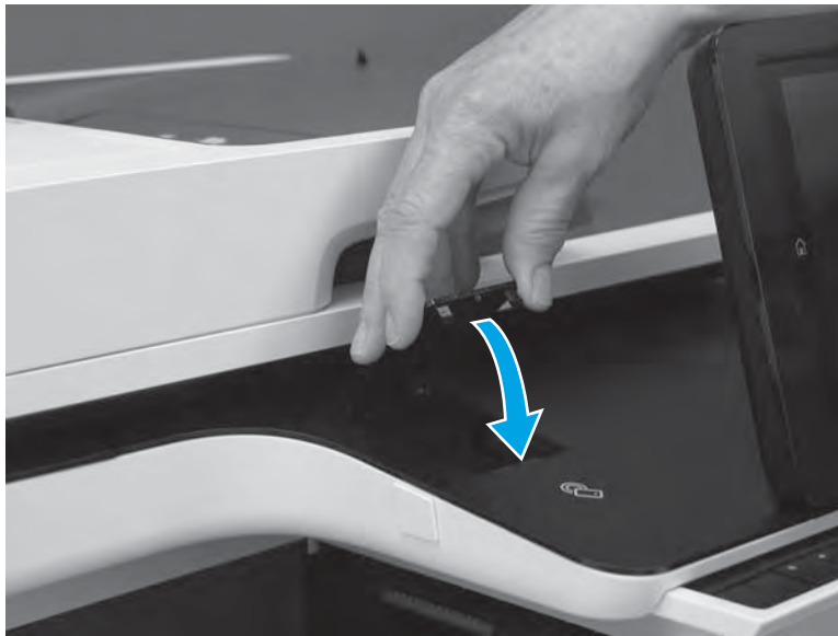
Figure 1-111 Rotate the cover down
