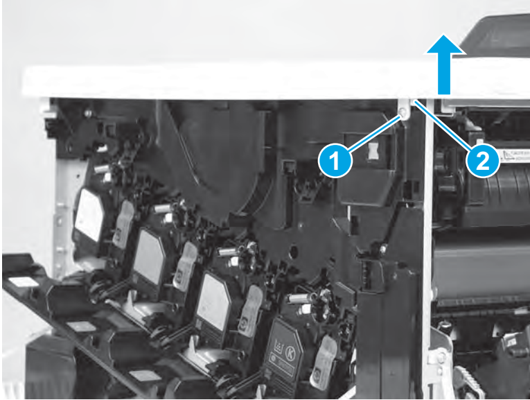
Figure 1-3792 Remove one screw and release one tab
